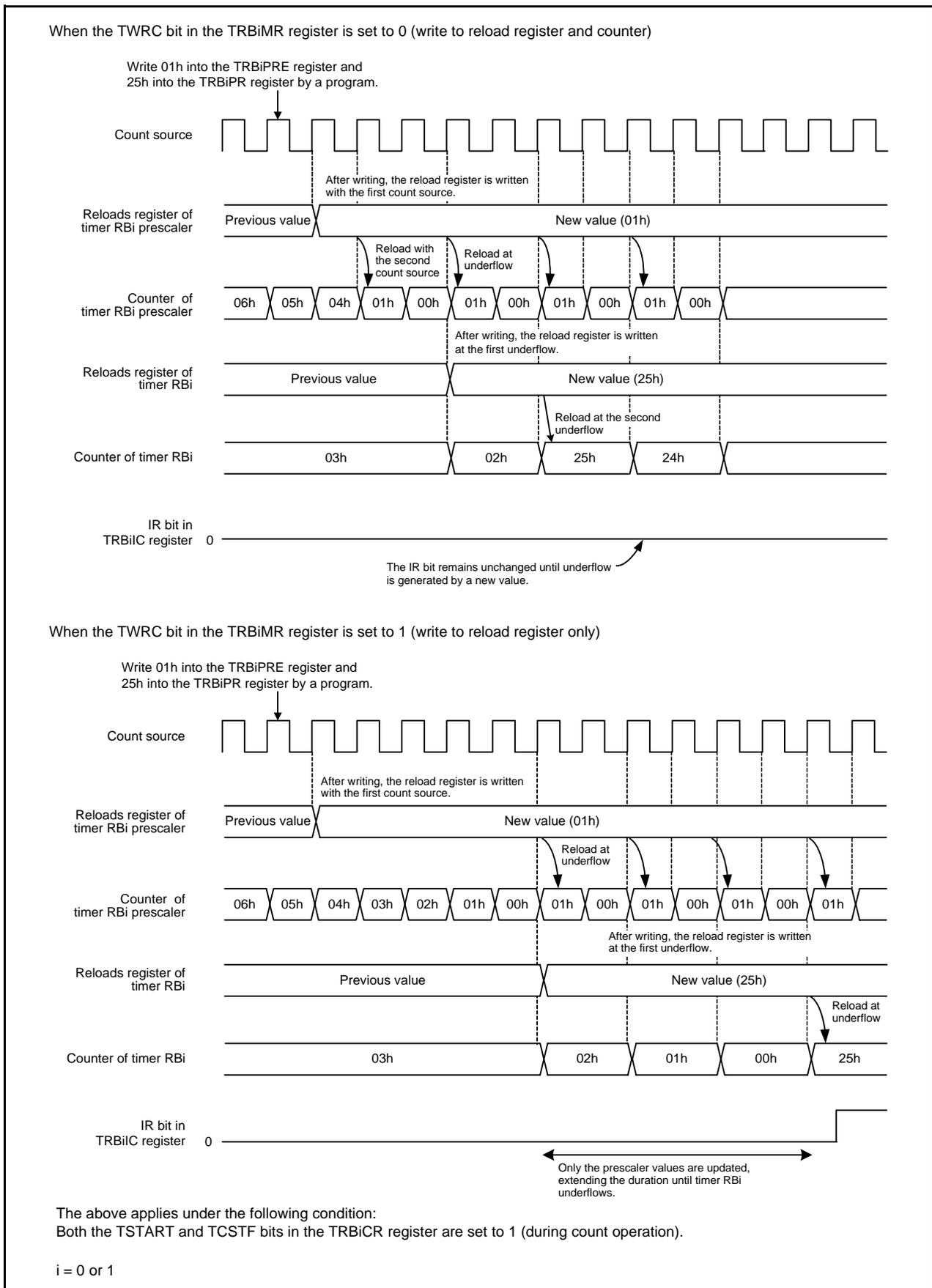
**Figure 17.2 Operating Example of Timer RBi when Counter Value is Rewritten during Count Operation**
