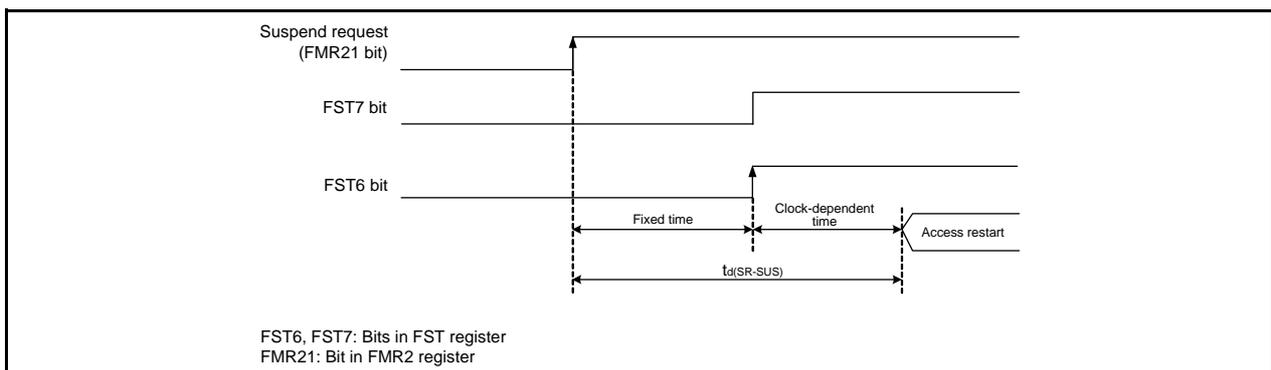
**Figure 25.2 Time delay until Suspend**
