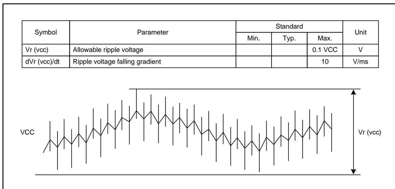
Figure 26.2 Definition of Ripple Voltage
