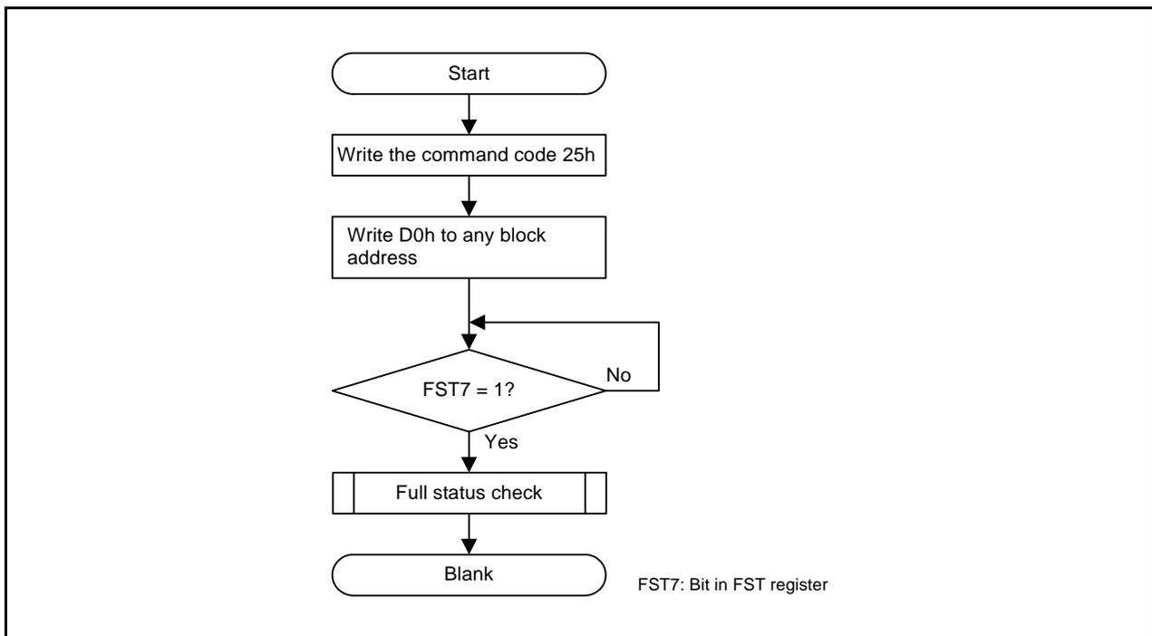
**Figure 24.19** Block Blank Check Flowchart
