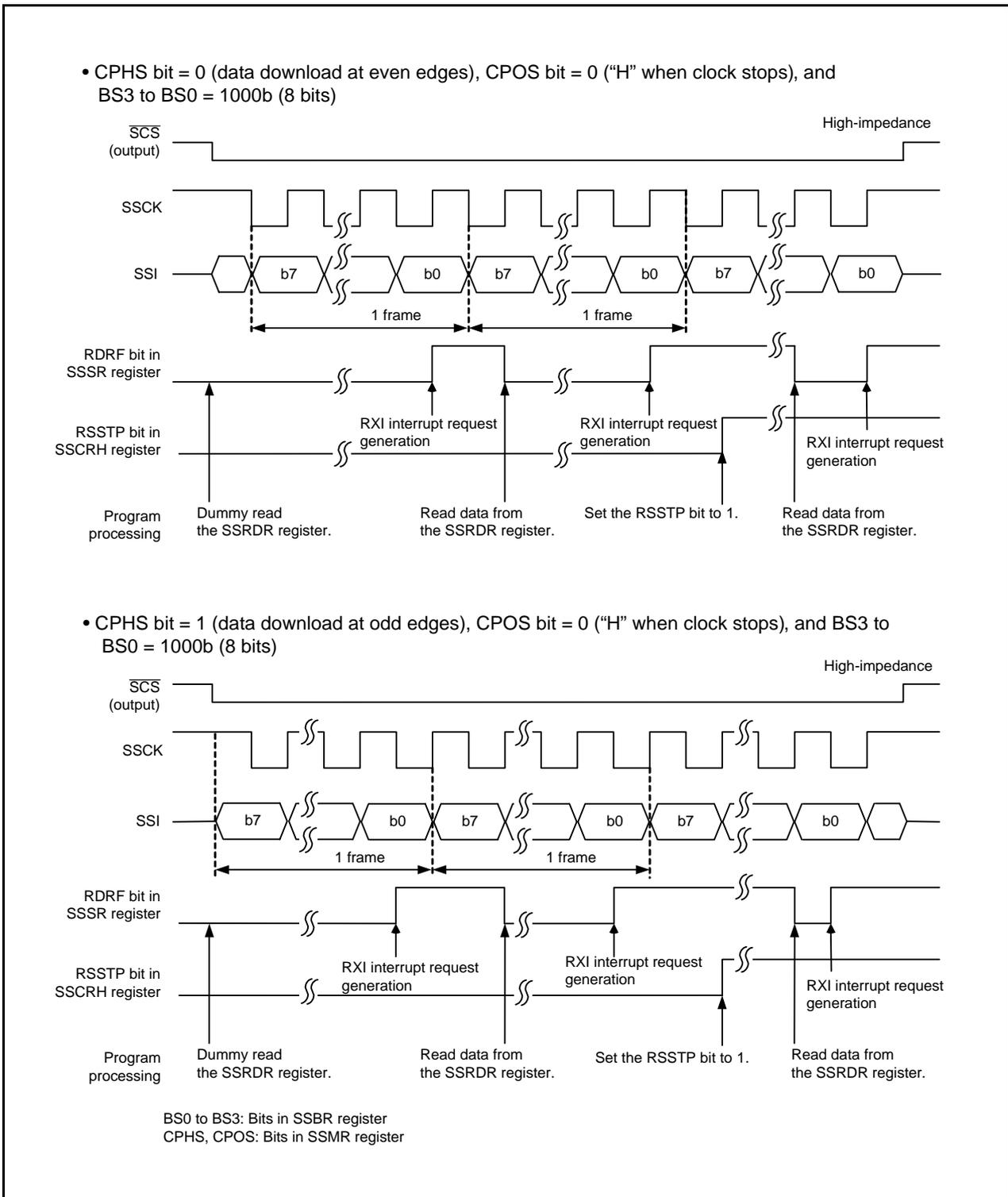
**Figure 22.12 Example of Synchronous Serial Communication Unit Operation during Data Reception (4-Wire Bus Communication Mode, 8-Bit SSU Data Transfer Length)**
