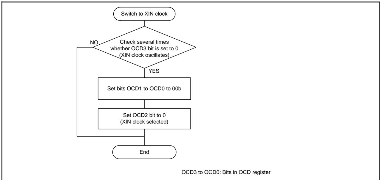
**Figure 9.4 Procedure for Switching to XIN Clock when XIN Clock Re-Oscillates after Oscillation Stop is Detected**
