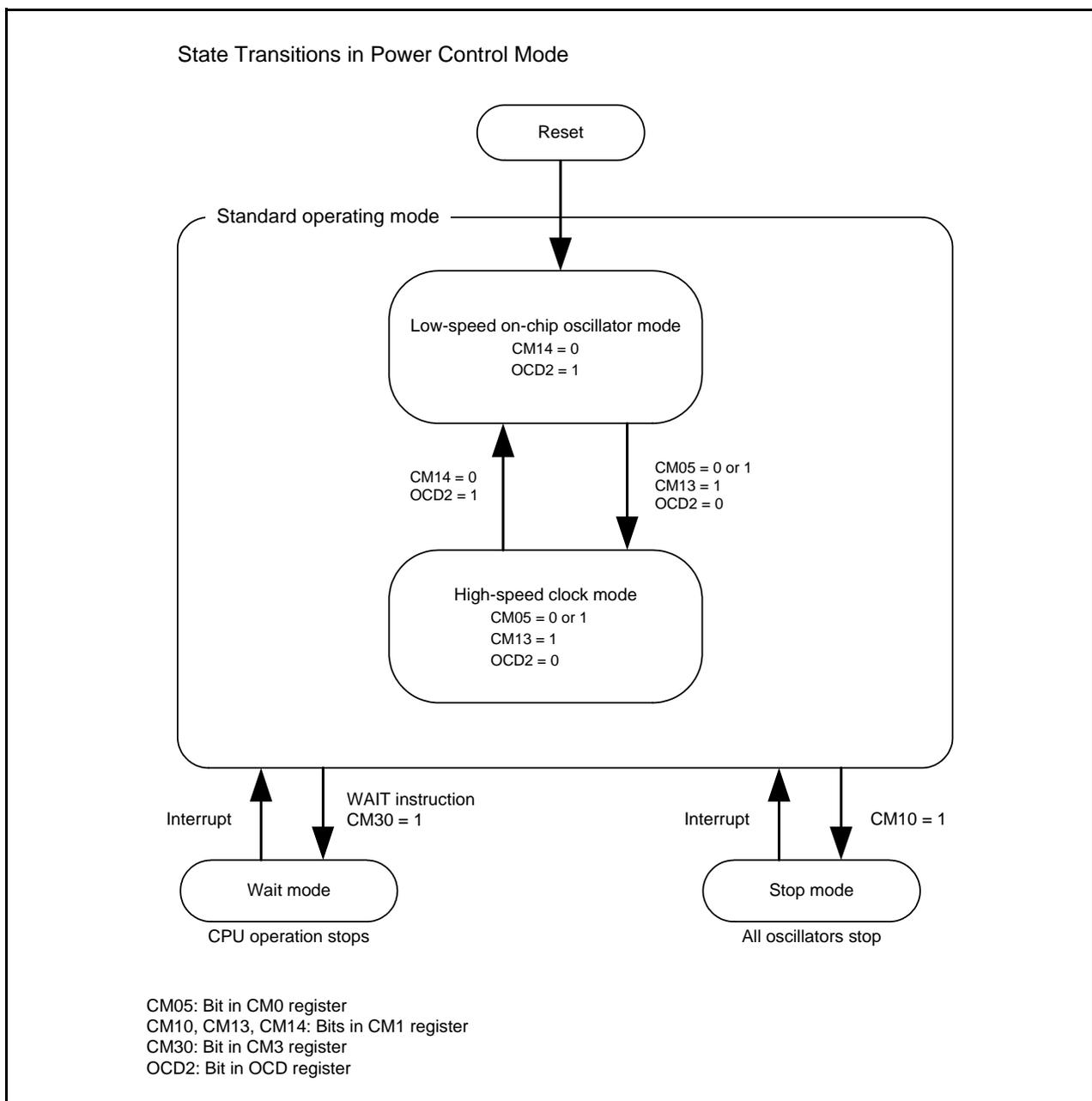
**Figure 10.1 State Transitions in Power Control Mode**
