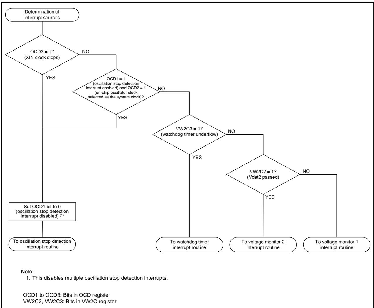
**Figure 9.5 Example of Determining Interrupt Sources for Oscillation Stop Detection, Watchdog Timer, Voltage Monitor 1, or Voltage Monitor 2 Interrupt**
