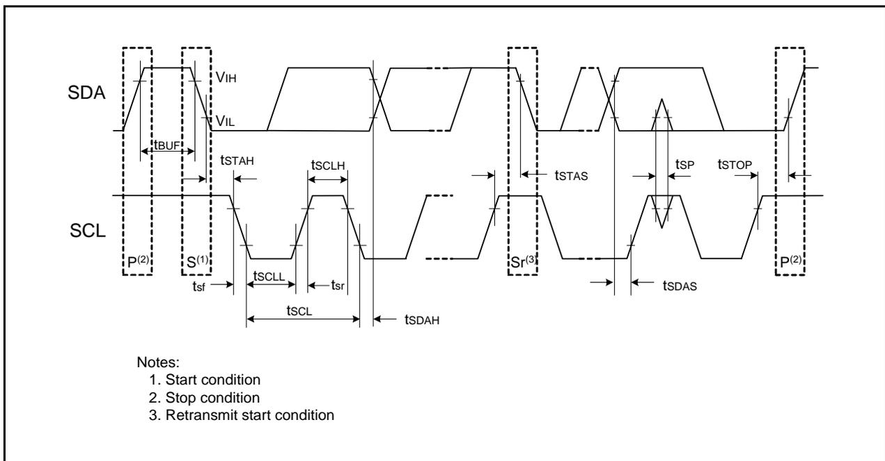
**Figure 25.7 I/O Timing of I<sup>2</sup>C bus Interface**
