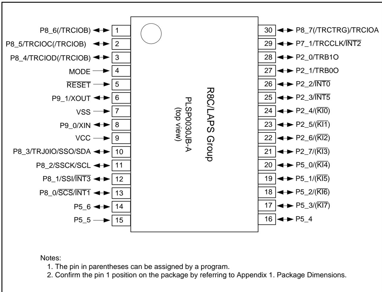
Figure 1.3 Pin Assignment (Top View) of PLSP0030JB-A Package
