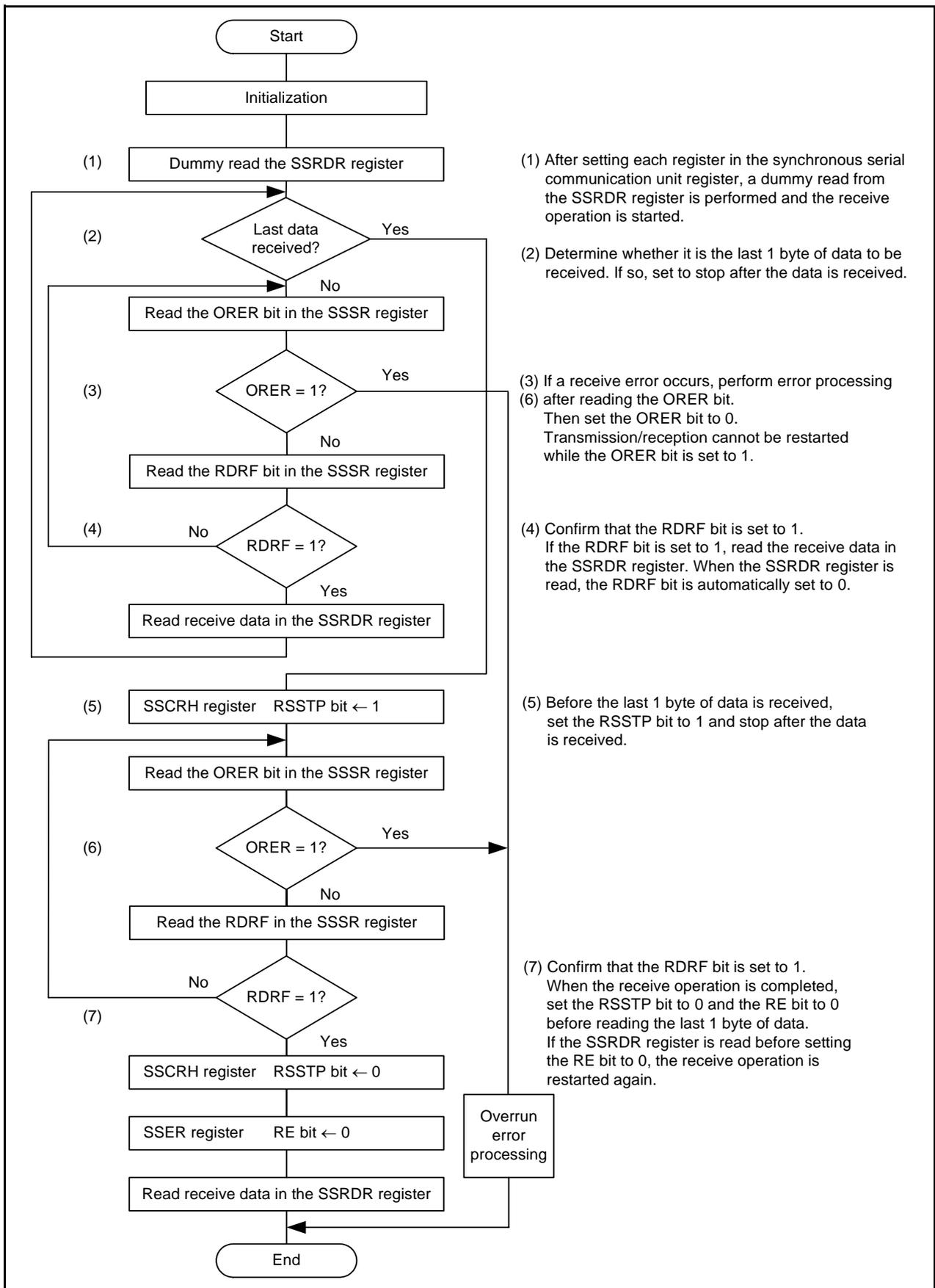
Figure 22.8 Sample Flowchart of Data Reception (MSS = 1) (Clock Synchronous Communication Mode)
