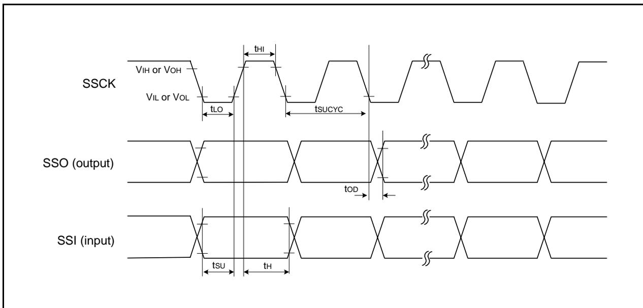
**Figure 25.6 I/O Timing of Synchronous Serial Communication Unit (SSU) (Clock Synchronous Communication Mode)**
