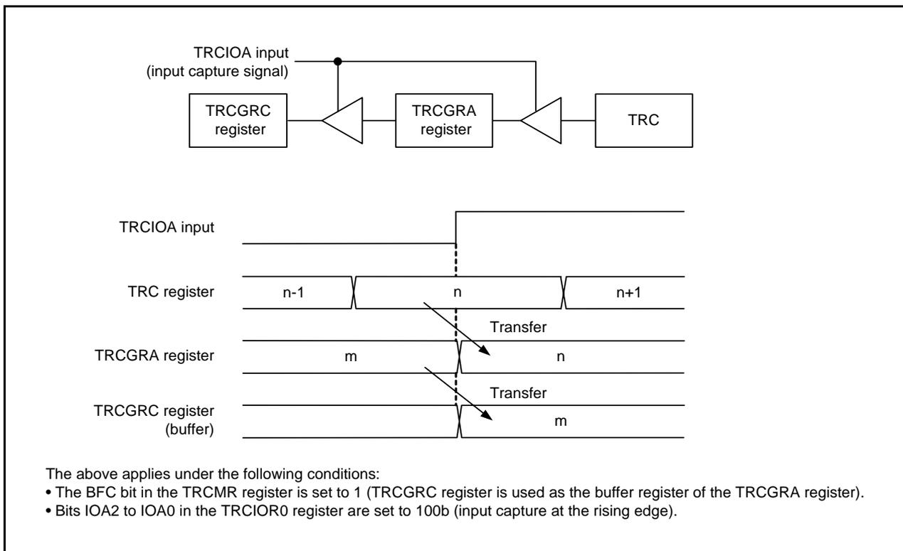
**Figure 18.3 Buffer Operation of Input Capture Function**
