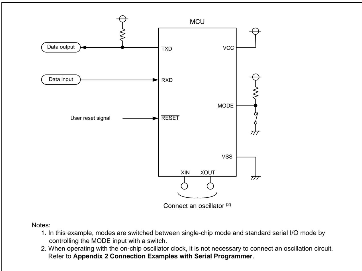
**Figure 24.21 Pin Handling in Standard Serial I/O Mode 2**
