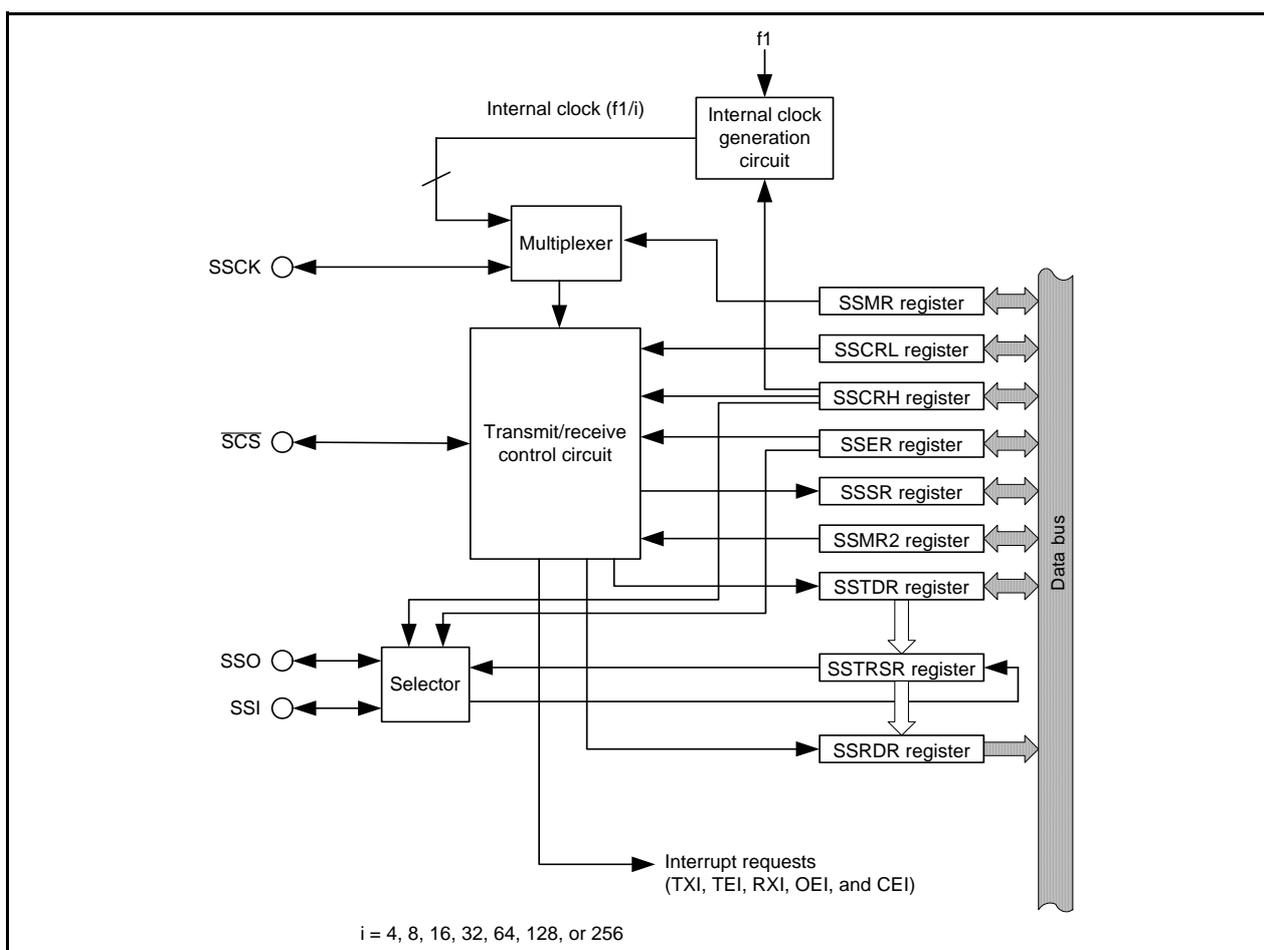
Figure 22.1 Block Diagram of Synchronous Serial Communication Unit
