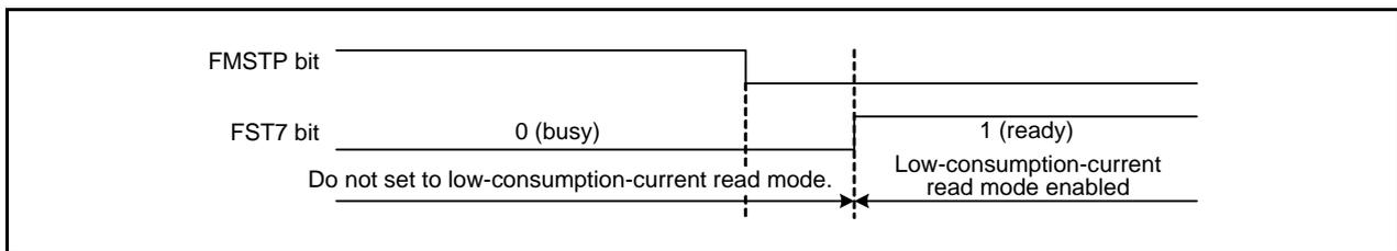
Figure 24.3 Transition to Low-Current-Consumption Read Mode
