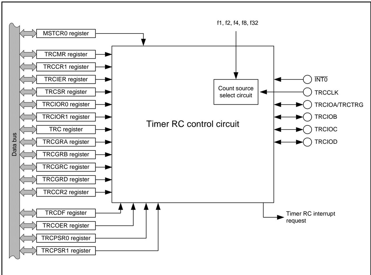
Figure 18.1 Timer RC Block Diagram
