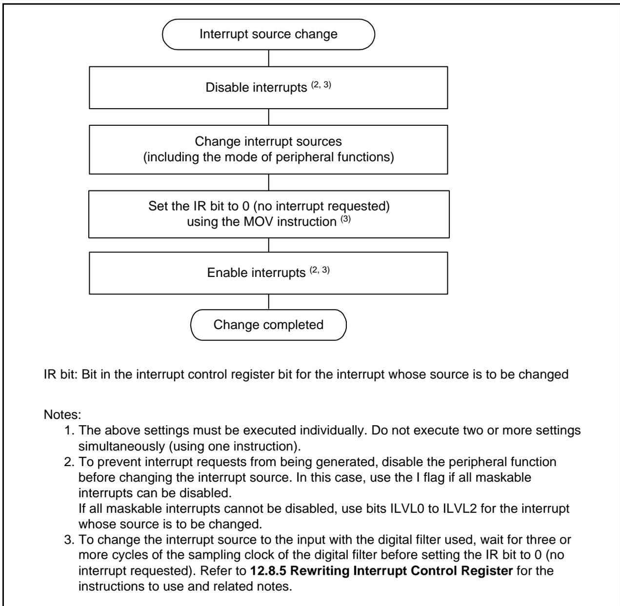
Figure 26.1 Procedure Example for Changing Interrupt Sources
