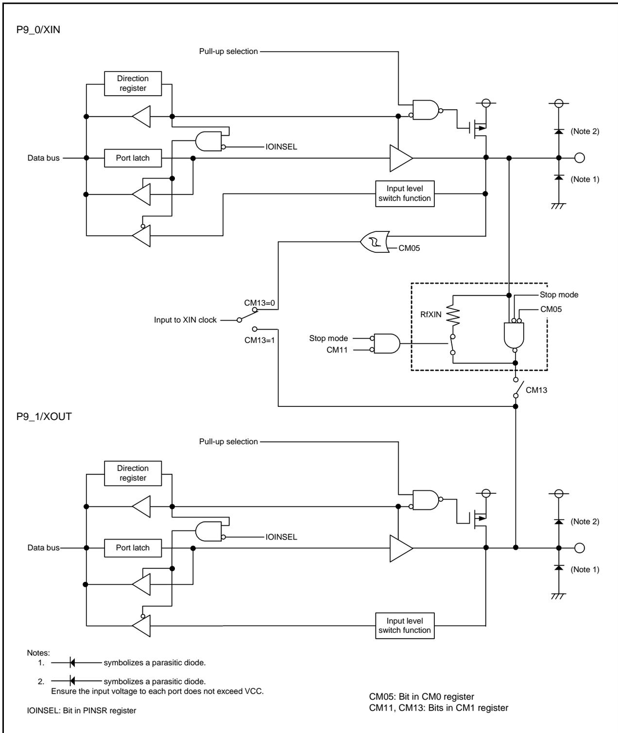
Figure 7.4 I/O Port Configuration (4)
