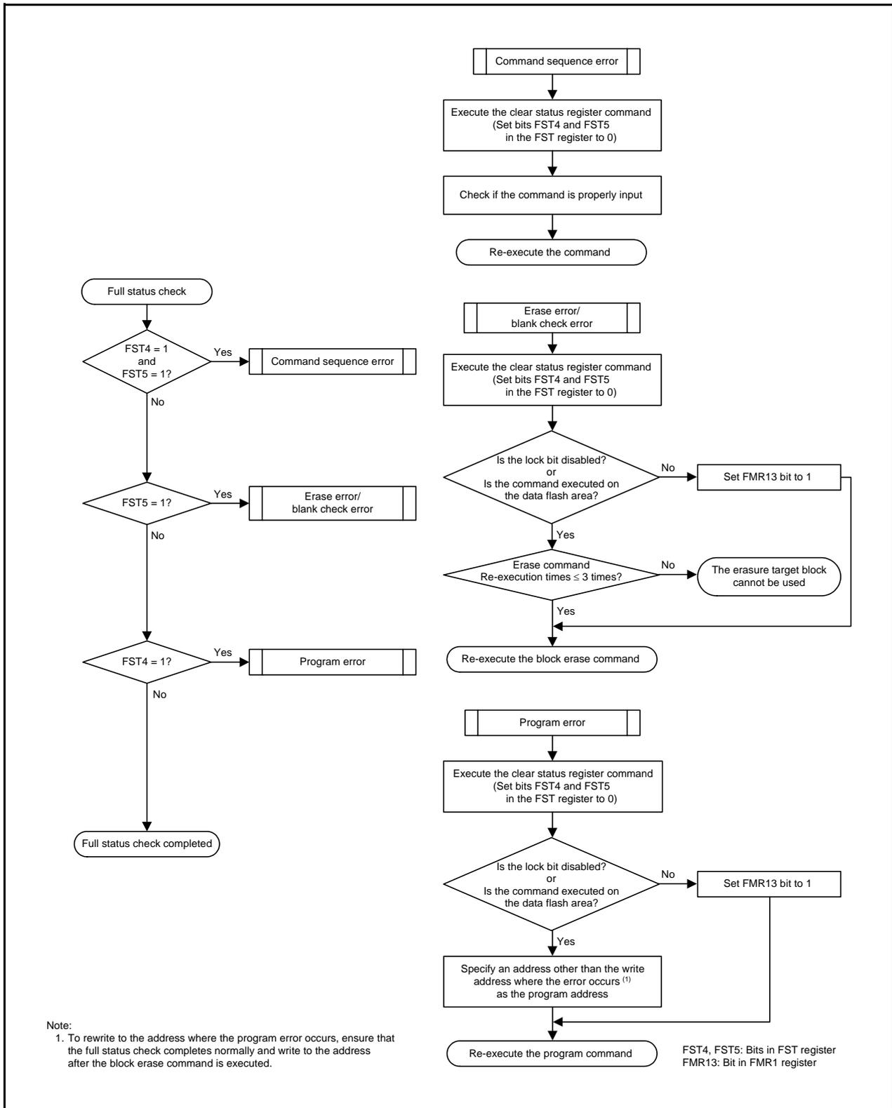
Figure 24.20 Full Status Check and Handling Procedure for Individual Errors
