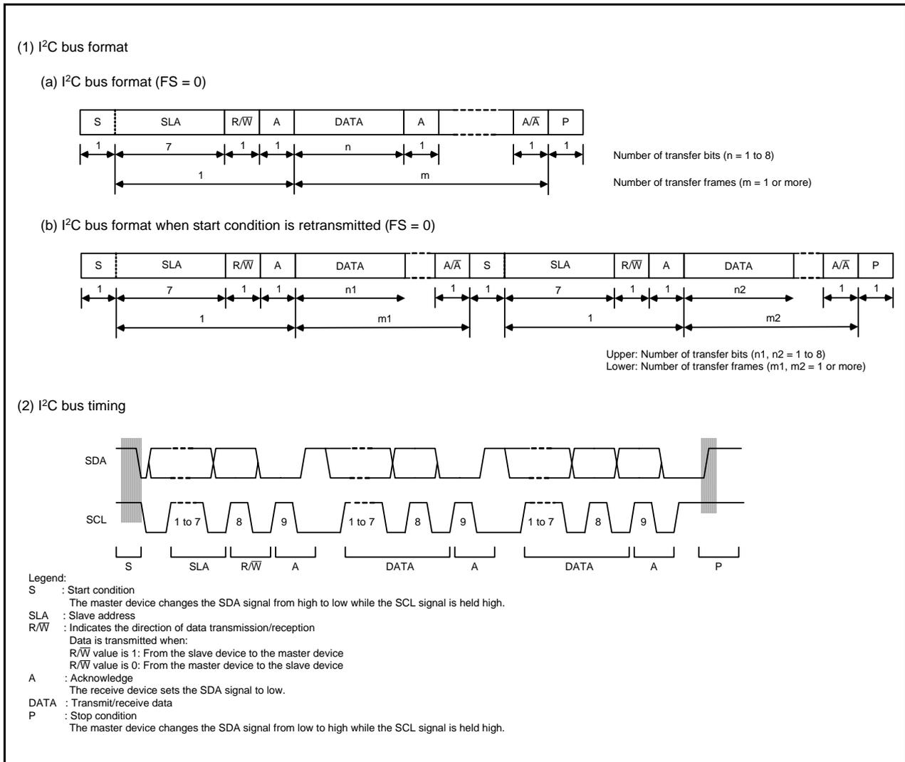
Figure 23.4 I<sup>2</sup>C bus Format and Bus Timing
