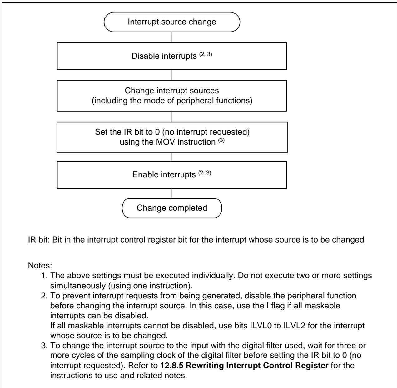
Figure 12.12 Procedure Example for Changing Interrupt Sources
