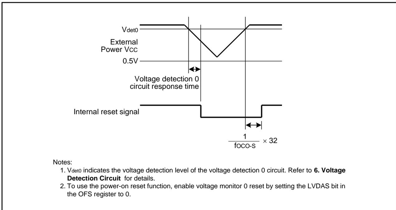
Figure 5.7 Example of Voltage Monitor 0 Reset Circuit and Operation
