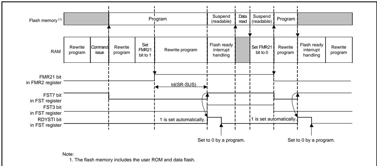
Figure 24.5 Program-Suspend Operation Timing in EW0 Mode
