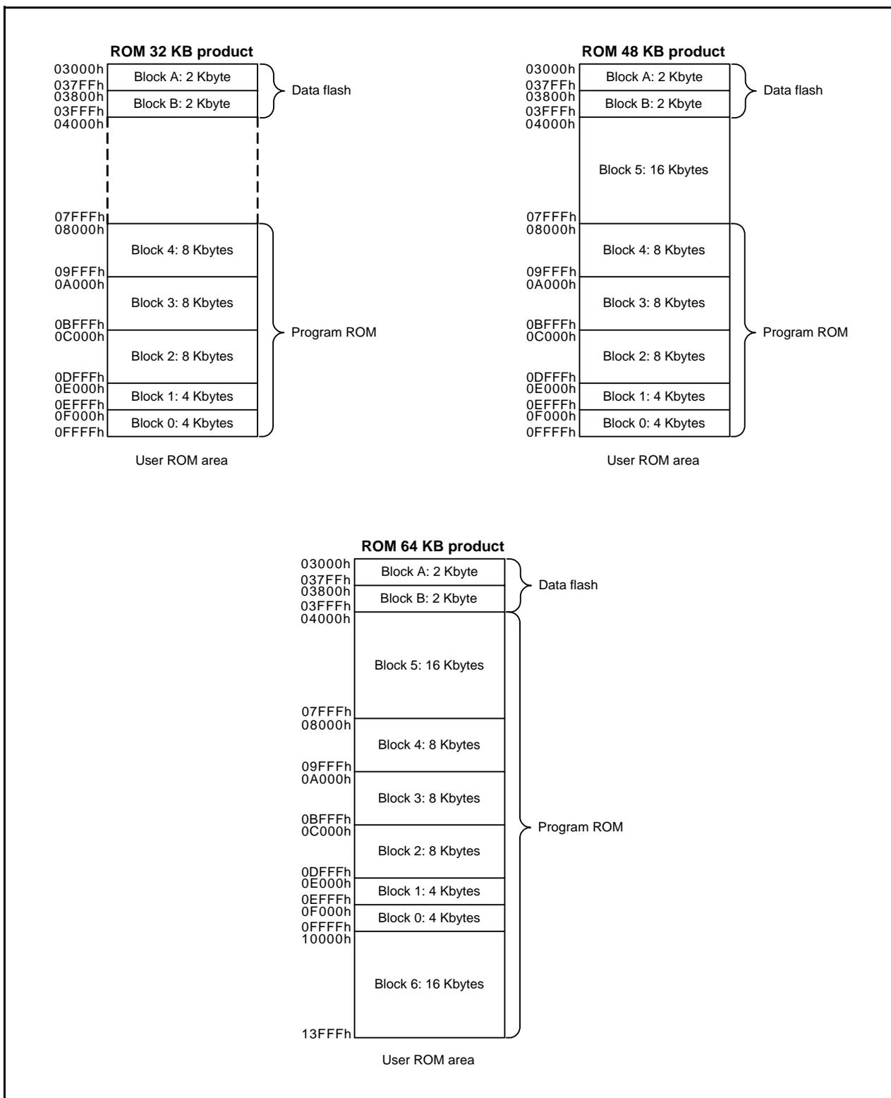
Figure 24.1 Flash Memory Block Diagrams of R8C/LAPS Group (1)
