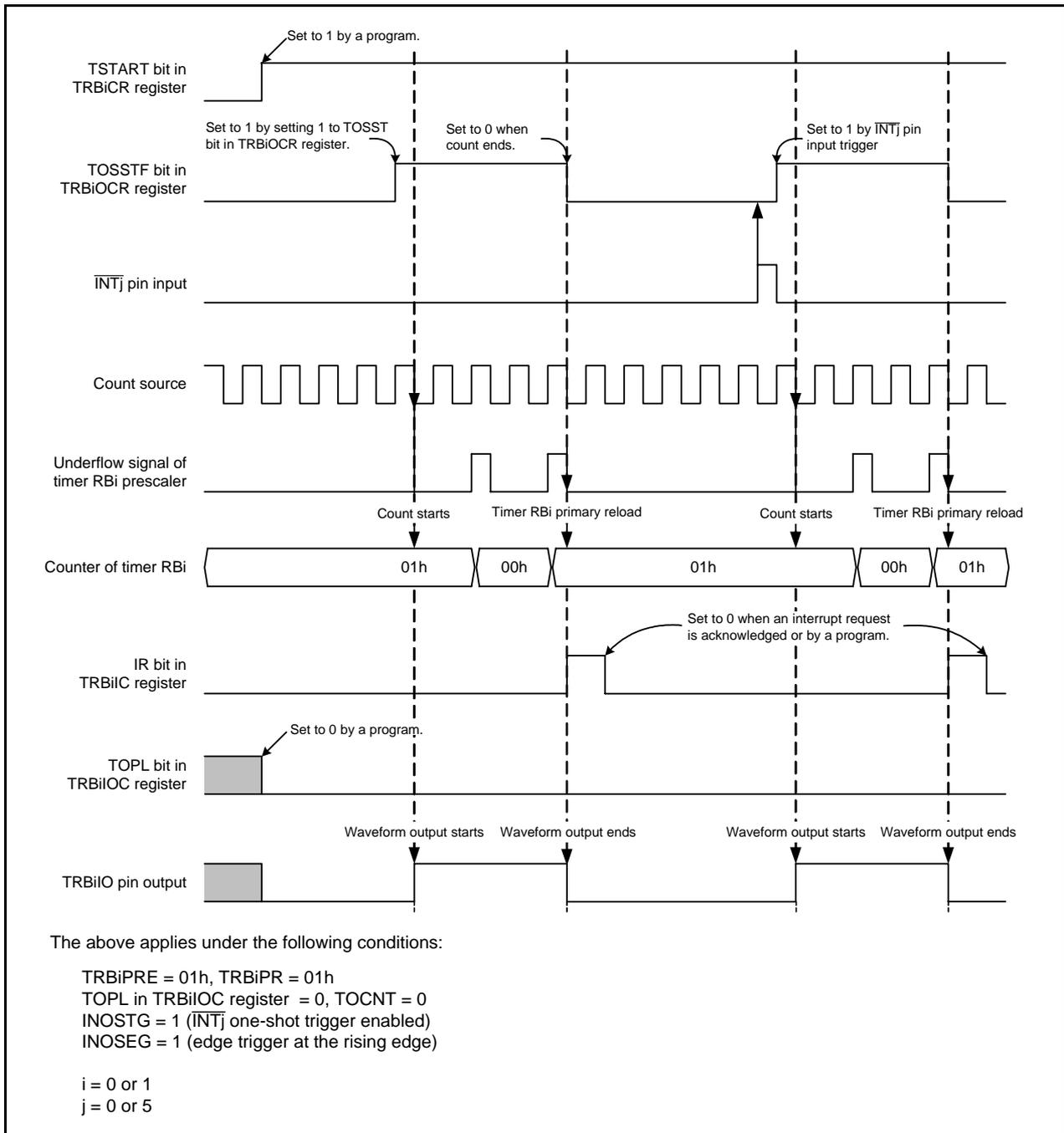
Figure 17.4 Operating Example in Programmable One-Shot Generation Mode
