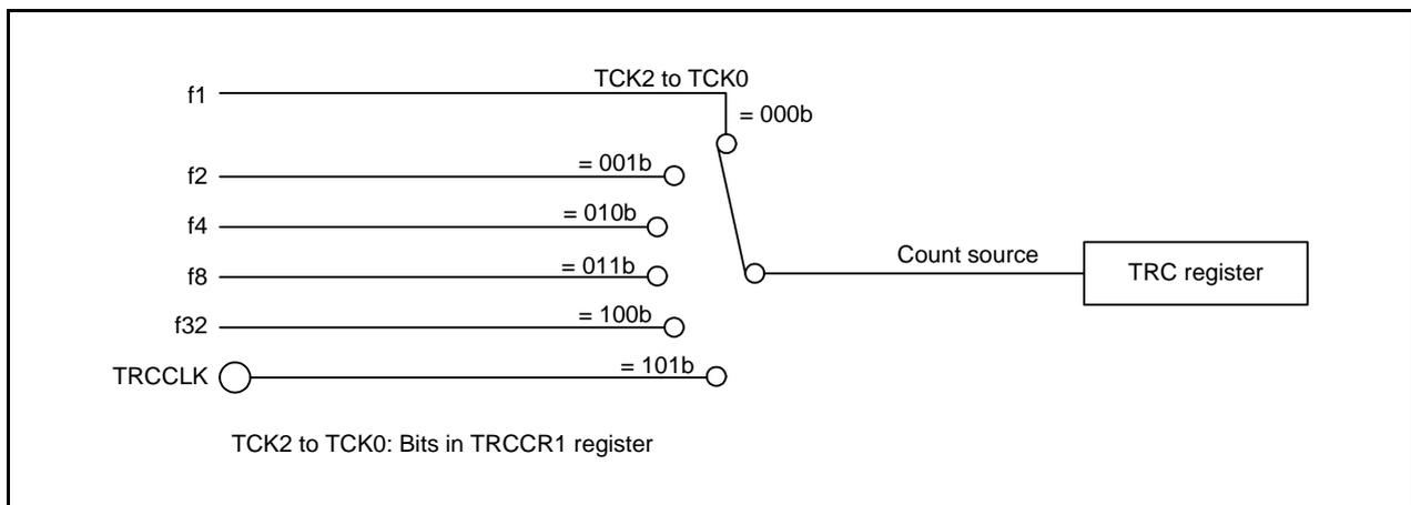
**Figure 18.2 Count Source Block Diagram**
