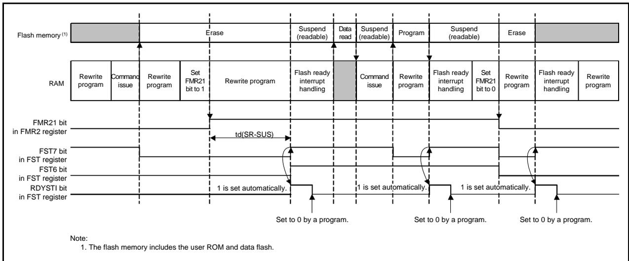
Figure 24.4 Erase-Suspend Operation Timing in EW0 Mode
