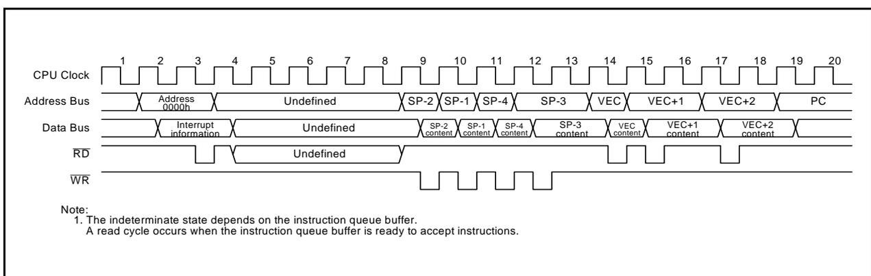
**Figure 12.3 Time Required for Executing Interrupt Sequence**
