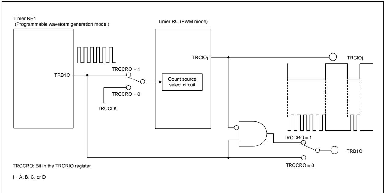
Figure 20.1 Block Diagram of Remote Control Carrier Wave Output Function
