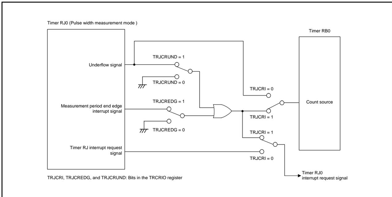
Figure 20.3 Block Diagram of Remote Control Carrier Wave Input Function
