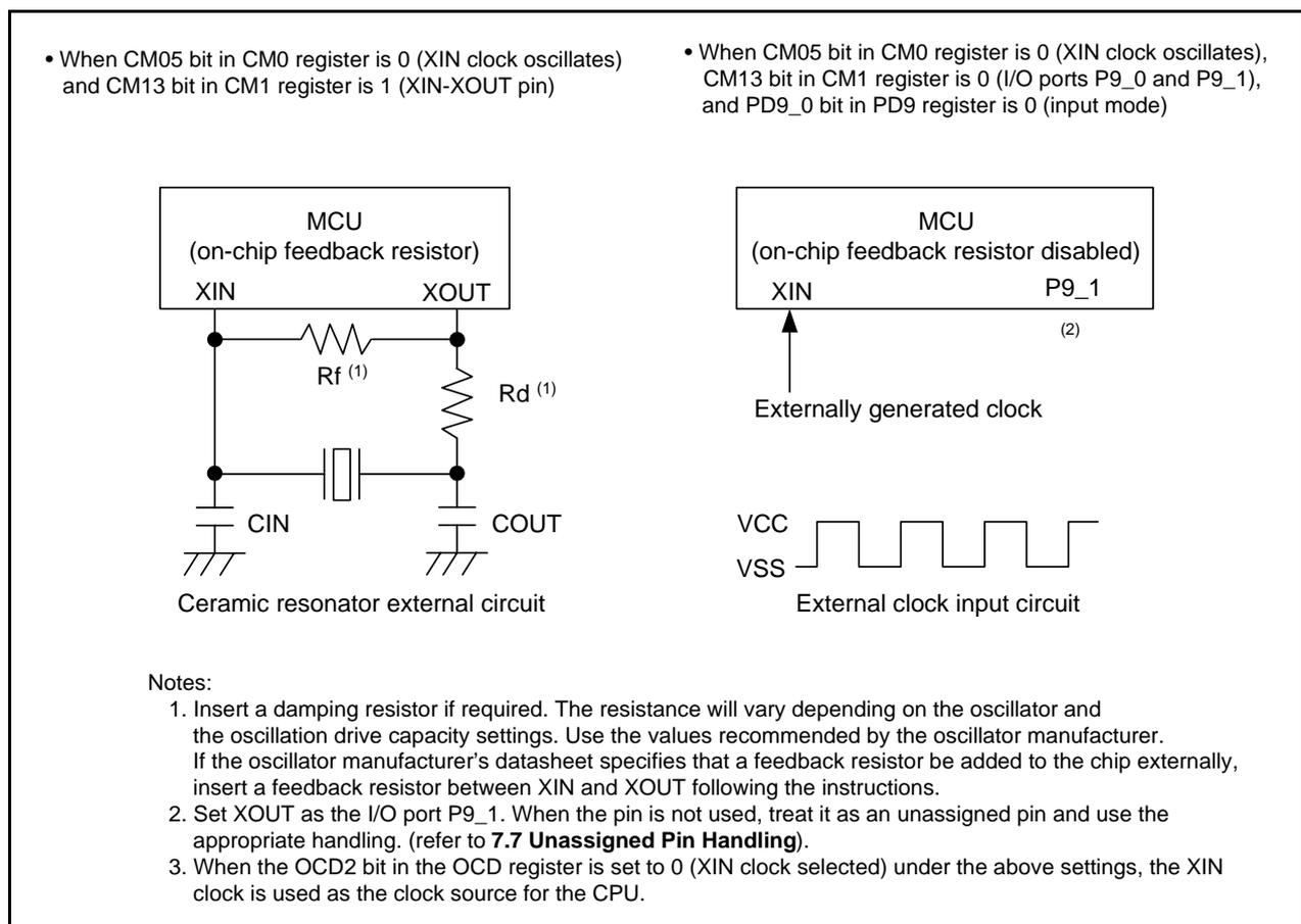
**Figure 9.3** Examples of XIN Clock Connection Circuit
