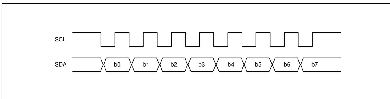
Figure 23.13 Transfer Format of Clock Synchronous Serial Format
