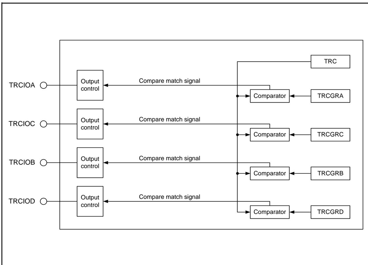
Figure 18.9 Block Diagram of Output Compare Function
