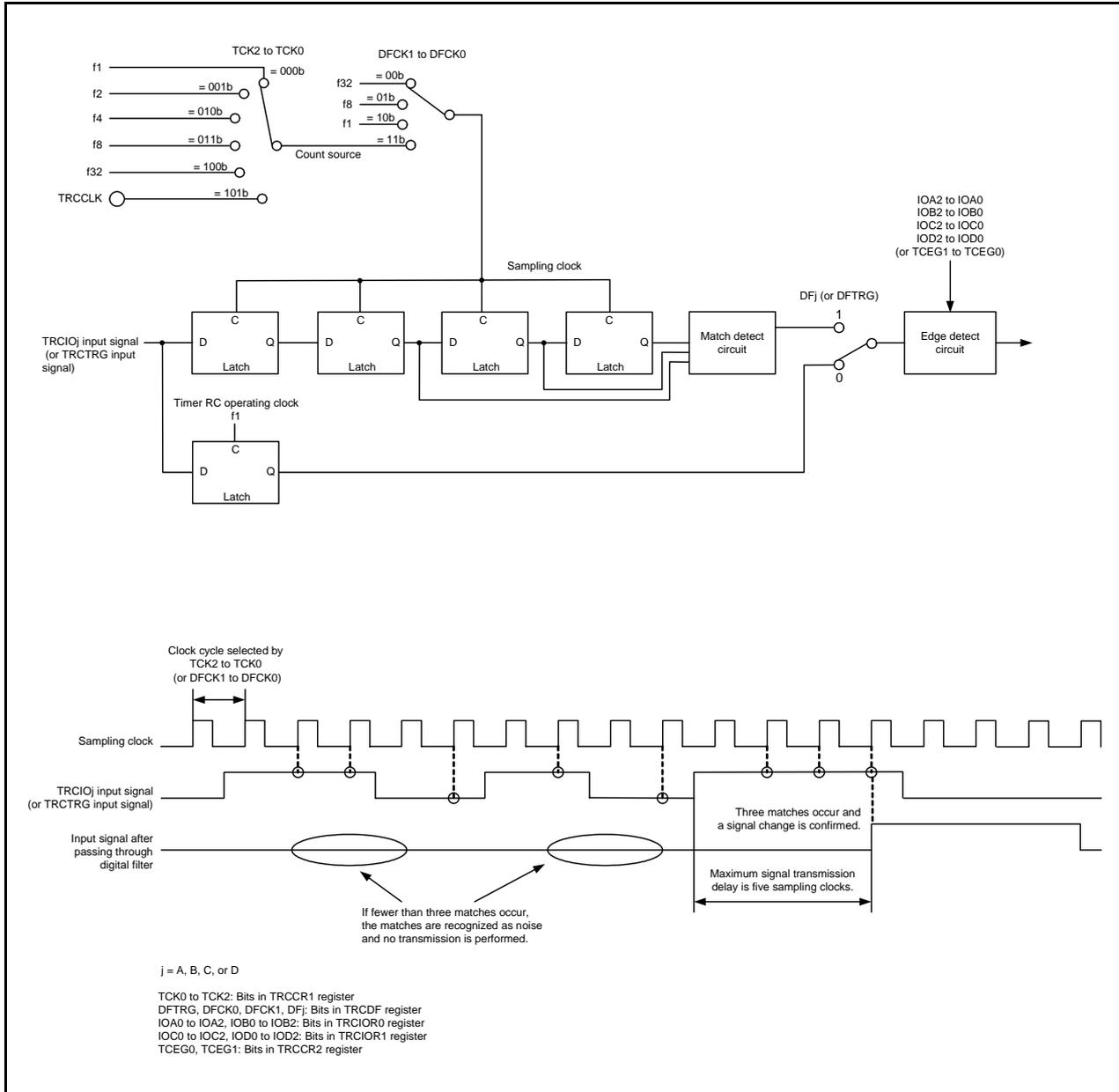
**Figure 18.5** Block Diagram of Digital Filter
