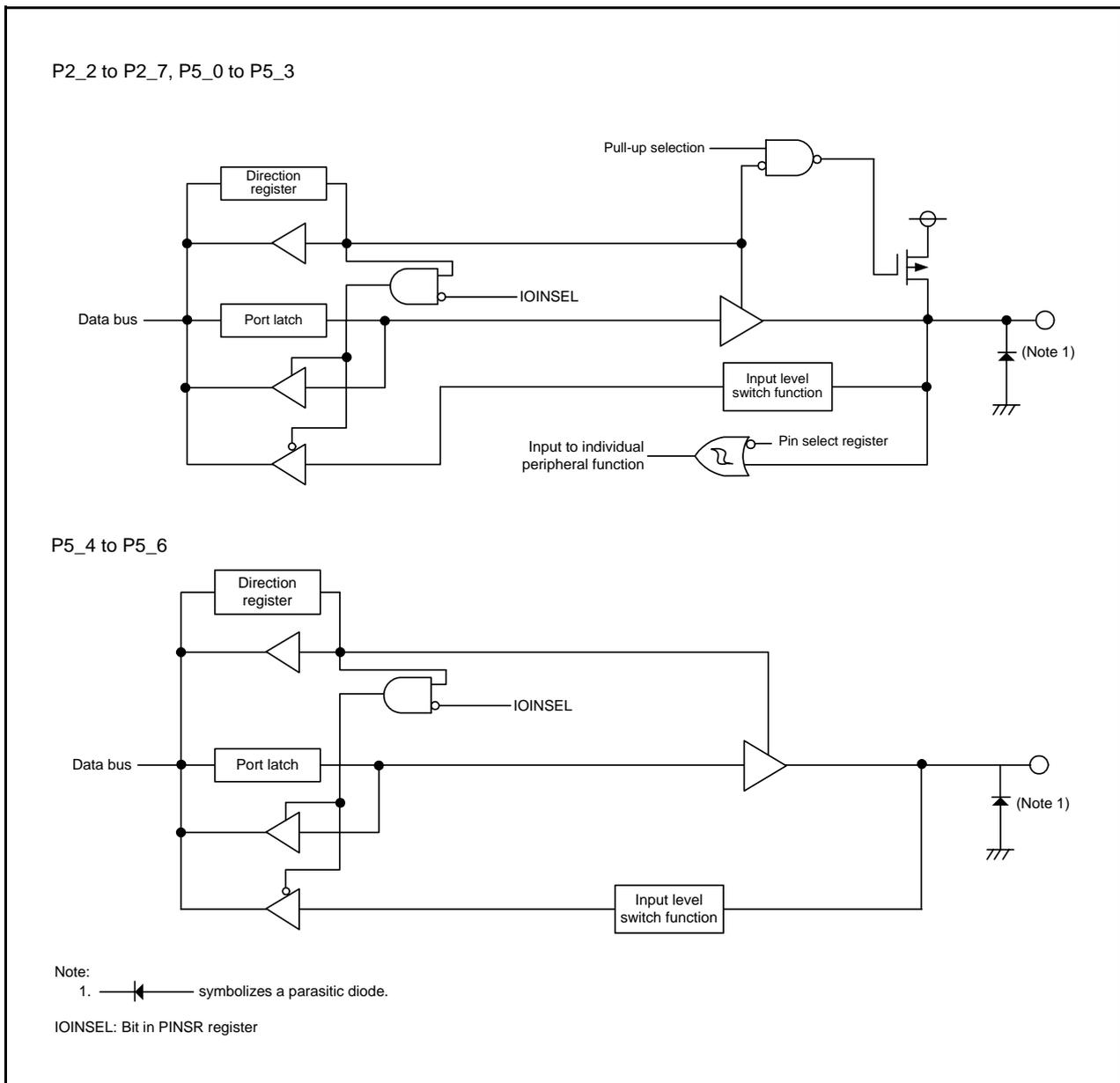
Figure 7.2 I/O Port Configuration (2)
