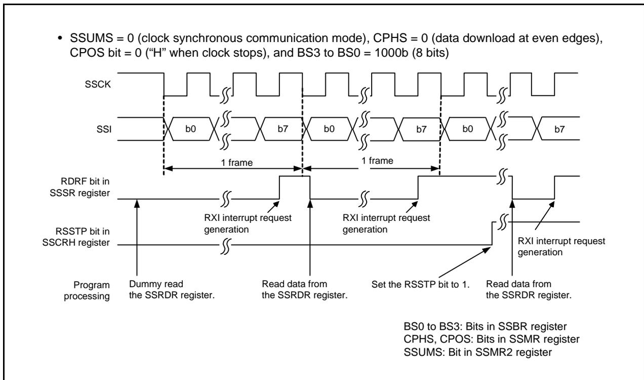
**Figure 22.7 Example of Synchronous Serial Communication Unit Operation during Data Reception (Clock Synchronous Communication Mode, 8-Bit SSU Data Transfer Length)**
