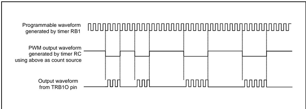
Figure 20.2 Waveform during Operation of Remote Control Carrier Wave Output Function
