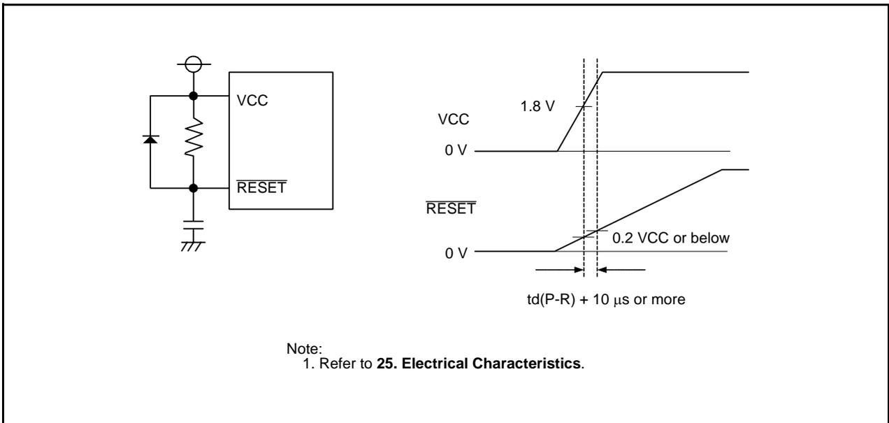
Figure 5.4 Example of Hardware Reset Circuit and Operation
