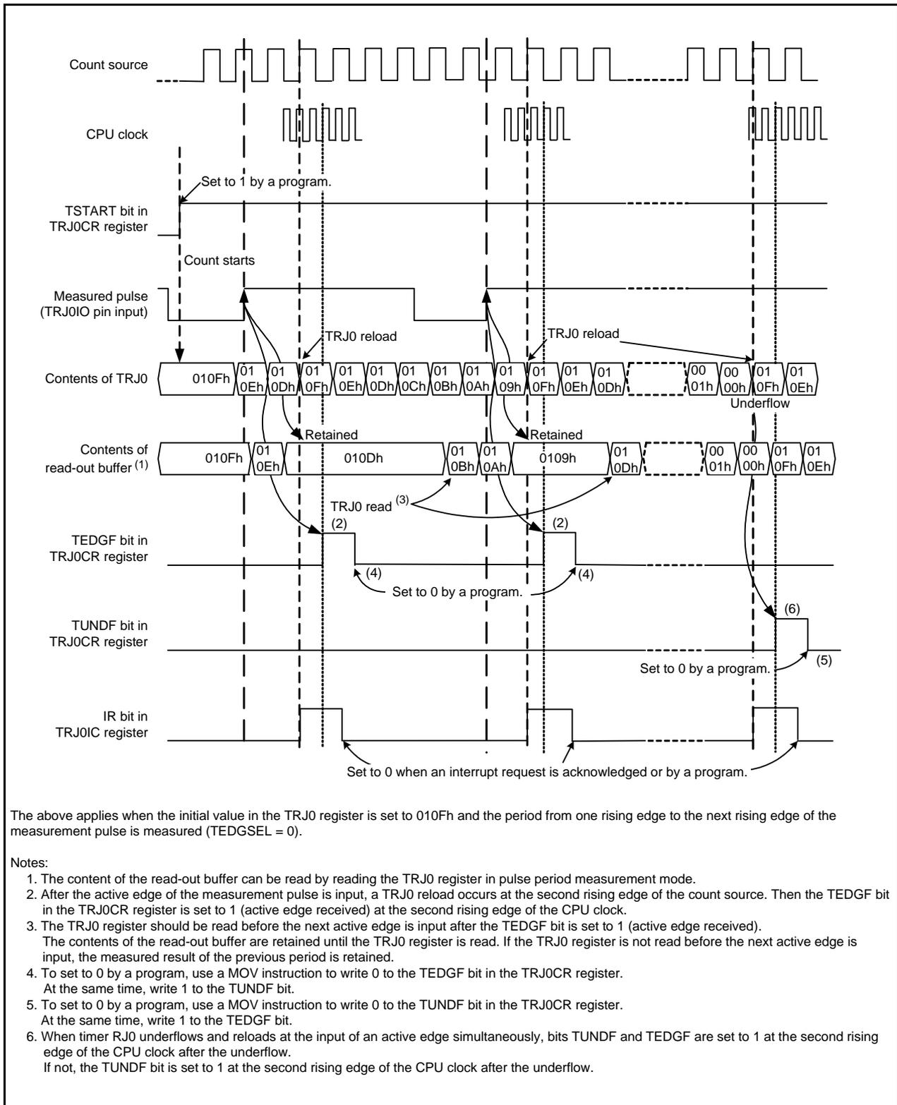
Figure 19.4 Operating Example in Pulse Period Measurement Mode
