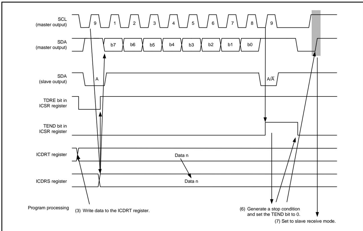
Figure 23.6 Operating Timing in Master Transmit Mode (I<sup>2</sup>C bus Interface Mode) (2)
