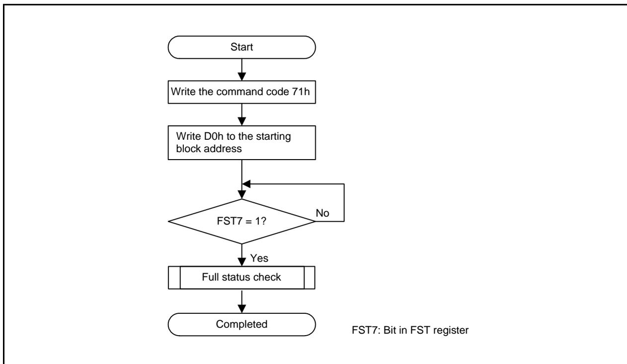
Figure 24.18 Read Lock Bit Status Flowchart
