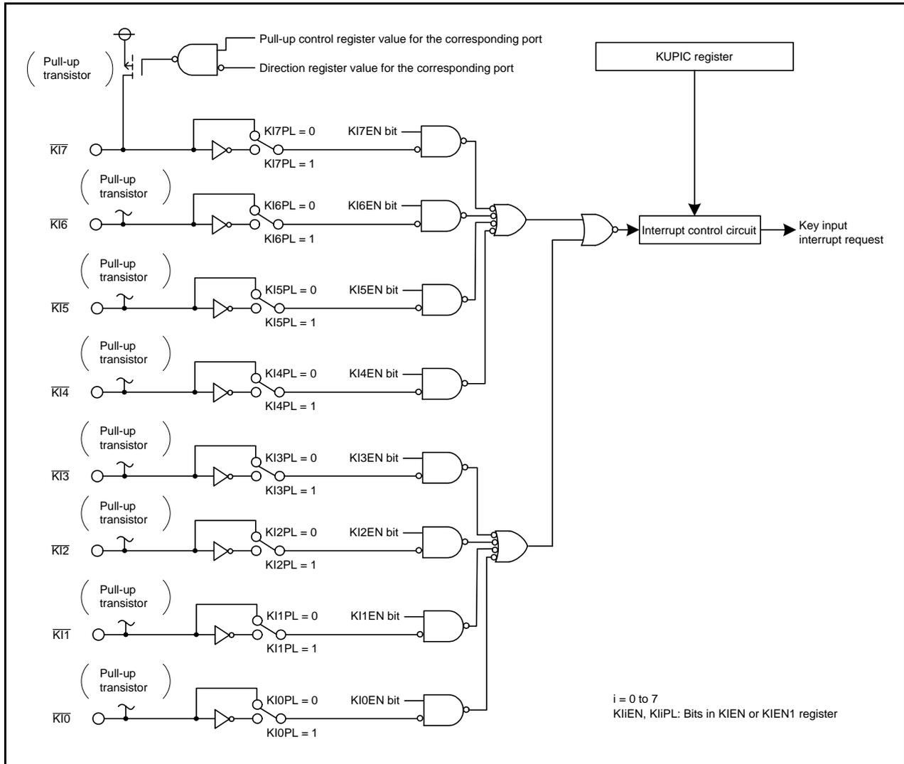
Figure 12.11 Block Diagram of Key Input Interrupt
