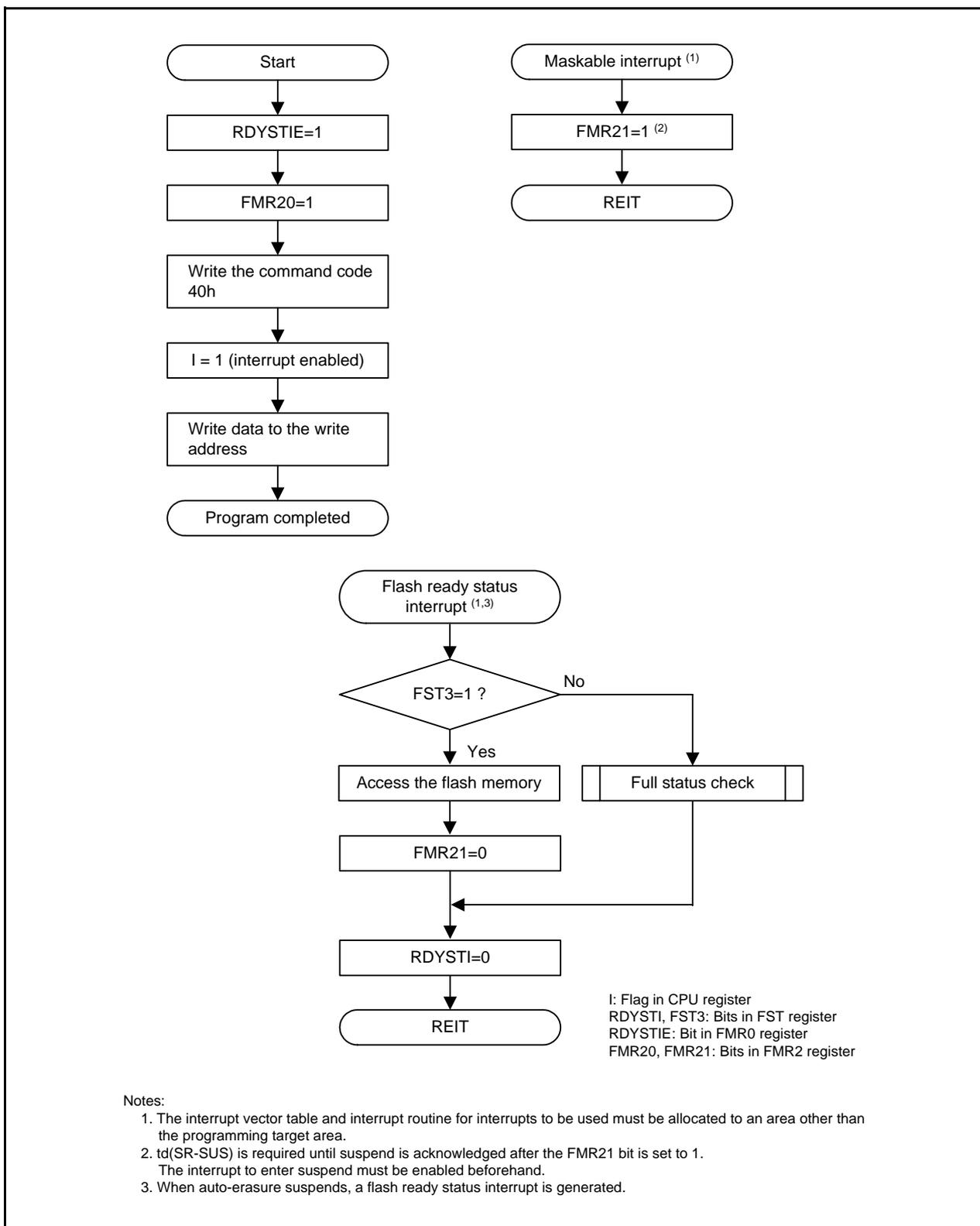
Figure 24.11 Program Flowchart in EW0 Mode (Flash Ready Status Interrupt Enabled and Suspend Enabled)
