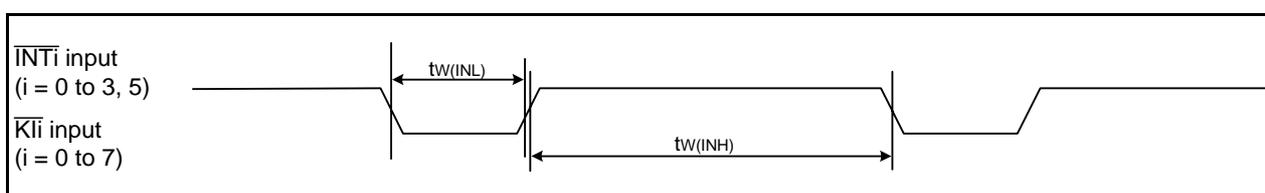
**Figure 25.10 Input Timing of External Interrupt  $\overline{\text{INT}}_i$  and Key Input Interrupt  $\overline{\text{KI}}_i$**
