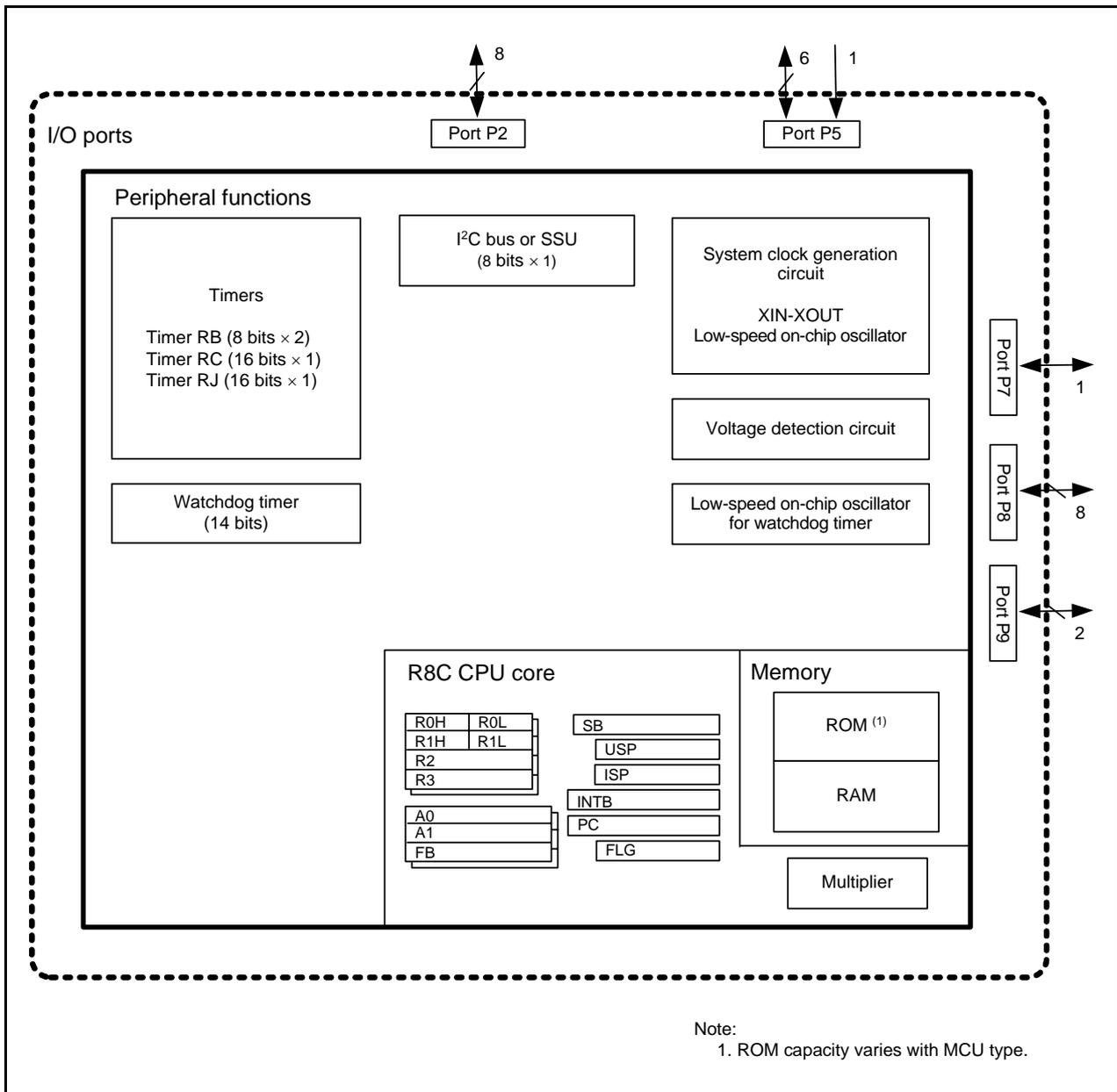
Figure 1.2 Block Diagram of R8C/LAPS Group
