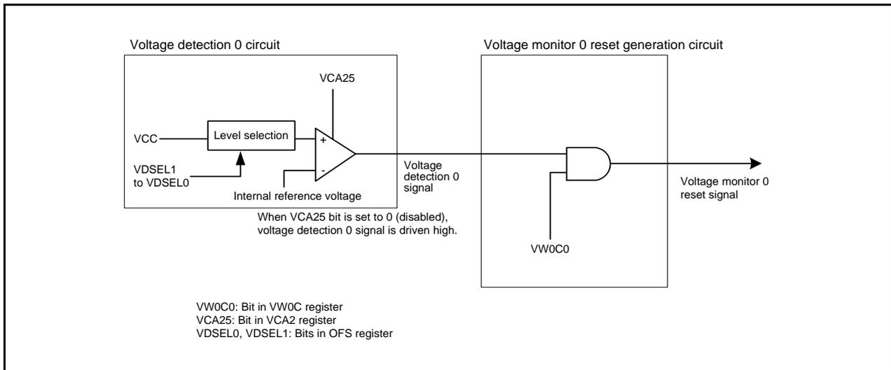
Figure 6.2 Block Diagram of Voltage Monitor 0 Reset Generation Circuit
