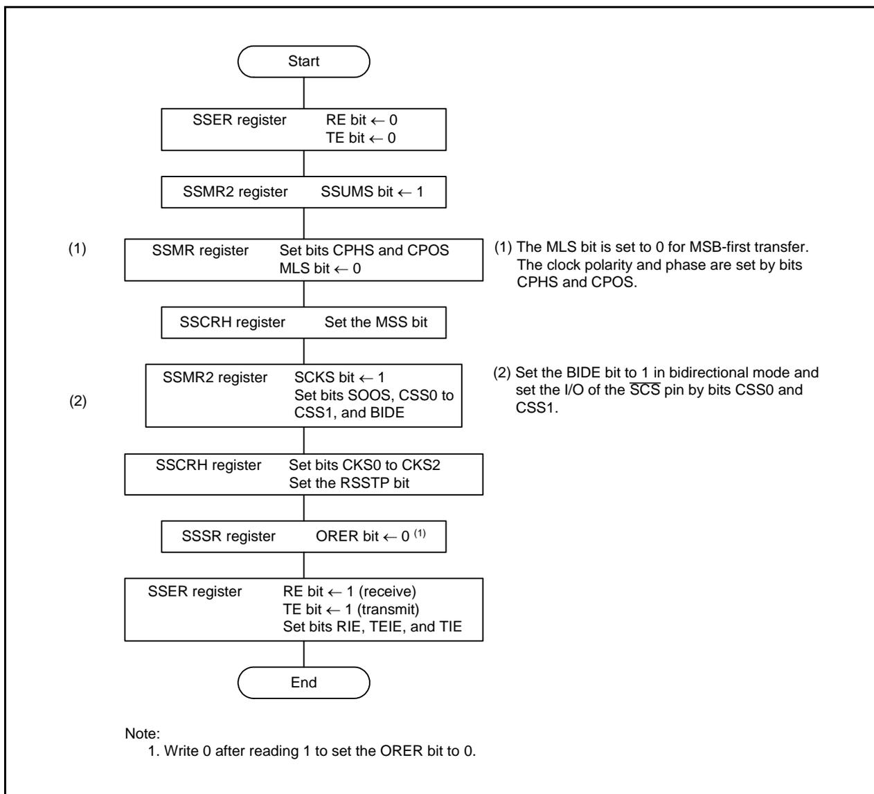
Figure 22.10 Initialization in 4-Wire Bus Communication Mode
