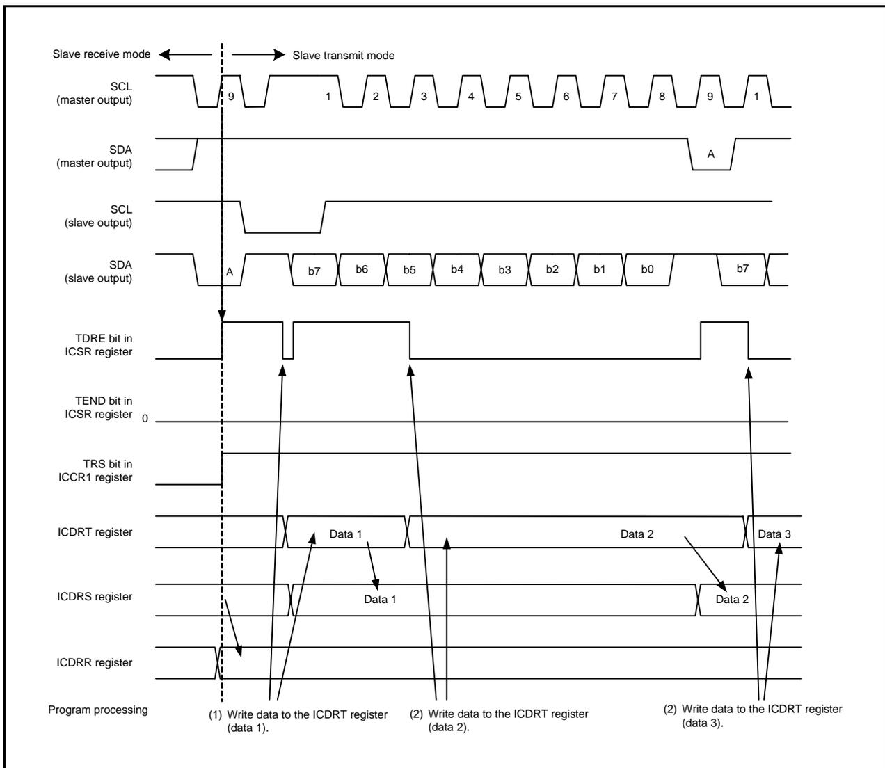
Figure 23.9 Operating Timing in Slave Transmit Mode (I<sup>2</sup>C bus Interface Mode) (1)
