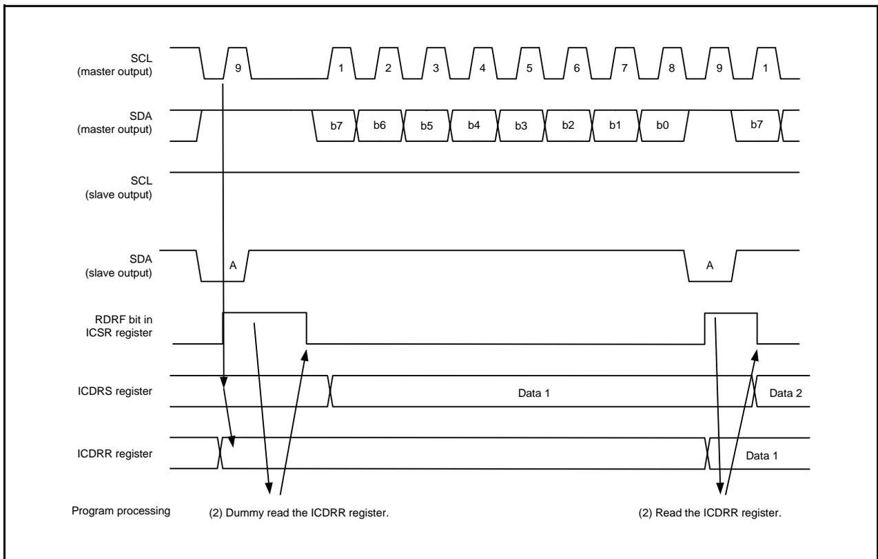
Figure 23.11 Operating Timing in Slave Receive Mode (I<sup>2</sup>C bus Interface Mode) (1)
