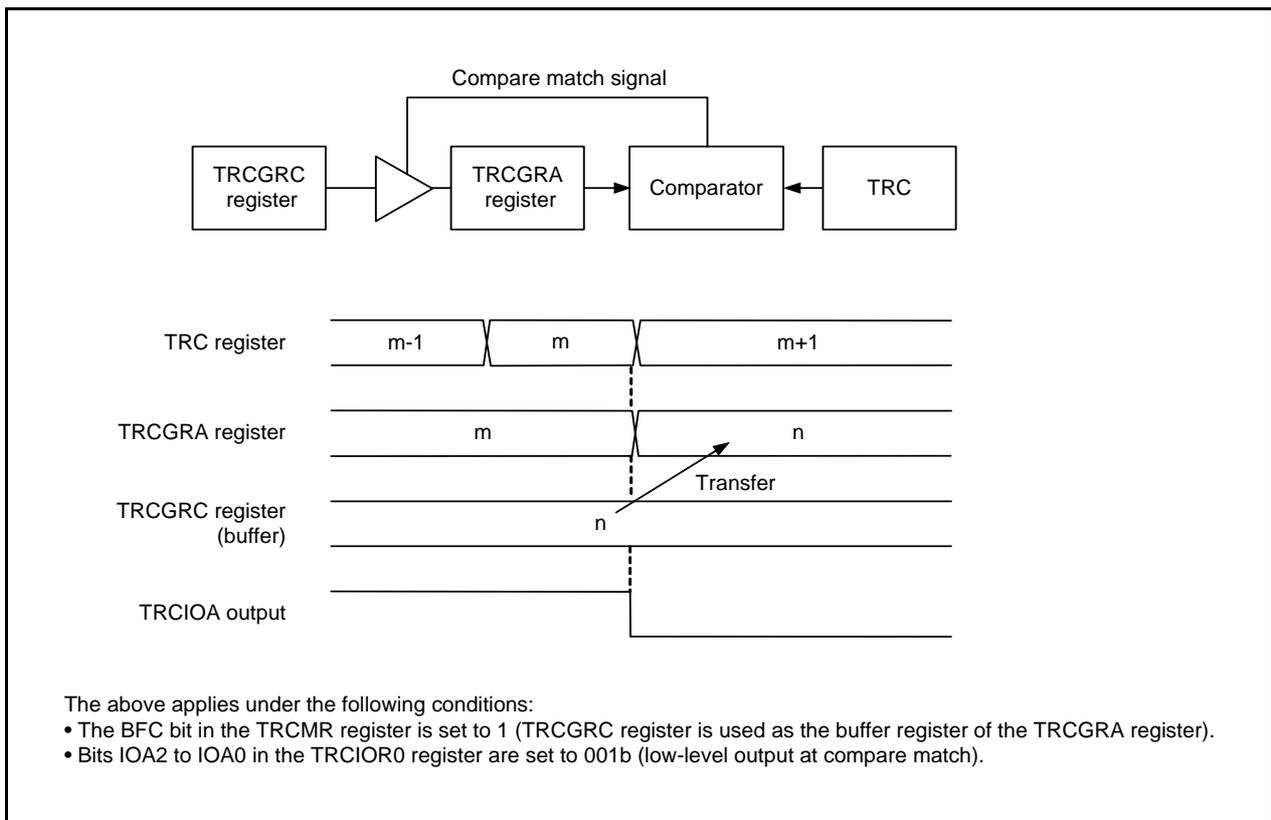
**Figure 18.4 Buffer Operation of Output Compare Function**
