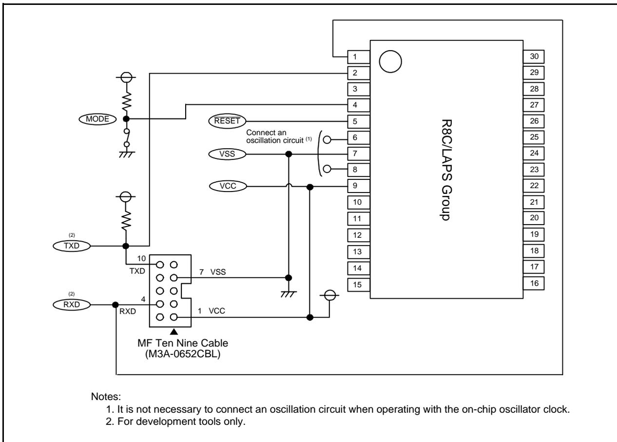
Appendix Figure 2.1 Connection Example with MF Ten Nine Cable (M3A-0652CBL)
