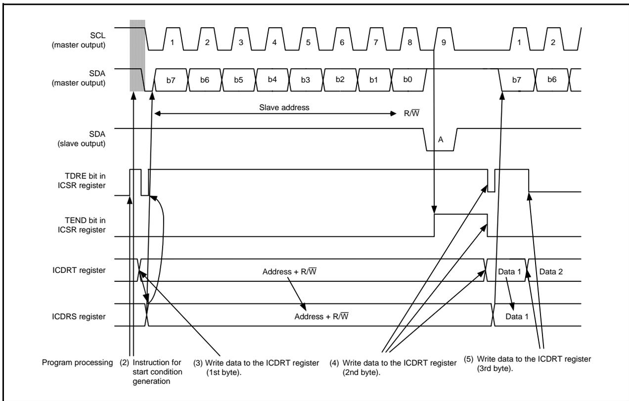
Figure 23.5 Operating Timing in Master Transmit Mode (I<sup>2</sup>C bus Interface Mode) (1)
