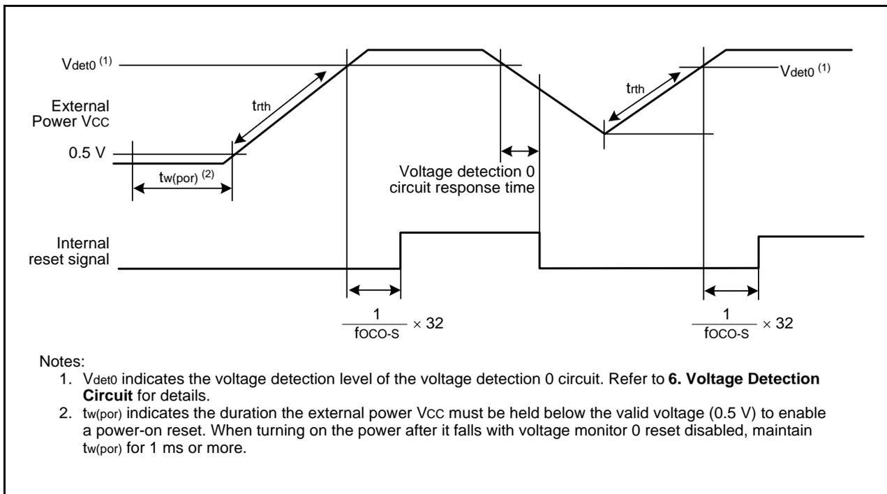
**Figure 25.3 Power-on Reset Circuit Characteristics**
