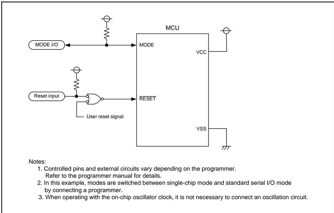
**Figure 24.22 Pin Handling in Standard Serial I/O Mode 3**
