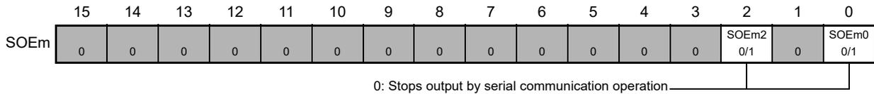
\* For channel n, whose serial output is stopped, the SOmn bit value of the SOm register can be set by software.
