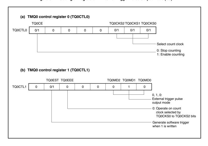
Figure 8-22. Setting of Registers in External Trigger Pulse Output Mode (2/3)
