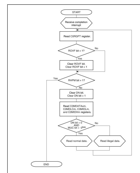
Figure 19-50. Reception via Interrupt (Using C0RGPT Register)
