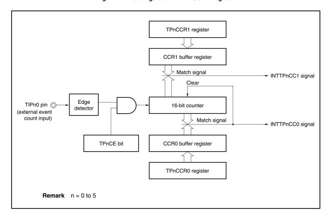
If the set value of the TPnCCR1 register is smaller than the set value of the TPnCCR0 register, the INTTPnCC1 signal is generated once per cycle.
