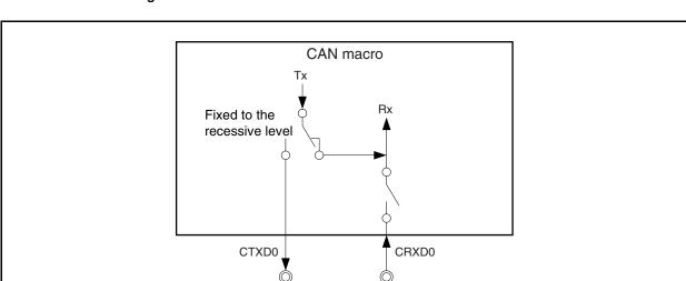
Figure 19-34. CAN Module Terminal Connection in Self-Test Mode
