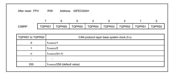
Figure 19-23. CAN Module Clock
