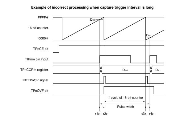
The following problem may occur when long pulse width is measured in the free-running timer mode.
