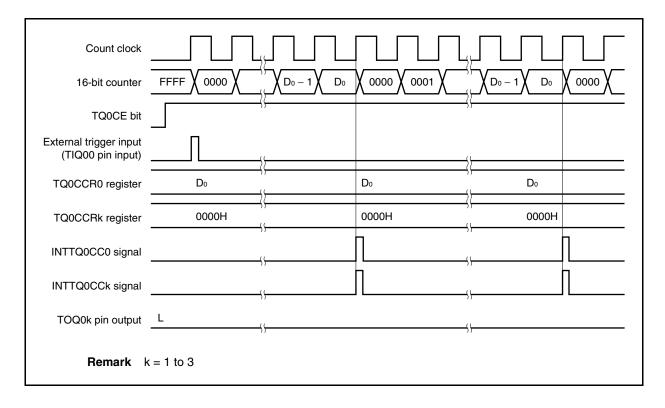
To output a 100% waveform, set a value of (set value of TQ0CCR0 register + 1) to the TQ0CCRk register. If the set value of the TQ0CCR0 register is FFFFH, 100% output cannot be produced.
