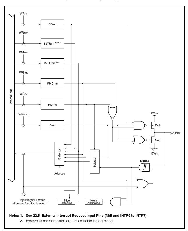
Figure 4-17. Block Diagram of Type N-1
