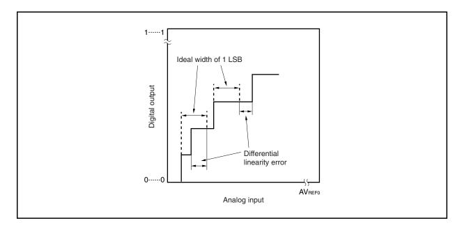
Figure 13-20. Differential Linearity Error
