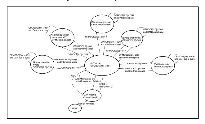
The transition from the initialization mode to an operation mode is controlled by the C0CTRL.OPMODE2 to C0CTRL.OPMODE0 bits.
