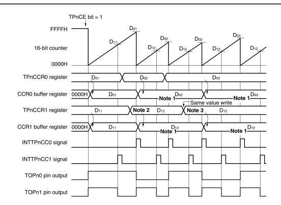
Figure 7-5. Timing of Batch Write
