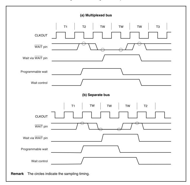
Figure 5-3. Inserting Wait Example
