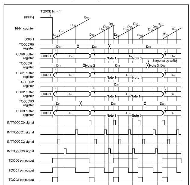
Figure 8-5. Timing of Batch Write
