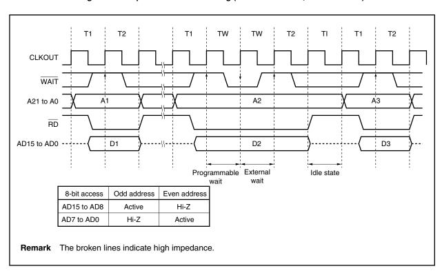
Т1 T2 Т1 T1 T2 TW TW T2 ΤI CLKOUT WAIT A21 to A0 Α<sub>1</sub> A2 ÅЗ RD AD7 to AD0 D1 D2 D3 Programmable External Idle state wait wait Remark The broken lines indicate high impedance.
