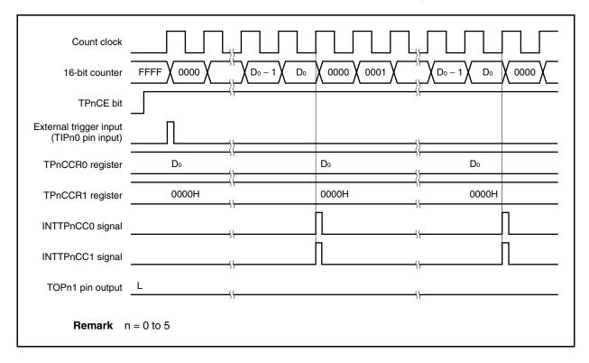
To output a 100% waveform, set a value of (set value of TPnCCR0 register + 1) to the TPnCCR1 register. If the set value of the TPnCCR0 register is FFFFH, 100% output cannot be produced.
