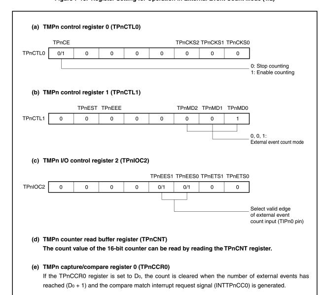
Figure 7-15. Register Setting for Operation in External Event Count Mode (2/2)
