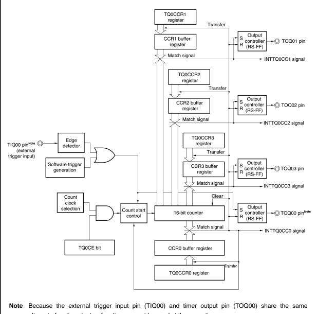
Figure 8-24. Configuration in One-Shot Pulse Output Mode
