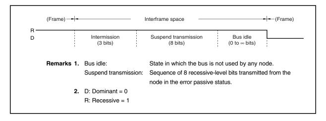
Usually, the intermission field is 3 bits. If the transmitting node detects a dominant level at the third bit of the intermission field, however, it executes transmission.
