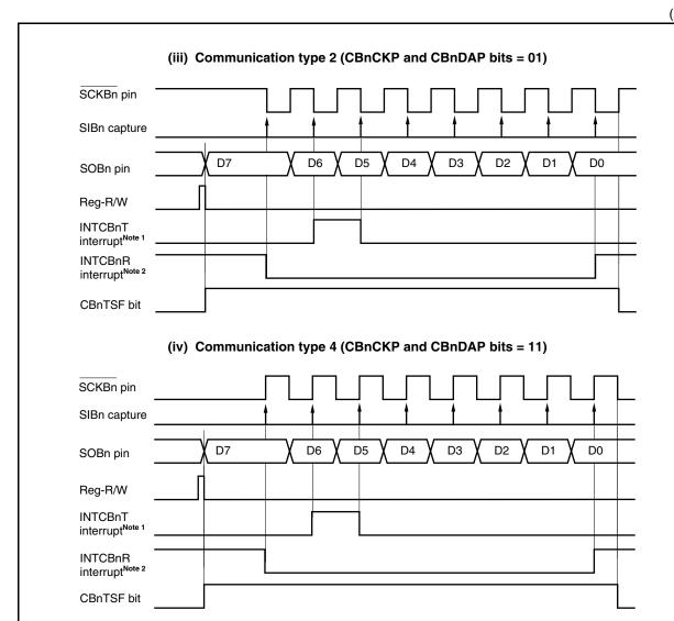
Notes 1. The INTCBnT interrupt is set when the data written to the CBnTX register is transferred to the data shift register in the continuous transmission or continuous transmission/reception modes. In the single transmission or single transmission/reception modes, the INTCBnT interrupt request signal is not generated, but the INTCBnR interrupt request signal is generated upon end of communication.
