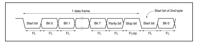
Assuming 1 bit data length: FL; stop bit length: FLstp; and base clock frequency: fuclk, we obtain the following equation.
