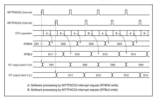
Figure 12-2. Example of Operation Timing and Software Processing of RTO0
