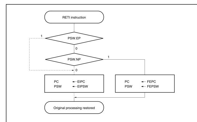
Caution When the EP and NP bits are changed by the LDSR instruction during non-maskable interrupt servicing, in order to restore the PC and PSW correctly during recovery by the RETI instruction, it is necessary to clear the EP bit to 0 and set the NP bit to 1 using the LDSR instruction immediately before the RETI instruction.
