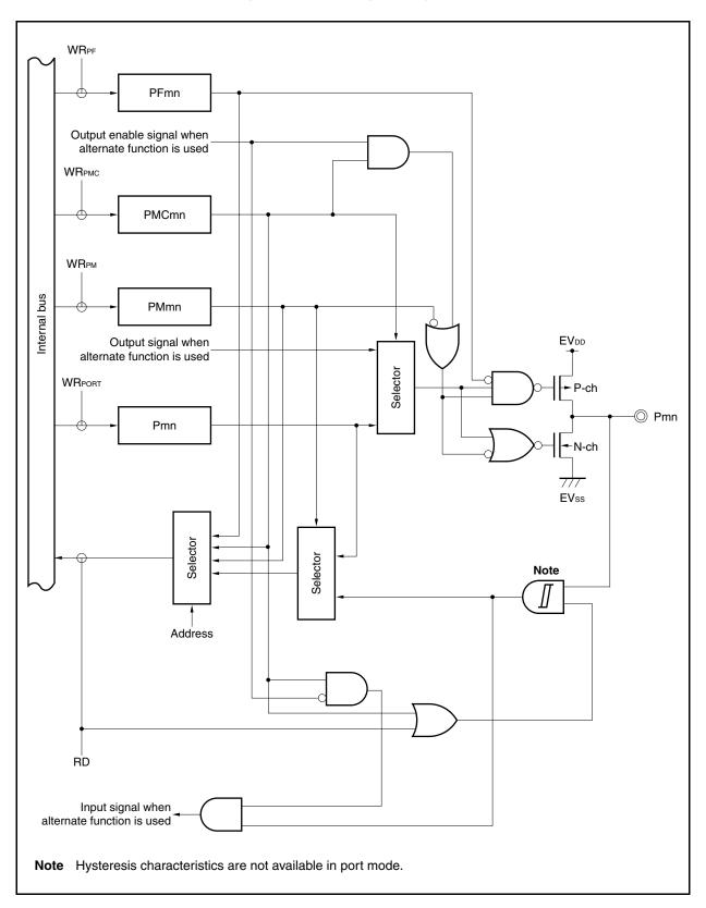
Figure 4-9. Block Diagram of Type G-1
