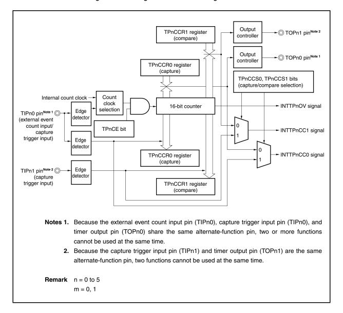
Figure 7-32. Configuration in Free-Running Timer Mode
