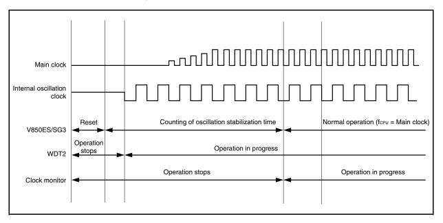
Figure 25-6. Operation After Reset Release
