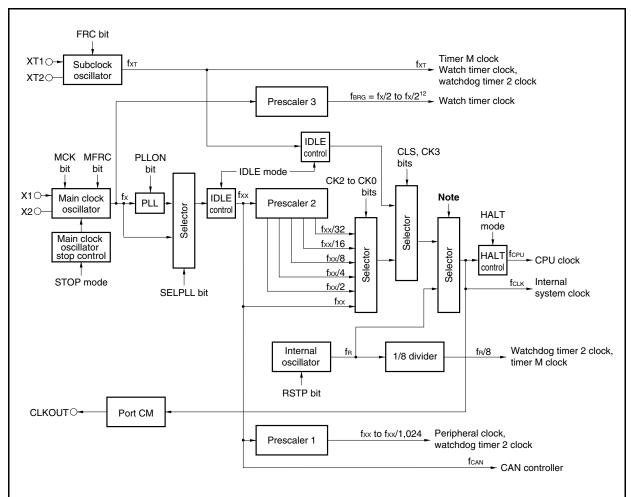
**Note** The internal oscillation clock (f<sub>R</sub>) is selected when watchdog timer 2 overflows during the oscillation stabilization time.
