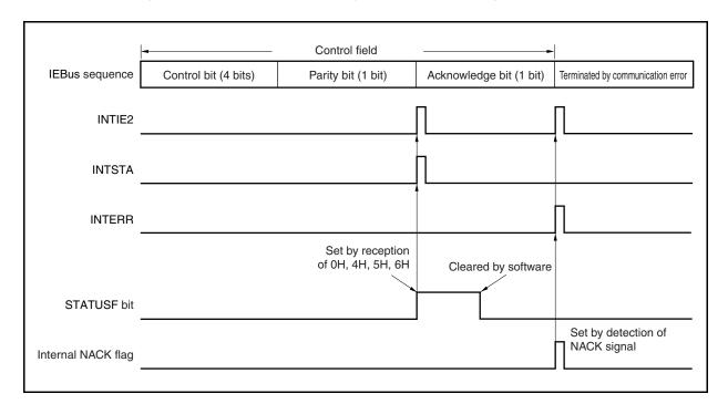
Figure 18-17. Interrupt Request Signal Generation Timing (for (2) and (5))
