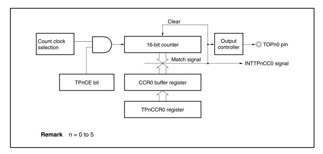
Figure 7-6. Configuration of Interval Timer
