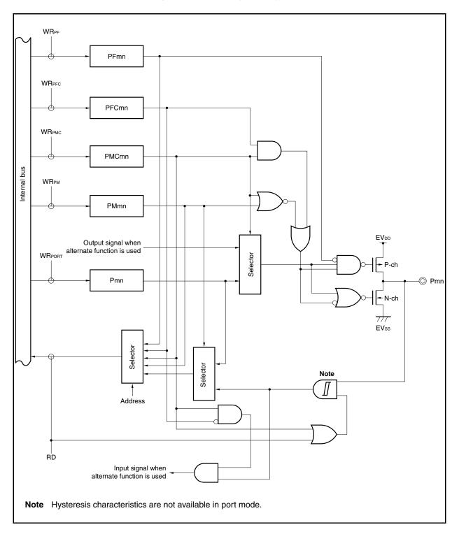
Figure 4-10. Block Diagram of Type G-2
