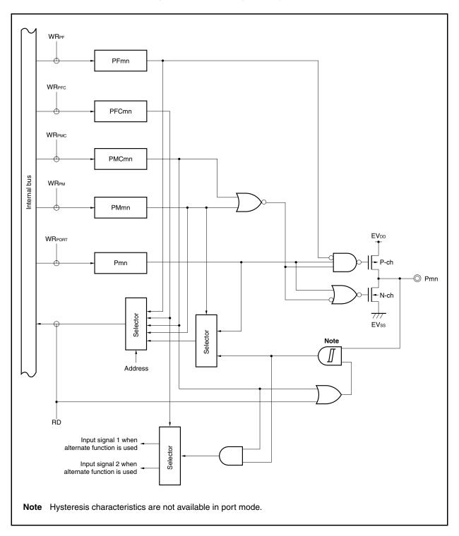
Figure 4-13. Block Diagram of Type G-5
