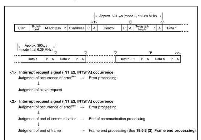
**Note** This processing is necessary only when the INTIE2 interrupt request signal is used as the start interrupt, and is not necessary when the INTSTA interrupt request signal is used (in this case, the error processing is performed by using the INTERR interrupt request signal).
