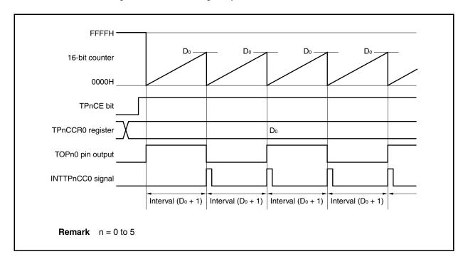
When the TPnCE bit is set to 1, the value of the 16-bit counter is cleared from FFFFH to 0000H in synchronization with the count clock, and the counter starts counting. At this time, the output of the TOPn0 pin is inverted. Additionally, the set value of the TPnCCR0 register is transferred to the CCR0 buffer register.
