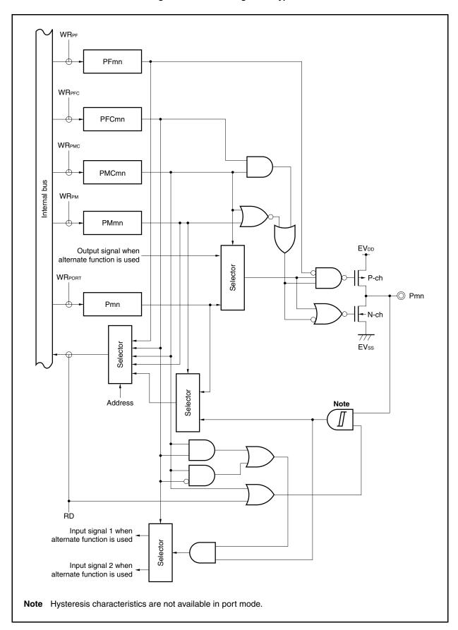
Figure 4-15. Block Diagram of Type G-12
