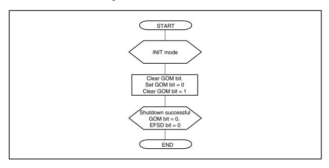
Figure 19-57. Forced Shutdown Process
