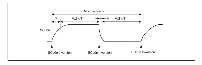
The clock to be selected can be set by the combination of the SMCn, CLn1, and CLn0 bits of the IICCLn register, the CLXn bit of the IICXn register, and the OCKSTHm, OCKSm1, and OCKSm0 bits of the OCKSm register (n = 0 to 2, m = 0, 1).
