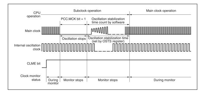
Figure 26-5. Operation When Main Clock Is Stopped (Arbitrary)
