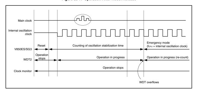
Figure 25-7. Operation After Reset Release
