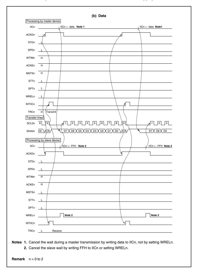
Figure 17-20. Example of Master to Slave Communication (When 9-Clock Wait Is Selected for Both Master and Slave) (3/3)
