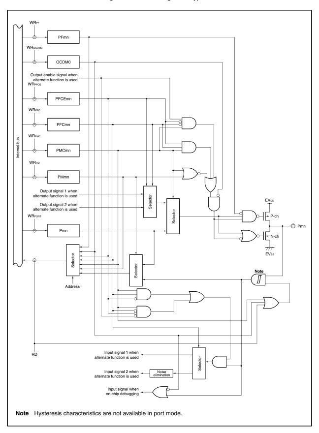
Figure 4-26. Block Diagram of Type U-10
