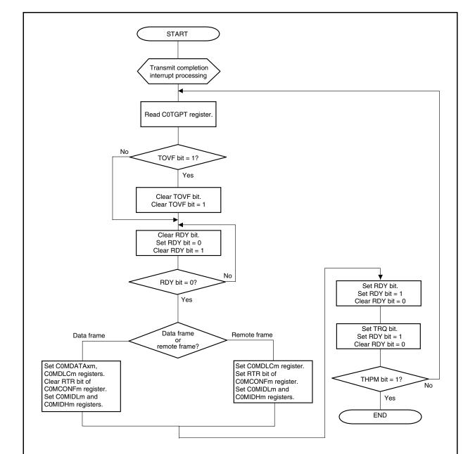
Figure 19-44. Transmission via Interrupt (Using C0TGPT Register)
