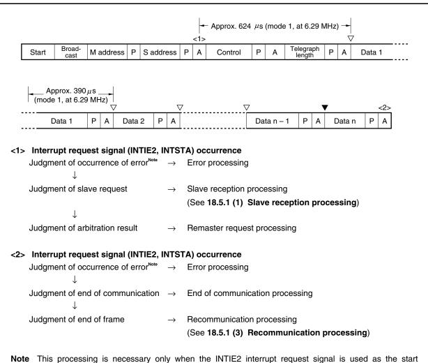
**Note** This processing is necessary only when the INTIE2 interrupt request signal is used as the start interrupt, and is not necessary when the INTSTA interrupt request signal is used (in this case, the error processing is performed by using the INTERR interrupt request signal).
