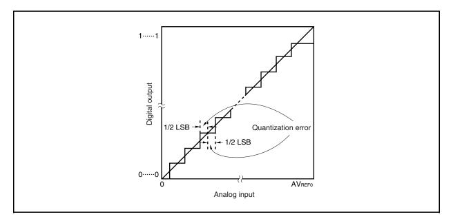
Figure 13-17. Quantization Error
