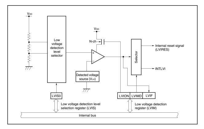
Figure 27-1. Block Diagram of Low-Voltage Detector
