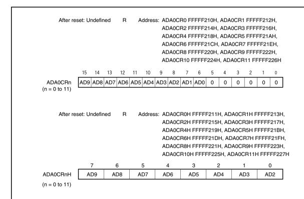
Caution A write operation to the ADA0M0 and ADA0S registers may cause the contents of the ADA0CRn register to become undefined. After the conversion, read the conversion result before writing to the ADA0M0 and ADA0S registers. Correct conversion results may not be read if a sequence other than the above is used.
