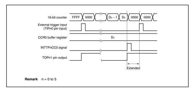
If the trigger is detected immediately before the INTTPnCC0 signal is generated, the INTTPnCC0 signal is not generated. The 16-bit counter is cleared to 0000H, the TOPn1 pin is asserted, and the counter continues counting. Consequently, the inactive period of the PWM waveform is shortened.
