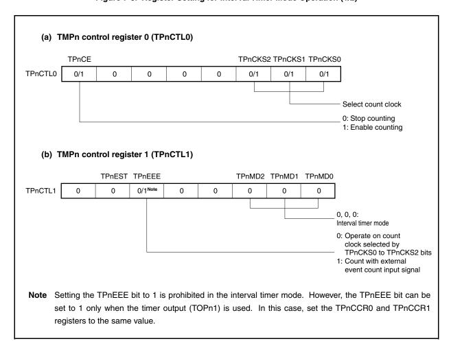
Figure 7-8. Register Setting for Interval Timer Mode Operation (2/2)
