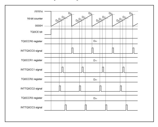
If the set value of the TQ0CCRk register is greater than the set value of the TQ0CCR0 register, the INTTQ0CCk signal is not generated because the count value of the 16-bit counter and the value of the TQ0CCRk register do not match.
