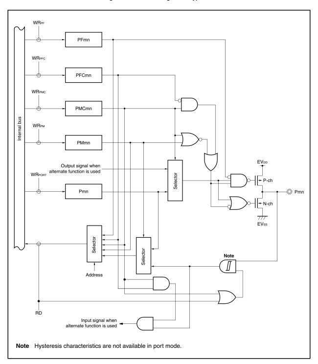
Figure 4-11. Block Diagram of Type G-3
