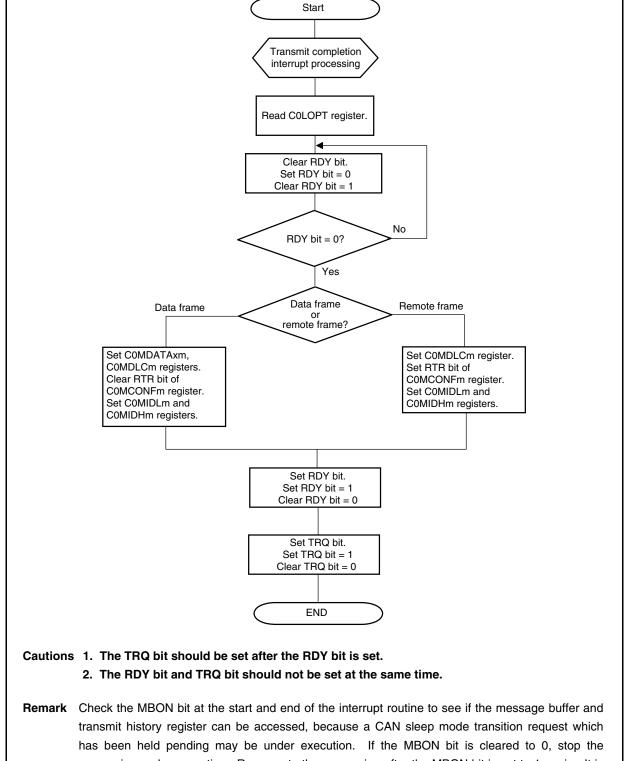
Figure 19-43. Transmission via Interrupt (Using C0LOPT Register)
