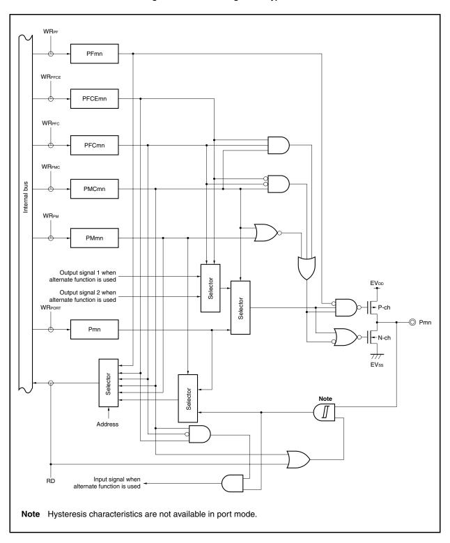
Figure 4-30. Block Diagram of Type U-14
