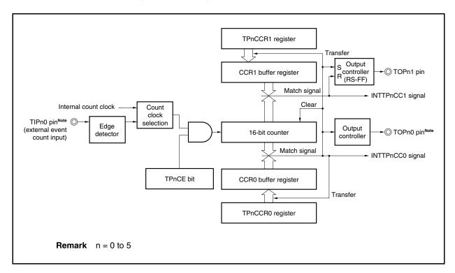
Figure 7-28. Configuration in PWM Output Mode
