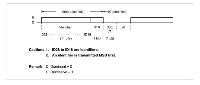
Figure 19-7. Arbitration Field (in Extended Format Mode)
