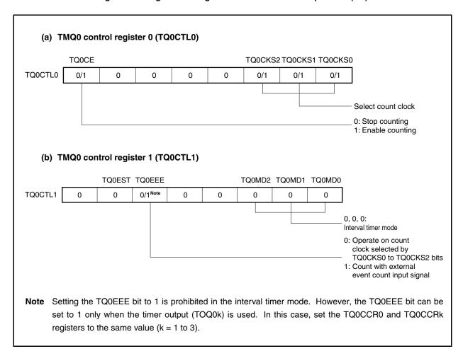
Figure 8-8. Register Setting for Interval Timer Mode Operation (2/3)
