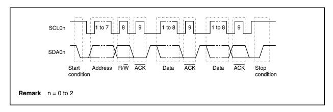
Figure 17-4. I<sup>2</sup>C Bus Serial Data Transfer Timing
