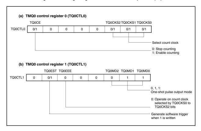
Figure 8-26. Register Setting in One-Shot Pulse Output Mode (2/3)
