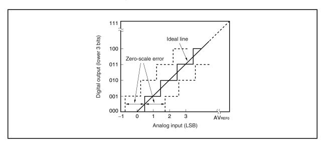
Figure 13-18. Zero-Scale Error
