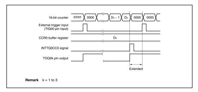
If the trigger is detected immediately before the INTTQ0CC0 signal is generated, the INTTQ0CC0 signal is not generated. The 16-bit counter is cleared to 0000H, the TOQ0k pin is asserted, and the counter continues counting. Consequently, the inactive period of the PWM waveform is shortened.
