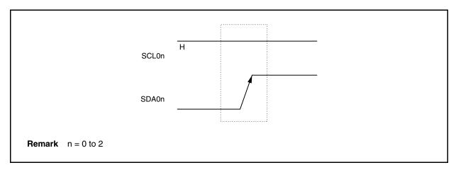
A stop condition is generated when the IICCn.SPTn bit is set to 1. When the stop condition is detected, the IICSn.SPDn bit is set to 1 and the interrupt request signal (INTIICn) is generated when the IICCn.SPIEn bit is set to 1 (n = 0 to 2).
