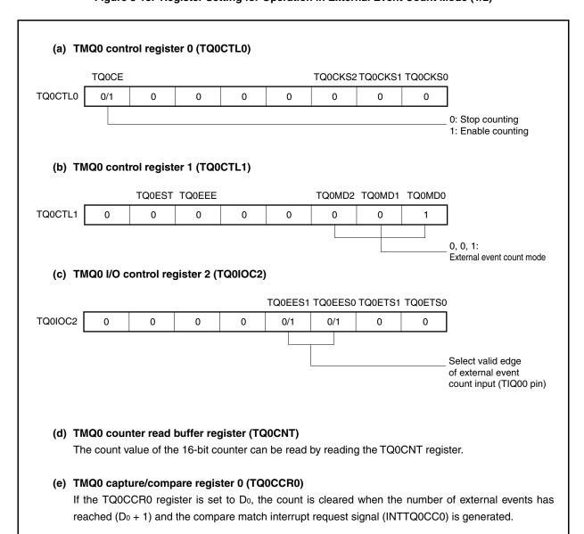
Figure 8-15. Register Setting for Operation in External Event Count Mode (2/2)
