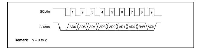
When the local address is received, ACK is automatically generated regardless of the value of the ACKEn bit. No ACK is generated if the received address is not a local address (NACK).
