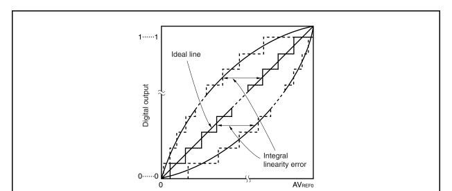
Figure 13-21. Integral Linearity Error
