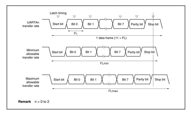
As shown in Figure 15-16, the receive data latch timing is determined by the counter set using the UAnCTL2 register following start bit detection. The transmit data can be normally received if up to the last data (stop bit) can be received in time for this latch timing.
