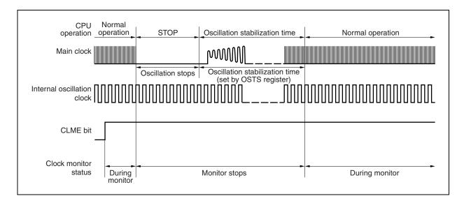
Figure 26-4. Operation in STOP Mode or After STOP Mode Is Released
