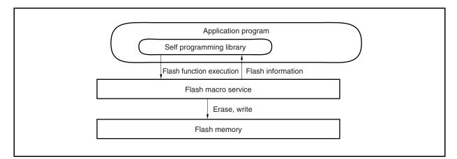
Figure 30-15. Concept of Self Programming
