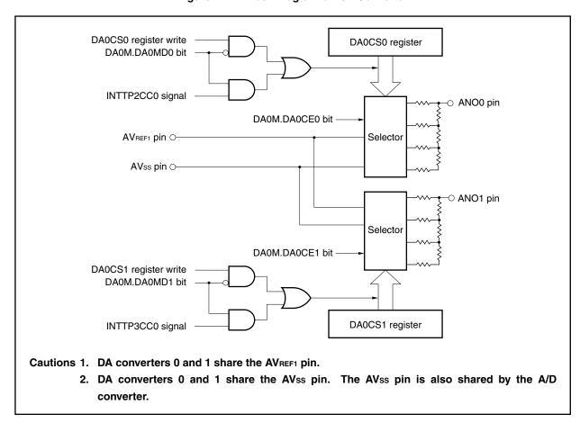
The D/A converter includes the following hardware.
