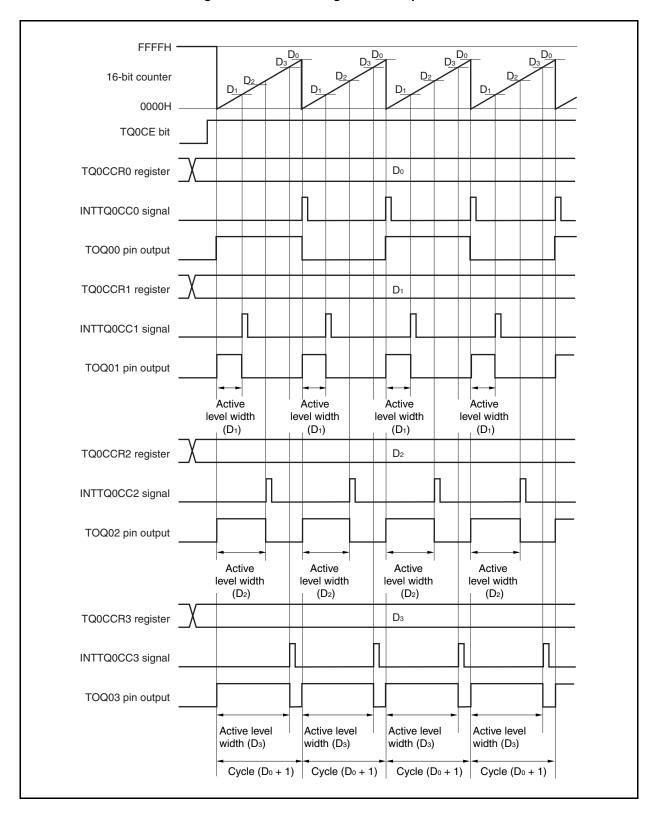
When the TQ0CE bit is set to 1, the 16-bit counter is cleared from FFFFH to 0000H, starts counting, and outputs PWM waveform from the TQQ0k pin.
