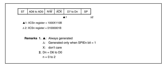
(6) When arbitration loss occurs due to low level of SDA0n pin when attempting to generate a restart
