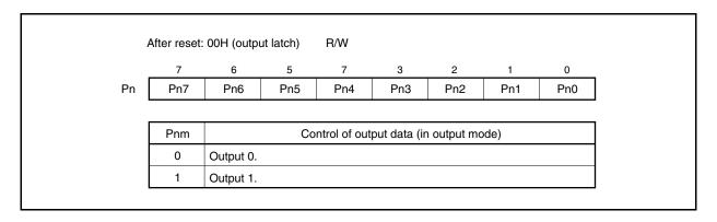
Data is written to or read from the Pn register as follows, regardless of the setting of the PMCn register.
