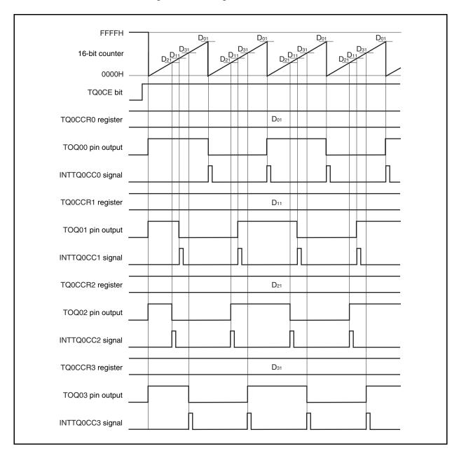
If the set value of the TQ0CCRk register is greater than the set value of the TQ0CCR0 register, the count value of the 16-bit counter does not match the value of the TQ0CCRk register. Consequently, the INTTQ0CCk signal is not generated, nor is the output of the TQQ0k pin changed.
