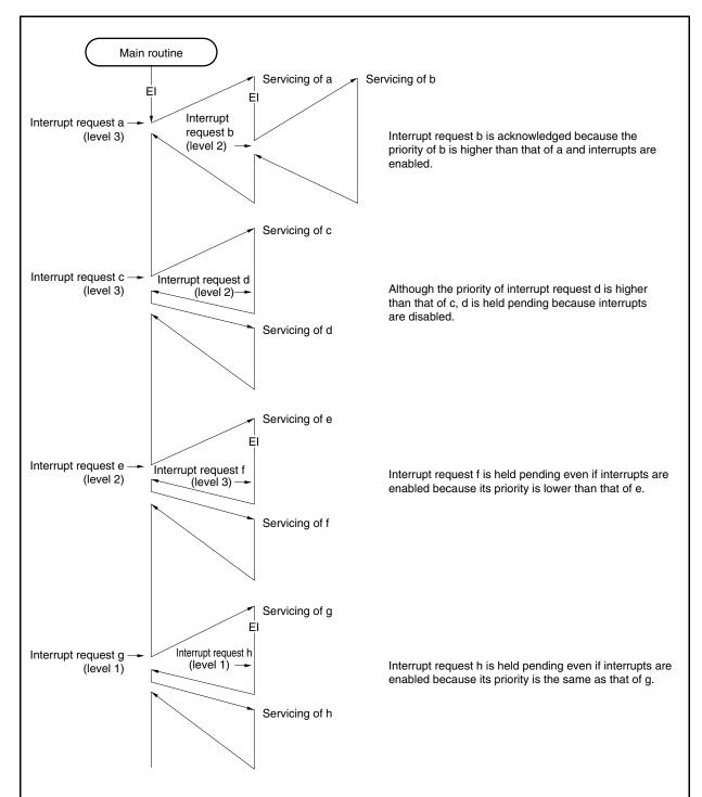
Caution To perform multiple interrupt servicing, the values of the EIPC and EIPSW registers must be saved before executing the El instruction. When returning from multiple interrupt servicing, restore the values of EIPC and EIPSW after executing the DI instruction.
