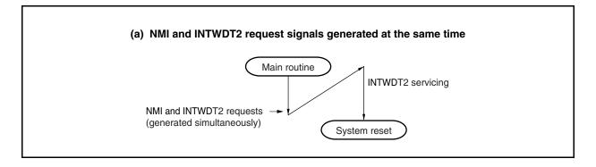
Figure 22-1. Non-Maskable Interrupt Request Signal Acknowledgment Operation (2/2)
