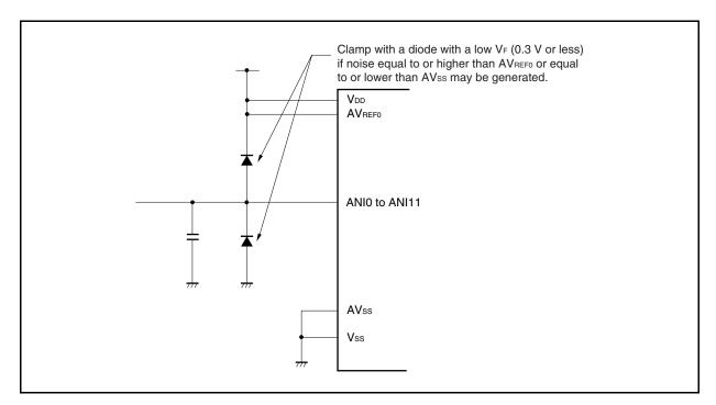
Figure 13-12. Processing of Analog Input Pin
