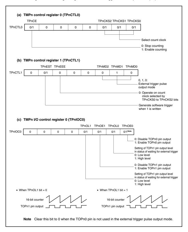
Figure 7-22. Setting of Registers in External Trigger Pulse Output Mode (2/2)
