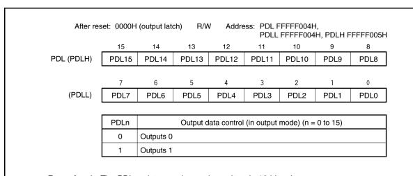
Remarks 1. The PDL register can be read or written in 16-bit units.
