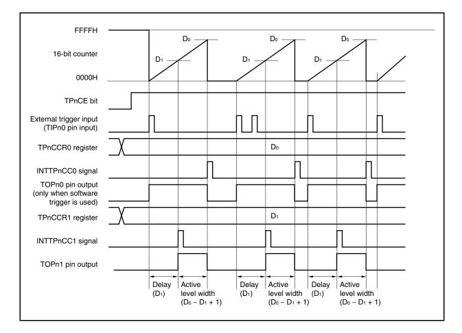
Figure 7-25. Basic Timing in One-Shot Pulse Output Mode
