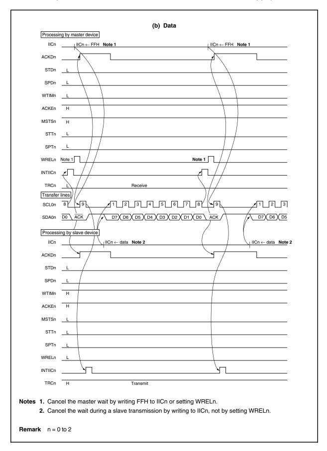
Figure 17-21. Example of Slave to Master Communication (When 8-Clock  $\rightarrow$  9-Clock Wait for Master and 9-Clock Wait for Slave Are Selected) (3/3)
