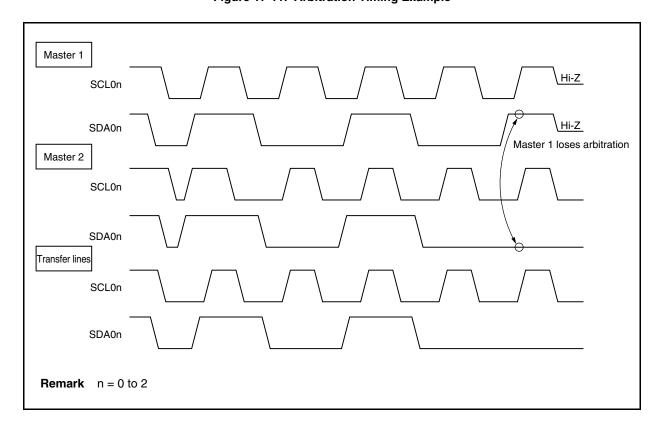
Figure 17-11. Arbitration Timing Example
