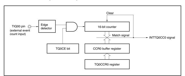
Figure 8-13. Configuration in External Event Count Mode
