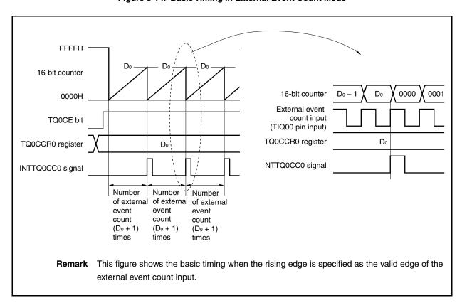
When the TQ0CE bit is set to 1, the value of the 16-bit counter is cleared from FFFFH to 0000H. The counter counts each time the valid edge of external event count input is detected. Additionally, the set value of the TQ0CCR0 register is transferred to the CCR0 buffer register.
