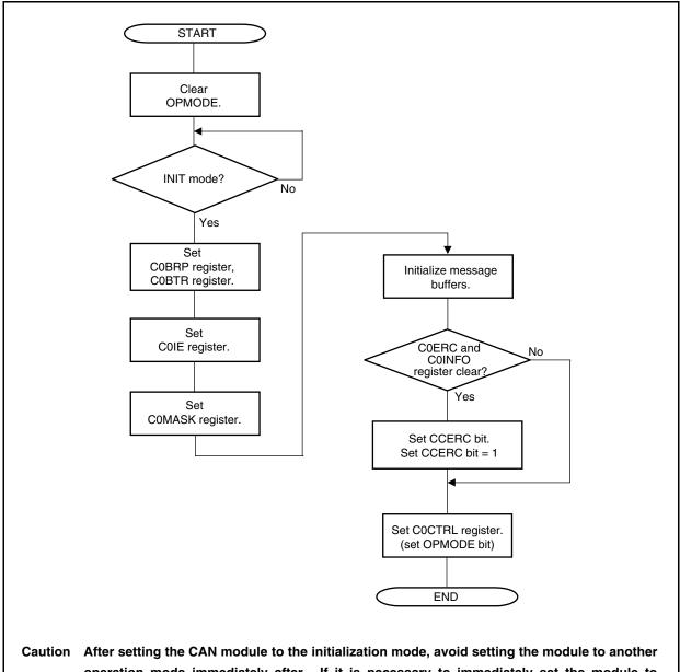
Caution After setting the CAN module to the initialization mode, avoid setting the module to another operation mode immediately after. If it is necessary to immediately set the module to another operation mode, be sure to access registers other than the COCTRL and COGMCTRL registers (e.g., set a message buffer).
