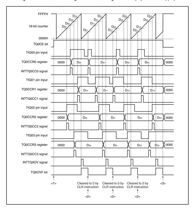
Figure 8-37. Software Processing Flow in Free-Running Timer Mode (Capture Function) (2/2)
