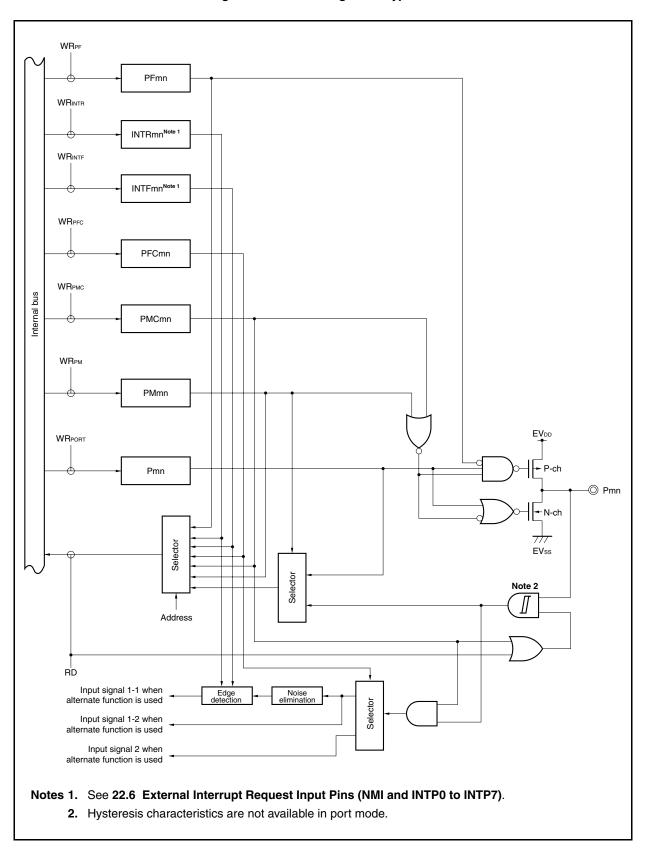
Figure 4-20. Block Diagram of Type U-1
