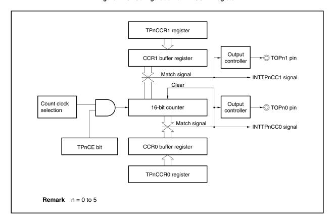
When the TPnCCR1 register is set to the same value as the TPnCCR0 register, the INTTPnCC1 signal is generated at the same timing as the INTTPnCC0 signal and the TOPn1 pin output is inverted. In other words, a square wave with a duty factor of 50% can be output from the TOPn1 pin.
