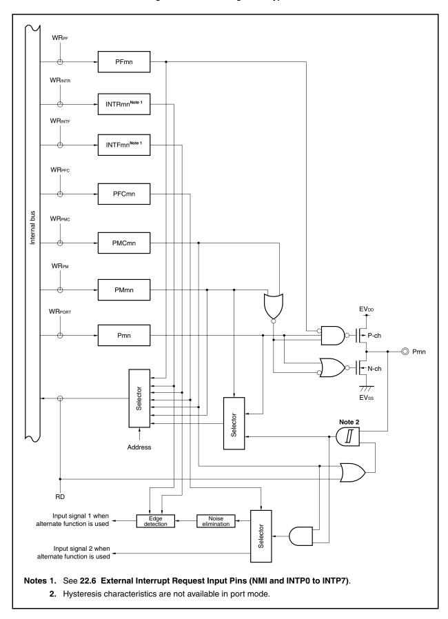
Figure 4-18. Block Diagram of Type N-2
