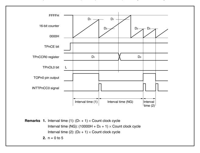
If the value of the TPnCCR0 register is changed from  $D_1$  to  $D_2$  while the count value is greater than  $D_2$  but less than  $D_1$ , the count value is transferred to the CCR0 buffer register as soon as the TPnCCR0 register has been rewritten. Consequently, the value of the 16-bit counter that is compared is  $D_2$ .
