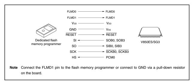
The dedicated flash memory programmer outputs the transfer clock, and the V850ES/SG3 operates as a slave. When the PG-FP4 or PG-FP5 is used as the dedicated flash memory programmer, it generates the following signals to the V850ES/SG3. For details, see the **PG-FP4 User's Manual (U15260E)**, **PG-FP5 User's Manual (U18865E)**.
