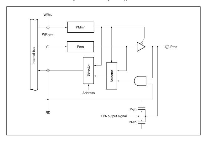
Figure 4-5. Block Diagram of Type D-1
