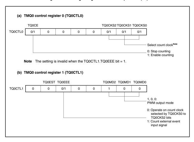
Figure 8-30. Setting of Registers in PWM Output Mode (2/3)
