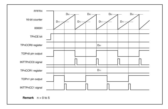
Figure 7-11. Timing Chart When D<sub>01</sub> ≥ D<sub>11</sub>
