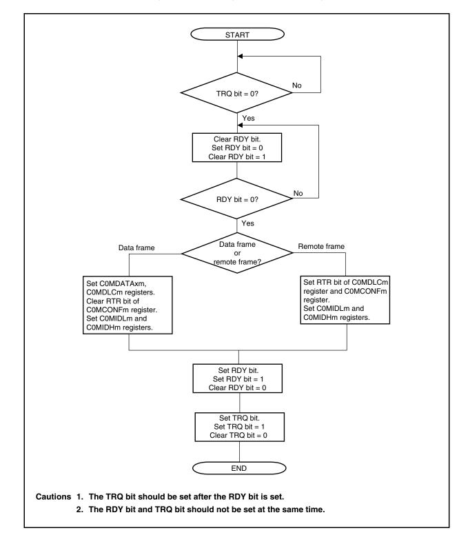
Figure 19-41. Message Transmit Processing
