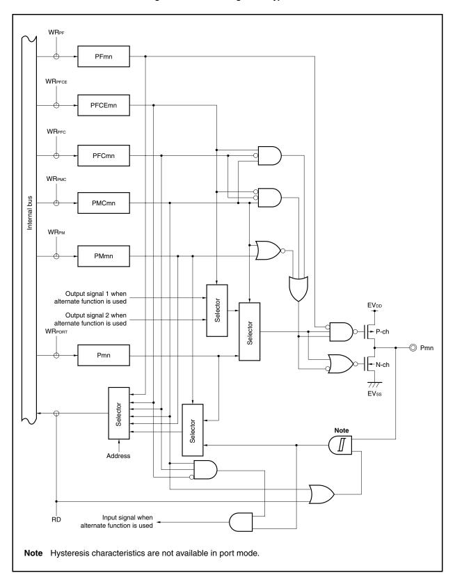
Figure 4-29. Block Diagram of Type U-13
