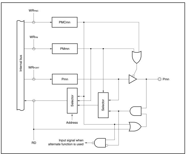
Figure 4-6. Block Diagram of Type D-2
