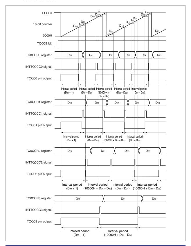
When performing an interval operation in the free-running timer mode, two intervals can be set with one channel.
