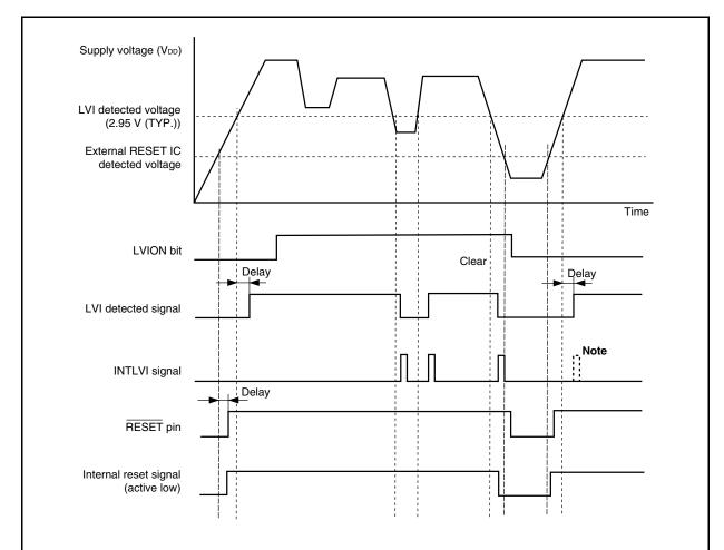
**Note** Since the LVION bit is the initial value (operation disabled) due to the external reset input, no INTLVI interrupts occur.
