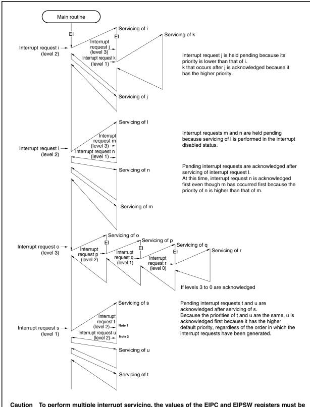
Caution To perform multiple interrupt servicing, the values of the EIPC and EIPSW registers must be saved before executing the EI instruction. When returning from multiple interrupt servicing, restore the values of EIPC and EIPSW after executing the DI instruction.
