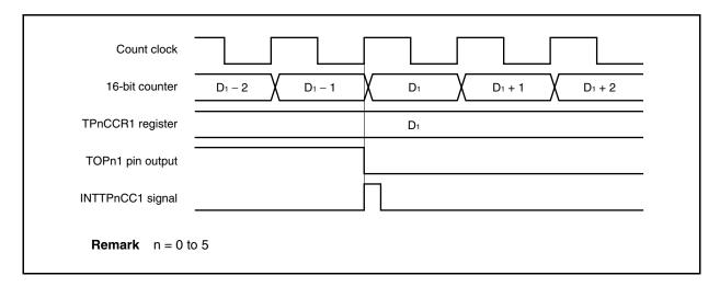
Usually, the INTTPnCC1 signal is generated when the 16-bit counter counts up next time after its count value matches the value of the TPnCCR1 register.
