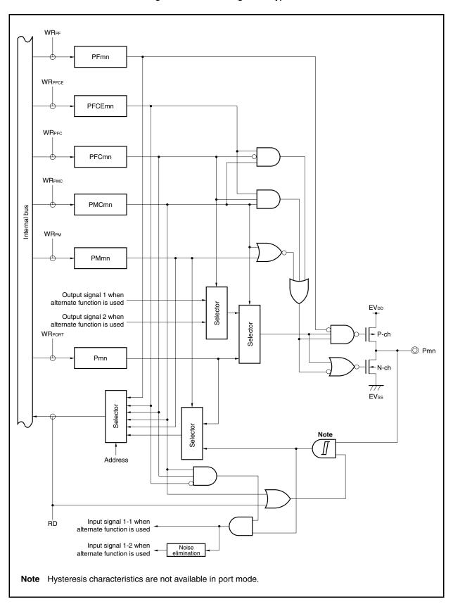
Figure 4-22. Block Diagram of Type U-6
