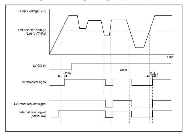
Figure 27-2. Operation Timing of Low-Voltage Detector (LVIMD Bit = 1)
