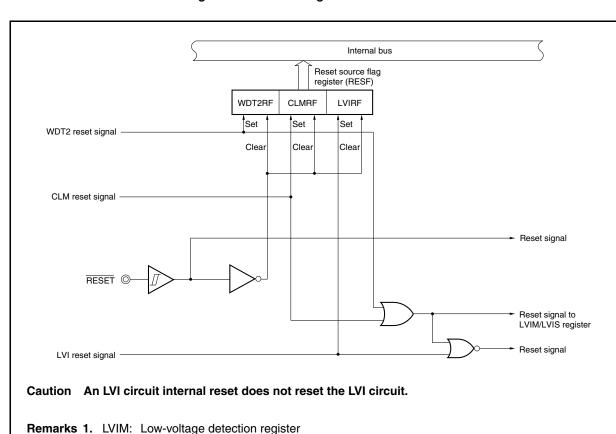
Figure 25-1. Block Diagram of Reset Function
