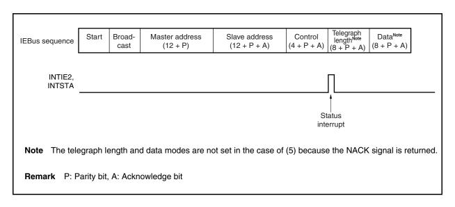
Figure 18-19. Timing of INTIE2 and INTSTA Interrupt Request Signal Generation in Locked State (for (3))
