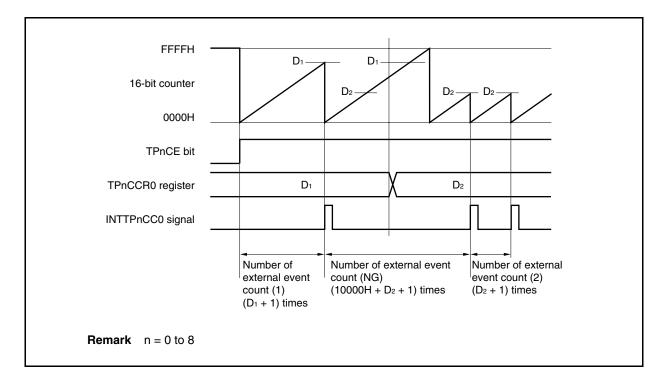
If the value of the TPnCCR0 register is changed from D<sub>1</sub> to D<sub>2</sub> while the count value is greater than D<sub>2</sub> but less than D<sub>1</sub>, the count value is transferred to the CCR0 buffer register as soon as the TPnCCR0 register has been rewritten. Consequently, the value that is compared with the 16-bit counter is D<sub>2</sub>.
