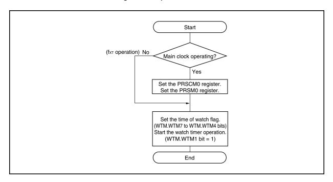
Figure 10-5. Operation Stop Flow
