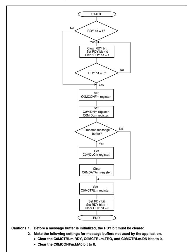
Figure 19-39 shows the processing for a receive message buffer (C0MCONFm.MT2 to C0MCONFm.MT0 bits = 001B to 101B).
