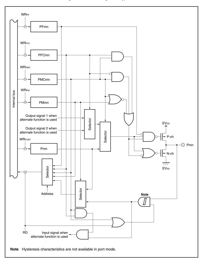
Figure 4-16. Block Diagram of Type L-1
