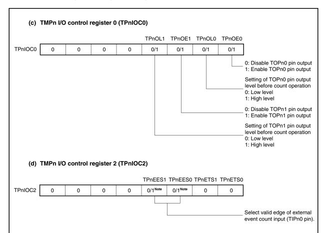
Note Setting the TPnEES1 and TPnESS0 bits to 1 is prohibited in the interval timer mode. However, the TPnEES1 and TPnEES0 bits can be set to 1 only when the timer output (TOPn1) is used. In this case, set the TPnCCR0 and TPnCCR1 registers to the same value.
