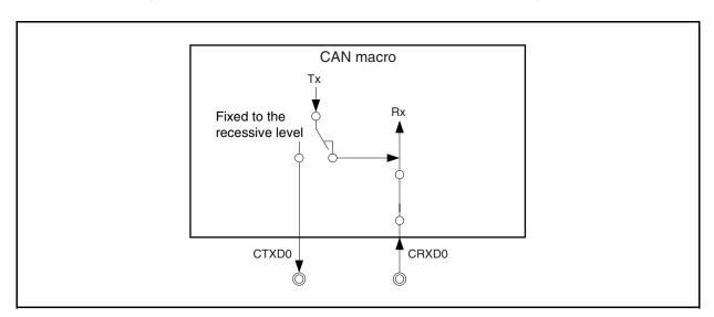
Figure 19-33. CAN Module Terminal Connection in Receive-Only Mode
