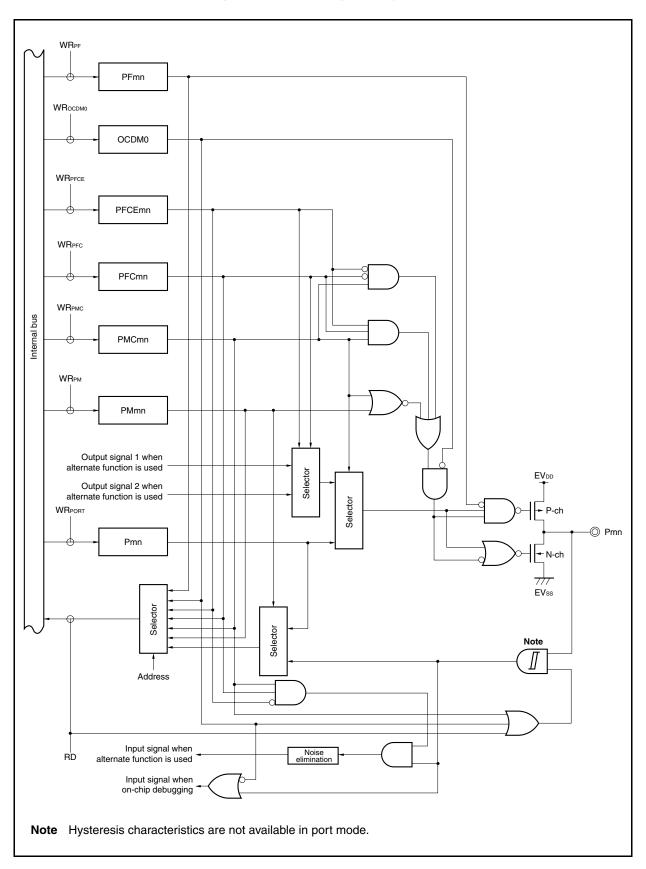
Figure 4-25. Block Diagram of Type U-9
