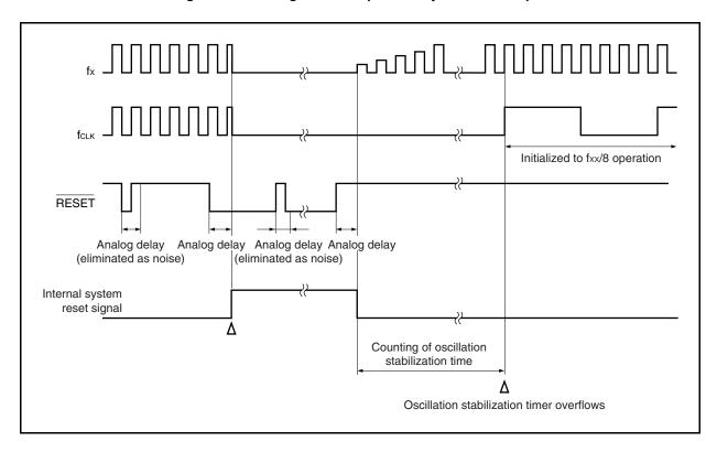
Figure 25-3. Timing of Power-on Reset Operation
