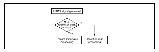
Figure 18-22. Example of Identifying INTERR Signal Interrupt (When INTIE1, INTERR, and INTSTA Signals Are Used)
