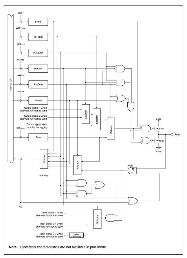
Figure 4-24. Block Diagram of Type U-8
