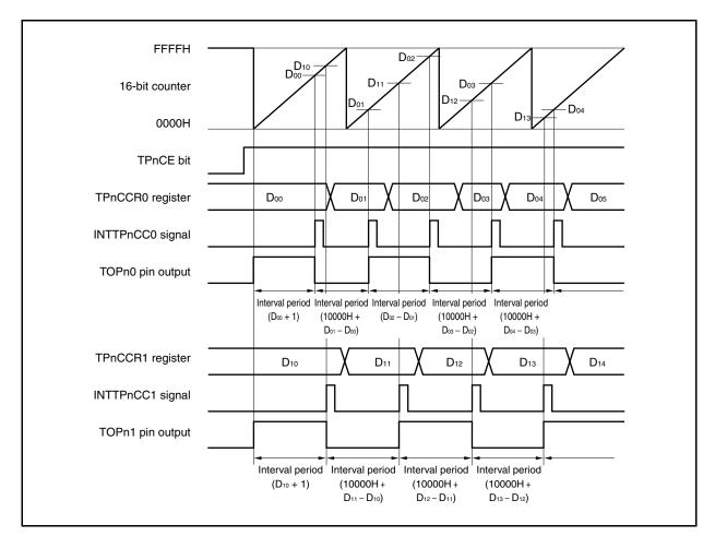
When performing an interval operation in the free-running timer mode, two intervals can be set with one channel.
