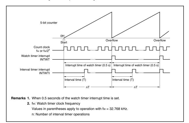
Figure 10-6. Operation Timing of Watch Timer/Interval Timer
