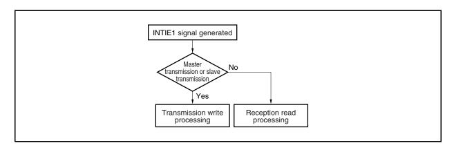
Figure 18-25. Example of Identifying INTIE2 Signal Interrupt (When INTIE1 and INTIE2 Signals Are Used)
