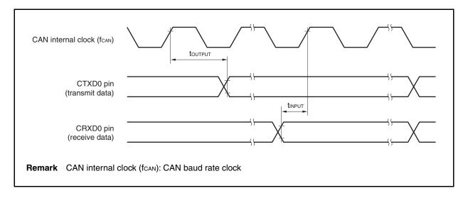
Internal delay time (tnode) = Internal transmission delay time (toutput) + Internal reception delay time (tnput)
