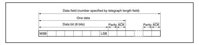
Following the data bit, the parity bit and acknowledge bit are respectively output by the master unit and slave unit.
