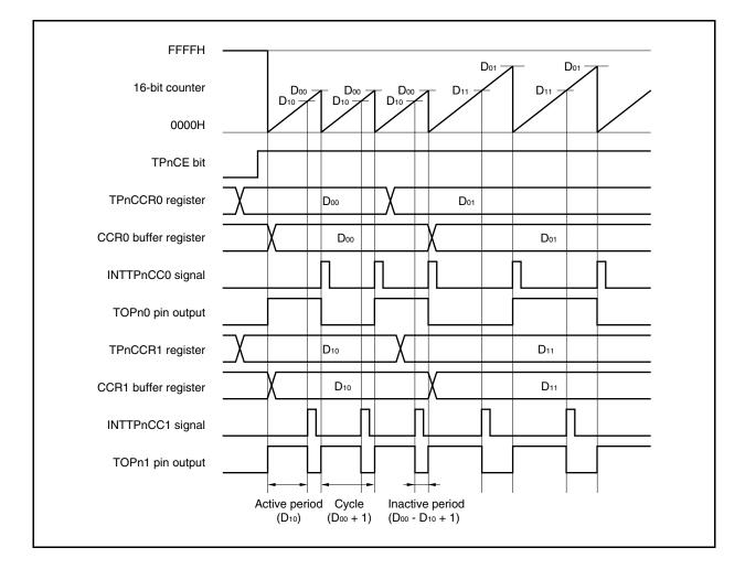
Figure 7-29. Basic Timing in PWM Output Mode
