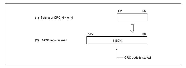
The code when 01H is sent LSB first is (1000 0000). Therefore, the CRC code from generation polynomial  $X^{16} + X^{12} + X^5 + 1$  becomes the remainder when (1000 0000)  $X^{16}$  is divided by (1 0001 0000 0010 0001) using the modulo-2 operation formula.
