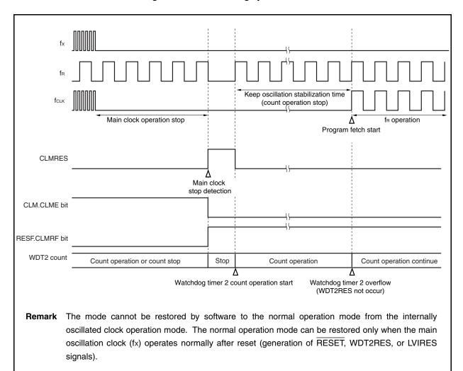
Figure 25-5. Reset Timing by Clock Monitor
