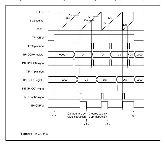
Figure 7-37. Software Processing Flow in Free-Running Timer Mode (Capture Function) (2/2)
