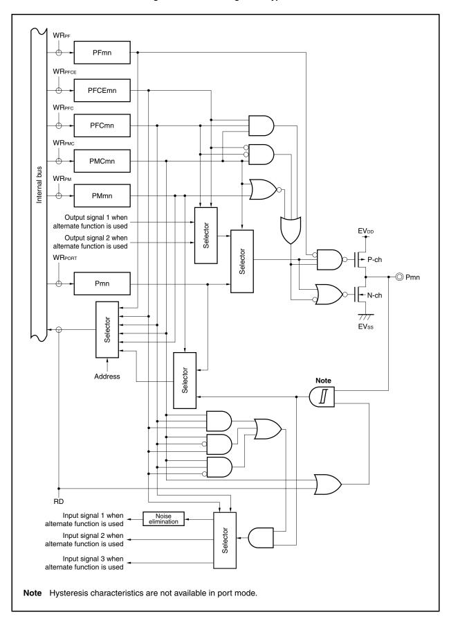
Figure 4-28. Block Diagram of Type U-12
