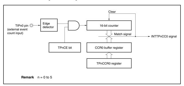
Figure 7-13. Configuration in External Event Count Mode
