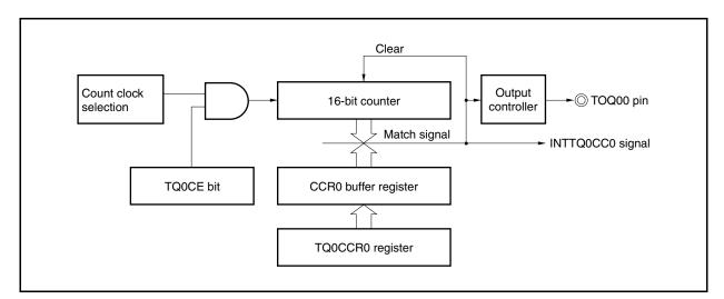
Figure 8-6. Configuration of Interval Timer
