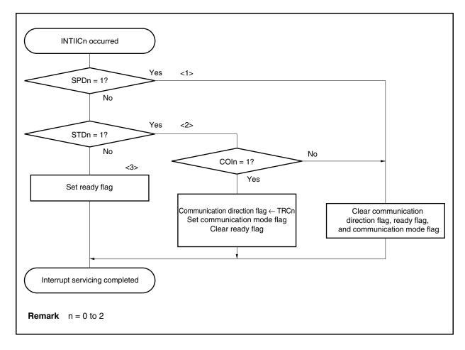
Figure 17-19. Slave Operation Flowchart (2)
