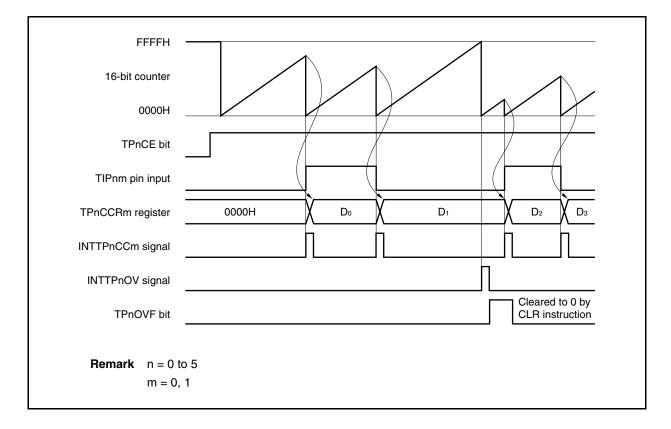
Figure 7-39. Basic Timing in Pulse Width Measurement Mode
