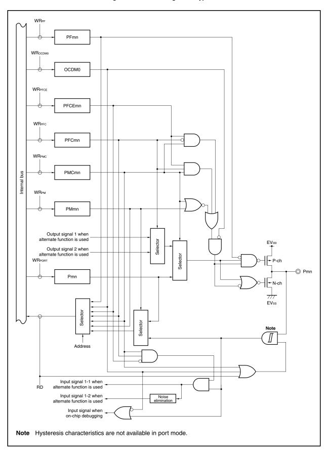
Figure 4-23. Block Diagram of Type U-7
