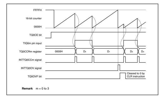
Figure 8-39. Basic Timing in Pulse Width Measurement Mode
