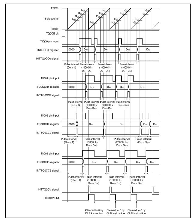
When executing pulse width measurement in the free-running timer mode, four pulse widths can be measured with one channel.
