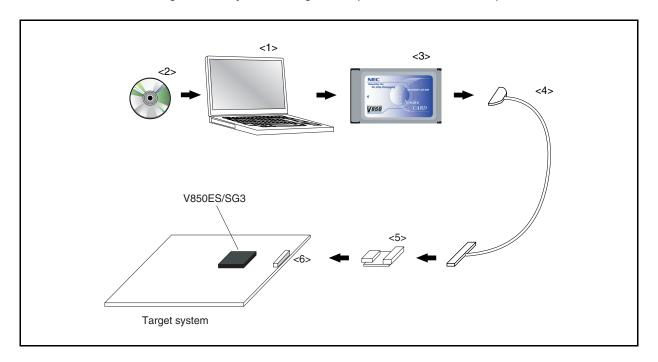
Figure A-4. System Configuration (IE-V850E1-CD-NW Used)
