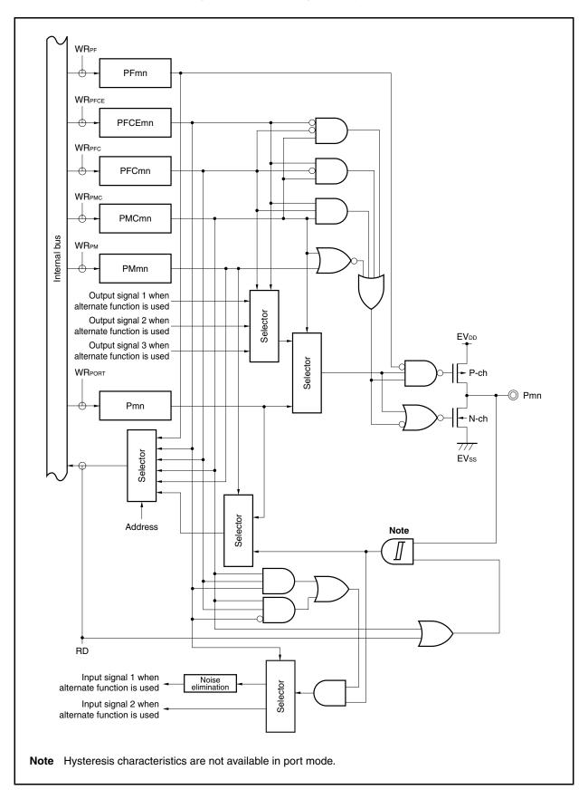
Figure 4-27. Block Diagram of Type U-11
