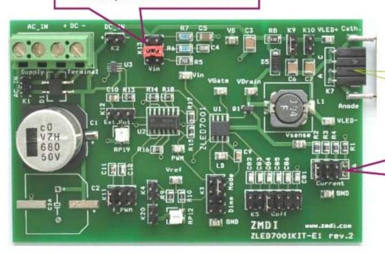
The driver circuit is intrinsically safe against open LED circuit.
