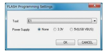
If not supplying power from the E1, sets the [None], and if supplying, set according to the input voltage of the board to be used.
