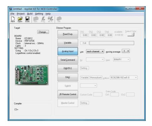
(1) Select the [Analog Input] button in Dimmer Program and specify from the [use] drop-down list the A/D conversion port to be used for the dimming value.
