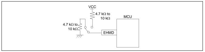
Figure 2.6 Connection of the EHMD Pin
