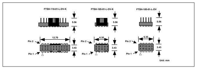
Figure 2.2 20-Pin and 10-Pin Connector Specifications
