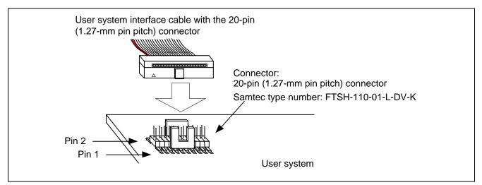
Figure 2.1 Connecting the User System Interface Cable to the 20-Pin Connector of the E2/E2 Lite
