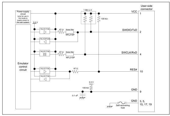
Figure 2.7 shows the internal circuits of the E2 with the MCU connected via the SWD interface.
