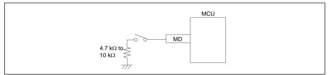
Figure 2.5 Connection of the MD Pin
