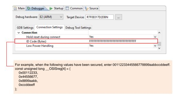
Figure 3.5 Setting of [ID Code (Bytes)]
