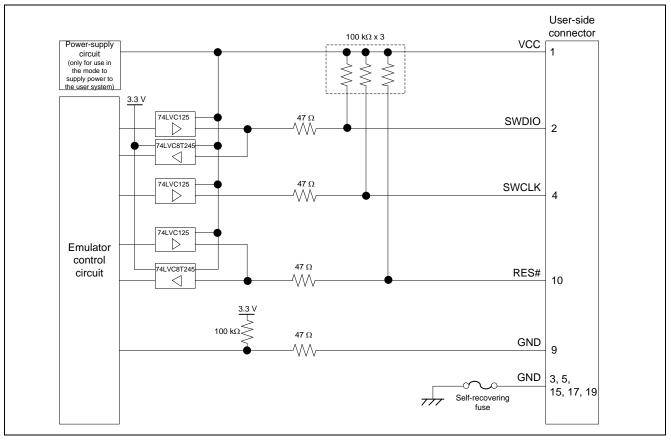
Figure 2.8 Internal Circuits of the E2 Lite with the MCU Connected via the SWD Interface
