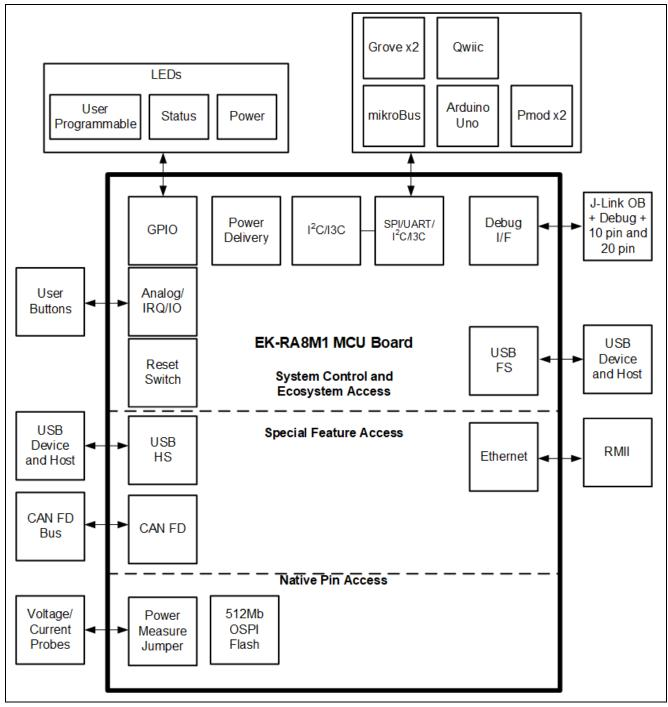
Figure 5. EK-RA8M1 Board Block Diagram
