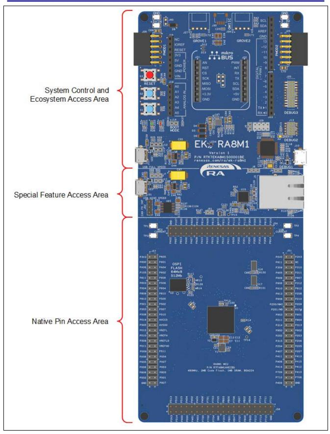
Figure 4. EK-RA8M1 Board Functional Area Definitions
