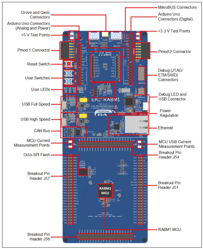
Figure 1. EK-RA8M1 Board Top Side
