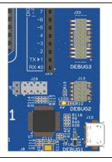
Figure 10. EK-RA8M1 Debug Interface
