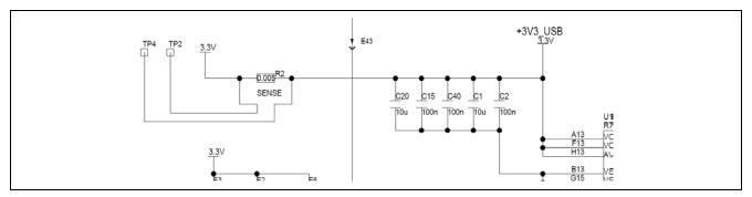
Figure 27. RA USB Current Measurement Circuit
