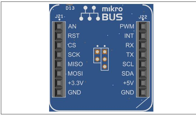
Figure 15. mikroBUS Connection
