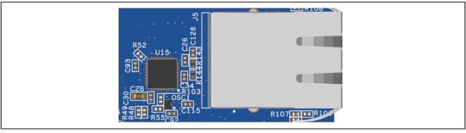
Figure 23. Ethernet Connector
