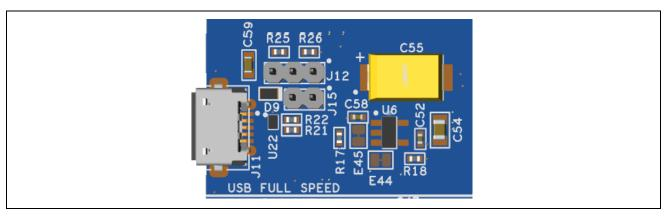
Figure 16. USB Full Speed Connector
