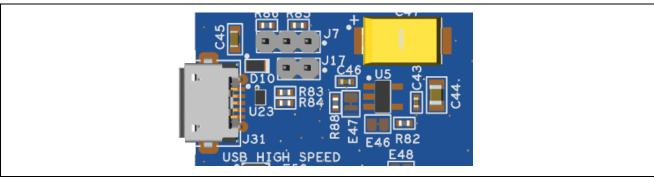
Figure 24. USB High Speed Connector
