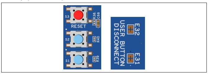
Figure 19. Reset and User Switches
