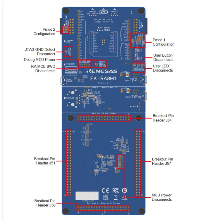
Figure 2. EK-RA8M1 Board Bottom Side
