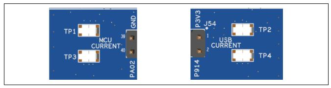
Figure 29. RA MCU and USB Current Measurement
