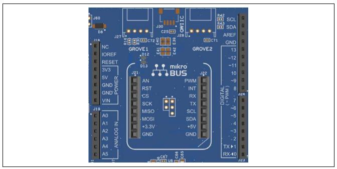
Figure 14. Arduino Uno Connectors
