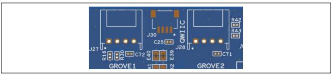
Figure 11. Seeed Grove and SparkFun Qwiic® Connector Footprints
