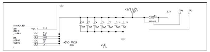
Figure 28. RA +3.3 V Current Measurement Circuit
