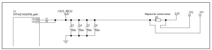
Figure 18. RA +3.3 V Current Measurement Circuit
