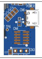
Figure 7. FPB-RA2E2 Debug Interface
