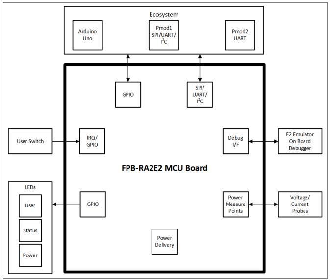
Figure 4. FPB-RA2E2 Board Block Diagram
