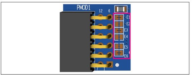
Figure 10. Pmod 1 Trace Cut Jumpers
