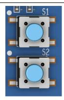
Figure 15. Reset (S2) and User Switch (S1)
