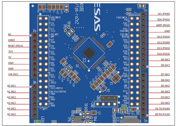
Figure 12. Arduino Uno Connectors
