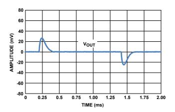
FIGURE 5. LOAD TRANSIENT ( $\triangle I_L = 1mA$ )
