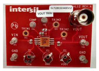
FIGURE 6. VOLTAGE REFERENCE EVALUATION BOARD (FRONT)
