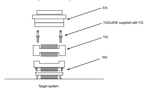
Figure 2-6. Mounting of EA, YQ and NQ
