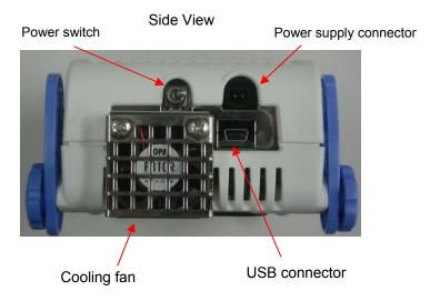
Figure 1-1. Names of Parts of QB-RL78L12
