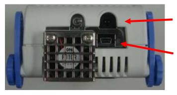
Power supply connector (Connect AC adapter)
