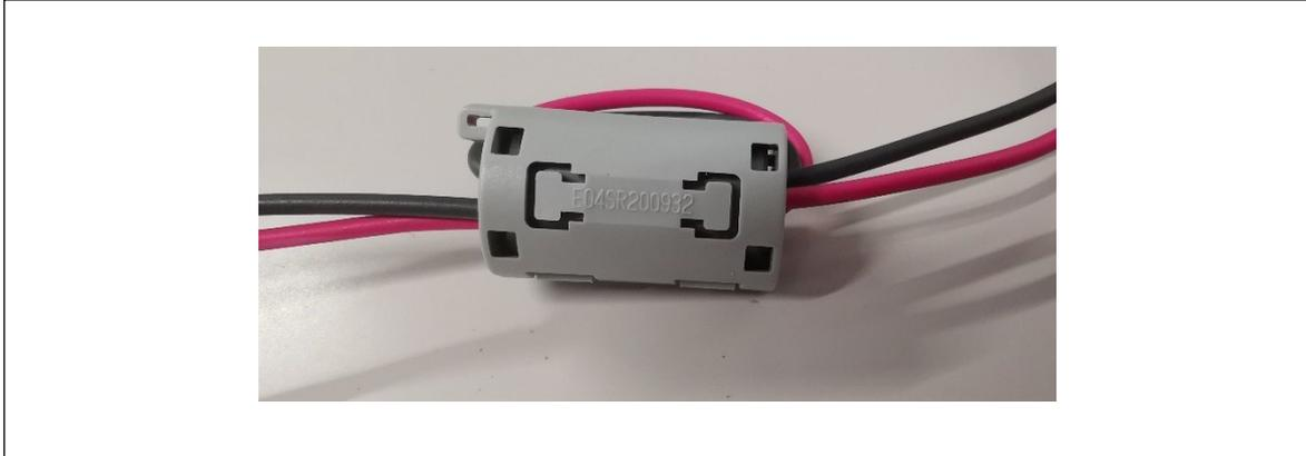
Figure 2-6 Ferrite Core
