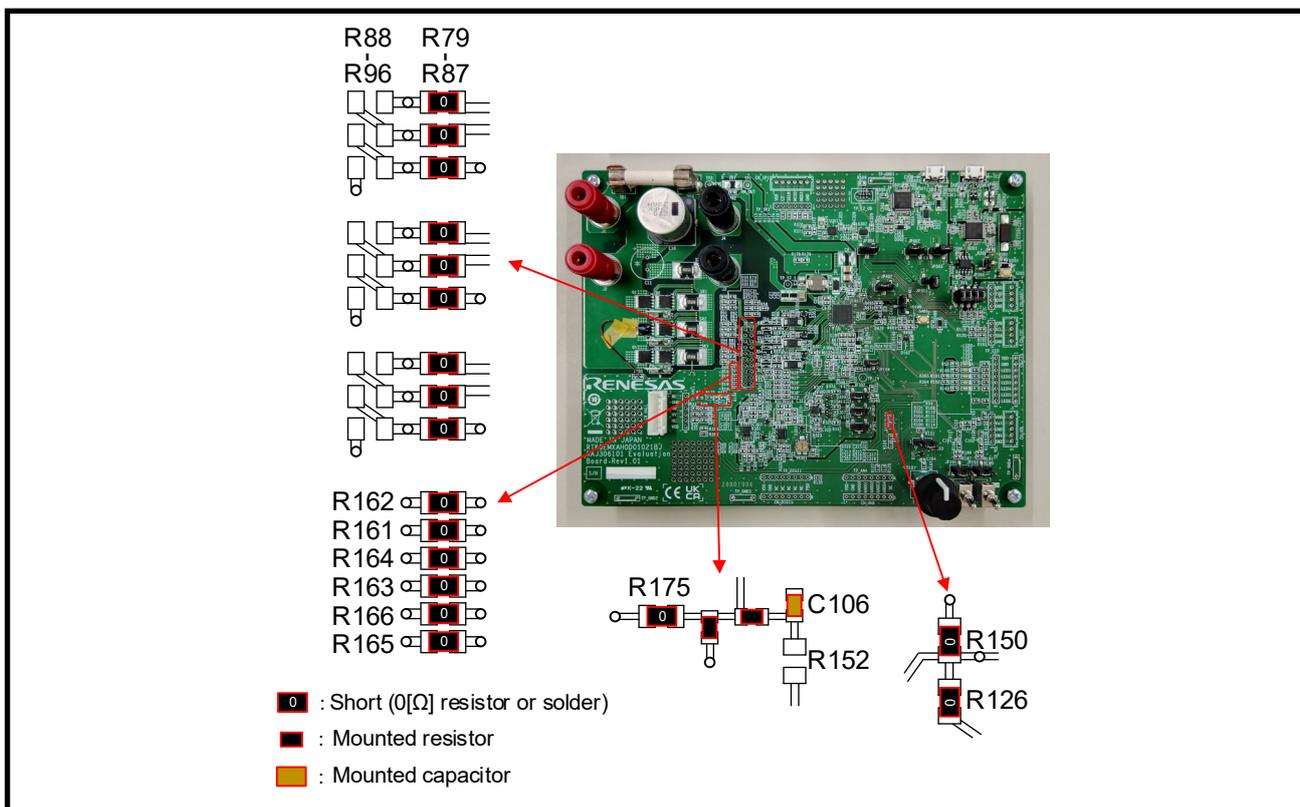
**Figure 4-3 Motor Drive Circuit Function Selection Resistors (Factory Default)**
