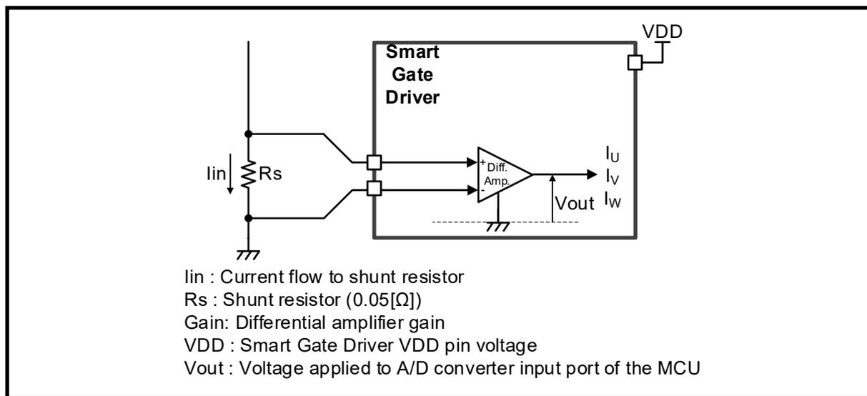
Figure 4-7 Current Sense Circuits (Internal)
