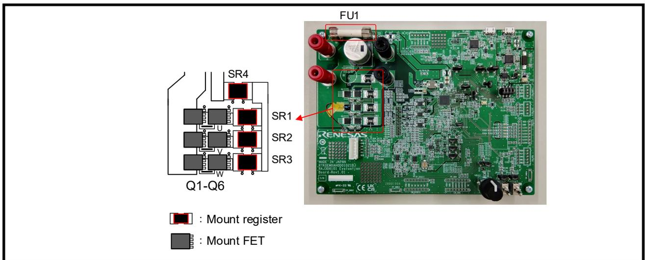
Figure 4-13 Components Change Location (Using Other Motor)
