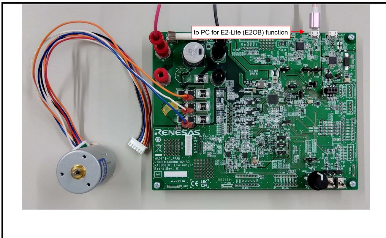
Figure 5-1 Connect with PC (E2 Lite Function)
