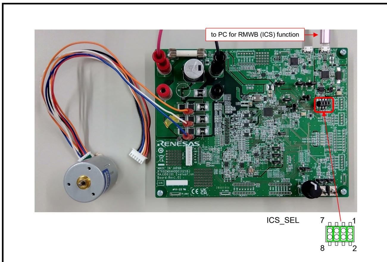
Figure 6-1 Connect with PC (RMWB (ICS) Function)
