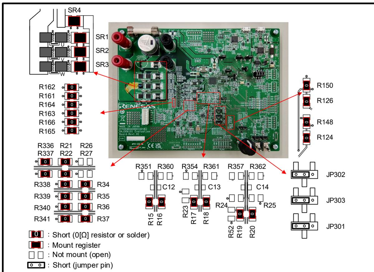
Figure 3-3 Board Connection Settings (Sensorless Vector Control)
