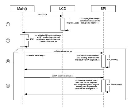
Figure 4-13: SPI Loopback Sequence Diagram
