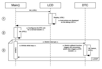
Figure 4-5: DTC Sequence Diagram
