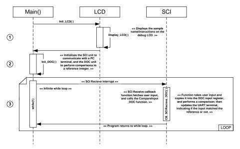
Figure 4-16: Data Operation Circuit (DOC) Sequence Diagram
