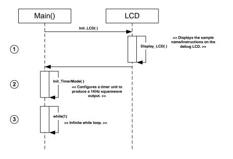
Figure 4-8: Timer Mode Sequence Diagram
