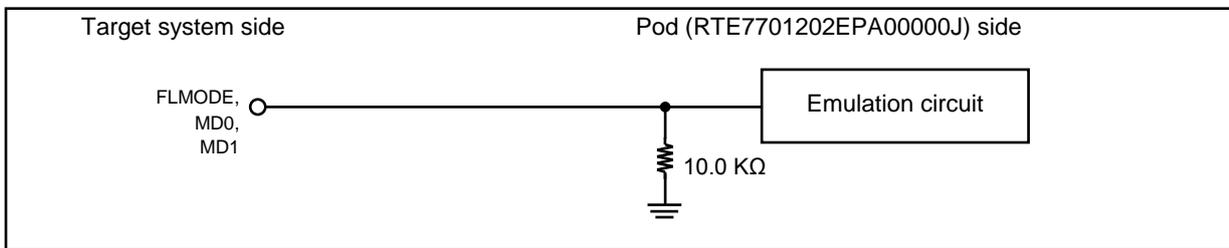
Figure A-5 Equivalent Circuit E
