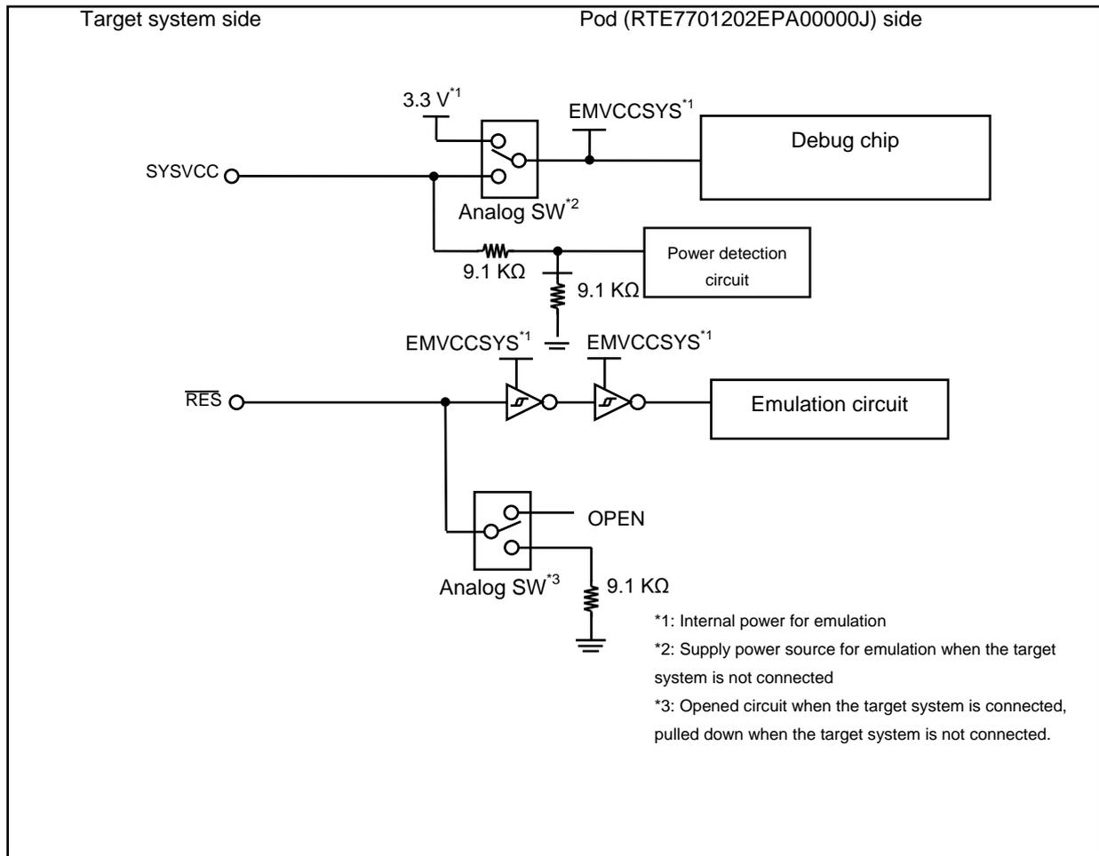
Figure A-8 Equivalent Circuit H
