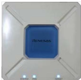
After the power is on, the TARGET LED lights up.
