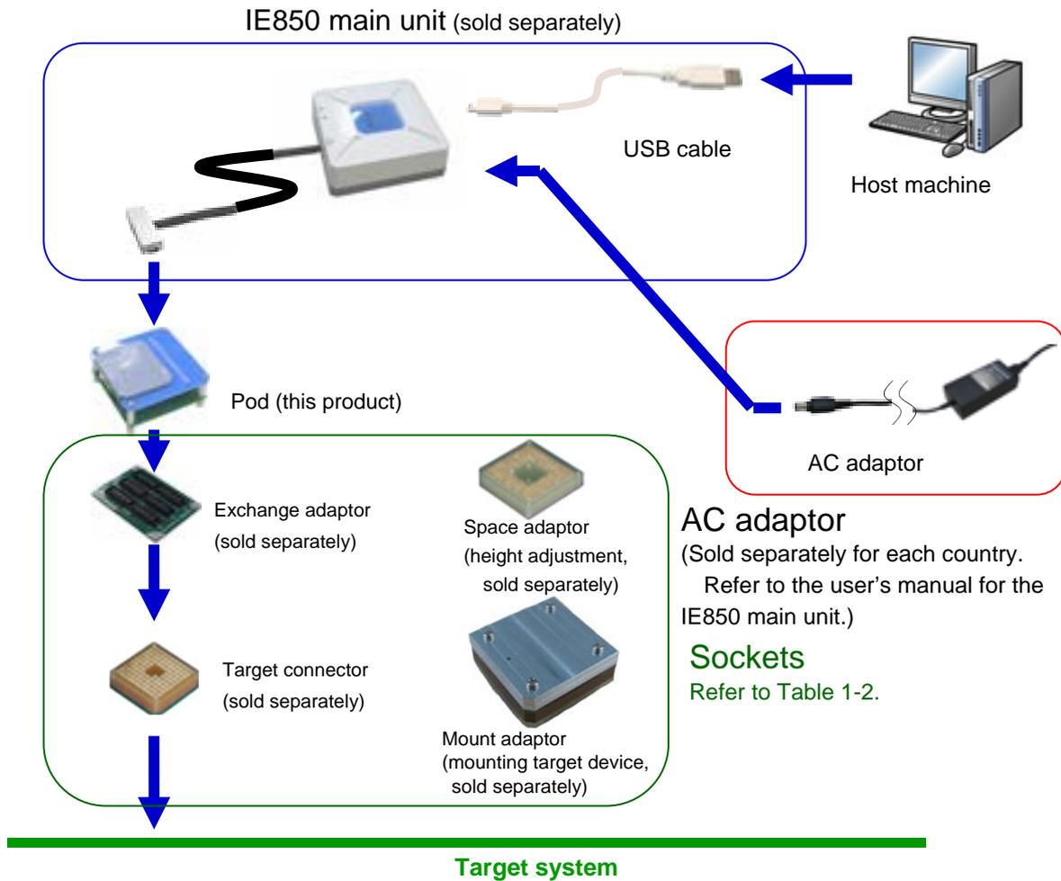
Figure 1-3 System Configuration (When the BGA Package is Selected)
