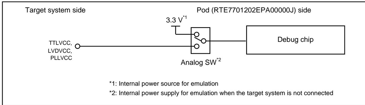
Figure A-4 Equivalent Circuit D
