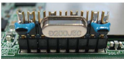
This product has a 20-MHz resonator. To change the resonator, connect a replacement to the IE850 main unit with reference to the positions of the resonator and capacitors as shown below.
