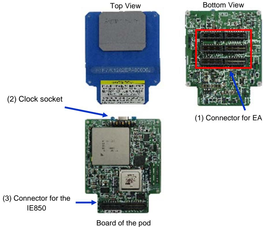
**Figure 2-1 Names of Parts of Pod**
