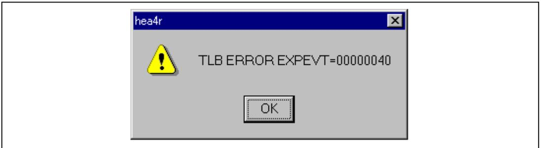
**Figure 2.1 Message Box for Clearing a TLB Error**
