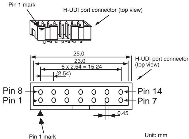
**Figure 1.1 Pin Assignments of the H-UDI Port Connector**
