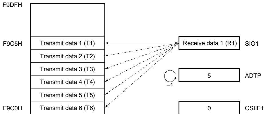
**Figure 10-9. Buffer RAM Operation in 6-Byte Transmission/Reception
