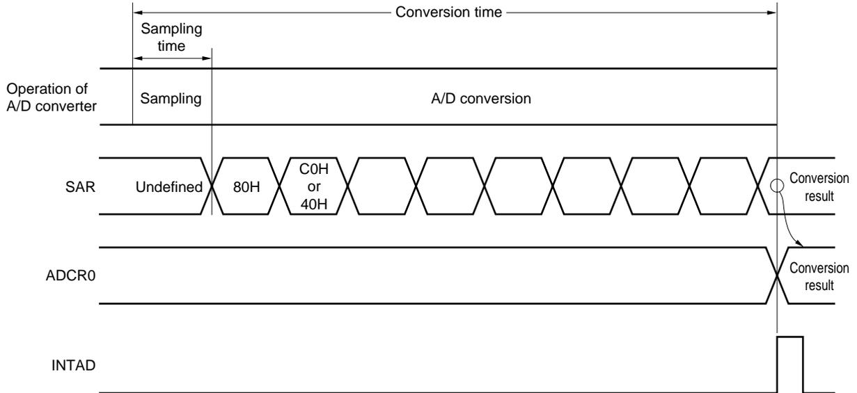
A/D conversion is performed continuously until bit 7 (ADCS0) of A/D converter mode register 0 (ADM0) is reset to 0 by software.
