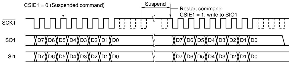
CSIE1: Bit 7 of serial operation mode register 1 (CSIM1)
