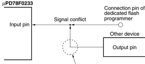
In the flash memory programming mode, the signal output by another device and the signal sent by the dedicated flash programmer conflict, therefore, isolate the signal of the other device.
