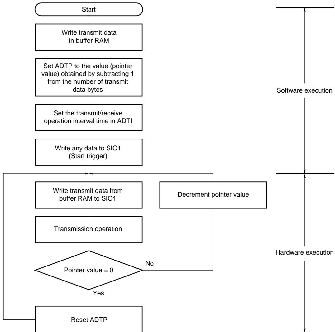
ADTP: Automatic data transmit/receive address pointer
