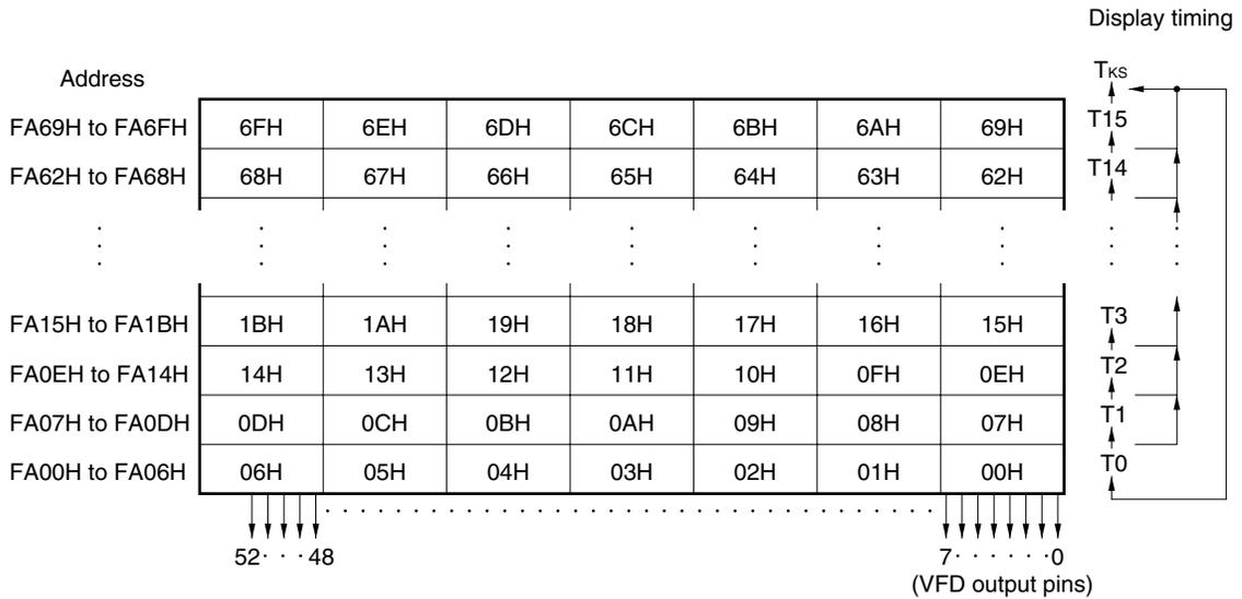
★ Regarding the display data memory, if 48 pins are used to display 1 pattern, the area that can be used as normal RAM is 1 byte, which increases by 1 byte for every 8-pin reduction. Moreover when the number of display patterns is 16 or less, whenever the number of patterns decreases, the area that can be used as normal RAM increases by 7 bytes each time.
