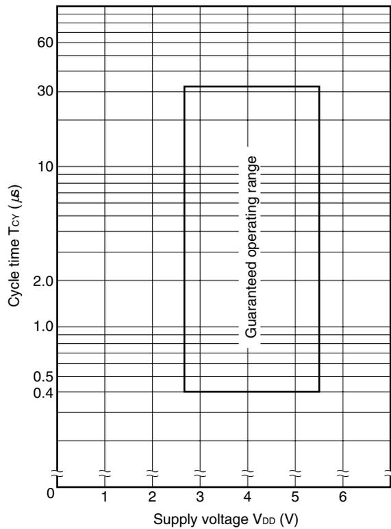
(2) Timer/counter ( $T_A = -40$  to  $+85^\circ\text{C}$ ,  $V_{DD} = 2.7$  to  $5.5$  V)
