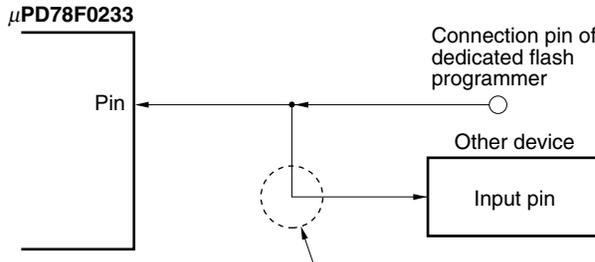
If the signal output by the dedicated flash programmer affects another device in the flash memory programming mode, isolate the signals of the other device.
