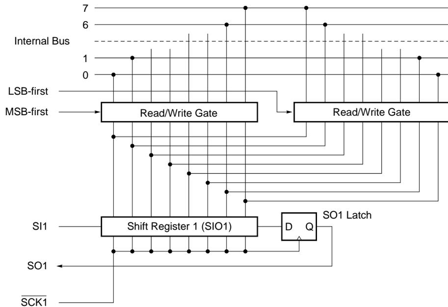
Start bit switching is realized by switching the bit order for data write to SIO1. The SIO1 shift order remains unchanged.
