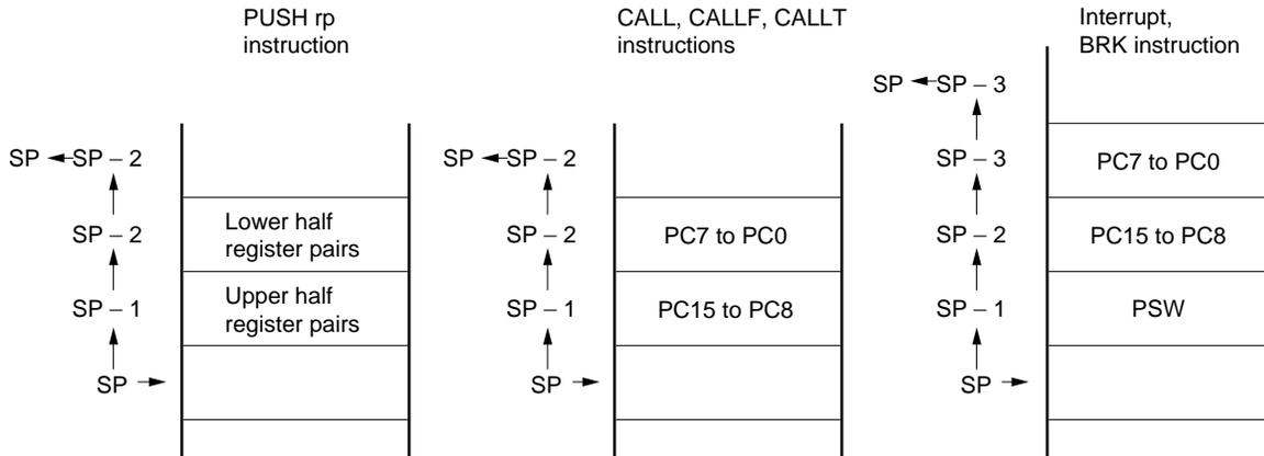
Figure 3-11. Data Restored from Stack Memory
