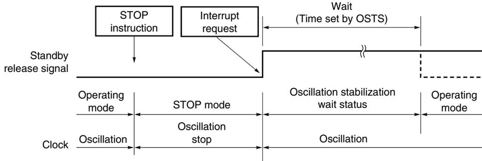
**Remark** The broken line indicates the case when the interrupt request which has cleared the standby status is acknowledged.
