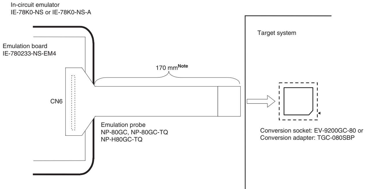
**Note** When NP-H80GC-TQ is used, the distance is 370 mm.
