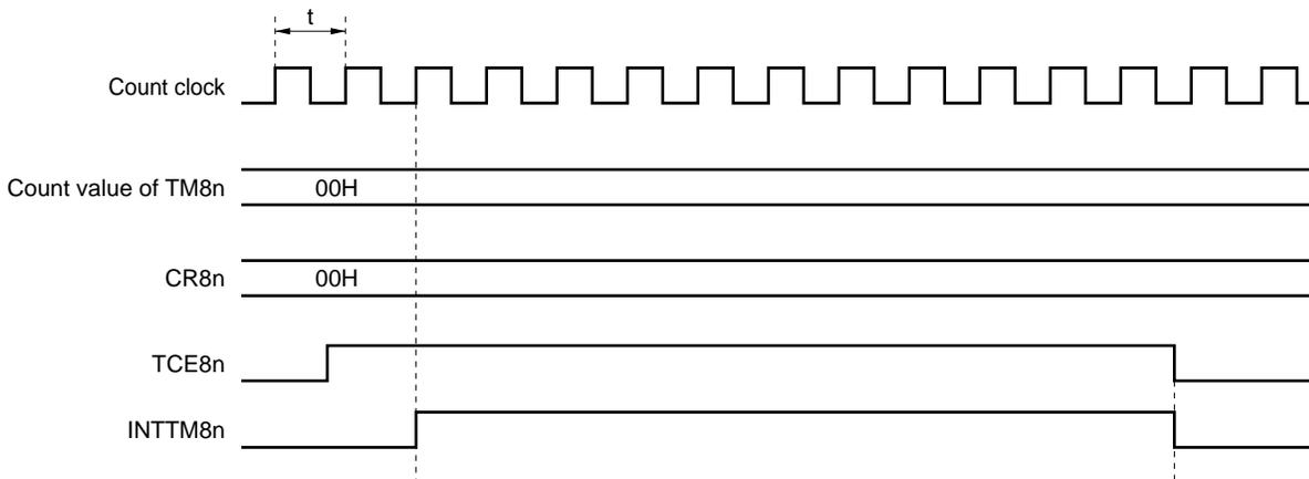
**Caution** When 00H is assigned to the CR8n, INTTM8n is fixed to high and a valid edge is output only at the first time.
