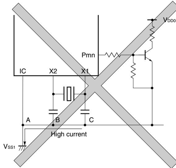
Figure 5-4. Examples of Incorrect Resonator Connection (2/2)
