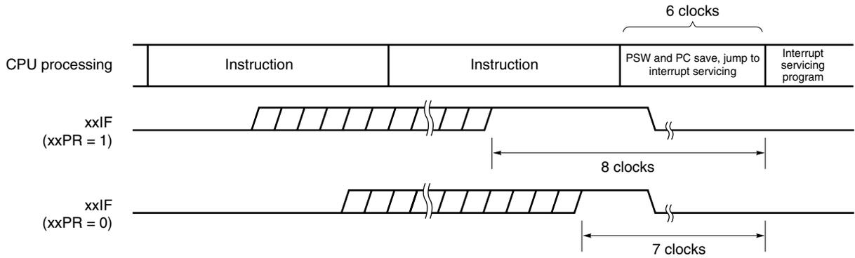
**Remark** 1 clock:  $\frac{1}{f_{CPU}}$  ( $f_{CPU}$ : CPU clock)
