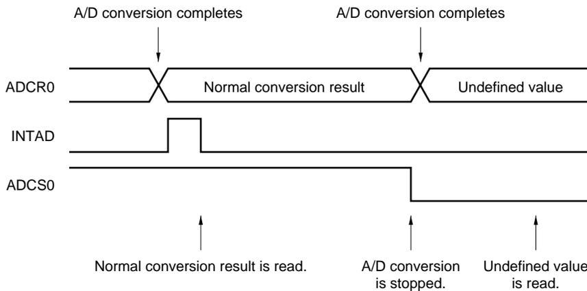
**Figure 9-14. Timing of Reading Conversion Result (When Conversion Result Is Normal)**
