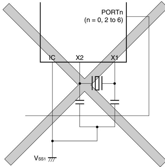
(c) Wiring near high fluctuating current
