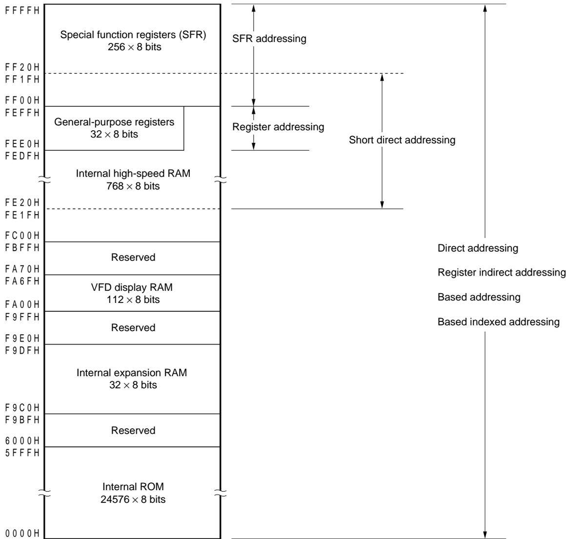
Figure 3-6. Data Memory Addressing ( $\mu$ PD78F0233)
