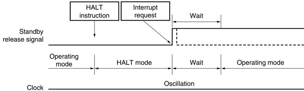
**Remarks 1.** The broken line indicates the case when the interrupt request which has released the standby status is acknowledged.
