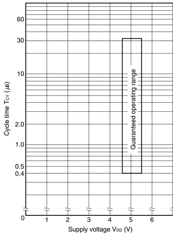
(2) Timer/counter ( $T_A = -40$  to  $+85^\circ\text{C}$ ,  $V_{DD} = 4.5$  to  $5.5$  V)
