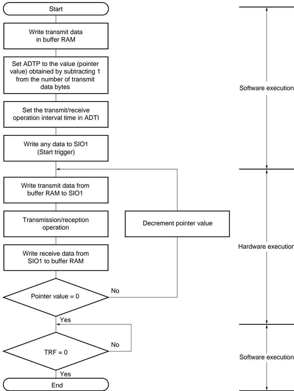
ADTP: Automatic data transmit/receive address pointer
