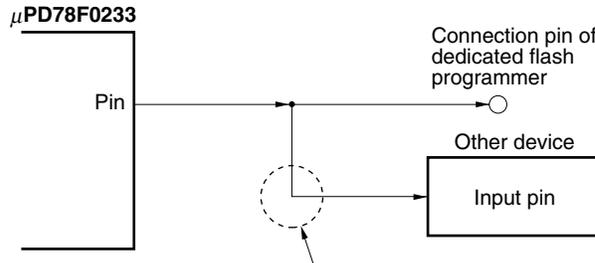
If the signal output by the  $\mu$ PD78F0233 affects another device in the flash memory programming mode, isolate the signals of the other device.
