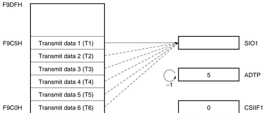
Figure 10-12. Buffer RAM Operation in 6-Byte Transmission (in Basic Transmit Mode) (2/2)
