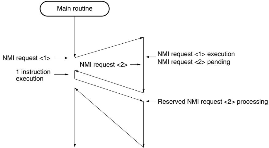
(b) If two non-maskable interrupt requests occur during non-maskable interrupt servicing program execution
