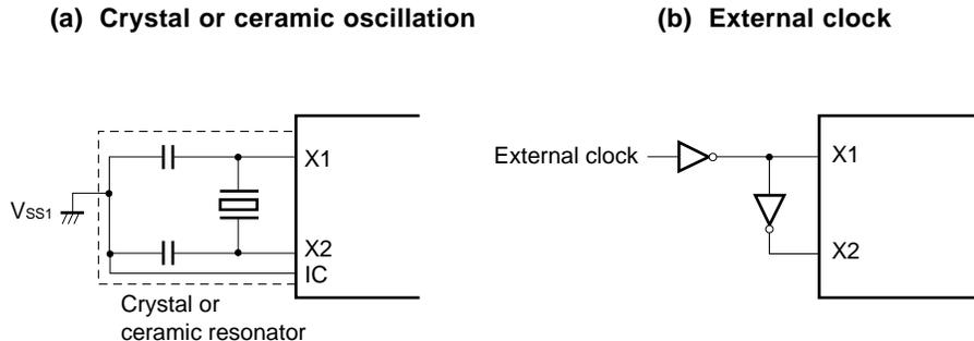
**Cautions** 1. The STOP mode cannot be set when the external clock is input. This is because the X2 pin is pulled up by  $V_{DD1}$ .
