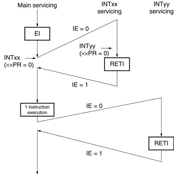
Because interrupts are not enabled (the EI instruction is not issued) in interrupt servicing INTxx, interrupt request INTyy is not acknowledged, and therefore, the interrupt is not nested. INTyy request is held pending, and is acknowledged after main processing one instruction has been executed.
