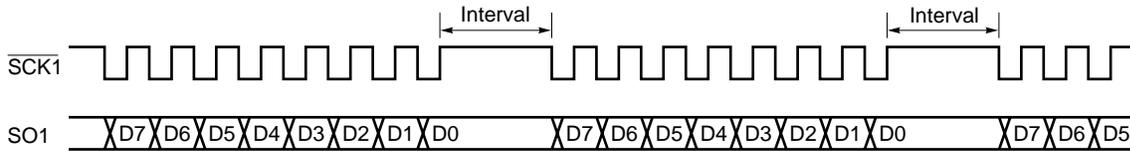
**Caution** Since, in the repeat transmit mode, a read is performed on the buffer RAM after the transmission of one byte, the interval is included in the period up to the next transmission. As the buffer RAM read is performed at the same time as CPU processing, the maximum interval is dependent upon the CPU operation and the value of the automatic data transmit/receive interval specification register (ADTI) (refer to (6) Automatic data transmit/receive interval).
