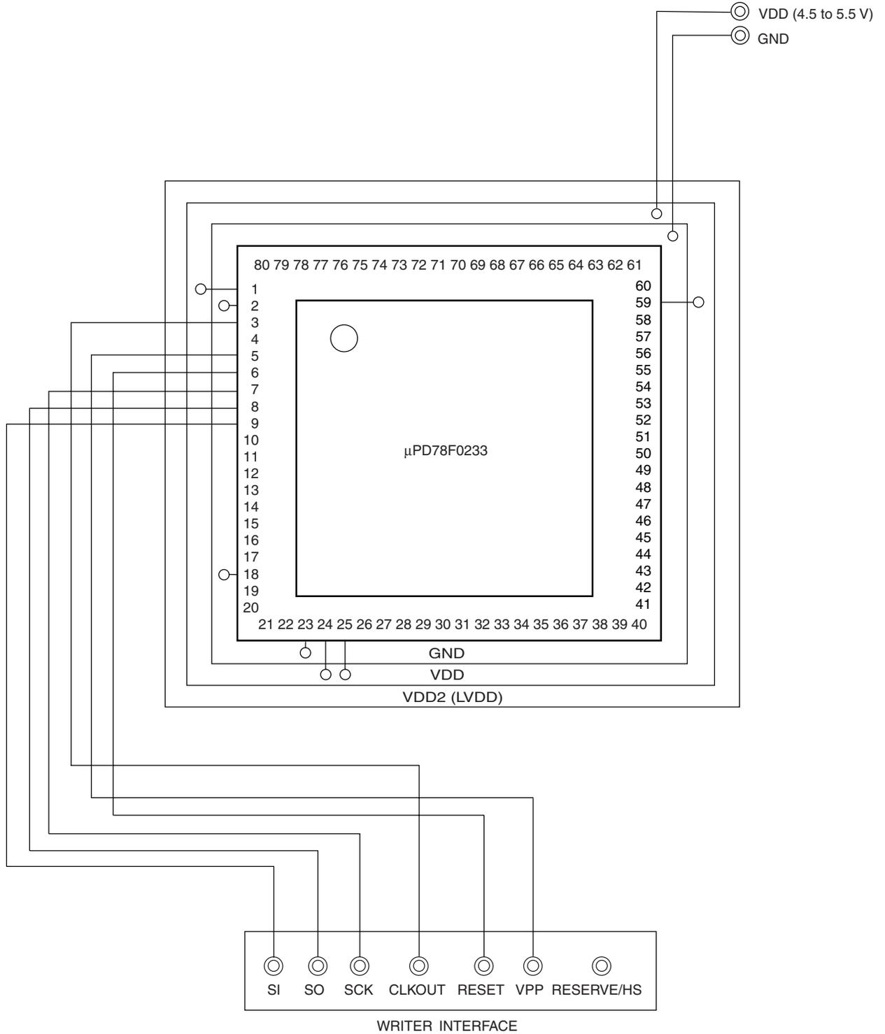
Figure 16-10. Wiring Example for Flash Writing Adapter with Pseudo 3-Wire Serial I/O
