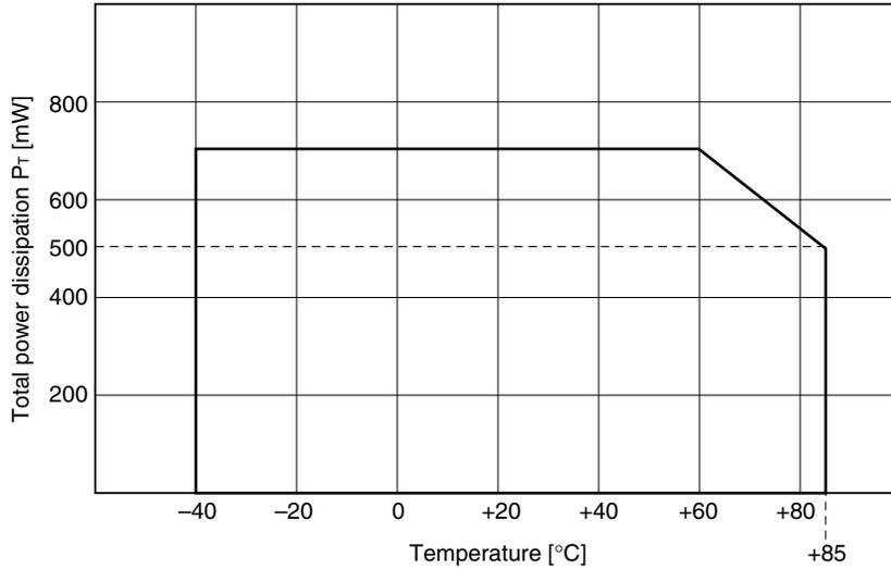
**How to calculate total power dissipation**
