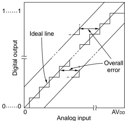
Figure 9-8. Quantization Error
