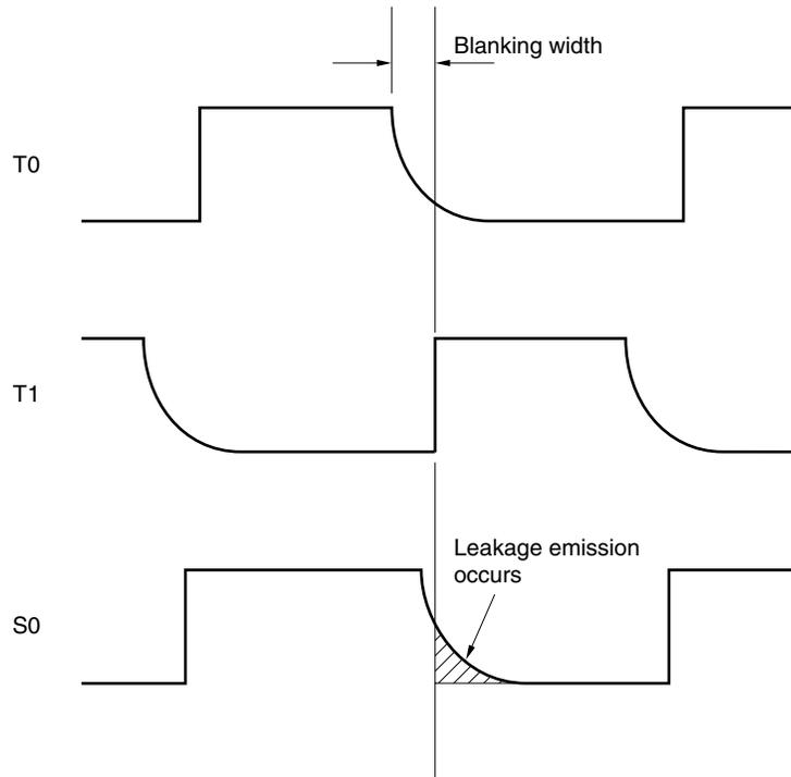
**(2) Segment-grid capacitance of fluorescent indicator panel**
