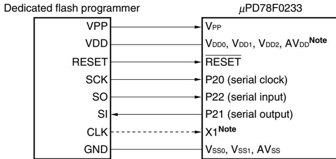
**Note** The power can be supplied to the VDD0, VDD1, VDD2, AVDD, and X1 pins on the board. In this case, although it is not required to connect the dedicated flash programmer, VDD voltage must be supplied before programming is started.
