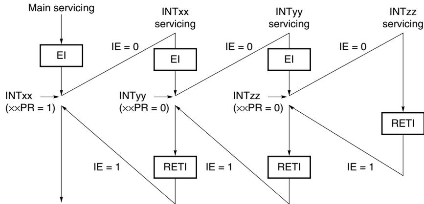
Two interrupt requests INTyy and INTzz are acknowledged and nesting is generated when interrupt INTxx request is being serviced. Before each interrupt request is acknowledged, the EI instruction is always issued and the interrupt request is enabled.
