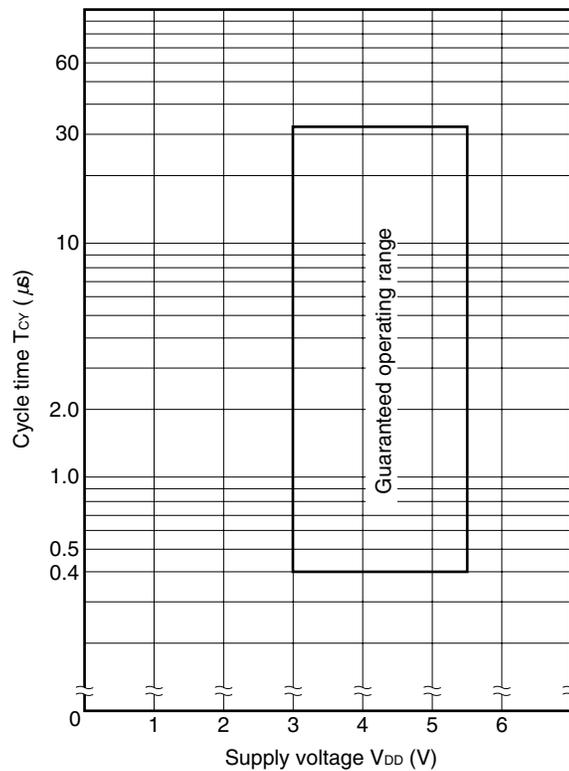
(2) Timer/counter ( $T_A = -40$  to  $+85^\circ\text{C}$ ,  $V_{DD} = 3.0$  to  $5.5$  V)
