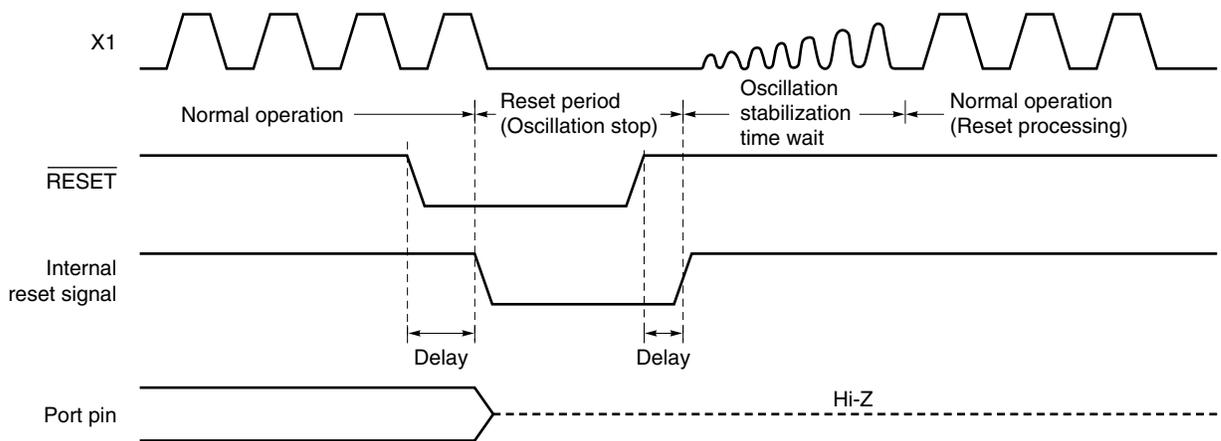
Figure 15-3. Timing of Reset Due to Watchdog Timer Overflow
