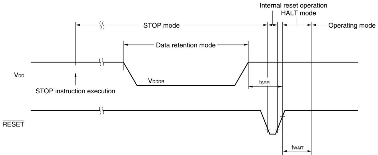
Data retention timing (standby release signal: STOP mode release by interrupt request signal)
