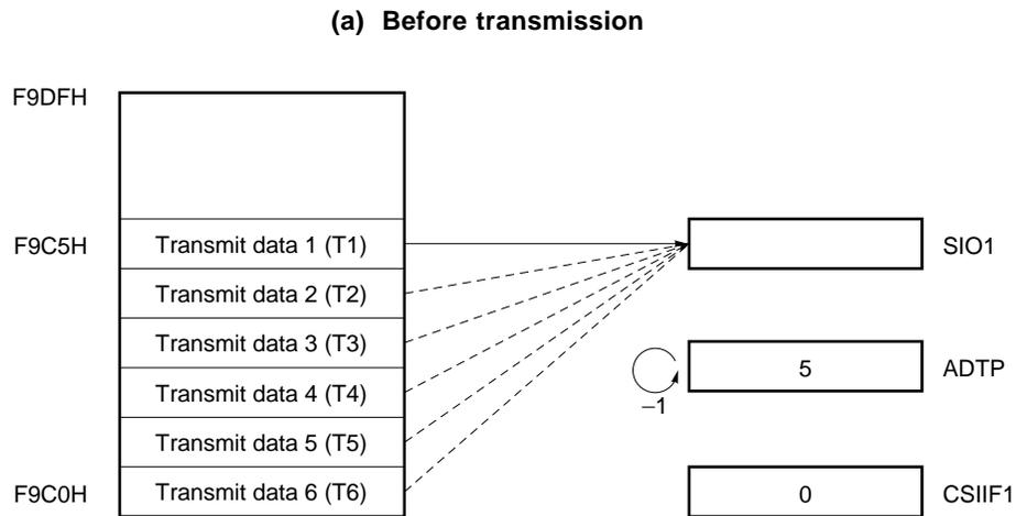
Figure 10-15. Buffer RAM Operation in 6-Byte Transmission (in Repeat Transmit Mode) (2/2)
