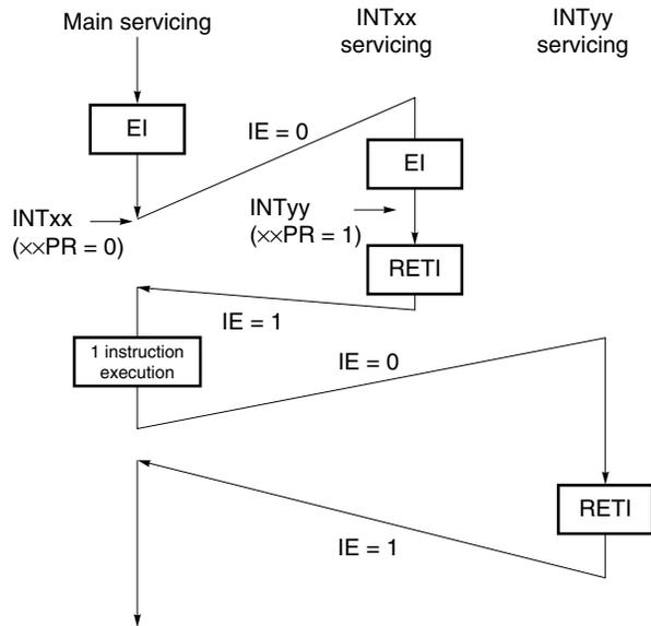
INTyy which is generated while INTxx is being serviced is not acknowledged and a nesting is not generated, because the priority of INTyy is lower than that of INTxx. INTyy is held pending and is acknowledged after one instruction of the main servicing has been executed.
