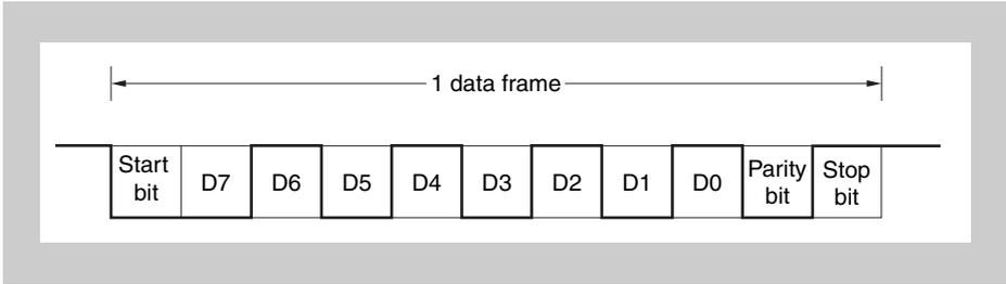
(c) 8-bit data length, MSB first, even parity, 1 stop bit, transfer data: 55<sub>H</sub>, URTE<sub>n</sub>TTXD inversion
