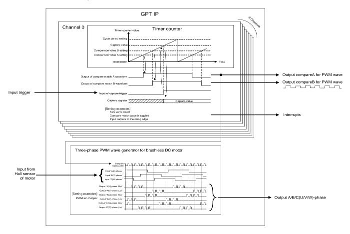
Note: 3-phase means full wave 6-outputs(A-Up, A-Lo, B-Up, B-Lo, C-Up, C-Lo). U/V/W are another names of A/B/C.
