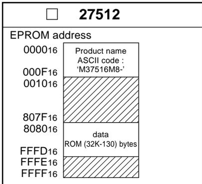
In the address space of the microcomputer, the internal ROM area is from address 8080<sub>16</sub> to FFFD<sub>16</sub>. The reset vector is stored in addresses FFFC<sub>16</sub> and FFFD<sub>16</sub>.
