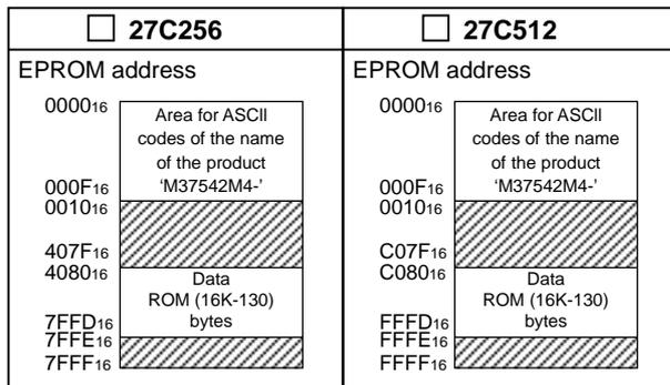
In the address space of the microcomputer, the internal ROM area is from address C080<sub>16</sub> to FFFD<sub>16</sub>. The reset vector is stored in addresses FFFC<sub>16</sub> and FFFD<sub>16</sub>.
