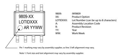
Figure 8.1: Top Marking for the iW9809
