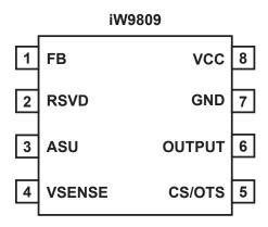
Figure 4.1: 8-Lead SOIC Package
