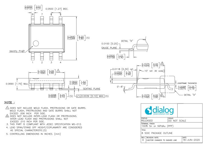
Figure 6.1: 8-Lead SOIC package outline drawing
