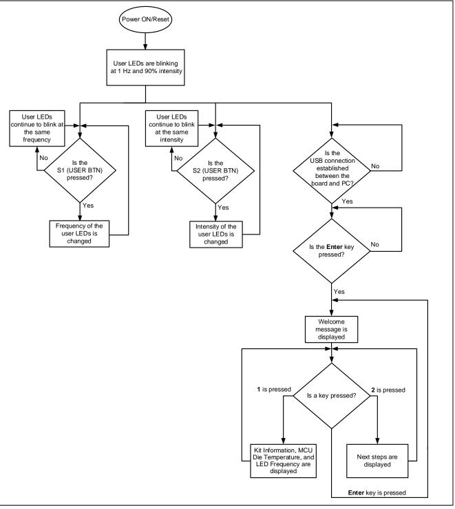
Figure 2. Quick Start Example Project Flow
