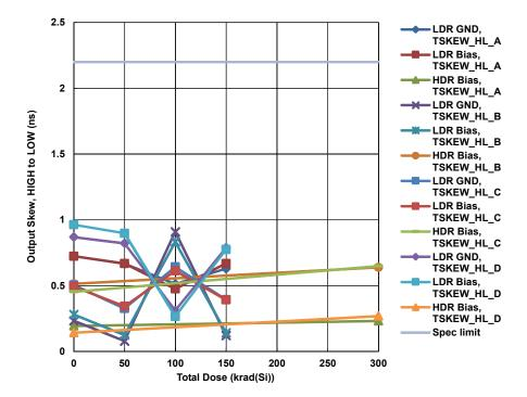
Figure 17. HS-26C31EH HIGH to LOW output skew, channels A through D, as a function of biased HDR total dose irradiation to 300krad(Si) and biased and unbiased (grounded) LDR irradiation to 150krad(Si). The sample size for the HDR cell was 48, while the sample sizes for the LDR cells were 20 each. SMD limit is 3ns maximum; the internal ATE limit (shown) is 2.2ns maximum.
