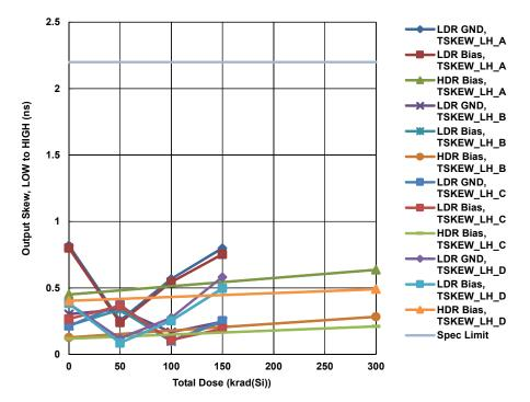
Figure 16. HS-26C31EH LOW to HIGH output skew, channels A through D, as a function of biased HDR total dose irradiation to 300krad(Si) and biased and unbiased (grounded) LDR irradiation to 150krad(Si). The sample size for the HDR cell was 48, while the sample sizes for the LDR cells were 20 each. The SMD limit is 3ns maximum; the internal ATE limit (shown) is 2.2ns maximum.
