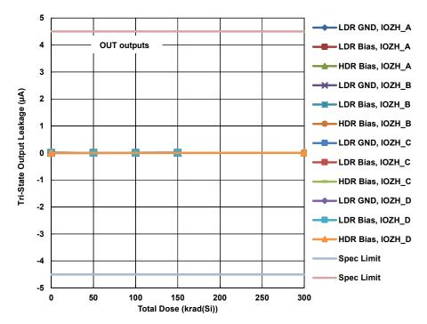
Figure 4. HS-26C31EH tristate output leakage, OUT outputs, channels A through D, as a function of biased HDR total dose irradiation to 300krad(Si) and biased and unbiased (grounded) LDR irradiation to 150krad(Si). The sample size for the HDR cell was 48, while the sample sizes for the LDR cells were 20 each. The SMD limits are -5µA to 5µA; the internal ATE limits (shown) are -4.5µA to 4.5µA.
