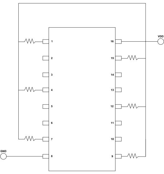
Figure 2. Irradiation Bias Configuration
