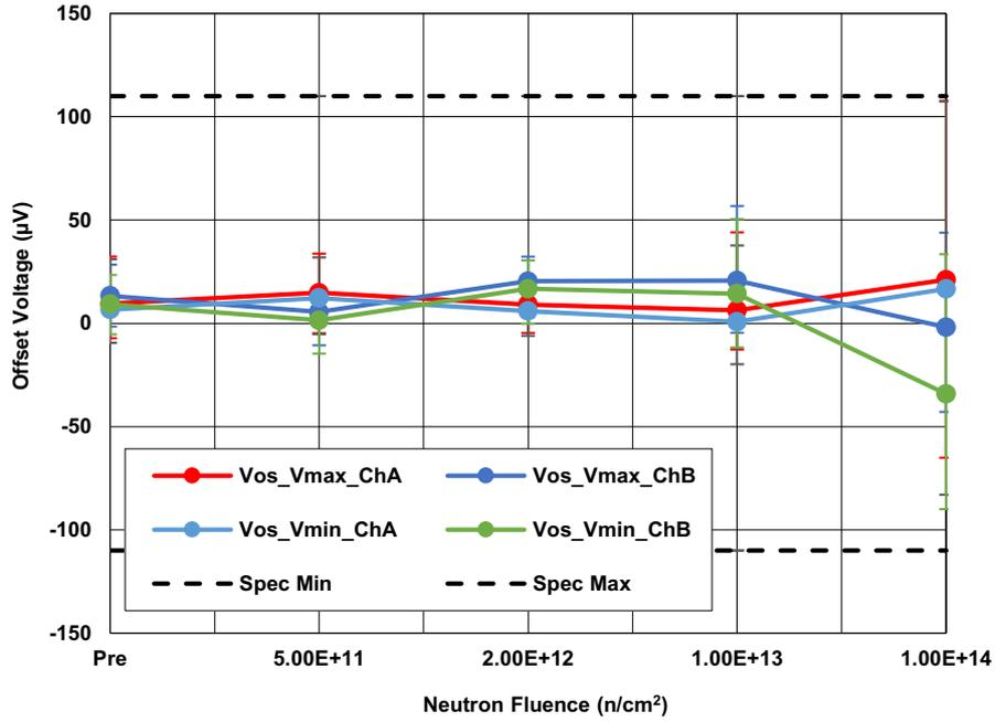
Figure 6. ISL70219ASEH Input Offset Voltage (V<sub>OS</sub>), Channels A and B, with V<sub>S</sub> = ±18V and ±2.25V, following irradiation to each level. The error bars (if visible) represent the minimum and maximum measured values. The SMD limits -110µV minimum and 110µV maximum.
