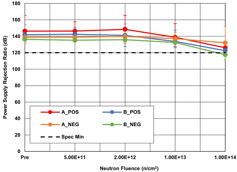
Figure 14. ISL70219ASEH Power Supply Rejection Ratio (PSRR), Channels A and B, with  $V_S = \pm 5V$ , following irradiation to each level. The error bars (if visible) represent the minimum and maximum measured values. The SMD limit is 120dB minimum.
