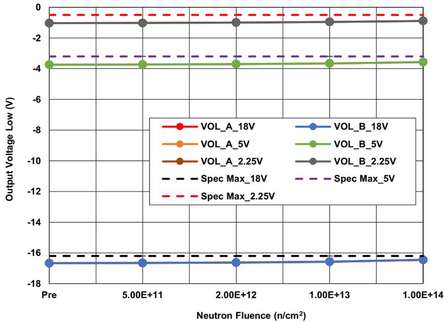
Figure 3. ISL70219ASEH Output Voltage Low (V<sub>OL</sub>), Channels A and B, with V<sub>S</sub> = ±18V, ±5V, and ±2.25V, R<sub>L</sub> = 10kΩ, following irradiation to each level. The error bars (if visible) represent the minimum and maximum measured values. The SMD limits are -16.2V maximum for V<sub>S</sub> = ±18V, -3.2V maximum for V<sub>S</sub> = ±5V, and -0.5V maximum for V<sub>S</sub> = ±2.25V.
