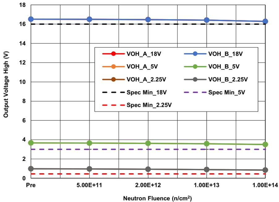
Figure 2. ISL70219ASEH Output Voltage High (V<sub>OH</sub>), Channels A and B, with V<sub>S</sub> = ±18V, ±5V, and ±2.25V, R<sub>L</sub> = 2kΩ, following irradiation to each level. The error bars (if visible) represent the minimum and maximum measured values. The SMD limits are 16V minimum for V<sub>S</sub> = ±18V, 3V minimum for V<sub>S</sub> = ±5V, and 0.45V minimum for V<sub>S</sub> = ±2.25V.
