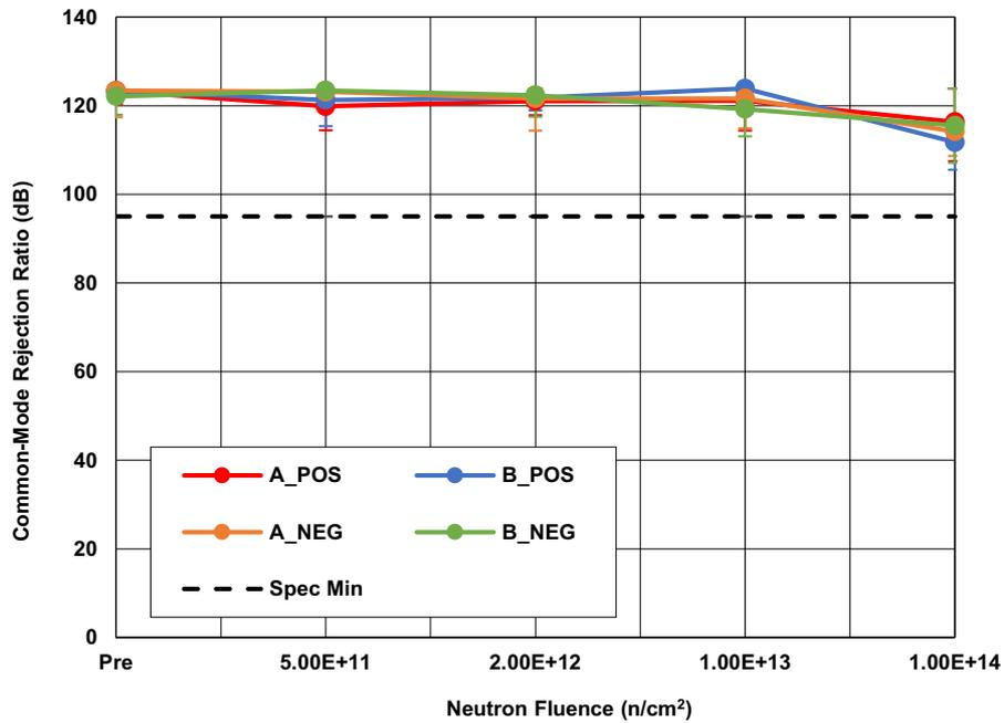
Figure 17. ISL70219ASEH Common-Mode Rejection Ratio (CMRR), Channels A and B, with  $V_S = \pm 2.25V$ , following irradiation to each level. The error bars (if visible) represent the minimum and maximum measured values. The SMD limit is 95dB minimum.
