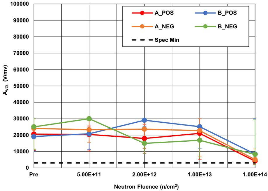
Figure 12. ISL70219ASEH Open-Loop Gain ( $A_{VOL}$ ), Channels A and B, with  $V_S = \pm 5V$ , following irradiation to each level. The error bars (if visible) represent the minimum and maximum measured values. The SMD limit is 3000V/mV minimum.
