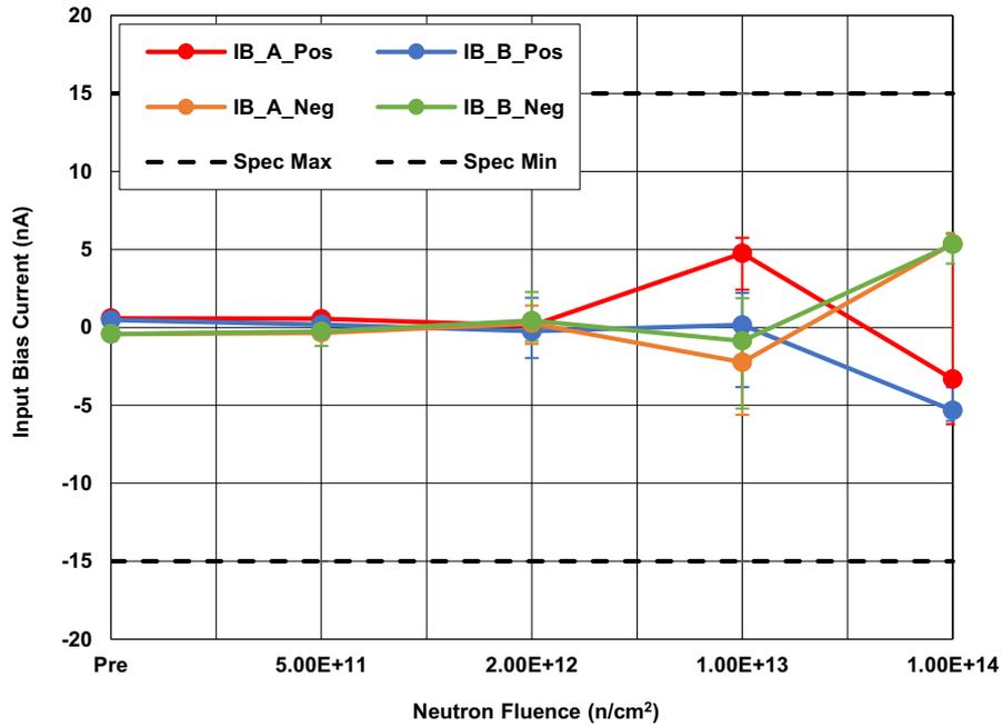
Figure 7. ISL70219ASEH Input Bias Current (I<sub>B</sub>), Channels A and B, with V<sub>S</sub> = ±18V, following irradiation to each level. The error bars (if visible) represent the minimum and maximum measured values. The SMD limits are -15nA minimum and 15nA maximum.
