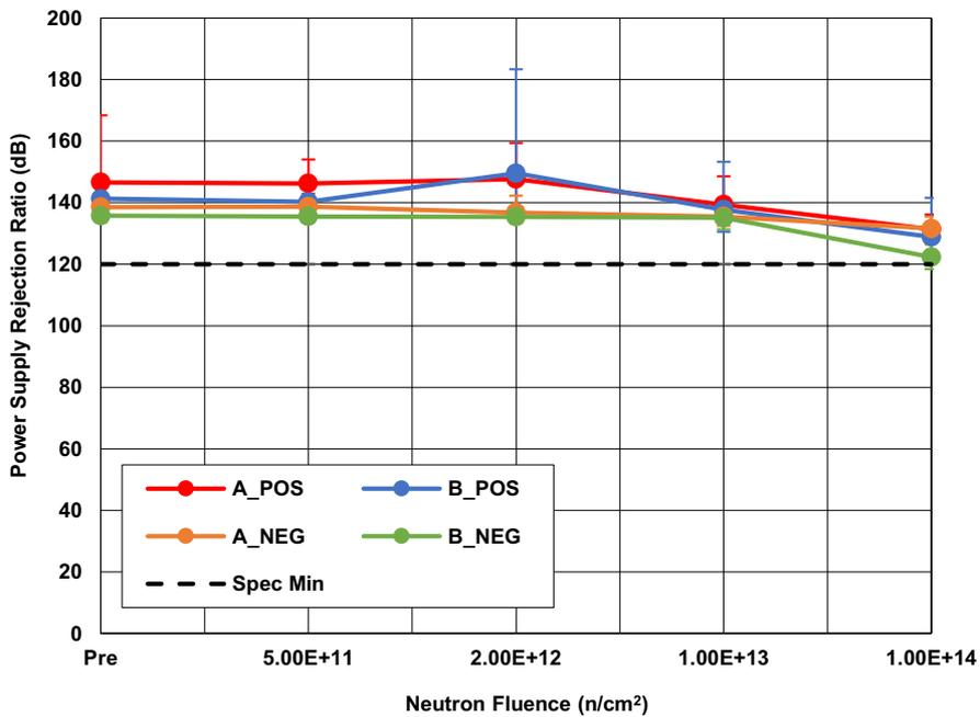
Figure 13. ISL70219ASEH Power Supply Rejection Ratio (PSRR), Channels A and B, with  $V_S = \pm 18V$ , following irradiation to each level. The error bars (if visible) represent the minimum and maximum measured values. The SMD limit is 120dB minimum.
