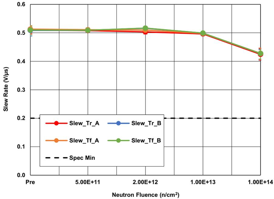
Figure 18. ISL70219ASEH Slew Rate (SR), Channels A and B, with  $V_S = \pm 18V$ ,  $A_V = 1$ ,  $R_L = 2k\Omega$ , following irradiation to each level. The error bars (if visible) represent the minimum and maximum measured values. The SMD limit is 0.2V/μs minimum.
