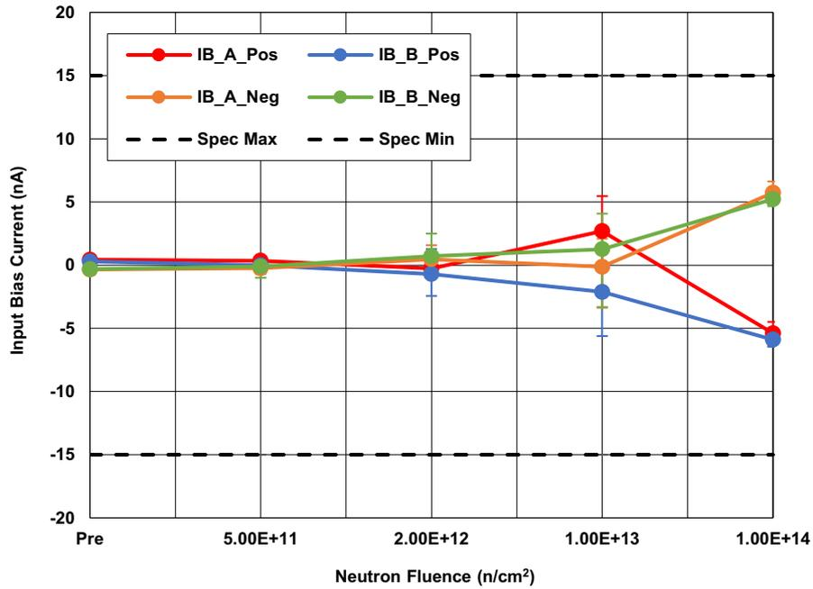
Figure 9. ISL70219ASEH Input Bias Current ( $I_B$ ), Channels A and B, with  $V_S = \pm 2.25V$ , following irradiation to each level. The error bars (if visible) represent the minimum and maximum measured values. The SMD limits are -15nA minimum and 15nA maximum.
