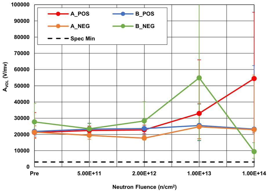
Figure 11. ISL70219ASEH Open-Loop Gain ( $A_{VOL}$ ), Channels A and B, with  $V_S = \pm 18V$ , following irradiation to each level. The error bars (if visible) represent the minimum and maximum measured values. The SMD limit is  $3000V/mV$  minimum.
