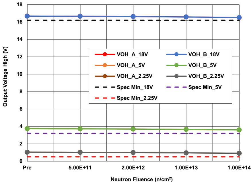
Figure 1. ISL70219ASEH Output Voltage High (V<sub>OH</sub>), Channels A and B, with V<sub>S</sub> = ±18V, ±5V, and ±2.25V, R<sub>L</sub> = 10kΩ, following irradiation to each level. The error bars (if visible) represent the minimum and maximum measured values. The SMD limits are 16.2V minimum for V<sub>S</sub> = ±18V, 3.2V minimum for V<sub>S</sub> = ±5V, and 0.5V minimum for V<sub>S</sub> = ±2.25V.
