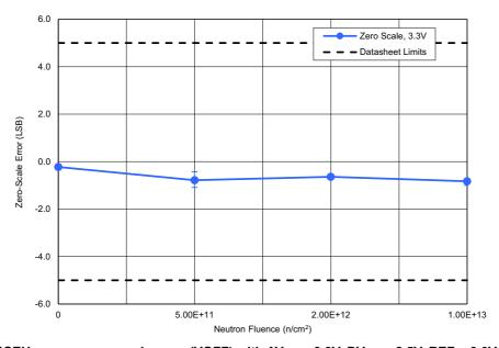
Figure 4. ISL73141SEH average zero scale error (VOFF) with  $AV_{CC}$  = 3.3V,  $DV_{CC}$  = 2.5V, REF = 3.0V,  $f_{SAMP}$  = 750ksps, and  $A_{IN}$  = GND following irradiation to each level. The error bars (if visible) represent the minimum and maximum measured values. The post – TID irradiation datasheet limits are a minimum of -5LSB with a maximum of 5LSB.
