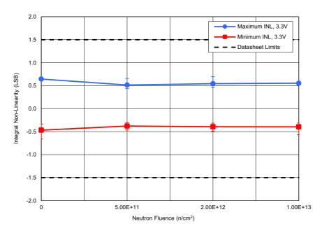
Figure 2. ISL73141SEH average minimum and maximum integral non-linearity (INL) with AV<sub>CC</sub> = 3.3V, DV = 2.5V, REF = 3.0V,  $f_{SAMP}$  = 750ksps, and  $A_{IN}$  = full-scale sine wave following irradiation to each level. The error bars (if visible) represent the minimum and maximum measured values. The post – TID irradiation datasheet limits are a minimum of -1.5LSB with a maximum of 1.5LSB.
