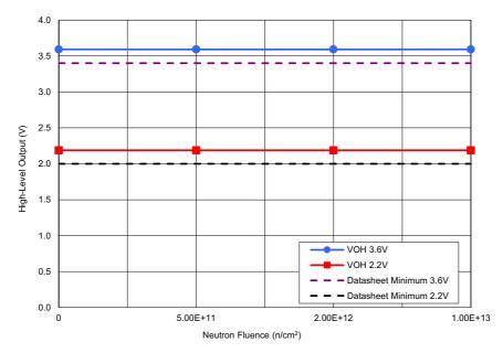
Figure 21. ISL73141SEH average high-level output ( $V_{OH}$ ) with AV $_{CC}$  = 3.3V, DV $_{CC}$  = 3.6V and 2.2V, REF = 3.0V, and  $I_{O}$  = -500 $\mu$ A following irradiation to each level. The error bars (if visible) represent the minimum and maximum measured values. The post – TID irradiation datasheet limits are minimums of 3.4V for DV $_{CC}$  = 3.6V and 2.0V for DV $_{CC}$  = 2.2V.
