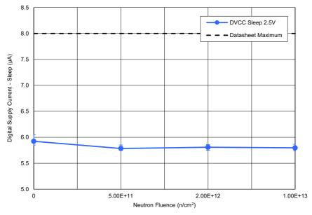
Figure 18. ISL73141SEH average digital supply current – sleep ( $I_{SLDVCC}$ ) with AV<sub>CC</sub> = 3.3V, DV<sub>CC</sub> = 2.5V, REF = 3.0V, and PD = GND following irradiation to each level. The error bars (if visible) represent the minimum and maximum measured values. The post – TID irradiation datasheet limit is a maximum of  $8\mu$ A.
