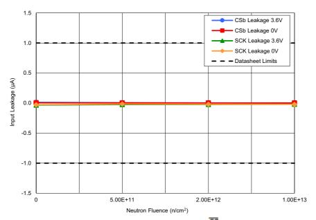
Figure 20. ISL73141SEH average input leakage current ( $I_{IN}$ ) on SCK and  $\overline{CS}$  with AV<sub>CC</sub> = 3.3V, DV<sub>CC</sub> = 2.5V, REF = 3.0V, and V<sub>IN</sub> = 3.6V and 0V following irradiation to each level. The error bars (if visible) represent the minimum and maximum measured values. The post – TID irradiation datasheet limits are a minimum of -1 $\mu$ A with a maximum of 1 $\mu$ A.
