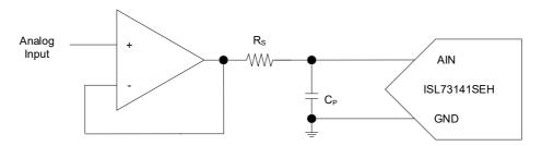
Figure 1. Typical Application Schematic
