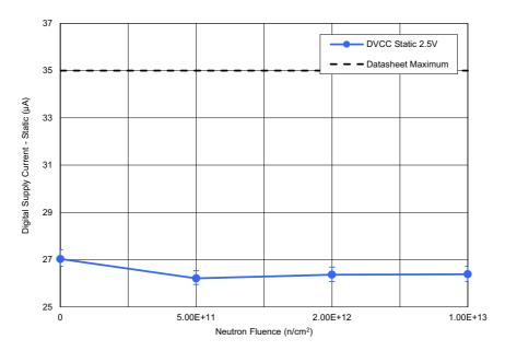
Figure 17. ISL73141SEH average digital supply current – static ( $I_{STDVCC}$ ) with AV<sub>CC</sub> = 3.3V, DV<sub>CC</sub> = 2.5V, REF = 3.0V, and CS = DV<sub>CC</sub> following irradiation to each level. The error bars (if visible) represent the minimum and maximum measured values. The post – TID irradiation datasheet limit is a maximum of 35 $\mu$ A.
