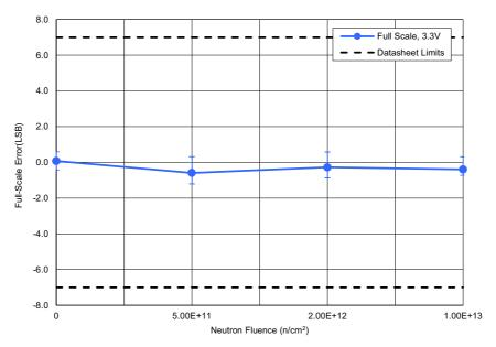
Figure 5. ISL73141SEH average full-scale error (FSE) with AV $_{CC}$  = 3.3V, DV $_{CC}$  = 2.5V, REF = 3.0V, f $_{SAMP}$  = 750ksps, and A $_{IN}$  = VREF following irradiation to each level. The error bars (if visible) represent the minimum and maximum measured values. The post – TID irradiation datasheet limits are a minimum of -7LSB with a maximum of 7LSB.
