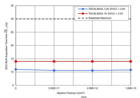
Figure 29. ISL73141SEH average SDO bus acquisition time from CS falling edge ( $t_{DCSLSDOL}$ ) with AV<sub>CC</sub> = 3.6V, DV<sub>CC</sub> = 3.6V and AV<sub>CC</sub> = 3.0V, DV<sub>CC</sub> = 2.2V, REF = 3.0V,  $t_{SAMP}$  = 750ksps, A<sub>IN</sub> = -1dBFS, and C<sub>L</sub> = 10pF following irradiation to each level. The error bars (if visible) represent the minimum and maximum measured values. The post – TID irradiation datasheet limit is a maximum of 30ns.
