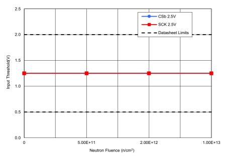
Figure 19. ISL73141SEH average high-level input ( $V_{IH}$ ) and low-level input ( $V_{IL}$ ) with AV<sub>CC</sub> = 3.3V, DV<sub>CC</sub> = 2.5V, and REF = 3.0V following irradiation to each level. The error bars (if visible) represent the minimum and maximum measured values. The post – TID irradiation datasheet limits are a 2.0V minimum for  $V_{IH}$  and a 0.5V maximum for  $V_{IL}$ .
