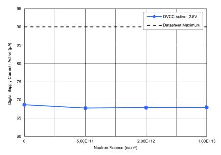
Figure 16. ISL73141SEH average digital supply current – active ( $I_{DVCC}$ ) with AV $_{CC}$  = 3.3V, DV $_{CC}$  = 2.5V, REF = 3.0V,  $I_{SCK}$  = 33MHz, and  $I_{CC}$  = 10pF following irradiation to each level. The error bars (if visible) represent the minimum and maximum measured values. The post – TID irradiation datasheet limit is a maximum of 90 $\mu$ A.
