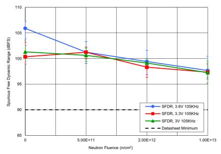
Figure 10. ISL73141SEH average spurious free dynamic range (SFDR) with AV $_{CC}$  = 3.6V, 3.3V and 3.0V, DV $_{CC}$  = 2.5V, REF = 3.0V, F $_{IN}$  = 105kHz (first five harmonics excluded), and A $_{IN}$  = -1dBFS following irradiation to each level. The error bars (if visible) represent the minimum and maximum measured values. The post – TID irradiation datasheet limit is a minimum of 90dB.
