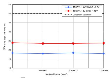
Figure 26. ISL73141SEH average  $\overline{\text{CS}}$  falling edge to BUSY rising edge ( $t_{\text{BUSYLH}}$ ) with AV<sub>CC</sub> = 3.6V, DV<sub>CC</sub> = 3.6V and AV<sub>CC</sub> = 3.0V, DV<sub>CC</sub> = 2.2V, REF = 3.0V,  $t_{\text{SAMP}}$  = 750ksps, A<sub>IN</sub> = -1dBFS, and C<sub>L</sub> = 10pF following irradiation to each level. The error bars (if visible) represent the minimum and maximum measured values. The post – TID irradiation datasheet limit is a maximum of 40ns.
