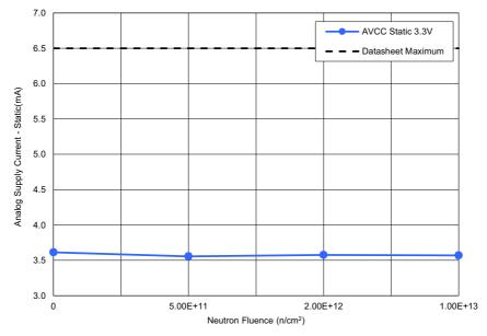
Figure 14. ISL73141SEH average analog supply current – static ( $I_{STATIC}$ ) with AV<sub>CC</sub> = 3.3V, DV<sub>CC</sub> = 2.5V, REF = 3.0V, and  $\overline{CS}$  = DV<sub>CC</sub> following irradiation to each level. The error bars (if visible) represent the minimum and maximum measured values. The post – TID irradiation datasheet limit is a maximum of 6.5mA.
