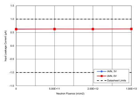
Figure 11. ISL73141SEH average input leakage current ( $I_{AIN}$ ) with AV $_{CC}$  = 3.3V, DV $_{CC}$  = 2.5V, REF = 3.0V,  $f_{SAMP}$  = 750ksps, and A $_{IN}$  = 3.0V and 0V following irradiation to each level. The error bars (if visible) represent the minimum and maximum measured values. The post – TID irradiation datasheet limits are a minimum of -1 $\mu$ A with a maximum of 1 $\mu$ A.
