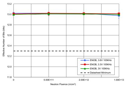
Figure 8. ISL73141SEH average effective number of bits (ENOB) with AV $_{CC}$  = 3.6V, 3.3V and 3.0V, DV $_{CC}$  = 2.5V, REF = 3.0V, F $_{IN}$  = 105kHz, and A $_{IN}$  = -1dBFS following irradiation to each level. The error bars (if visible) represent the minimum and maximum measured values. The post – TID irradiation datasheet limit is a minimum of 12.3bits.
