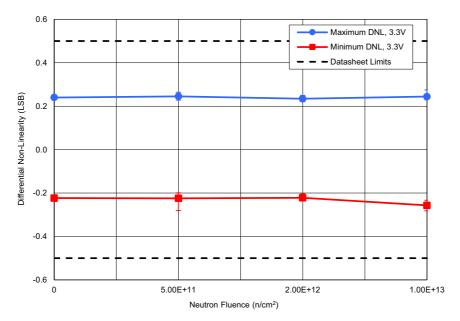
Figure 3. ISL73141SEH average minimum and maximum differential non-linearity (DNL) with  $AV_{CC} = 3.3V$ ,  $DV_{CC} = 2.5V$ , REF = 3.0V,  $f_{SAMP} = 750$ ksps, and  $A_{IN} = full$ -scale sine wave following irradiation to each level. The error bars (if visible) represent the minimum and maximum measured values. The post – TID irradiation datasheet limits are a minimum of -0.5LSB with a maximum of 0.5LSB.
