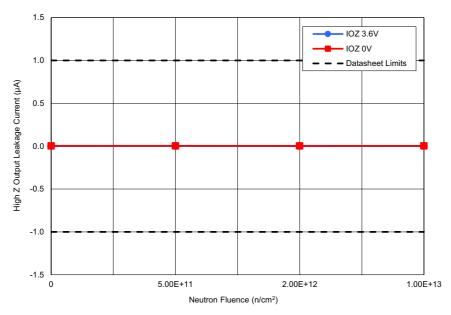
Figure 23. ISL73141SEH average Hi-Z output leakage current ( $I_{OZ}$ ) with AV<sub>CC</sub> = 3.3V, DV<sub>CC</sub> = 3.6V, V<sub>OUT</sub> = 3.6V and 0V, and REF = 3.0V following irradiation to each level. The error bars (if visible) represent the minimum and maximum measured values. The post – TID irradiation datasheet limits are a minimum of -1 $\mu$ A with a maximum of 1 $\mu$ A.
