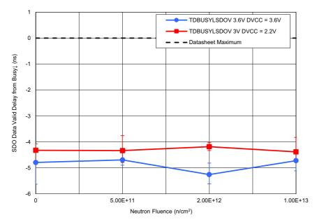
Figure 27. ISL73141SEH average SDO data valid delay from BUSY falling edge ( $t_{DBUSYLSDOV}$ ) with AV<sub>CC</sub> = 3.6V, DV<sub>CC</sub> = 3.6V and AV<sub>CC</sub> = 3.0V, DV<sub>CC</sub> = 2.2V, REF = 3.0V,  $t_{SAMP}$  = 750ksps, A<sub>IN</sub> = -1dBFS, and C<sub>L</sub> = 10pF following irradiation to each level. The error bars (if visible) represent the minimum and maximum measured values. The post – TID irradiation datasheet limit is a maximum of 0ns.
