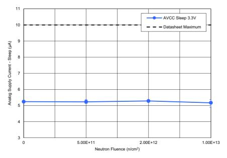
Figu<u>re 15.</u> ISL73141SEH average analog supply current – sleep ( $I_{SLAVCC}$ ) with AV<sub>CC</sub> = 3.3V, DV<sub>CC</sub> = 2.5V, REF = 3.0V, and PD = GND following irradiation to each level. The error bars (if visible) represent the minimum and maximum measured values. The post – TID irradiation datasheet limit is a maximum of 10 $\mu$ A.
