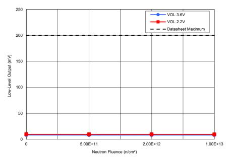
Figure 22. ISL73141SEH average low-level output ( $V_{OL}$ ) with AV<sub>CC</sub> = 3.3V, DV<sub>CC</sub> = 3.6V and 2.2V, REF = 3.0V, and I<sub>O</sub> = 500µA following irradiation to each level. The error bars (if visible) represent the minimum and maximum measured values. The post – TID irradiation datasheet limit is a maximum of 200mV.
