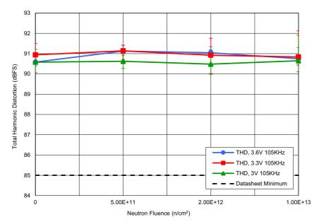
Figure 9. ISL73141SEH average total harmonic distortion (THD) with AV $_{CC}$  = 3.6V, 3.3V and 3.0V, DV $_{CC}$  = 2.5V, REF = 3.0V, F $_{IN}$  = 105kHz (first five harmonics), and A $_{IN}$  = -1dBFS following irradiation to each level. The error bars (if visible) represent the minimum and maximum measured values. The post – TID irradiation datasheet limit is a minimum of 85dB.
