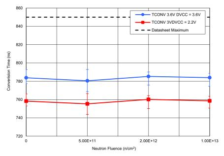
Figure 25. ISL73141SEH average conversion time ( $t_{CONV}$ ) with AV<sub>CC</sub> = 3.6V, DV<sub>CC</sub> = 3.6V and AV<sub>CC</sub> = 3.0V, DV<sub>CC</sub> = 2.2V, REF = 3.0V,  $t_{SAMP}$  = 750ksps, and A<sub>IN</sub> = -1dBFS following irradiation to each level. The error bars (if visible) represent the minimum and maximum measured values. The post – TID irradiation datasheet limit is a maximum of 850ns.
