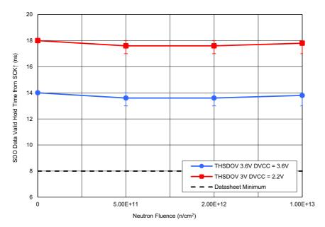
Figure 28. ISL73141SEH average SDO data valid hold time from SCK rising edge ( $t_{HSDOV}$ ) with AV<sub>CC</sub> = 3.6V, DV<sub>CC</sub> = 3.6V and AV<sub>CC</sub> = 3.0V, DV<sub>CC</sub> = 2.2V, REF = 3.0V,  $t_{SAMP}$  = 750ksps, A<sub>IN</sub> = -1dBFS, and C<sub>L</sub> = 10pF following irradiation to each level. The error bars (if visible) represent the minimum and maximum measured values. The post – TID irradiation datasheet limit is a minimum of 8ns.
