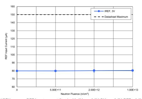
Figure 12. ISL73141SEH average REF input current ( $I_{REF}$ ) with AV<sub>CC</sub> = 3.3V, DV<sub>CC</sub> = 2.5V, REF = 3.0V,  $f_{SAMP}$  = 750ksps, and A<sub>IN</sub> = -1dBFS following irradiation to each level. The error bars (if visible) represent the minimum and maximum measured values. The post – TID irradiation datasheet limit is a maximum of 150 $\mu$ A.
