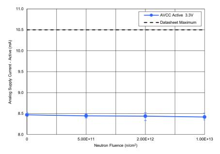
Figure 13. ISL73141SEH average analog supply current – active ( $I_{AVCC}$ ) with  $AV_{CC}$  = 3.3V,  $DV_{CC}$  = 2.5V, REF = 3.0V,  $f_{SAMP}$  = 750ksps, and  $A_{IN}$  = -1dBFS following irradiation to each level. The error bars (if visible) represent the minimum and maximum measured values. The post – TID irradiation datasheet limit is a maximum of 10.5mA.
