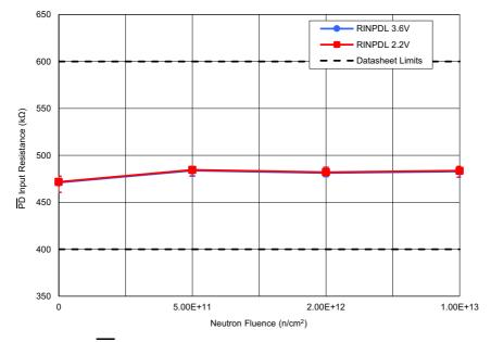
Figure 24. ISL73141SEH average  $\overline{PD}$  input resistance (R<sub>INPDL</sub>) with AV<sub>CC</sub> = 3.3V, DV<sub>CC</sub> = 3.6V and 2.2V, and REF = 3.0V following irradiation to each level. The error bars (if visible) represent the minimum and maximum measured values. The post – TID irradiation datasheet limits are a minimum of 400kΩ with a maximum of 600kΩ.
