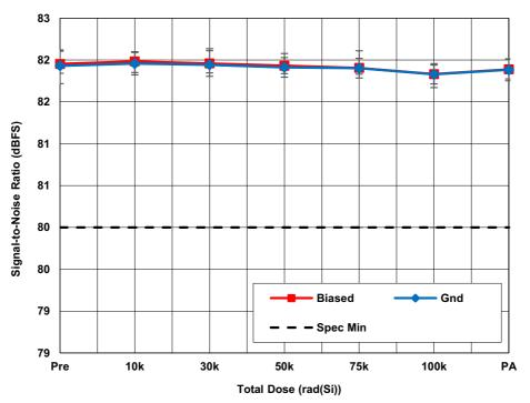
Figure 8. iISL73141SEHMF7 average signal-to-noise ratio (SNR) with  $AV_{CC} = 5.0V$ ,  $DV_{CC} = 2.5V$ , REF = 4.096V,  $f_{SAMP} = 105$ ksps and  $A_{IN} = -1$ dBFS as a function of LDR irradiation and anneal. The error bars represent the minimum and maximum measured values. The datasheet limit is 80dB minimum.
