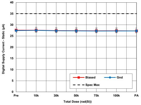
Figure 19. ISL7314<u>1SEHMF7</u> average digital supply current - static ( $I_{STDVCC}$ ) with AV<sub>CC</sub> = 5V, DV<sub>CC</sub> = 2.5V, REF = 4.096V, and CS = DV<sub>CC</sub> as a function of LDR irradiation and anneal. The error bars represent the minimum and maximum measured values. The datasheet limit is 35µA maximum.
