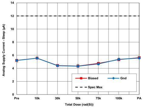
Figure 17. ISL7314<u>1SEHMF7</u> average analog supply current - sleep ( $I_{SLAVCC}$ ) with  $AV_{CC} = 5V$ ,  $DV_{CC} = 2.5V$ , REF = 4.096V, and PD = GND as a function of LDR irradiation and anneal. The error bars represent the minimum and maximum measured values. The datasheet limit is 12µA maximum.
