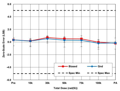
Figure 6. ISL73141SEHMF7 average zero-scale error (VOFF) with  $AV_{CC} = 5V$ ,  $DV_{CC} = 2.5V$ , REF = 4.096V,  $f_{SAMP} = 1Msps$ , and  $A_{IN} = GND$  as a function of LDR irradiation and anneal. The error bars represent the minimum and maximum measured values. The datasheet limits are -5 LSB minimum and 5 LSB maximum.
