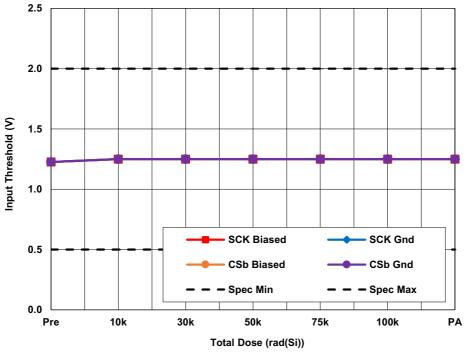
Figure 21. ISL73141SEHMF7 average high-level input ( $V_{IH}$ ) and low level input ( $V_{IL}$ ) with AV<sub>CC</sub> = 5V, DV<sub>CC</sub> = 2.5V, REF = 4.096V as a function of LDR irradiation and anneal. The error bars (if visible) represent the minimum and maximum measured values. The datasheet limit for  $V_{IH}$  is 2.0V minimum and the datasheet limit for  $V_{IL}$  is 0.5V maximum.
