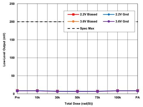
Figure 24. ISL73141SEHMF7 average low-level output ( $V_{OL}$ ) with AV<sub>CC</sub> = 5V, DV<sub>CC</sub> = 2.5V and 3.6V, REF = 4.096V, and I<sub>O</sub> = 500µA as a function of LDR irradiation and anneal. The error bars (if visible) represent the minimum and maximum measured values. The datasheet limit is 200mV maximum.
