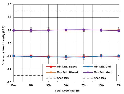
Figure 5. ISL73141SEHMF7 average minimum and maximum differential non-linearity (DNL) with  $AV_{CC} = 5V$ ,  $DV_{CC} = 2.5V$ , REF = 4.096V,  $f_{SAMP} = 1Msps$ , and  $A_{IN} = full$ -scale sine wave as a function of LDR irradiation and anneal. The error bars represent the minimum and maximum measured values. The datasheet limits are -0.5 LSB minimum and 0.5 LSB maximum.
