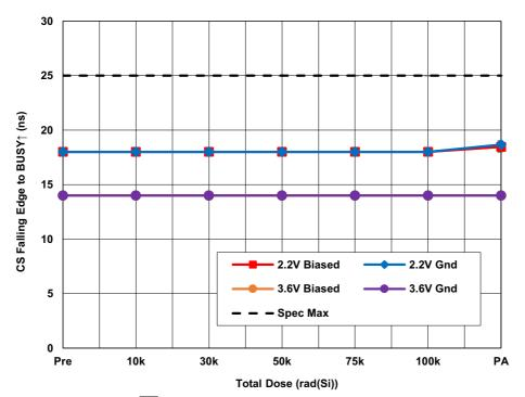
Figure 28. ISL73141SEHMF7 average  $\overline{CS}$  falling edge to BUSY rising edge (t<sub>BUSYLH</sub>) with AV<sub>CC</sub> = 4.5V, DV<sub>CC</sub> = 2.2V and AV<sub>CC</sub> = 5.5V, DV<sub>CC</sub> = 3.6V, REF = 4.096V, f<sub>SAMP</sub> = 1Msps, A<sub>IN</sub> = -1dbFS and C<sub>L</sub> = 10pF as a function of LDR irradiation and anneal. The error bars represent the minimum and maximum measured values. The datasheet limit is 25ns maximum.
