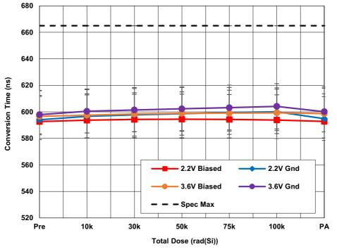
Figure 27. ISL73141SEHMF7 average conversion time ( $t_{CONV}$ ) with AV<sub>CC</sub> = 4.5V, DV<sub>CC</sub> = 2.2V and AV<sub>CC</sub> = 5.5V, DV<sub>CC</sub> = 3.6V, REF = 4.096V,  $f_{SAMP}$  = 1Msps, and  $A_{IN}$  = -1dbFS as a function of LDR irradiation and anneal. The error bars represent the minimum and maximum measured values. The datasheet limit is 665ns maximum.
