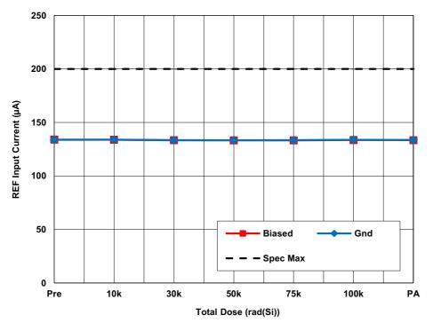
Figure 14. .ISL73141SEHMF7 average REF input current ( $I_{REF}$ ) with AV<sub>CC</sub> = 5V, DV<sub>CC</sub> = 2.5V, REF = 4.096V as a function of LDR irradiation and anneal. The error bars represent the minimum and maximum measured values. The datasheet limit is 200µA maximum.
