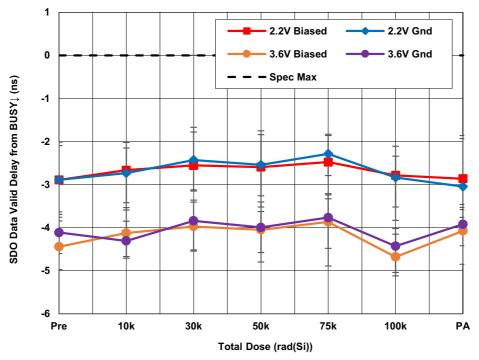
Figure 29. ISL73141SEHMF7 average SDO data valid delay from BUSY falling edge ( $t_{DBUSYLSDOV}$ ) with AV<sub>CC</sub> = 4.5V, DV<sub>CC</sub> = 2.2V and AV<sub>CC</sub> = 5.5V, DV<sub>CC</sub> = 3.6V, REF = 4.096V,  $f_{SAMP}$  = 1Msps, A<sub>IN</sub> = -1dbFS and C<sub>L</sub> = 10pF as a function of LDR irradiation and anneal. The error bars represent the minimum and maximum measured values. The datasheet limit is 0ns maximum.
