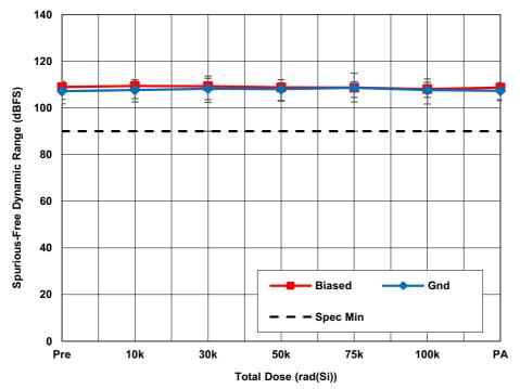
Figure 12. ISL73141SEHMF7 average spurious-free dynamic range (SFDR) with  $AV_{CC} = 5V$ ,  $DV_{CC} = 2.5V$ , REF = 4.096V,  $f_{SAMP} = 105$ ksps (first five harmonics), and  $A_{IN} = -1$ dBFS as a function of LDR irradiation and anneal. The error bars represent the minimum and maximum measured values. The datasheet limit is 90 dB minimum.
