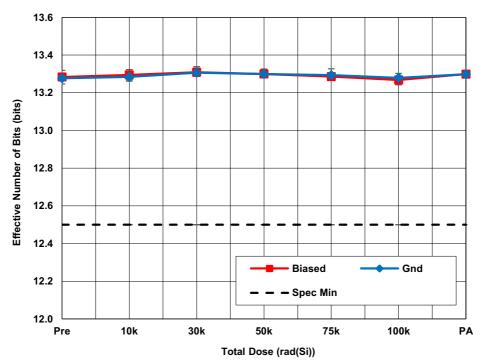
Figure 10. ISL73141SEHMF7 average effective number of bits (ENOB) with  $AV_{CC} = 5.0V$ ,  $DV_{CC} = 2.5V$ , REF = 4.096V,  $f_{SAMP} = 105$ ksps, and  $A_{IN} = -1$ dBFS as a function of LDR irradiation and anneal. The error bars represent the minimum and maximum measured values. The datasheet limit is 12.5 bits minimum.
