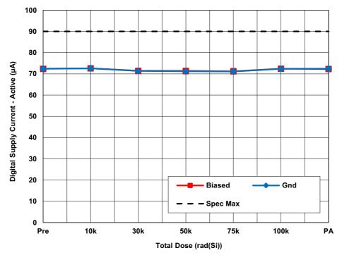
Figure 18. ISL73141SEHMF7 average digital supply current - active ( $I_{DVCC}$ ) with AV<sub>CC</sub> = 5V, DV<sub>CC</sub> = 2.5V, REF = 4.096V,  $f_{SCK}$  = 50MHz, and C<sub>L</sub> = 10pF as a function of LDR irradiation and anneal. The error bars represent the minimum and maximum measured values. The datasheet limit is 90µA maximum.
