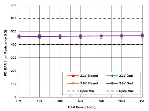
Figure 26. ISL73141SEHMF7 average  $\overline{PD}$  input resistance (R<sub>INPDL</sub>) with AV<sub>CC</sub> = 5V, DV<sub>CC</sub> = 2.2V and 3.6V and REF = 4.096V as a function of LDR irradiation and anneal. The error bars represent the minimum and maximum measured values. The datasheet limits are 400k $\Omega$  minimum and 600k $\Omega$  maximum.
