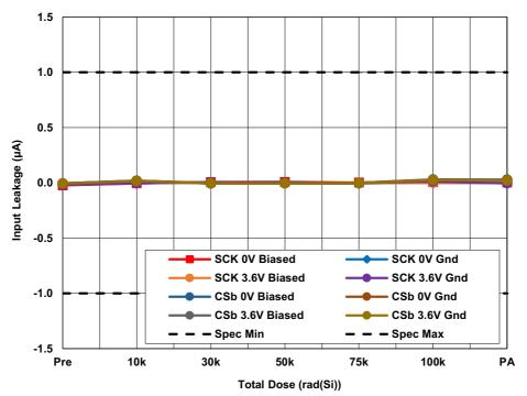
Figure 22. ISL73141SEHMF7 average input leakage current ( $I_{IN}$ ) on SCK and  $\overline{CS}$  with AV<sub>CC</sub> = 5V, DV<sub>CC</sub> = 2.5V, REF = 4.096V and V<sub>IN</sub> = 0V and 5V as a function of LDR irradiation and anneal. The error bars (if visible) represent the minimum and maximum measured values. The datasheet limits are -1µA minimum and 1µA maximum.
