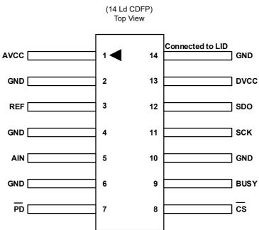
Note: The ESD triangular mark is indicative of Pin #1. It is a part of the device marking and is placed on the lid in the quadrant where Pin #1 is located.
