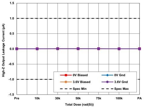
Figure 25. ISL73141SEHMF7 average output leakage current ( $I_{OZ}$ ) with AV<sub>CC</sub> = 5V, DV<sub>CC</sub> = 3.6V, REF = 4.096V, as a function of LDR irradiation and anneal. The error bars (if visible) represent the minimum and maximum measured values. The datasheet limits are -1µA minimum and 1µA maximum.
