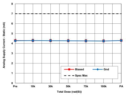
Figure 16. ISL7314<u>1SEHMF7</u> average analog supply current - static ( $I_{STATIC}$ ) with AV<sub>CC</sub> = 5V, DV<sub>CC</sub> = 2.5V, REF = 4.096V, and CS = DVCC as a function of LDR irradiation and anneal. The error bars represent the minimum and maximum measured values. The datasheet limit is 7mA maximum.
