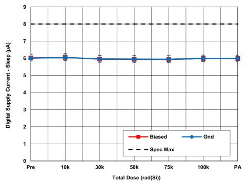
Figure 20. ISL73141SEHMF7 average digital supply current - sleep ( $I_{SLDVCC}$ ) with AV<sub>CC</sub> = 5V, DV<sub>CC</sub> = 2.5V, REF = 4.096V, PD = GND as a function of LDR irradiation and anneal. The error bars represent the minimum and maximum measured values. The datasheet limit is 8µA maximum.
