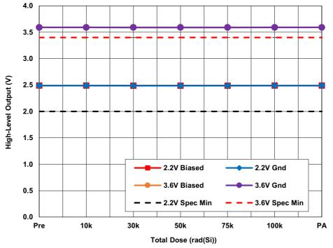
Figure 23. ISL73141SEHMF7 average high-level output (V<sub>OH</sub>) with AV<sub>CC</sub> = 5V, DV<sub>CC</sub> = 2.2V and 3.6V, REF = 4.096V and  $I_O = -500\mu$ A as a function of LDR irradiation and anneal. The error bars (if visible) represent the minimum and maximum measured values. The datasheet limits are 2.0V minimum for DV<sub>CC</sub> = 2.2V and 3.4V minimum for DV<sub>CC</sub> = 3.6V.
