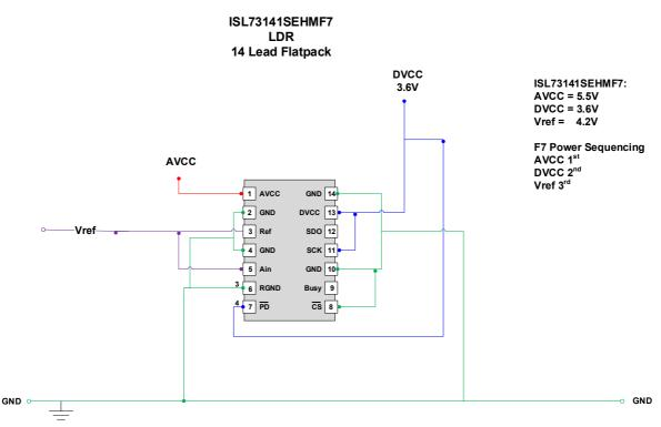
Figure 3. ISL73141SEHMF7 TID Bias Schematic
