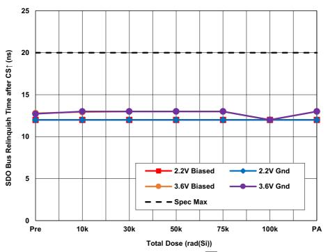
Figure 32. ISL73141SEHMF7 average SDO bus relinquish time after  $\overline{CS}$  rising edge ( $t_{DCSHSDOZ}$ ) with AV<sub>CC</sub> = 4.5V, DV<sub>CC</sub> = 2.2V and AV<sub>CC</sub> = 5.5V, DV<sub>CC</sub> = 3.6V, REF = 4.096V,  $f_{SAMP}$  = 1Msps,  $A_{IN}$  = -1dbFS, and  $C_L$  = 10pF as a function of LDR irradiation and anneal. The error bars represent the minimum and maximum measured values. The datasheet limit is 20ns maximum.
