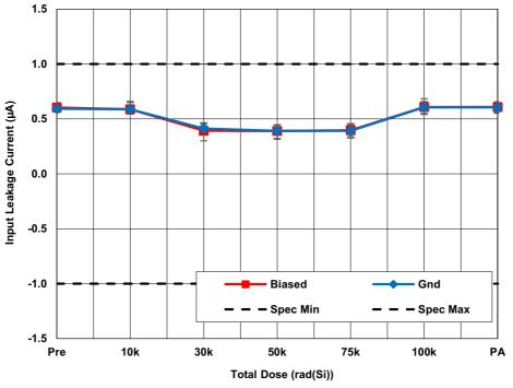
Figure 13. ISL73141SEHMF7 average input leakage current (IA<sub>IN</sub>) with AV<sub>CC</sub> = 5V, DV<sub>CC</sub> = 2.5V, REF = 4.096V as a function of LDR irradiation and anneal. The error bars represent the minimum and maximum measured values. The datasheets limits are -1 $\mu$ A minimum and 1 $\mu$ A maximum.
