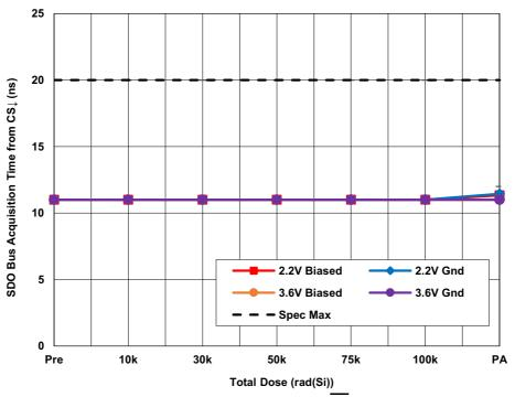
Figure 31. ISL73141SEHMF7 average SDO bus acquisition time from  $\overline{CS}$  falling edge ( $t_{DCSLSDOL}$ ) with AV<sub>CC</sub> = 4.5V, DV<sub>CC</sub> = 2.2V and AV<sub>CC</sub> = 5.5V, DV<sub>CC</sub> = 3.6V, REF = 4.096V,  $f_{SAMP}$  = 1Msps,  $A_{IN}$  = -1dbFS and  $C_L$  = 10pF as a function of LDR irradiation and anneal. The error bars represent the minimum and maximum measured values. The datasheet limit is 20ns maximum.
