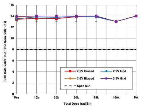
Figure 30. ISL73141SEHMF7 average SDO data valid hold time from SCK rising edge ( $t_{HSDOV}$ ) with AV<sub>CC</sub> = 4.5V, DV<sub>CC</sub> = 2.2V and AV<sub>CC</sub> = 5.5V, DV<sub>CC</sub> = 3.6V, REF = 4.096V,  $f_{SAMP}$  = 1Msps,  $A_{IN}$  = -1dbFS, and  $C_L$  = 10pF as a function of LDR irradiation and anneal. The error bars represent the minimum and maximum measured values. The datasheet limit is 8ns minimum.
