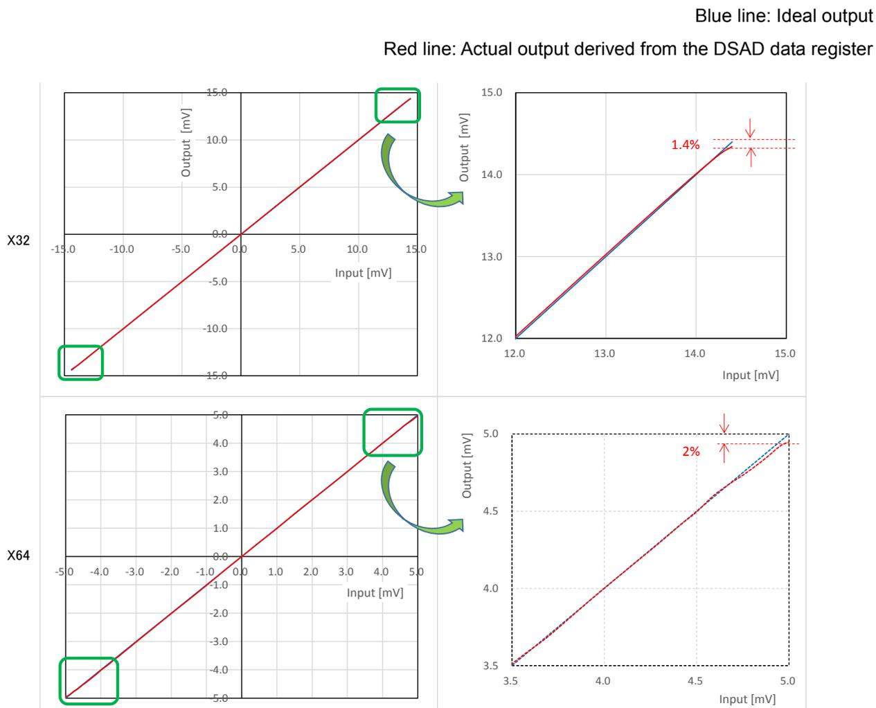
Figure 1. An example of the output from the channel whose accuracy is not good.
