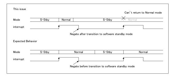
Peripheral interrupts affected are those that use LOCO and sub-oscillator as clock sources:
