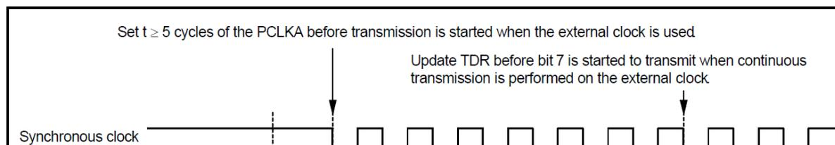
Figure 34.77 Constraints on use of external clock in clock synchronous transmission
