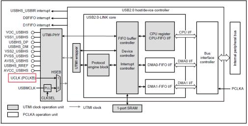
Figure 33.1 USBHS block diagram
