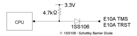
The type and the inserting direction of the diode
