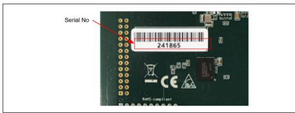
Figure 1: Serial No. location (CPU board solder side)
