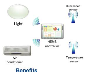
Sensor devices are used to control various home appliances so that users can live comfortably.
