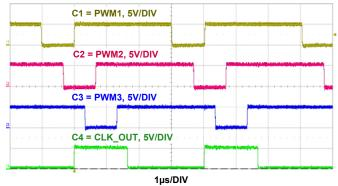
FIGURE 9. WAVEFORMS WITH PWM\_INV = V<sub>CC</sub>
