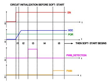
FIGURE 14. CIRCUIT INITIALIZATION BEFORE SOFT-START
