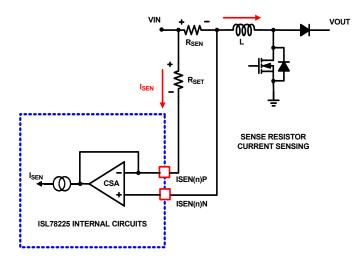
FIGURE 20. SENSE RESISTOR CURRENT SENSING
