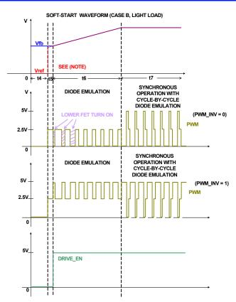
NOTE: t<sub>4</sub>, t<sub>5</sub> PERIOD ARE FROM <u>FIGURE 5</u> FIGURE 16. SOFT-START WAVEFORM (CASE B, LIGHT LOAD)
