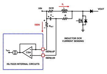
FIGURE 21. INDUCTOR DCR CURRENT SENSING
