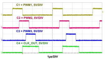
FIGURE 8. WAVEFORMS WITH PWM\_INV = GND
