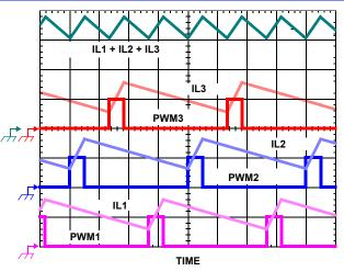
FIGURE 13. PWM AND INDUCTOR-CURRENT WAVEFORMS FOR 3-PHASE CONVERTER
