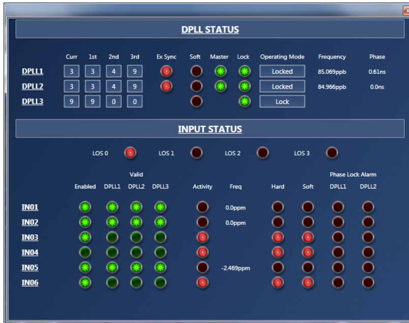
Figure 2. DPLL Status for the Typical Configuration
