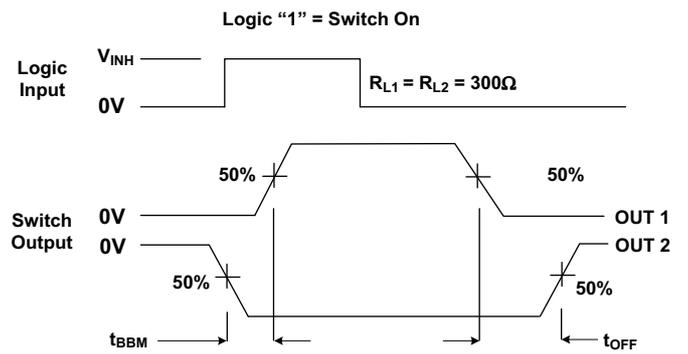
Figure 6. Break-Before-Make Test Circuit Waveforms
