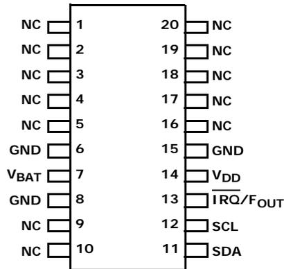
FIGURE 1. ISL12022M PINOUT
