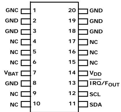
FIGURE 2. ISL12022MA PINOUT
