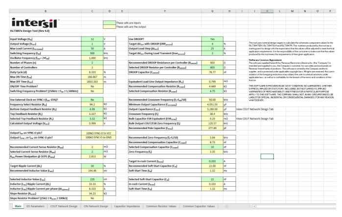
Figure 1. Automatic Design Results for a 2-Phase ISL73847 Application Design
