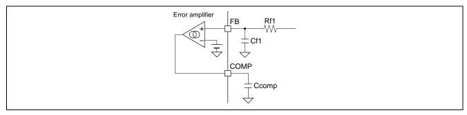
Figure 7.3 External Circuit for FB & COMP Terminals
