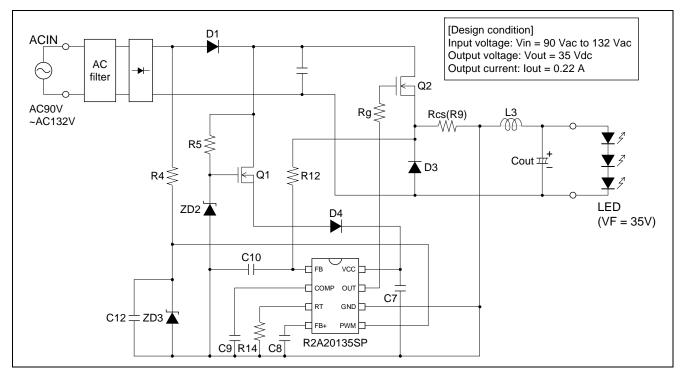
Figure 7.1 R2A20135EVB-ND1 Schematic
