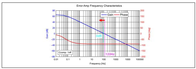
Figure 7.4 R2A20135EVB-ND1 Frequency Characteristics
