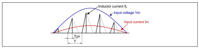
Figure 7.2 Input Current & Inductor Current
