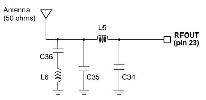
Table 1 - 2 Examples of the Constants for the Transmitted Output Matching Circuit
