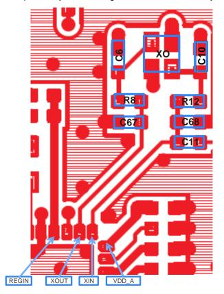
Figure 2 - 2 Example of Layout of Wiring Patterns around the Crystal Resonator
