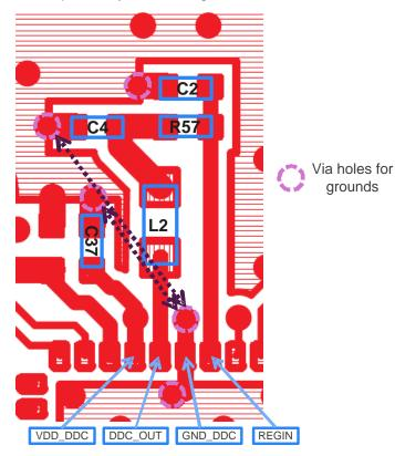
Figure 2 - 3 Example of Layout of Wiring Patterns for the DC-DC Converter Circuit
