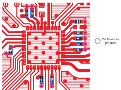
Figure 2 - 4 Example of Layout of Wiring Patterns around Power Supplies
