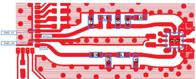
Figure 2 - 1 Examples of Layout of the Patterns around the RF Signal Lines
