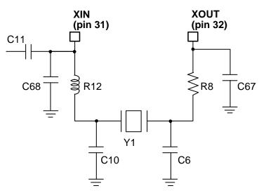
Figure 1 - 5 Example of the Configuration of the Crystal Oscillator
