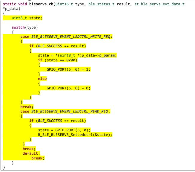
(6) In e<sup>2</sup> studio project explorer, open the file qe\_gen\ble\ profile\_cmn\r\_ble\_servc\_if.c including the R\_BLE\_SERVS\_GetChar function and add the yellow highlighted code, resulting in the code shown below:
