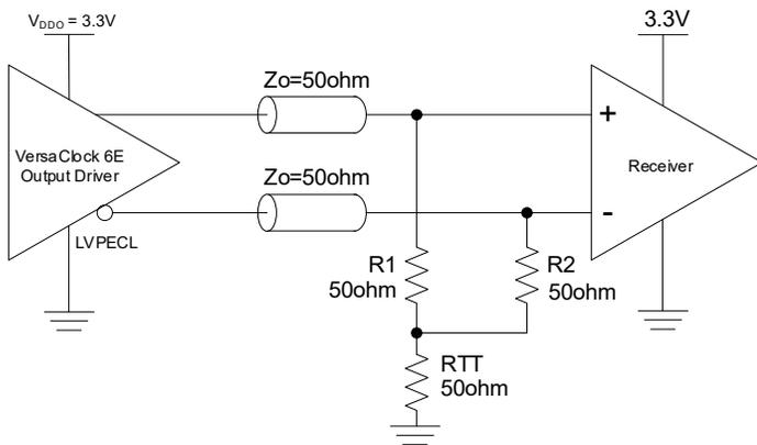
**Figure 15. 2.5V LVPECL Output Termination (1)**
