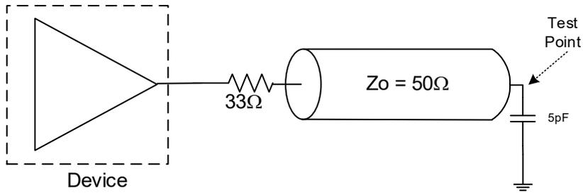
**Figure 3. HCSL/LPHCSL Test Load**
