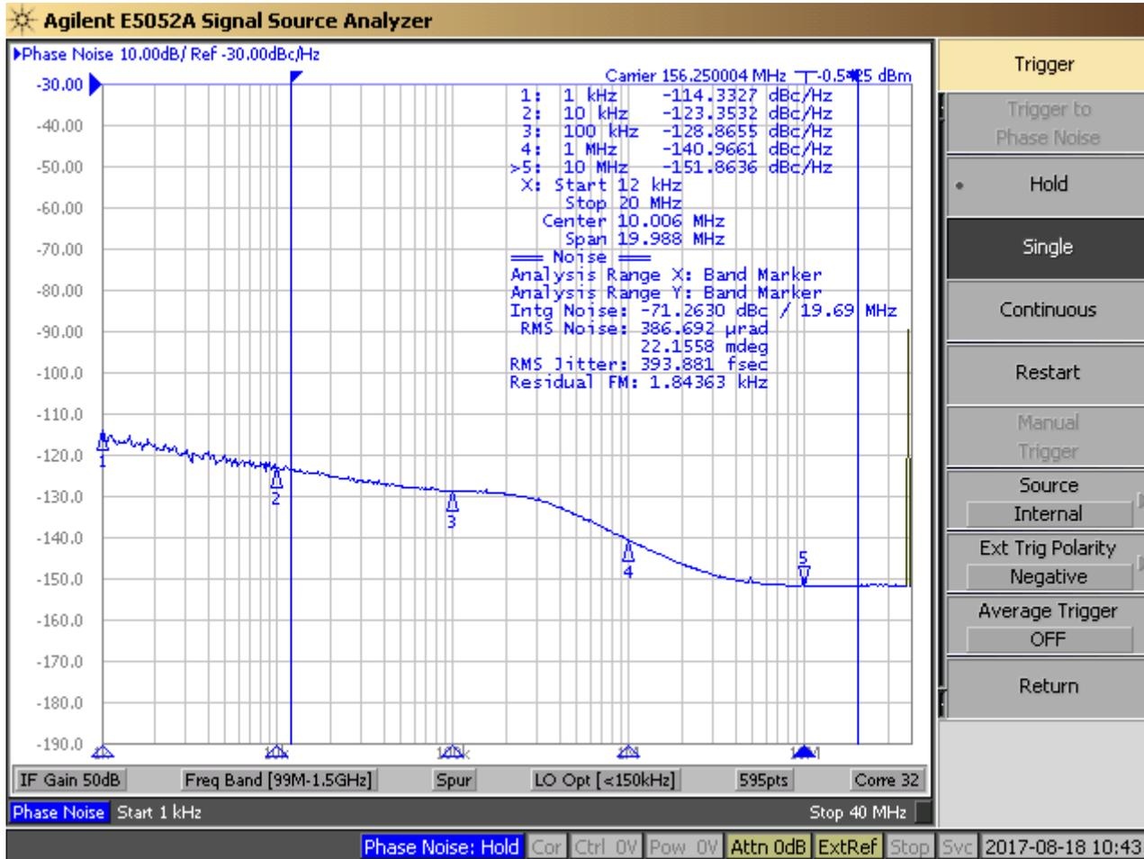
Note: Measured with OUT2=156.25MHz on, 39.625MHz input.
