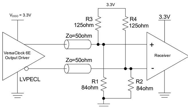
**Figure 16. 2.5V LVPECL Output Termination (2)**
