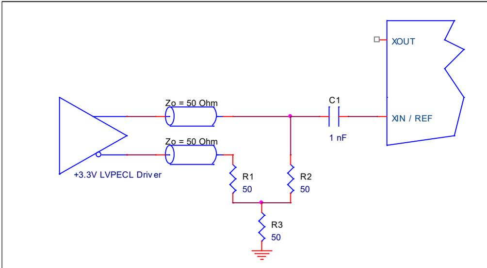
Table 23 shows resistor values that ensure the maximum drive level for the CLKIN port is not exceeded for all combinations of 5% tolerance on the driver  $V_{DD}$ ,  $V_{DD00}$ , and 5% resistor tolerances. The resistor values can be adjusted to reduce the loading for a slower and weaker LVCMOS driver by increasing the impedance of the R1–R2 divider. To better assist with this assessment, the total load ( $R_o+R_s+R_1+R_2$ ) on the driver is included in the table.
