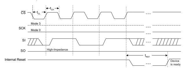
Figure 22. JEDEC Standard Hardware Reset
