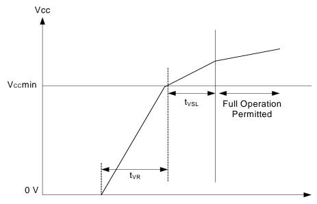
Figure 31. AC Timing During Device Power Up
