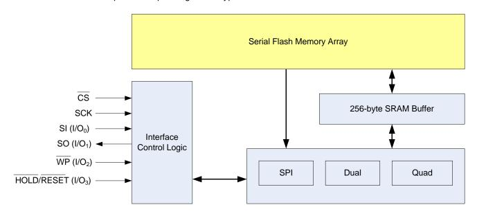
Figure 2. Block Diagram
