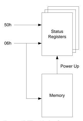
Figure 23. AT25FF041A Register Structure
