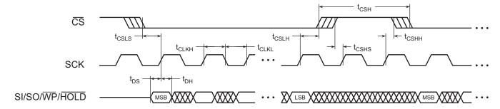
Figure 33. Serial Input Timing
