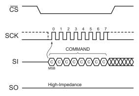
Figure 3. SPI Transfer — Command Only
