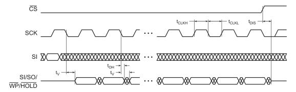
Figure 34. Serial Output Timing
