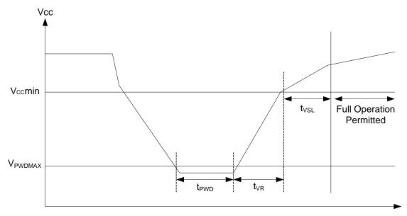
Figure 32. AC Power-up Timing After a Brown-Out
