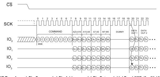
Figure 15. XiP Transfer — 1-Pin Command, 4-Pin Address, and 4-Pin Data — Initial Read (M[5:4] = 2'b10)
