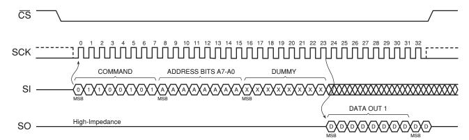
Figure 24. Status Register Read Operation Showing Eight-bit Address Field
