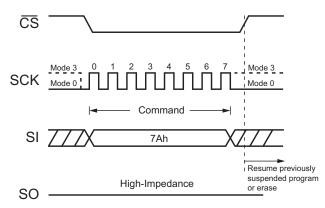
Figure 40. Erase / Program Resume command (SPI Mode)
