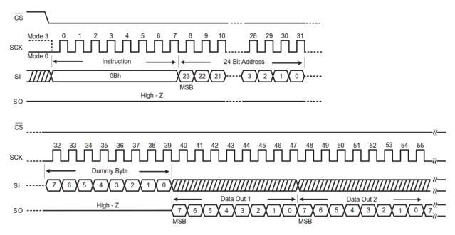
Figure 16. Fast Read Command (SPI Mode)
