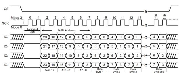
Figure 30. Quad Page Program Command (QPI mode)
