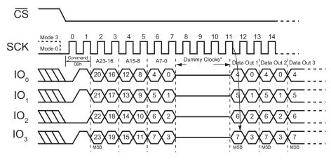
\* = "Set Read Parameters" command (C0h) can set the number of dummy clocks
