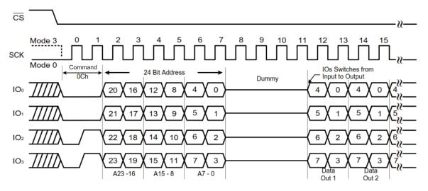
Figure 58. Burst Read with Wrap command (QPI Mode, 80MHz)
