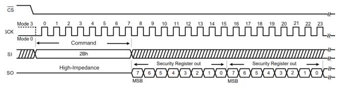
Figure 66. Read Security Register Command (SPI Mode)
