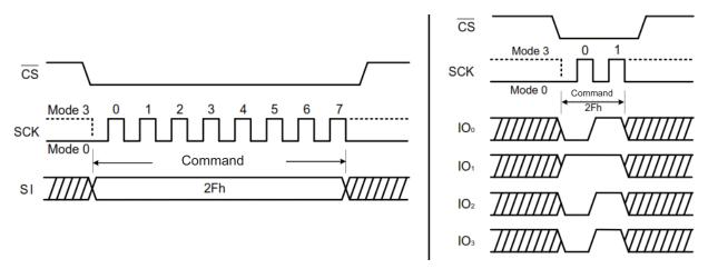
Figure 68. Write Security Register Command for SPI Mode (left) and QPI Mode (right)
