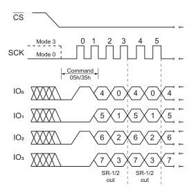
Figure 10. Read Status Register Command (QPI Mode)
