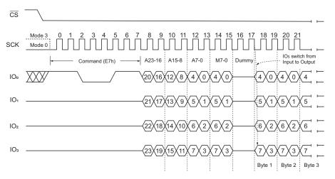
Figure 55. Word Read Quad I/O Command (Initial command or previous set M7-0 ≠ Axh, SPI Mode)
