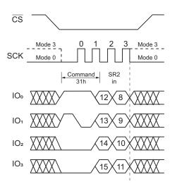
Figure 14. Write Status Register-2 Command (QPI Mode)
