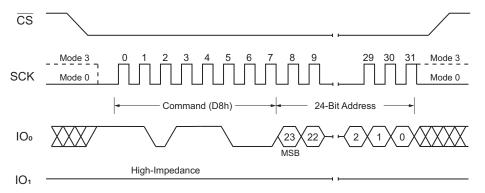
Figure 35. 64 kbytes Block Erase Command (SPI Mode)
