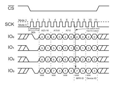
Figure 48. Read Manufacturer/ Device ID Command (QPI Mode)
