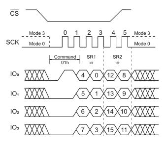
Figure 12. Write Status Register Command (QPI Mode)
