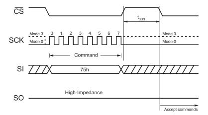
Figure 38. Erase Suspend command (SPI Mode)
