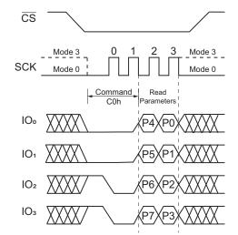
Figure 60. Set Read Parameters command (QPI Mode)
