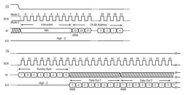
Figure 16. Fast Read Command (SPI Mode)
