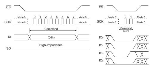
Figure 8. Write Disable Command for SPI Mode (left) and QPI Mode (right)
