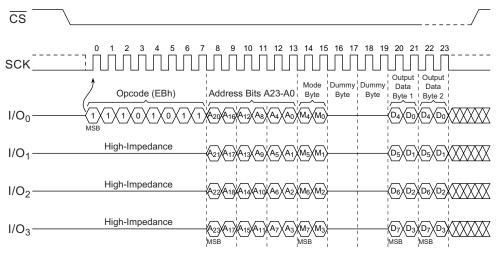
Figure 23. Fast Read Quad I/O Command (Initial command or previous M7-0 ≠ Axh, SPI mode)
