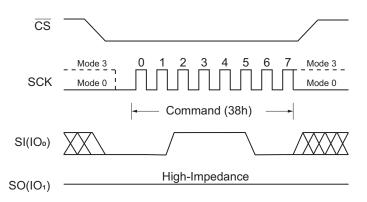
Figure 53. Enable QPI Command (SPI Mode only)
