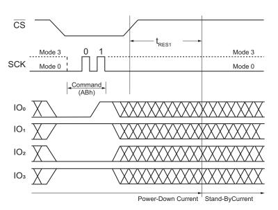
Figure 45. Release Power-Down Command (QPI Mode)
