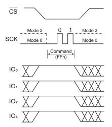
Figure 54. Disable QPI Command for QPI Mode
