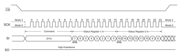
Figure 11. Write Status Register Command (SPI Mode)
