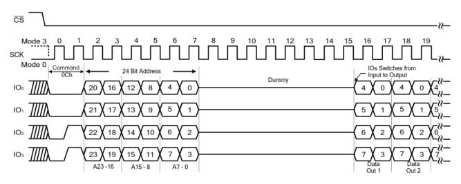
Figure 59. Burst Read with Wrap command (QPI Mode, 133 MHz)
