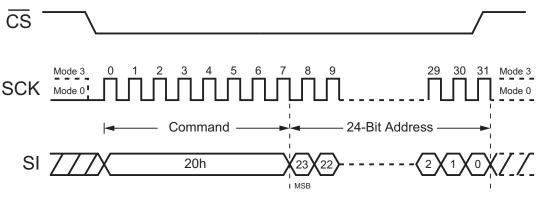
Figure 31. Block Erase Command (SPI Mode)
