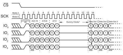
\* = "Set Read Parameters" command (C0h) can set the number of dummy clocks
