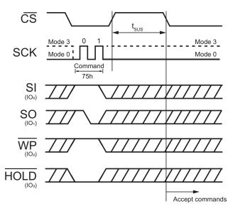
Figure 39. Erase Suspend command (QPI Mode)
