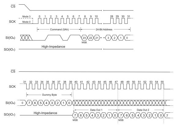
Figure 63. Read SFDP Register Command
