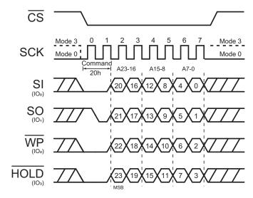
Figure 32. Block Erase Command (QPI Mode)
