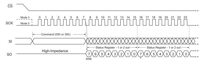
Figure 9. Read Status Register Command (SPI Mode)
