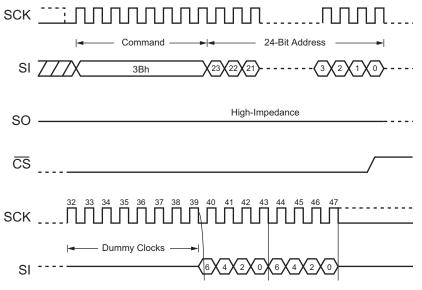
Figure 19. Fast Read Dual Output Command (SPI Mode)
