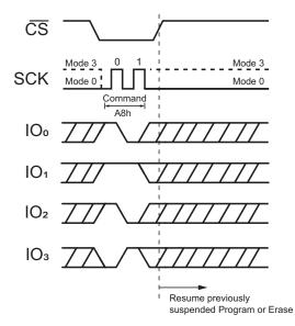
Figure 41. Erase / Program Resume command (QPI Mode)
