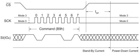
Figure 42. Deep Power-Down Command (SPI Mode)
