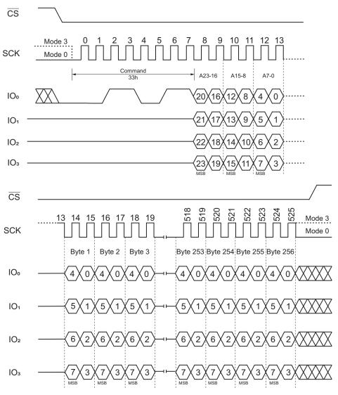
Figure 29. Quad Page Program Command (SPI mode)
