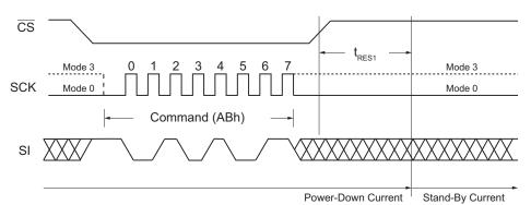
Figure 44. Release Power-Down Command (SPI Mode)
