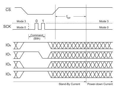
Figure 43. Deep Power-Down Command (QPI Mode)
