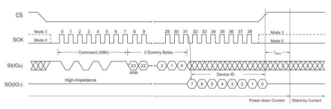
Figure 46. Release Power-Down / Device ID Command (SPI Mode)
