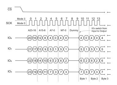
Figure 56. Word Read Quad I/O Command (Previous command set M7-0 = Axh, SPI Mode)
