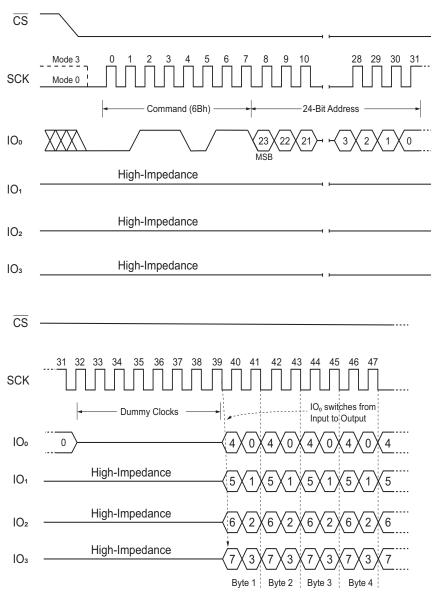
Figure 20. Fast Read Quad Output Command (SPI Mode)
