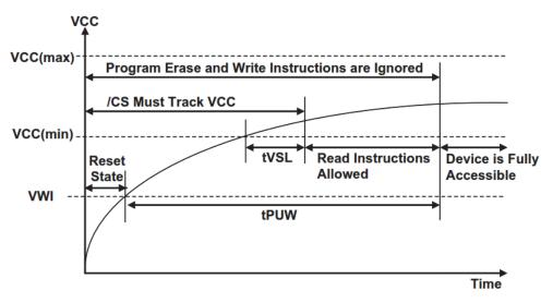
Figure 69. Power-Up Timing and Voltage Levels
