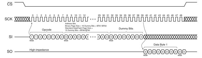
Figure 42. Buffer Read Timing (Opcode D4h or D6h)
