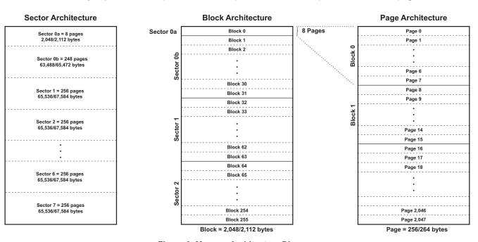
Figure 3. Memory Architecture Diagram
