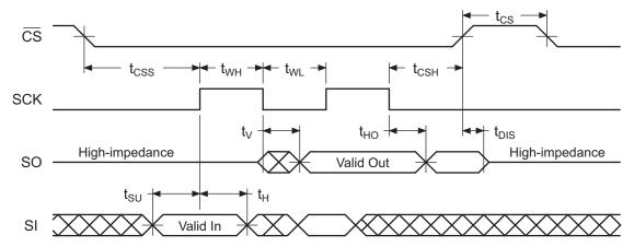
Figure 27. Waveform 1 = SPI Mode 0 Compatible
