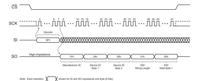
Figure 48. Manufacturer and Device Read Timing (Opcode 9Fh)
