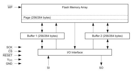
Figure 2. Block Diagram
