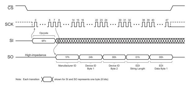
Figure 21. Read Manufacturer and Device ID Timing
