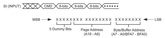
Figure 25. Command Sequence for Read/Write Operations for Page Size 256 bytes (Except Status Register Read, Manufacturer and Device ID Read)
