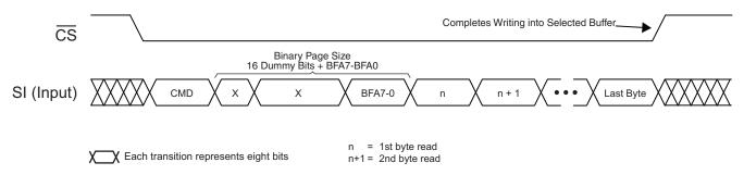
Figure 32. Buffer Write
