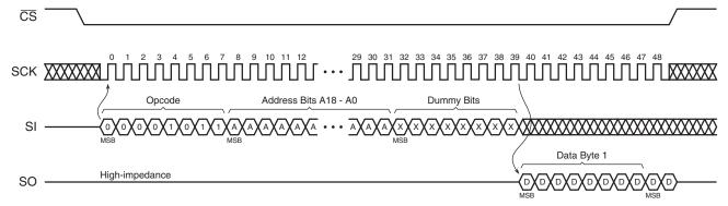
Figure 39. Continuous Array Read Timing (Opcode 0Bh)
