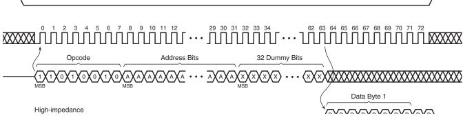
Figure 41. Main Memory Page Read Timing (Opcode D2h)
