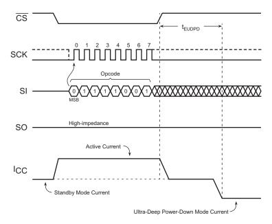
Figure 18. Ultra-Deep Power-Down Timing
