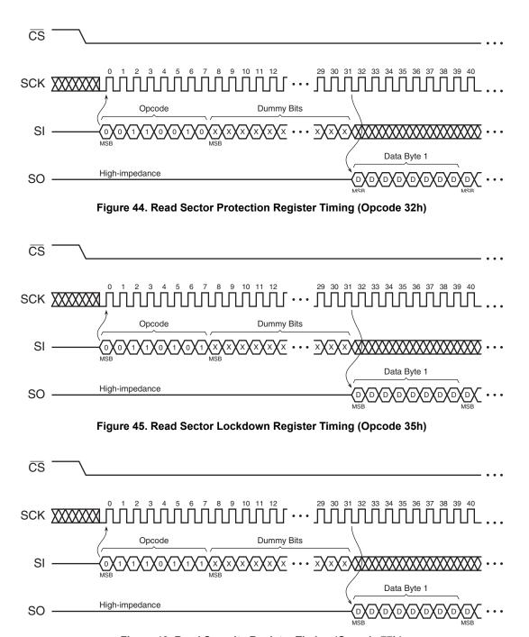
Figure 46. Read Security Register Timing (Opcode 77h)
