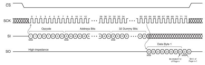
Figure 38. Continuous Array Read Timing (Legacy Opcode E8h)
