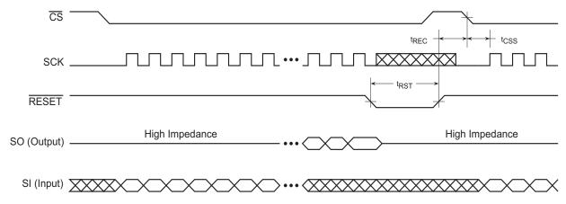
Figure 49. Reset Timing
