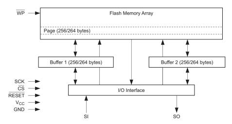
Figure 31. Block Diagram
