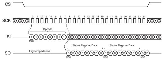
Figure 47. Status Register Read Timing (Opcode D7h)
