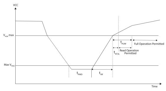
Figure 23. Power-Up Timing
