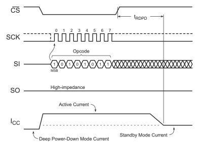
Figure 17. Resume from Deep Power-Down Timing
