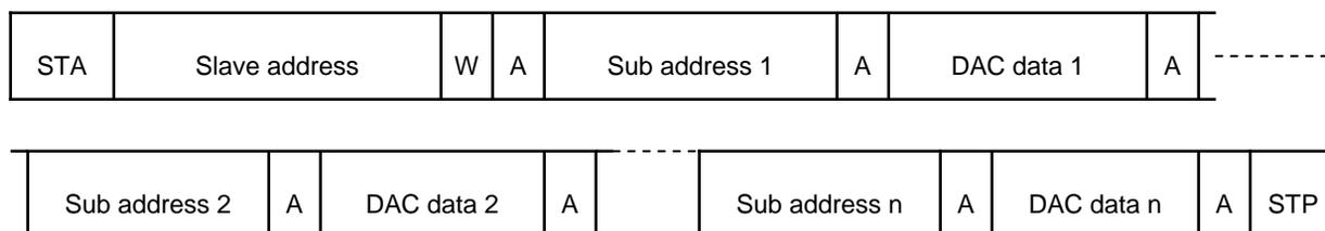
After the Start condition, the transmitting IC accesses the slave IC by Slave address, and transmits the data to each channel by two bites (Sub address and DAC data).
