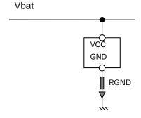
External diode is recommended in order to prevent reverse current toward control logic part at reverse battery condition.
