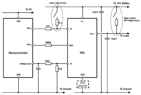
RIN, RSEN, RAN values are in range of 2k to 50kohm depending microcontroller while R\_L value is typically 4kohm. If necessary to raise HBM tolerated dose, adding resister between OUT terminal and Ground is effective. Resister's value is typically 100kohm
