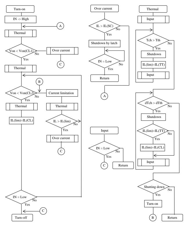
IL(lim) initial value is power MOSFET saturation current.
