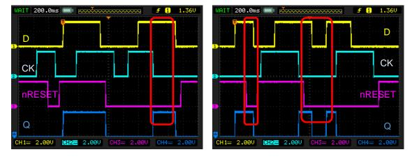
The scope shots shown above show the incorrect nRESET function operation marked with red rectangles. From these waveforms can be seen that the reset function operates only when the CK signal is HIGH, in all other cases it is inoperational.
