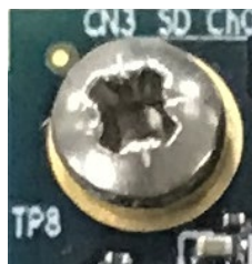
Specially shaped screw threads
