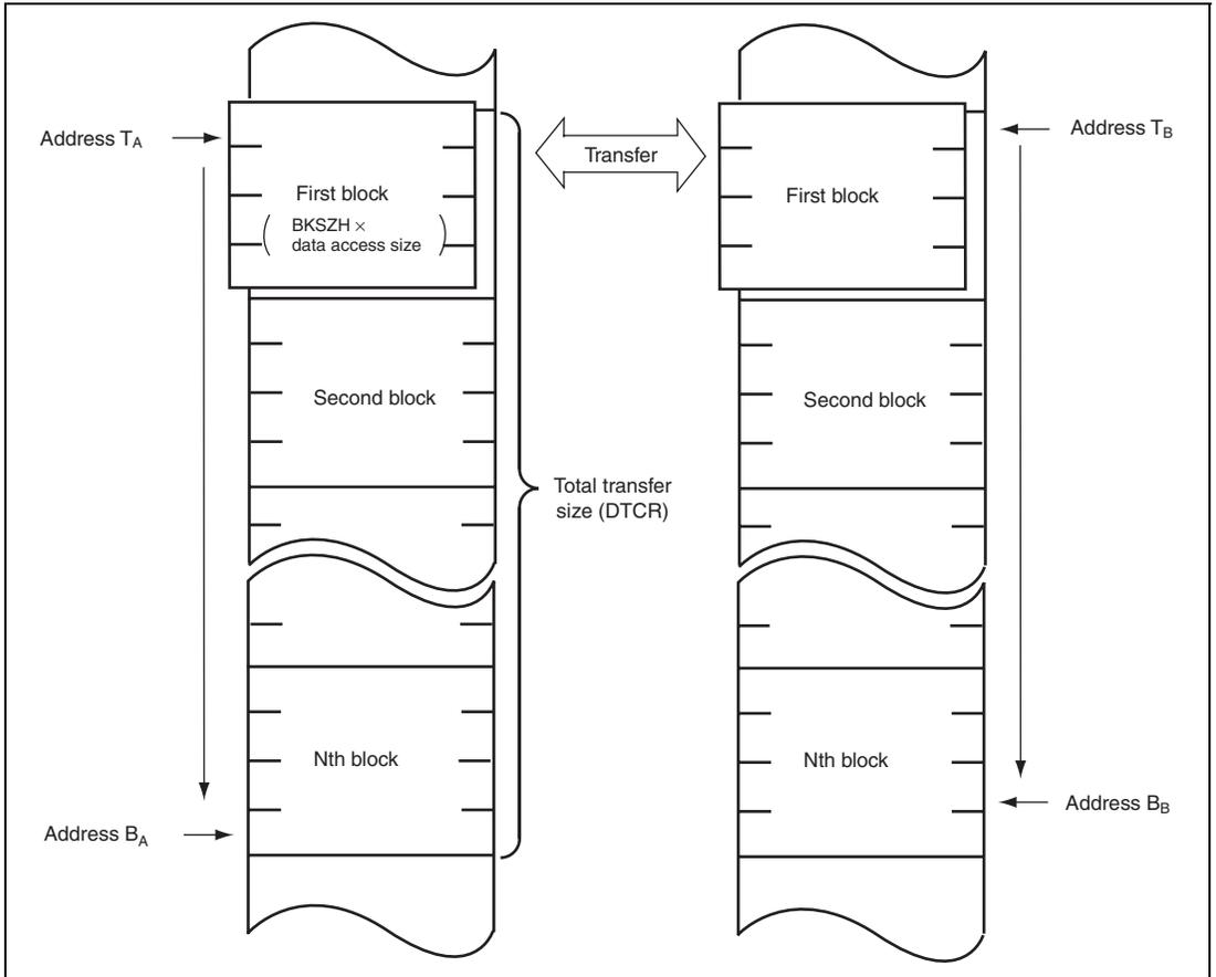
**Figure 10.12 Operation in Dual Address Mode in Block Transfer Mode
