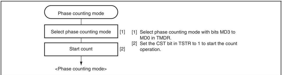
**Figure 13.25 Example of Phase Counting Mode Setting Procedure**
