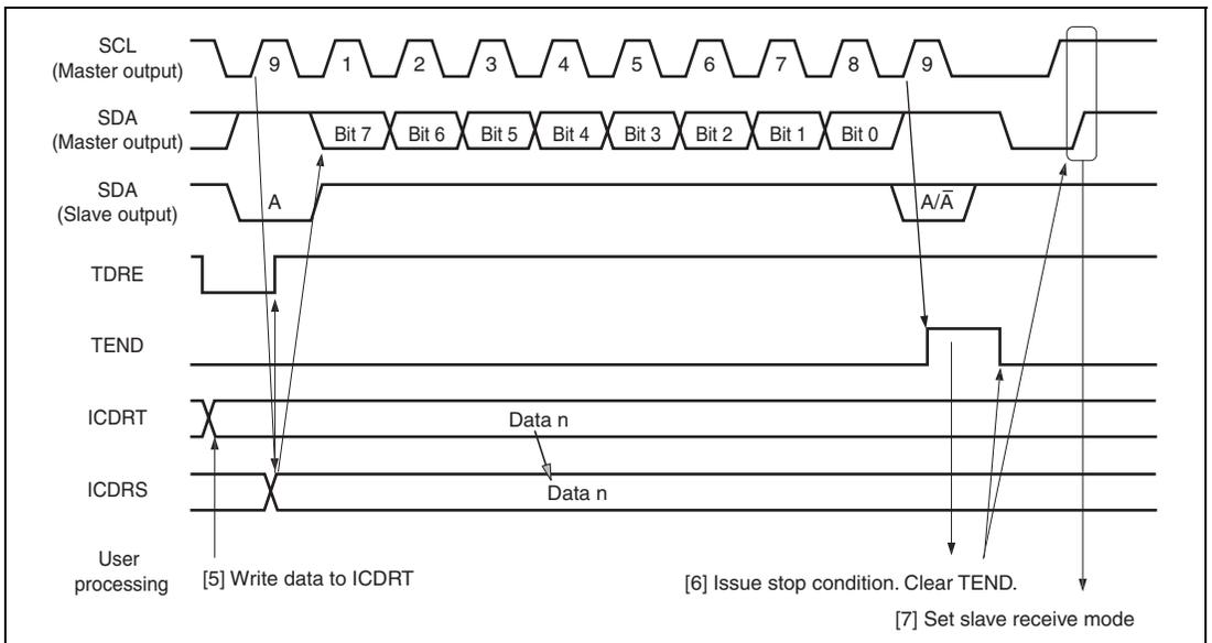
**Figure 18.6 Master Transmit Mode Operation Timing 2**
