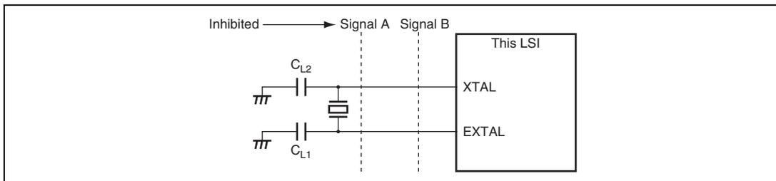
**Figure 24.7 Note on Board Design for Oscillation Circuit**
