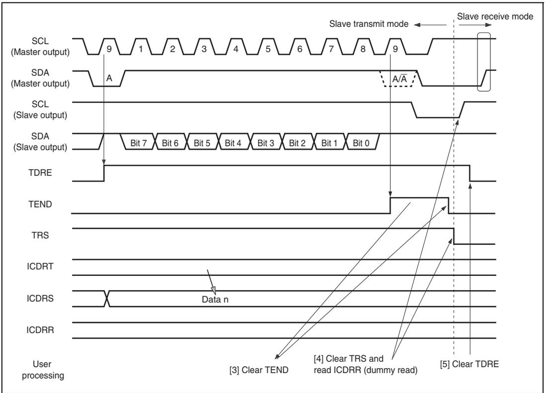
**Figure 18.10 Slave Transmit Mode Operation Timing 2**
