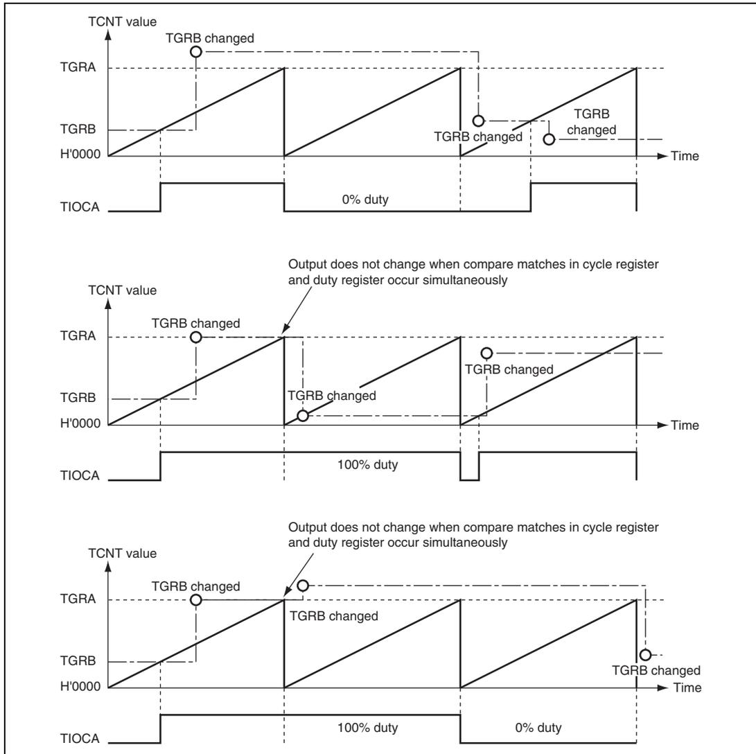
**Figure 13.24 Example of PWM Mode Operation (3)**
