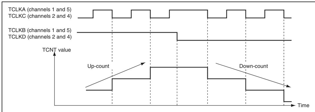
**Figure 13.27 Example of Phase Counting Mode 2 Operation**
