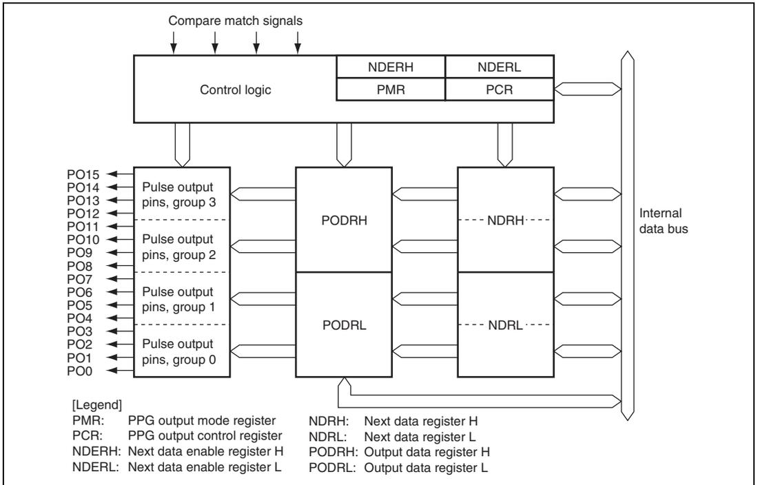
**Figure 14.1 Block Diagram of PPG (Unit 0)**
