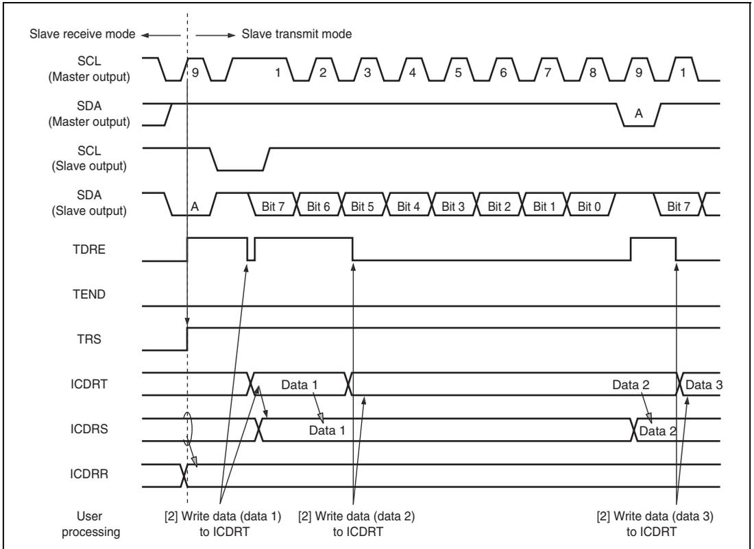
**Figure 18.9 Slave Transmit Mode Operation Timing 1**
