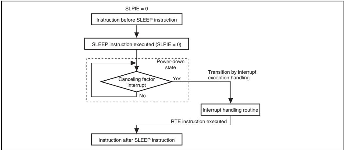
**Figure 25.10 When Canceling Factor Interrupt is Generated after SLEEP Instruction Execution**
