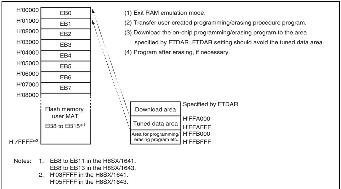
**Figure 22.19 Programming Tuned Data (H8SX/1645)**
