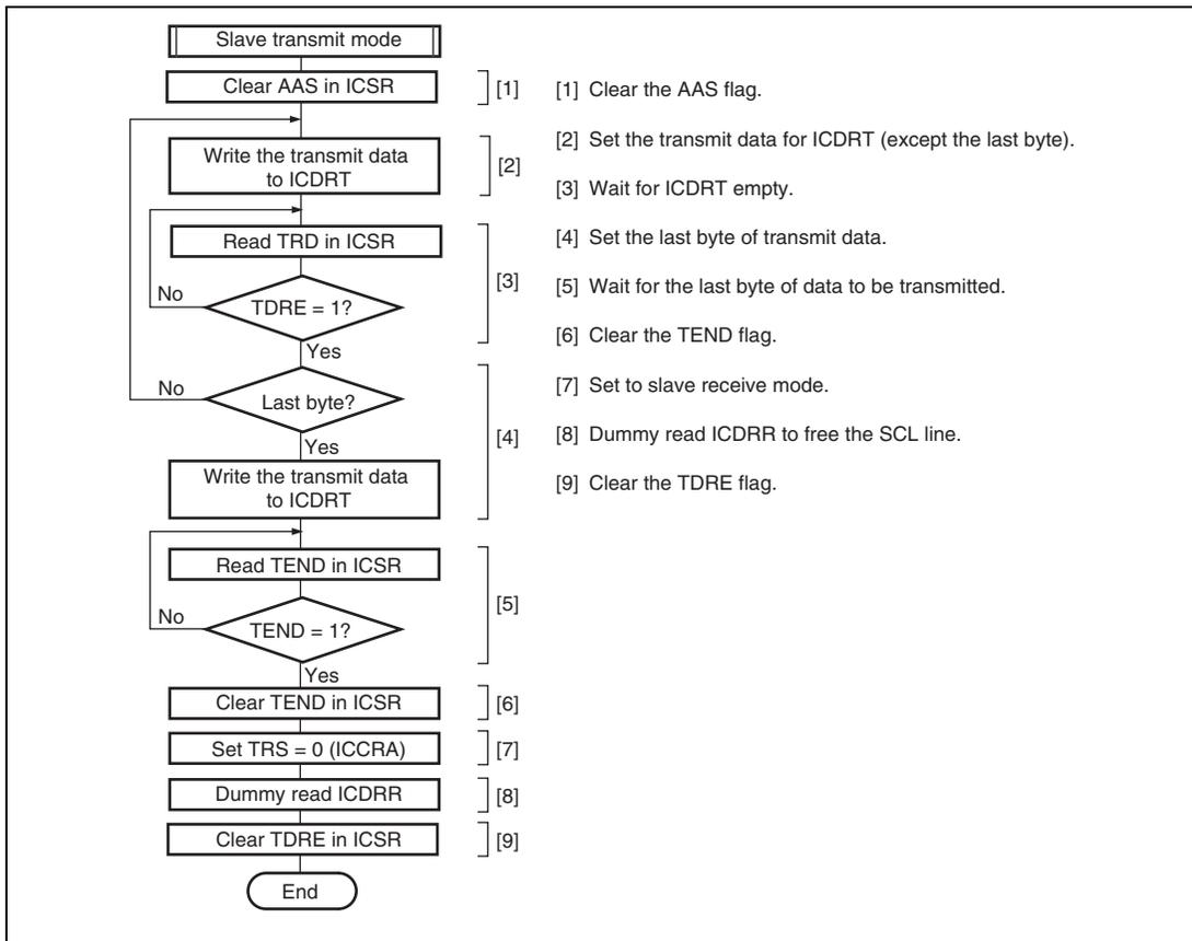
**Figure 18.16 Sample Flowchart for Slave Transmit Mode**
