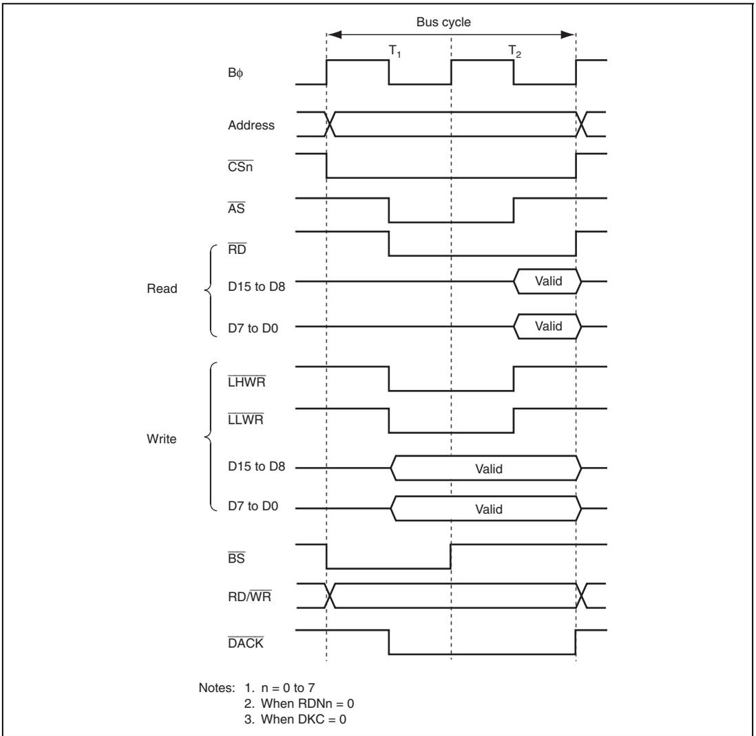
**Figure 9.16 16-Bit 2-State Access Space Bus Timing (Word Access for Even Address)**
