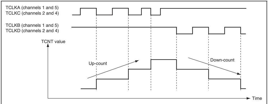
**Figure 13.28 Example of Phase Counting Mode 3 Operation**
