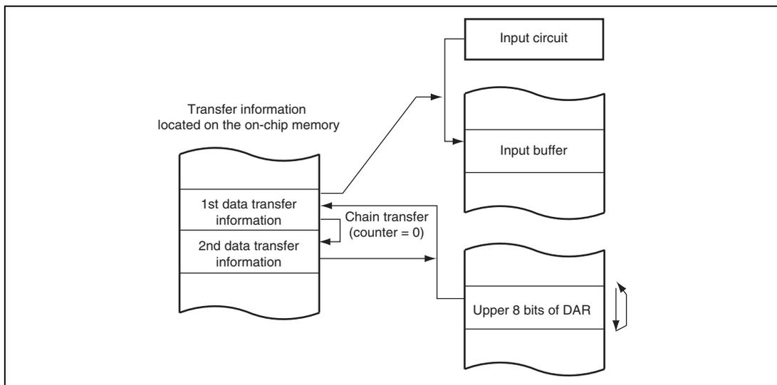
**Figure 11.16 Chain Transfer when Counter = 0**
