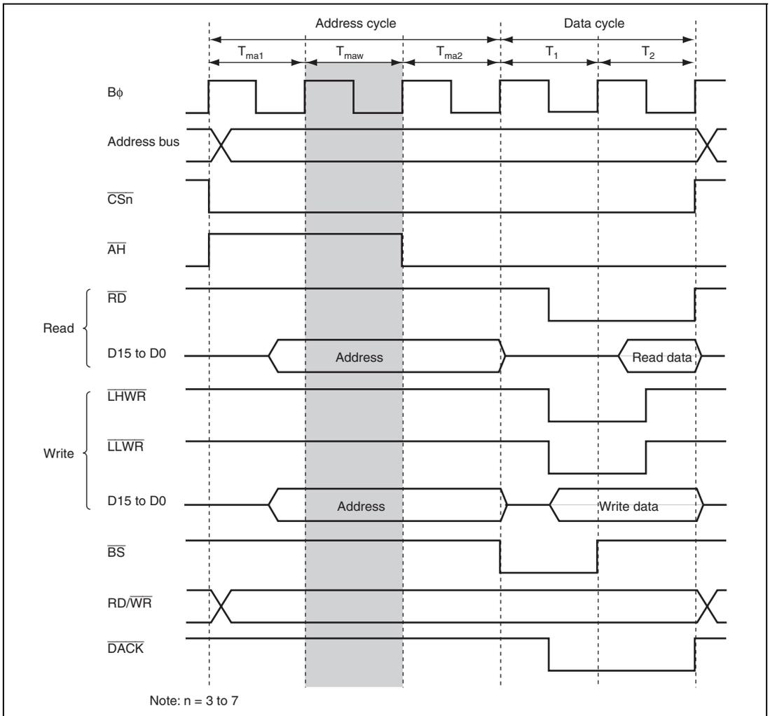
**Figure 9.32 Access Timing of 3 Address Cycles ( $\overline{ADDEX} = 1$ )**
