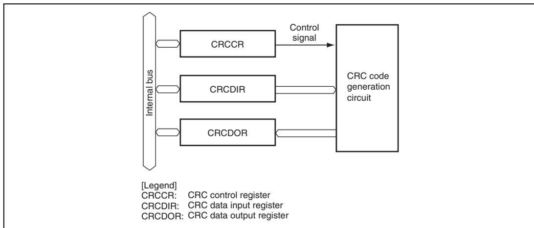
**Figure 17.43 Block Diagram of CRC Operation Circuit**
