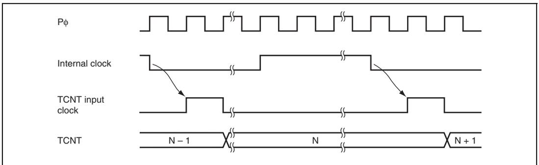
**Figure 15.7** Count Timing for Internal Clock Input
