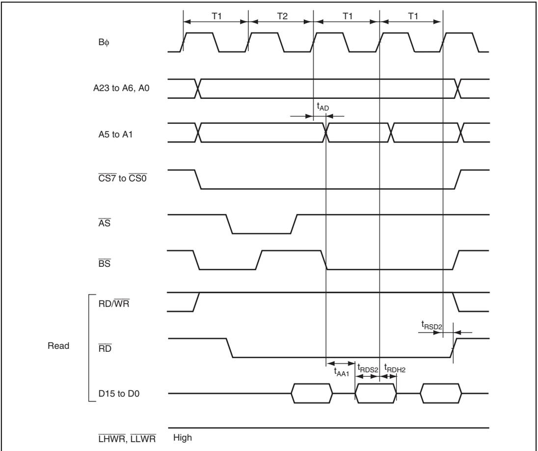
**Figure 27.15 Burst ROM Access Timing: One-State Burst Access**
