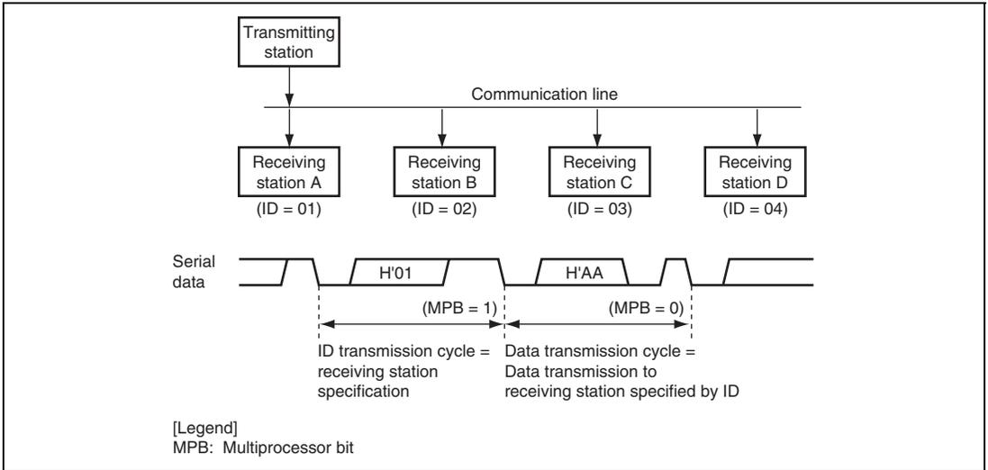
**Figure 17.13 Example of Communication Using Multiprocessor Format
