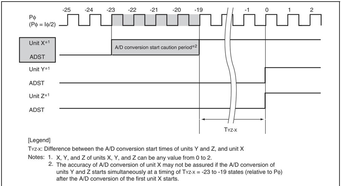
**Figure 19.16 When A/D Conversion Accuracy of Unit X whose A/D Conversion Starts First is not Assured: Case 1**
