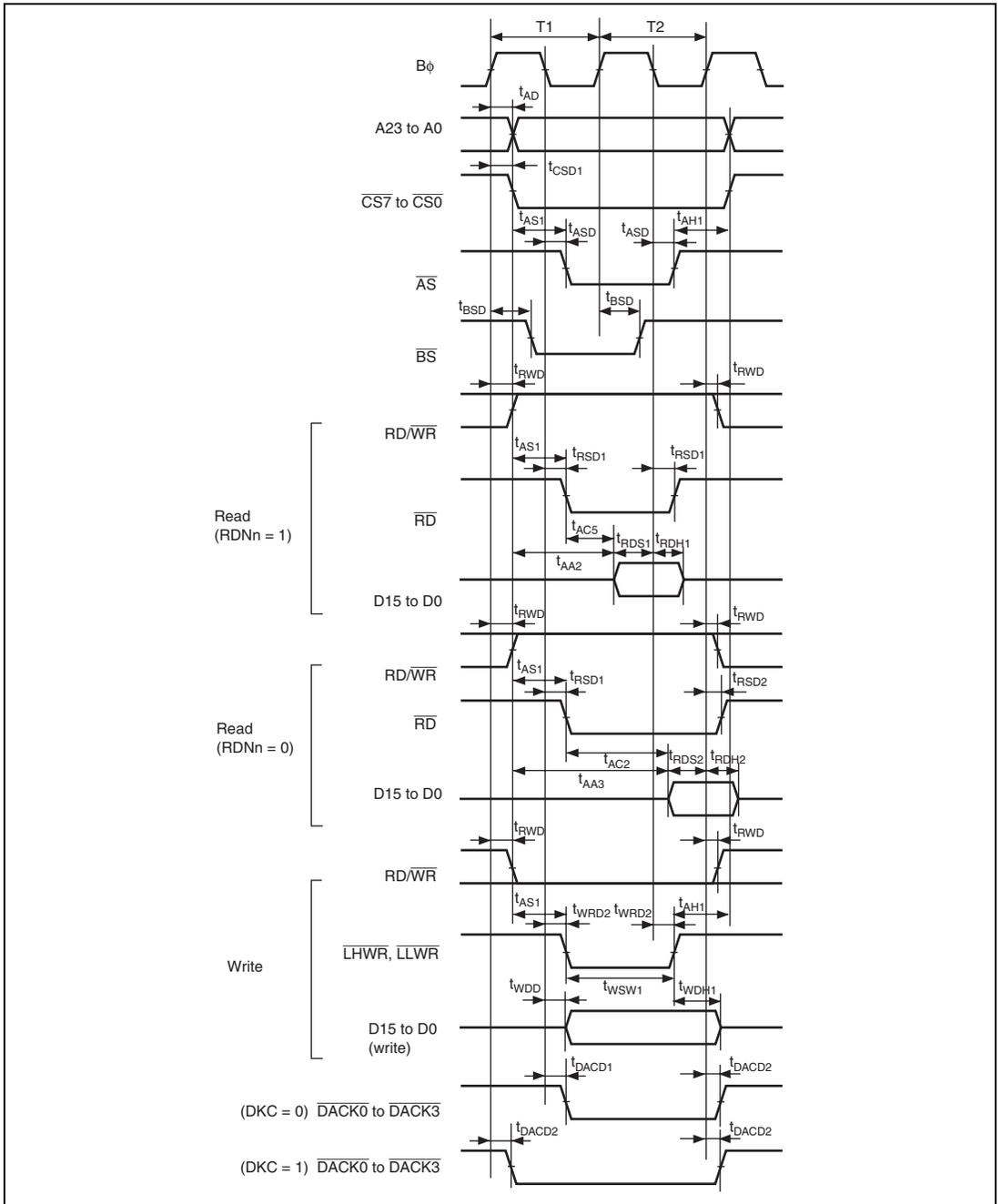
Figure 27.8 Basic Bus Timing: Two-State Access
