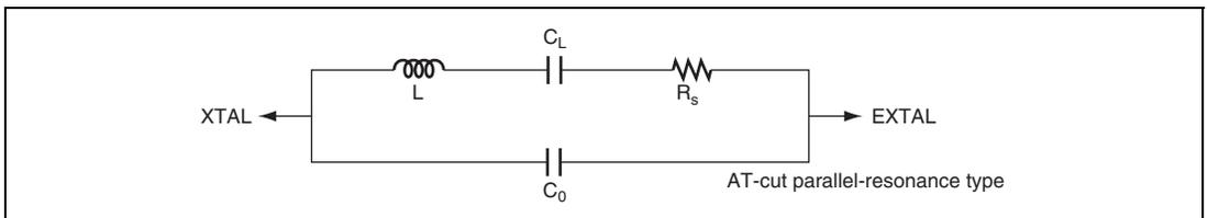
**Figure 24.3 Crystal Resonator Equivalent Circuit**
