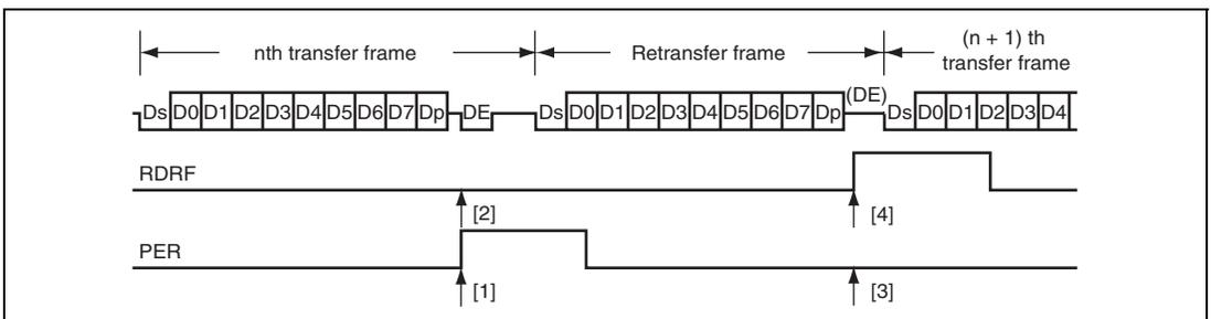
**Figure 17.32 Data Re-Transfer Operation in SCI Reception Mode**
