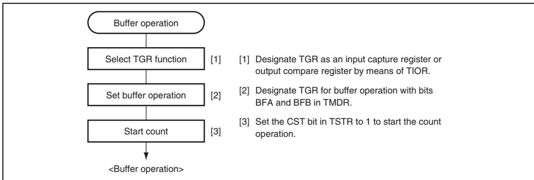
**Figure 13.15 Example of Buffer Operation Setting Procedure**
