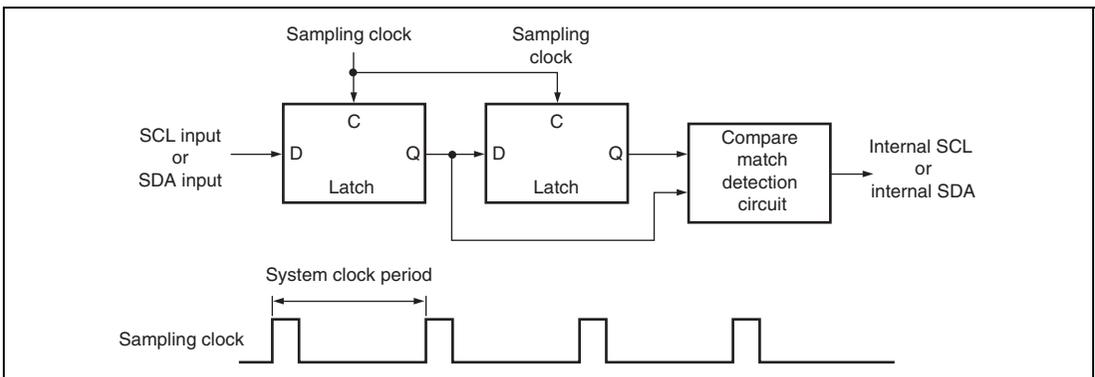
**Figure 18.13 Block Diagram of Noise Canceller**
