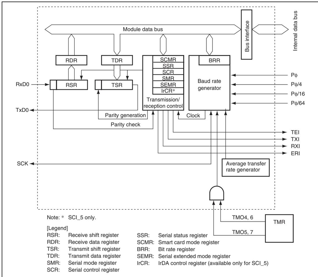
**Figure 17.2 Block Diagram of SCI\_5 and SCI\_6**
