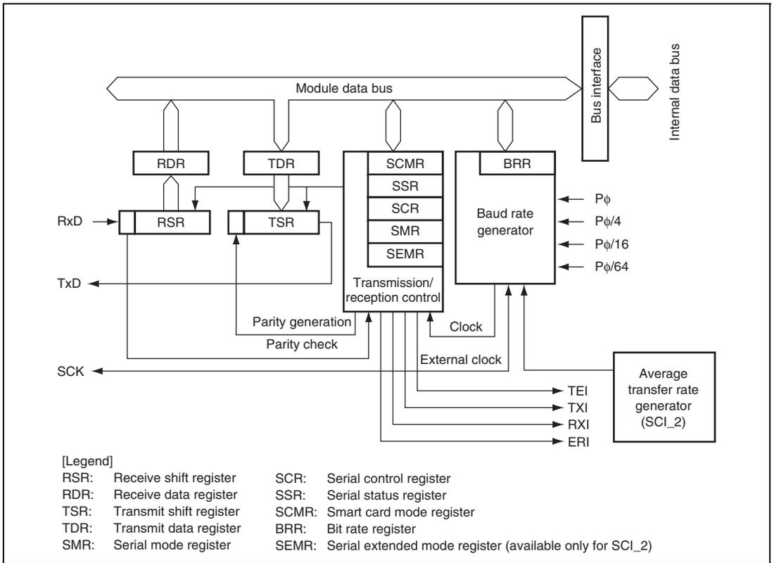
**Figure 17.1 Block Diagram of SCI\_0, 1, 2, 3, and 4**
