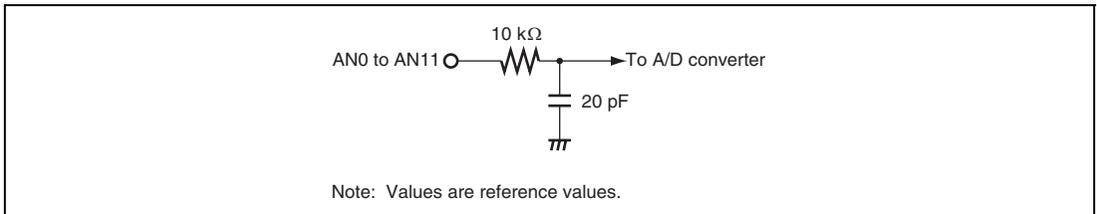
**Figure 19.23 Analog Input Pin Equivalent Circuit**
