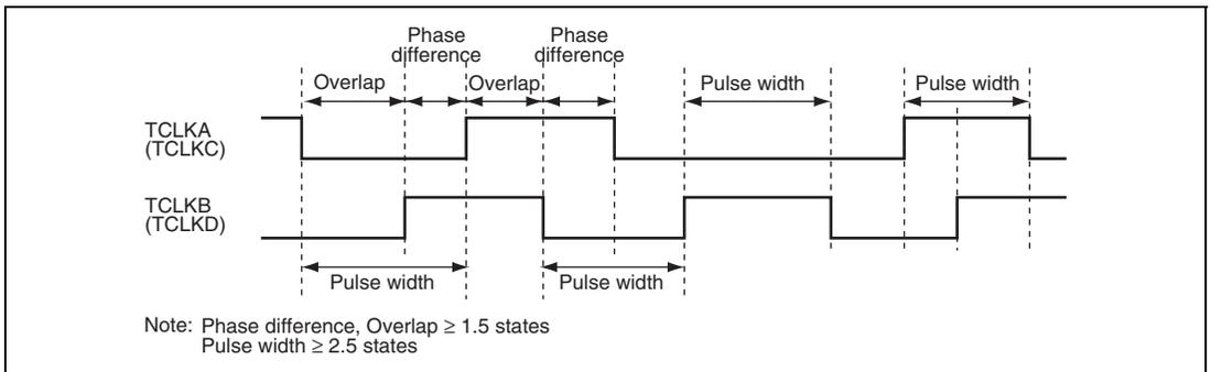
**Figure 13.46 Phase Difference, Overlap, and Pulse Width in Phase Counting Mode**
