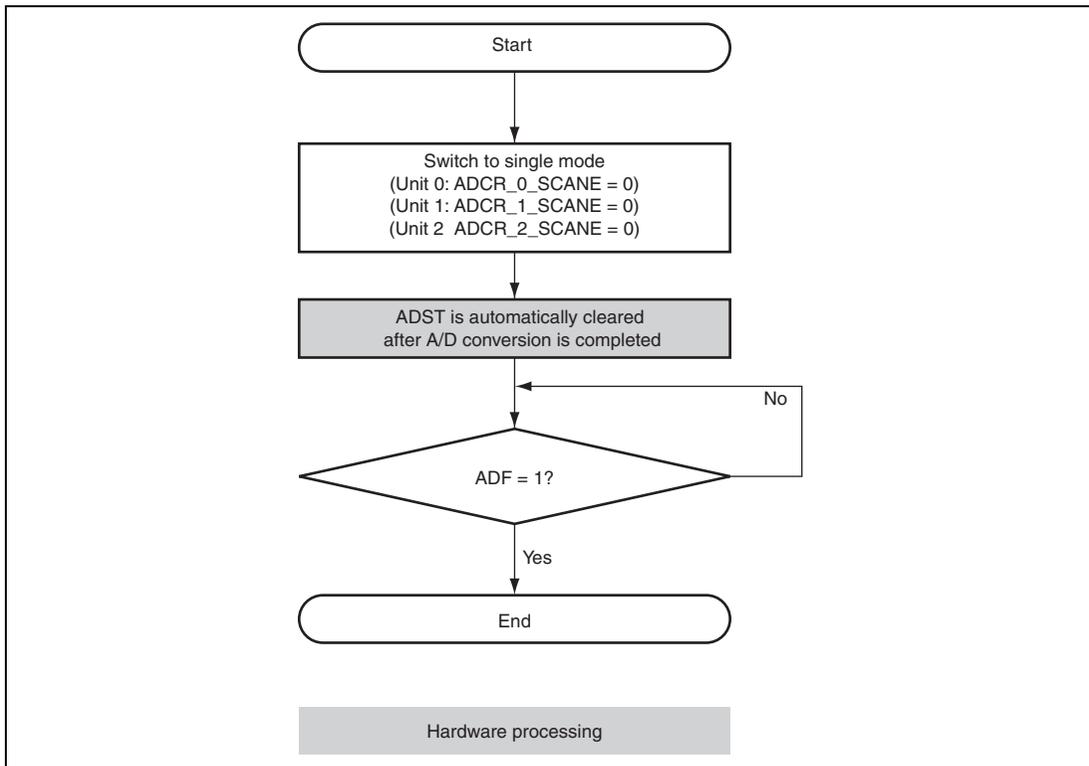
**Figure 19.12 Stopping Continuous Scan Mode Activated by Software**
