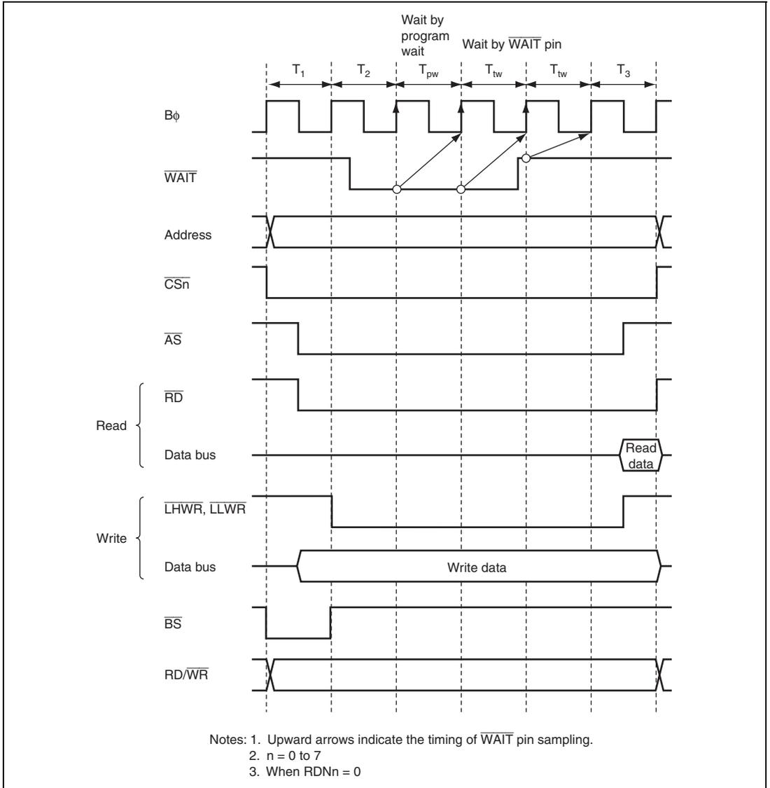
**Figure 9.20 Example of Wait Cycle Insertion Timing**
