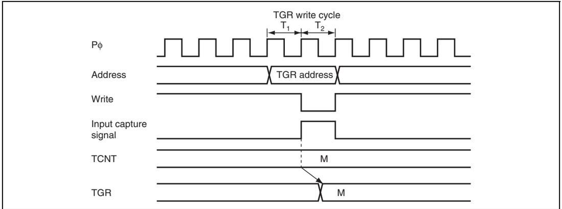
**Figure 13.52 Conflict between TGR Write and Input Capture**
