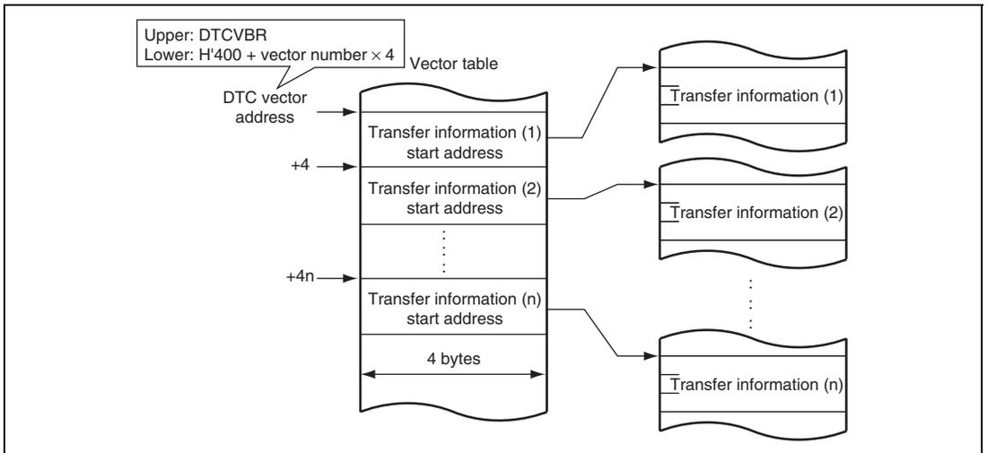
**Figure 11.3 Correspondence between DTC Vector Address and Transfer Information**
