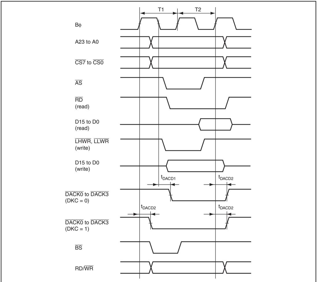
**Figure 27.23 Single Address Transfer Timing for the DMAC (Two-State Access)**
