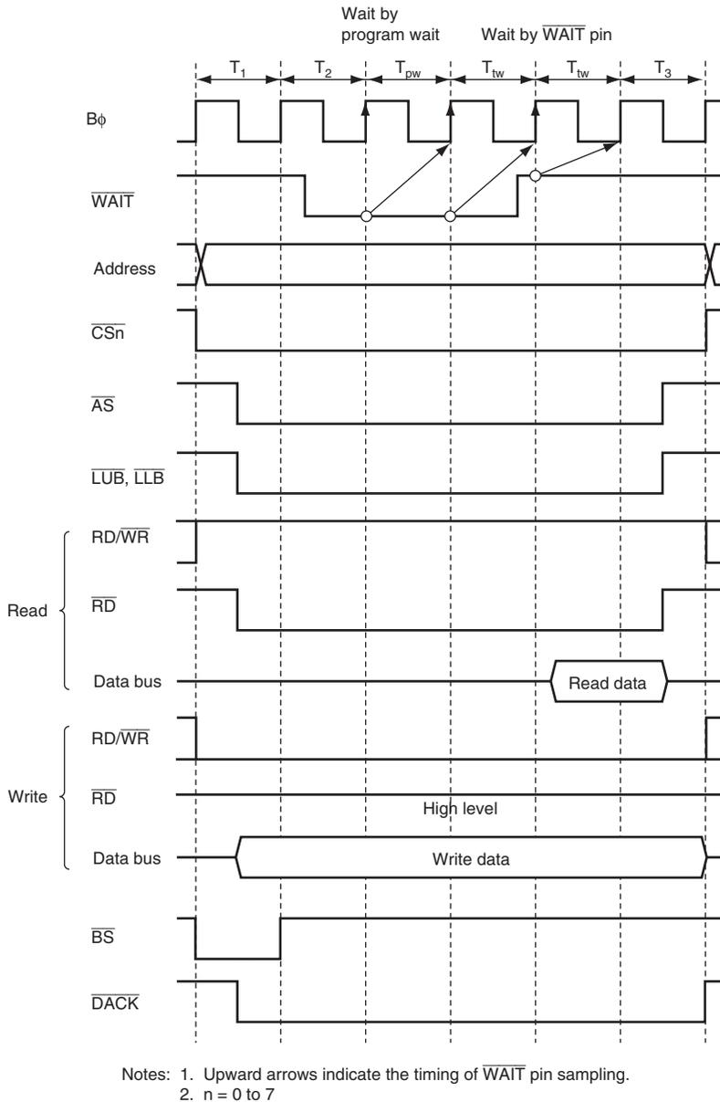
**Figure 9.26 Example of Wait Cycle Insertion Timing**
