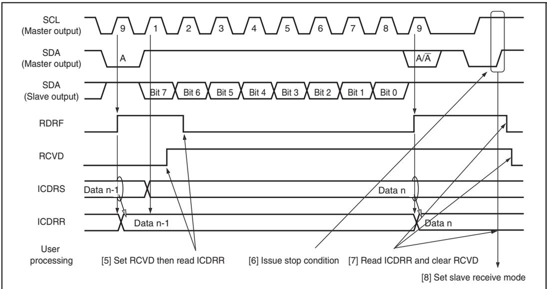
**Figure 18.8 Master Receive Mode Operation Timing 2**
