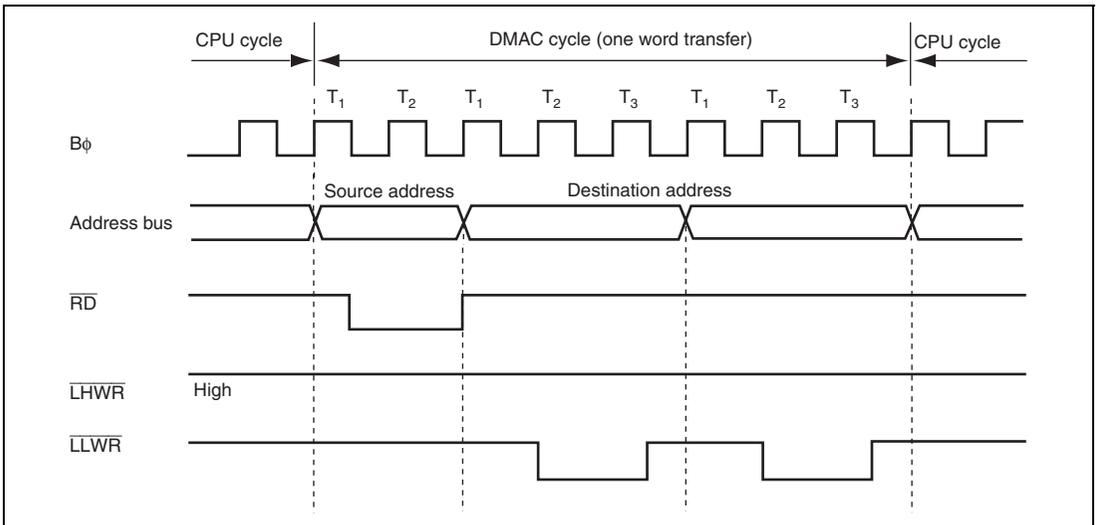
**Figure 10.23 Example of Bus Timing of DMA Transfer**
