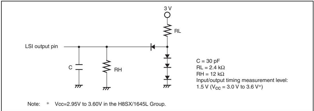
**Figure 27.1 Output Load Circuit**
