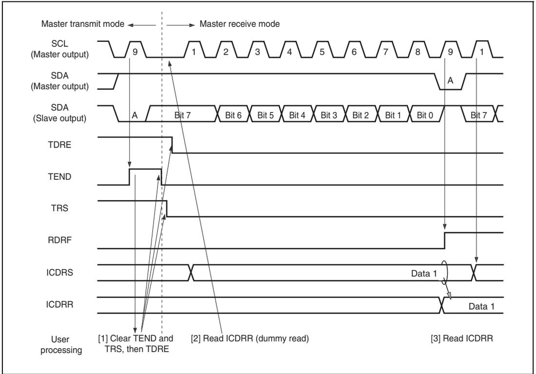
**Figure 18.7 Master Receive Mode Operation Timing 1**
