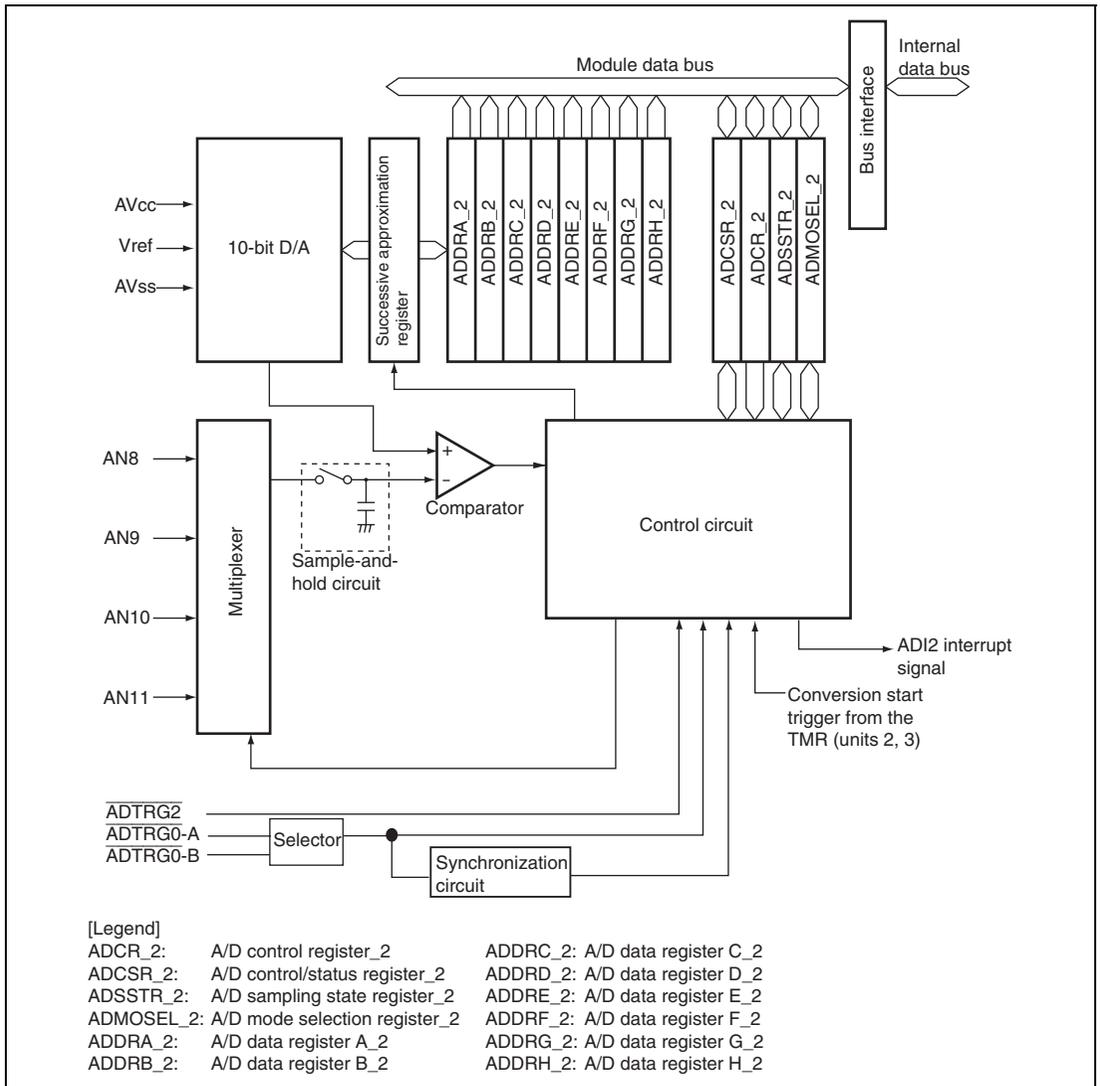
**Figure 19.3 Block Diagram of A/D Converter Unit 2 (AD\_2)**
