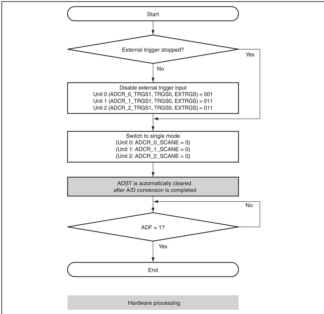
**Figure 19.13 Stopping Continuous Scan Mode Activated by External Trigger**
