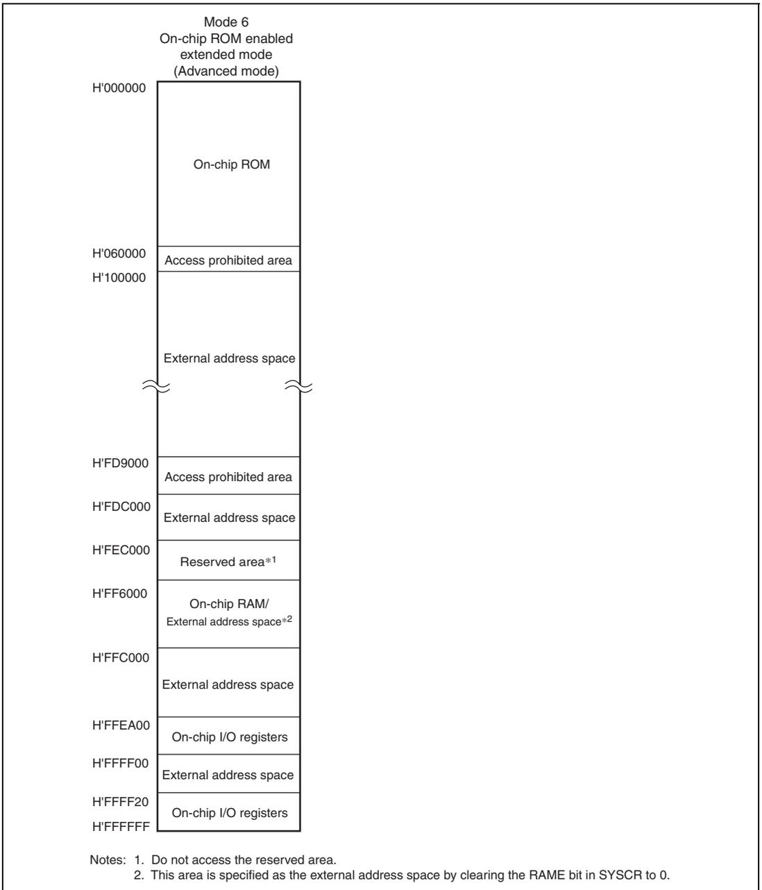
**Figure 3.3 Address Map in Each Operating Mode of H8SX/1641 and H8SX/1641L (2)**
