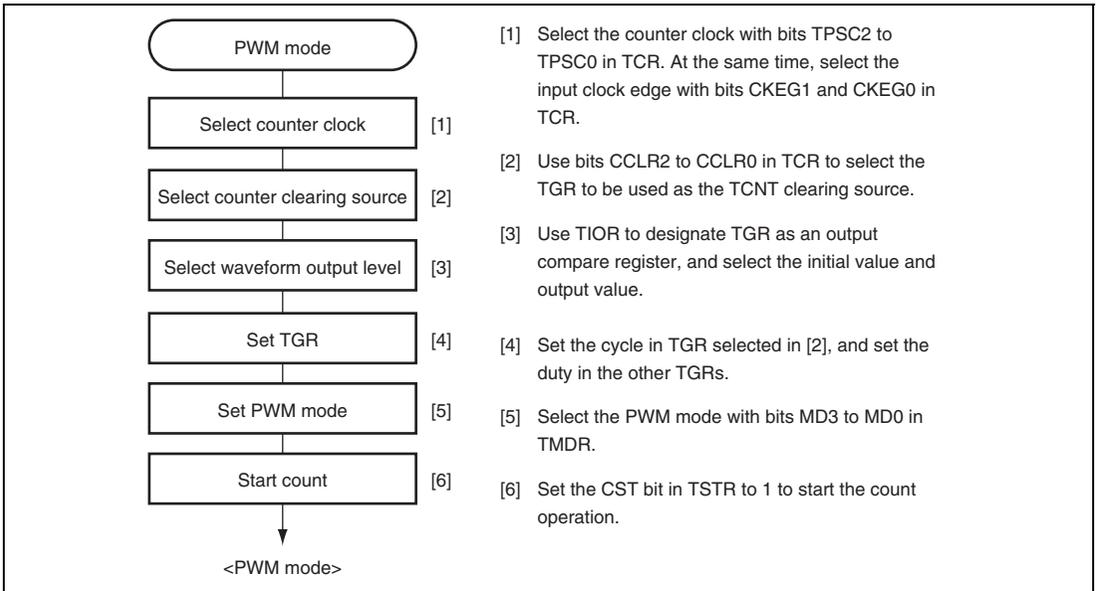
**Figure 13.21 Example of PWM Mode Setting Procedure**
