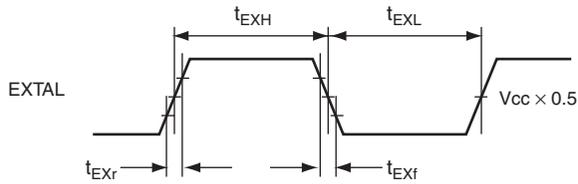
**Figure 27.5 External Input Clock Timing**
