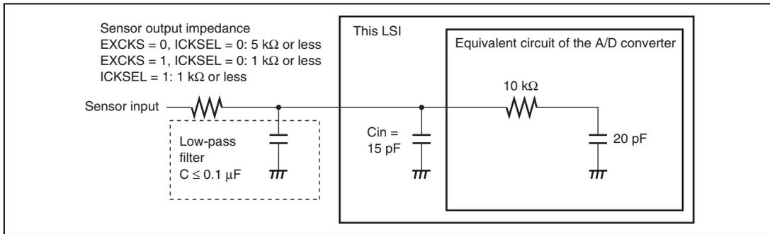
**Figure 19.21 Example of Analog Input Circuit**
