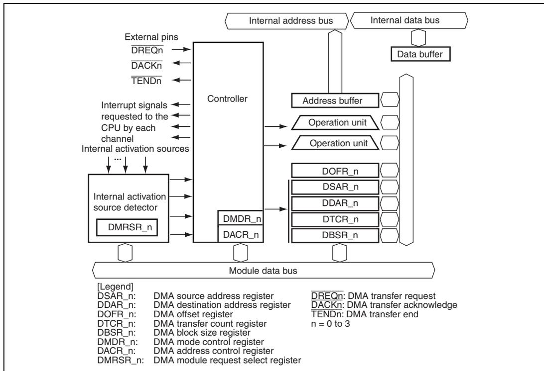
**Figure 10.1 Block Diagram of DMAC**
