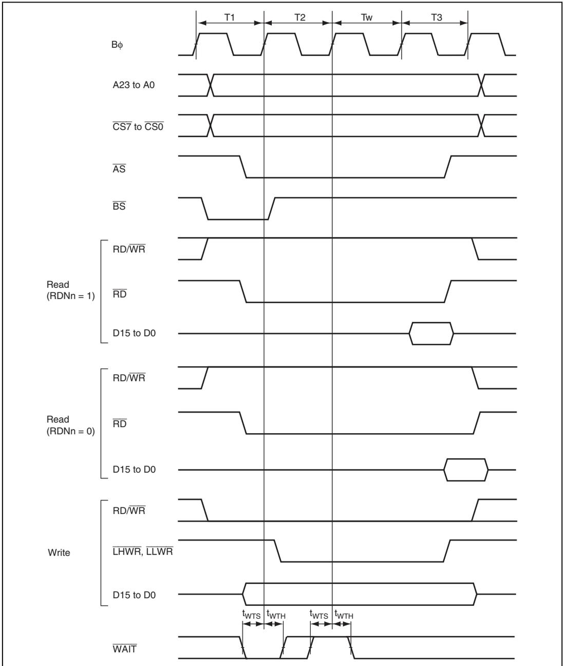
**Figure 27.10 Basic Bus Timing: Three-State Access, One Wait**
