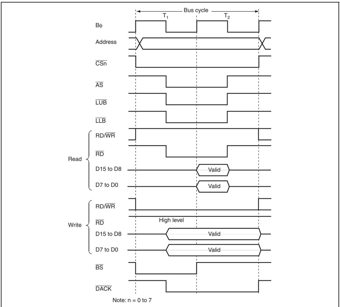
**Figure 9.24 16-Bit 2-State Access Space Bus Timing**
