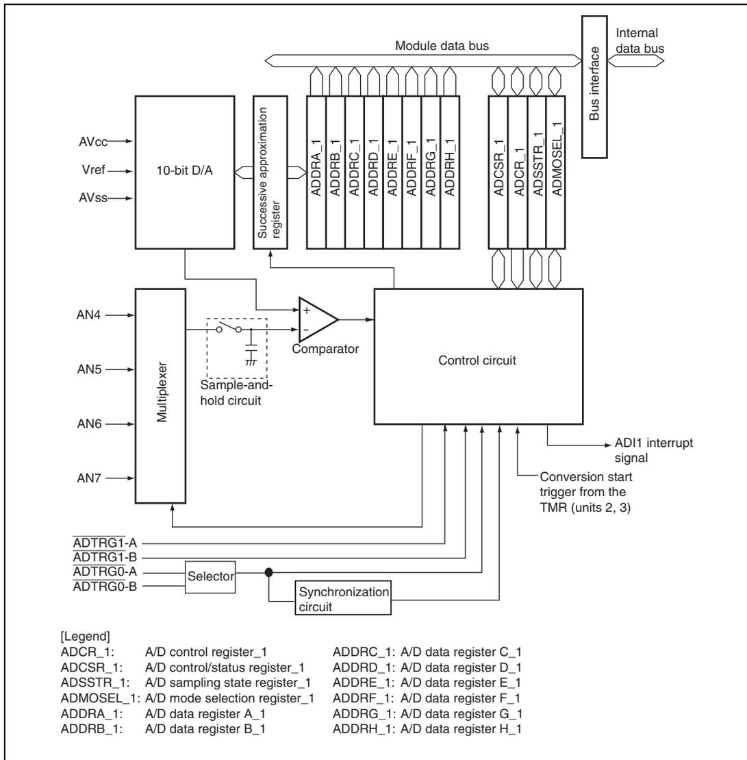
**Figure 19.2 Block Diagram of A/D Converter Unit 1 (AD\_1)**
