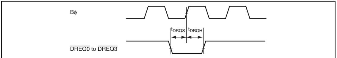
**Figure 27.21 Timing of  $\overline{DREQ}$  Input (for the DMAC)**
