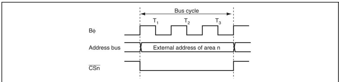
**Figure 9.8**  $\overline{CSn}$  Signal Output Timing ( $n = 0$  to 7)
