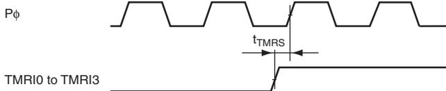
**Figure 27.30 8-Bit Timer Reset Input Timing**
