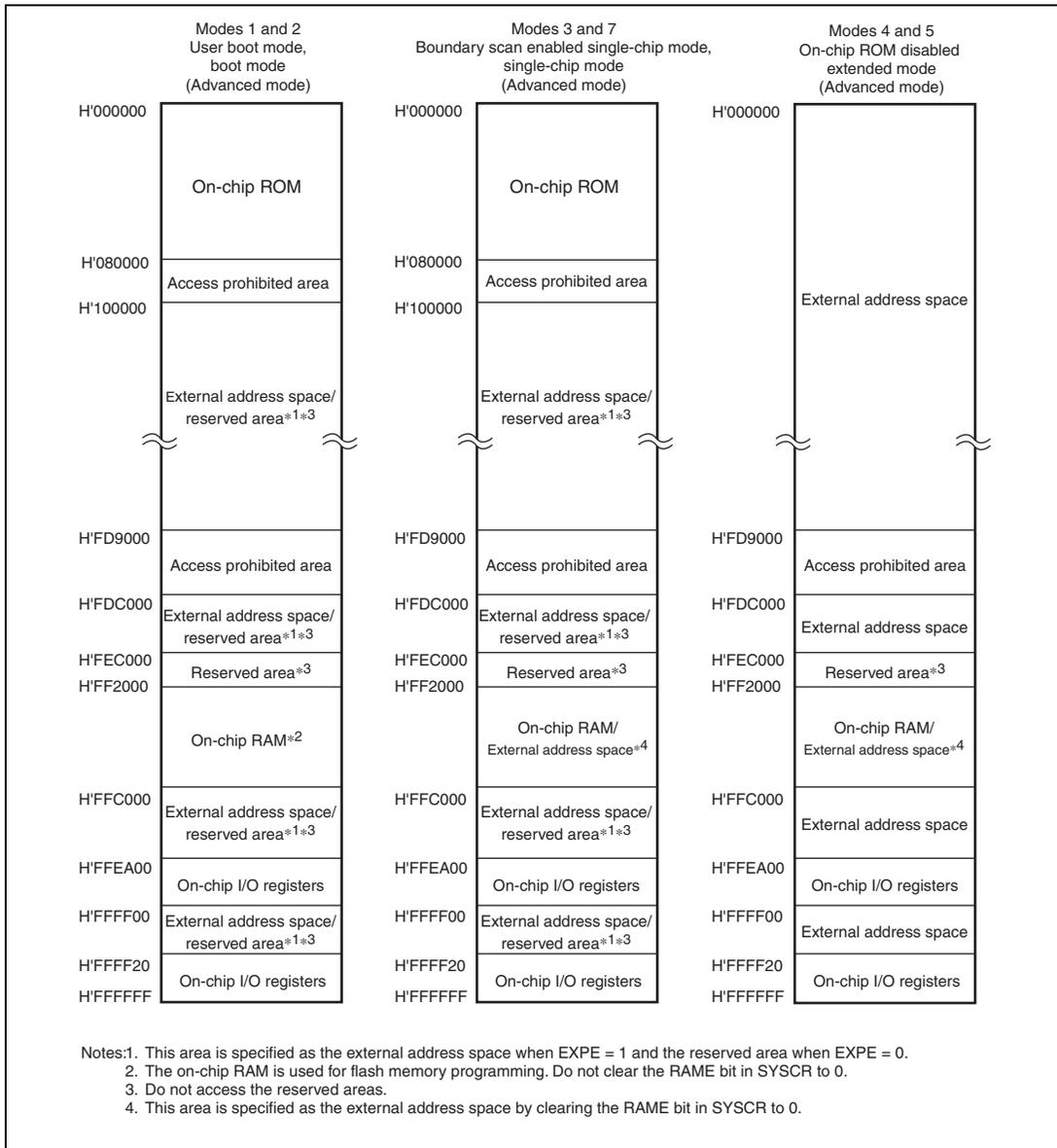
Figure 3.1 Address Map in Each Operating Mode of H8SX/1645 and H8SX/1645L (1)
