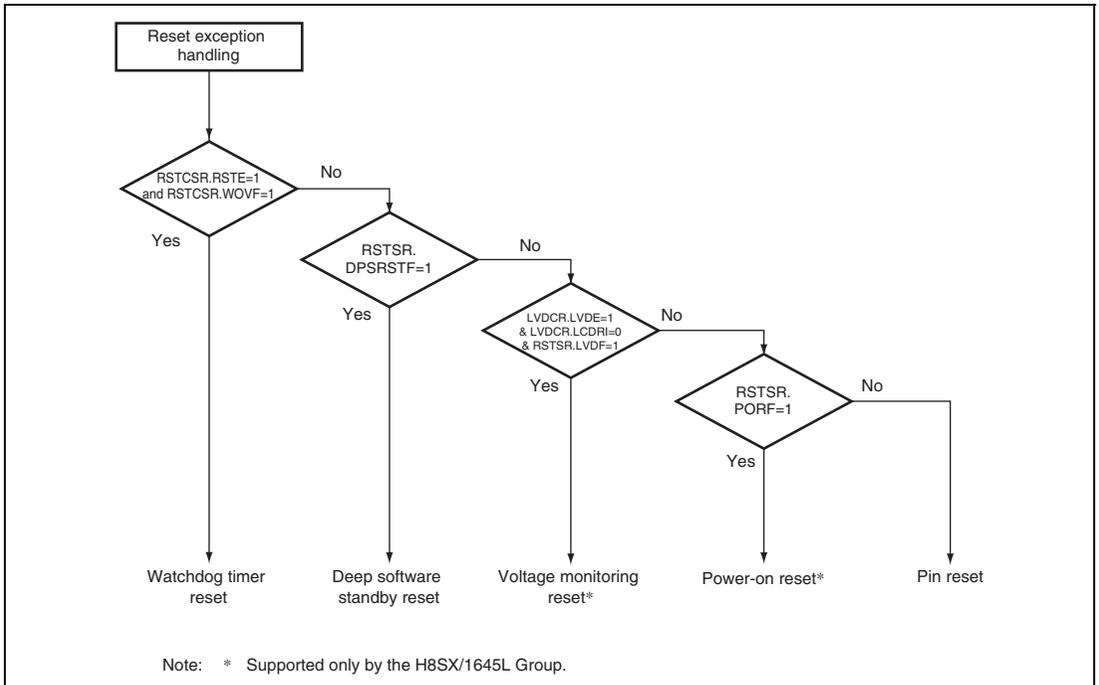
**Figure 4.3 Example of Reset Generation Source Determination Flow**
