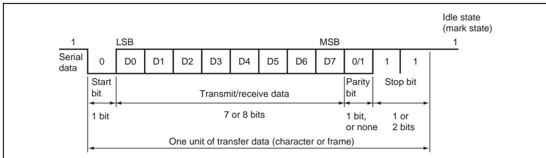
**Figure 17.5 Data Format in Asynchronous Communication**
