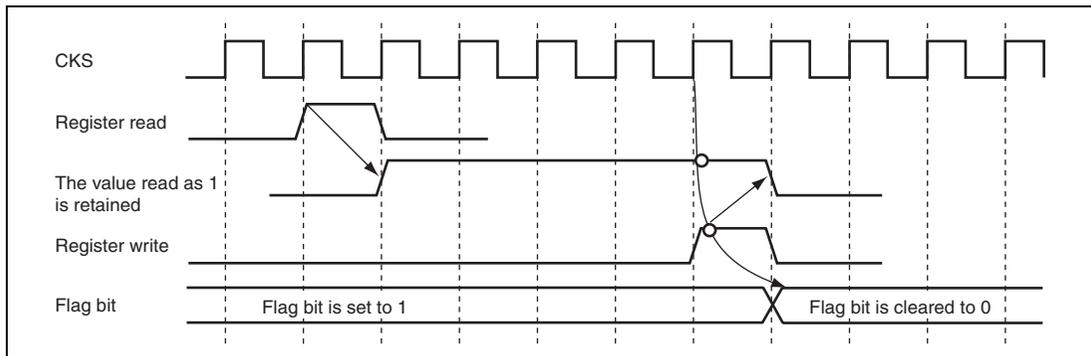
**Figure 8.3 Flag Bit Clearing Sequence (Condition Match Flag)**
