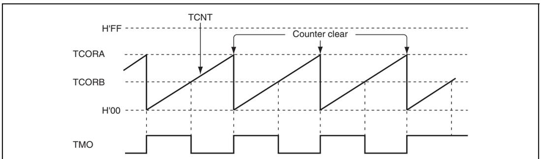
**Figure 15.5 Example of Pulse Output**
