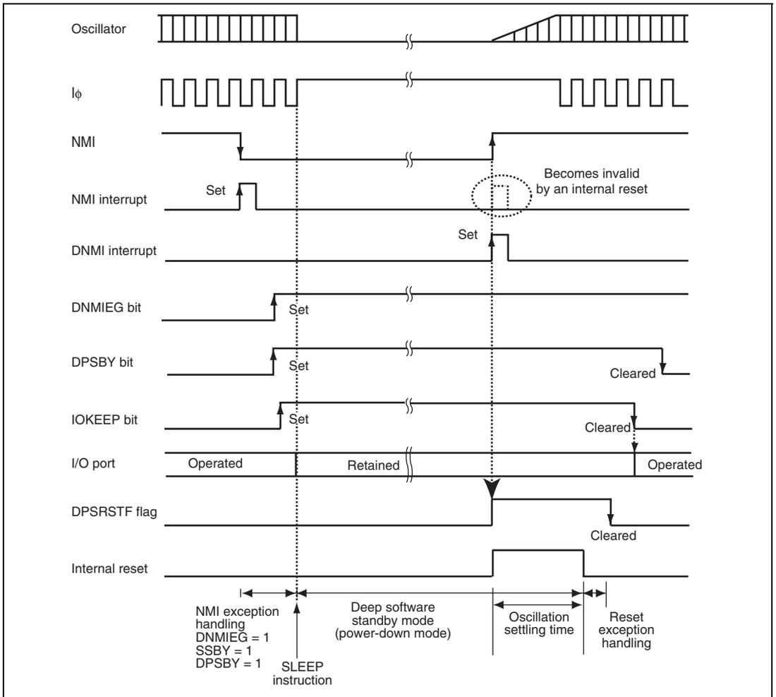
**Figure 25.4 Deep Software Standby Mode Application Example (IOKEEP = 1)**
