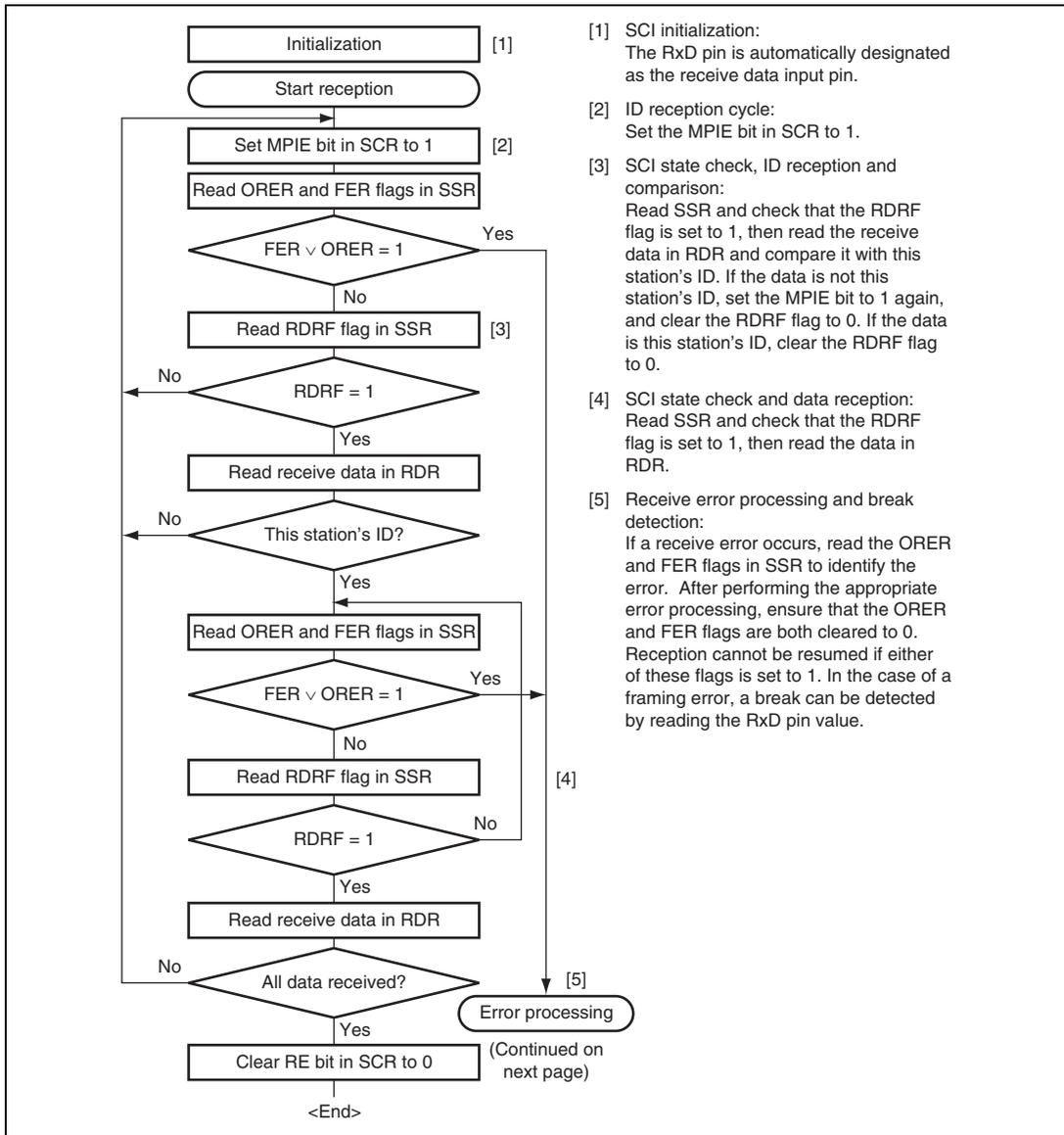
Figure 17.16 Sample Multiprocessor Serial Reception Flowchart (1)
