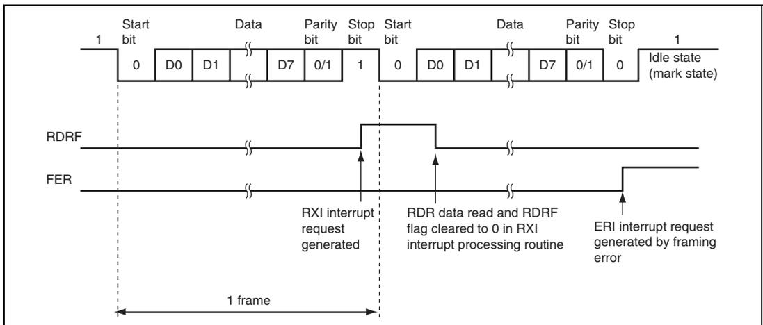
**Figure 17.11 Example of SCI Operation for Reception
