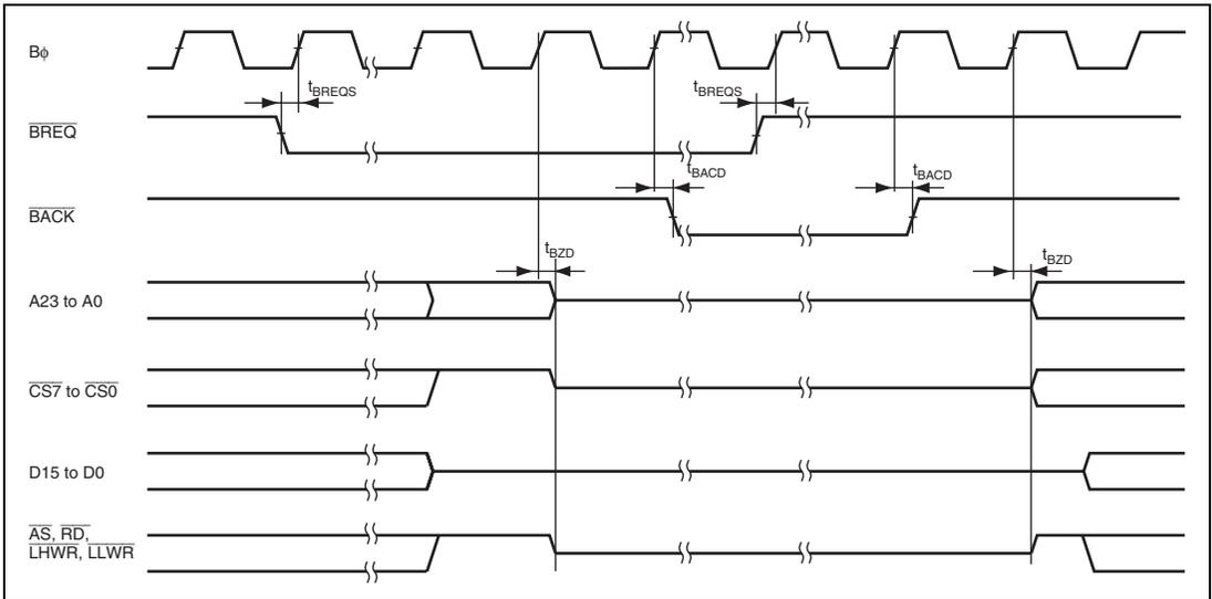
**Figure 27.19 External Bus Release Timing**
