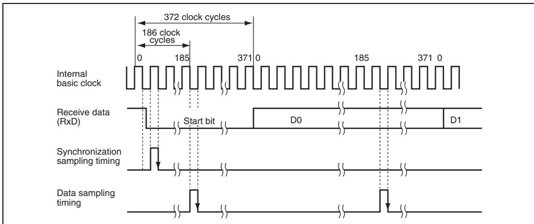
**Figure 17.28 Receive Data Sampling Timing in Smart Card Interface Mode
