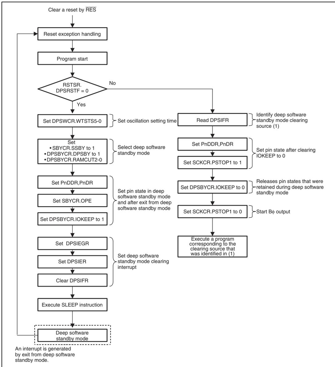
**Figure 25.7 Flowchart of Deep Software Standby Mode Operation**
