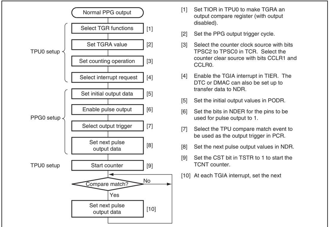
**Figure 14.5 Setup Procedure for Normal Pulse Output (PPG0)**
