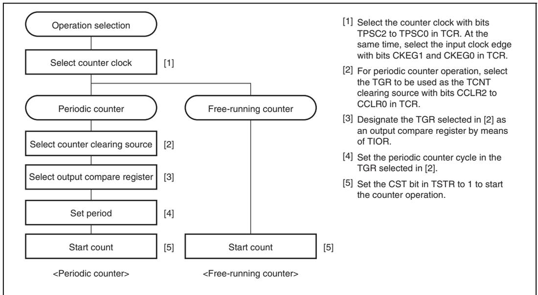
**Figure 13.3 Example of Counter Operation Setting Procedure**
