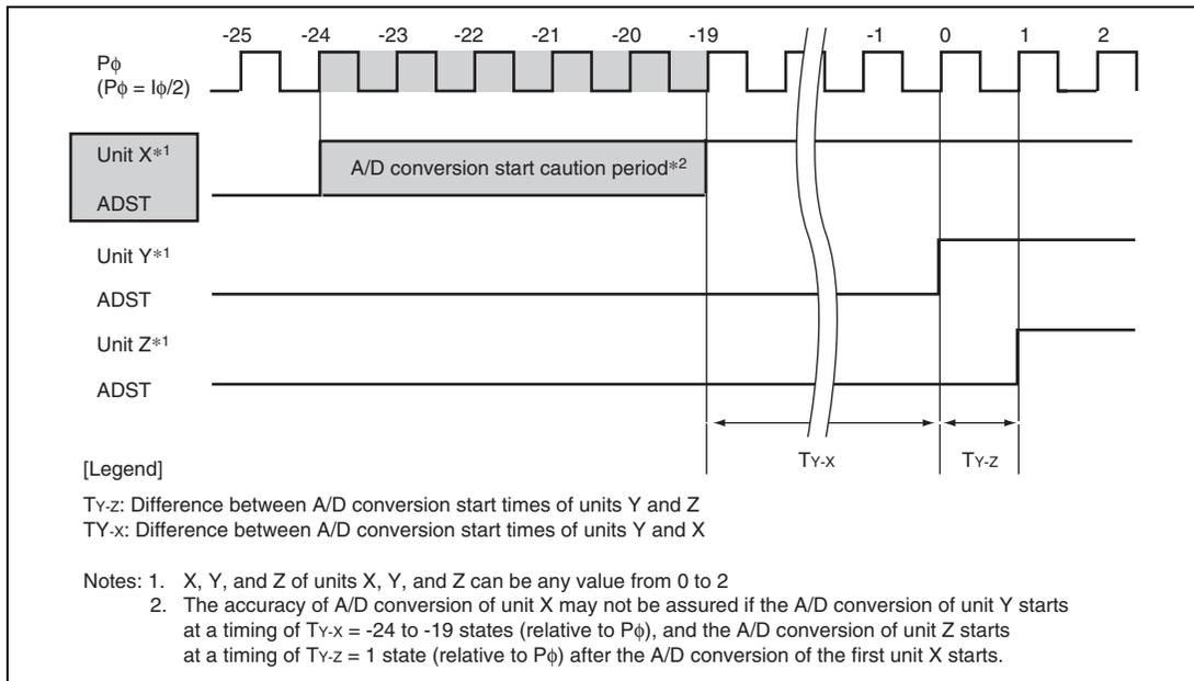
**Figure 19.17 When A/D Conversion Accuracy of Unit X whose A/D Conversion Starts First is not Assured: Case 2**
