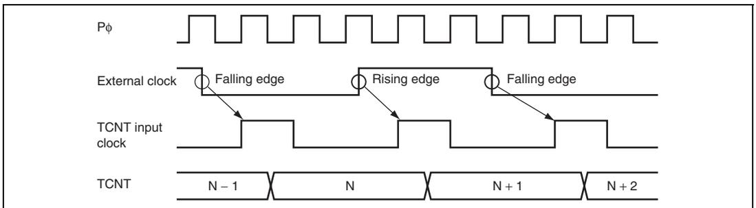
**Figure 13.32 Count Timing in External Clock Operation**
