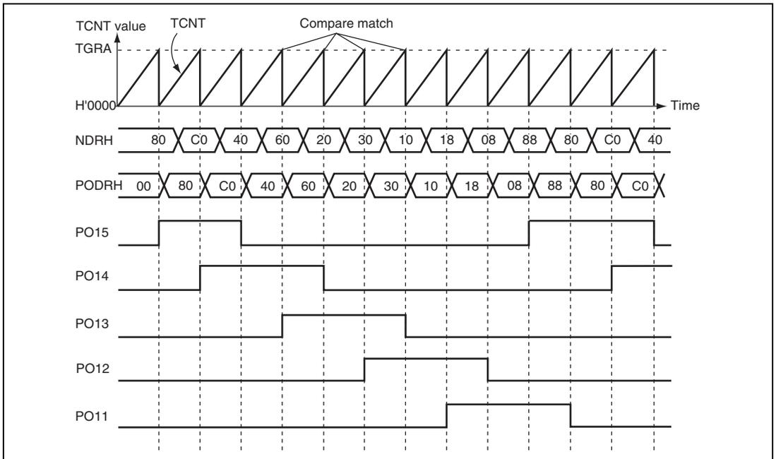
**Figure 14.7 Normal Pulse Output Example (5-Phase Pulse Output)**
