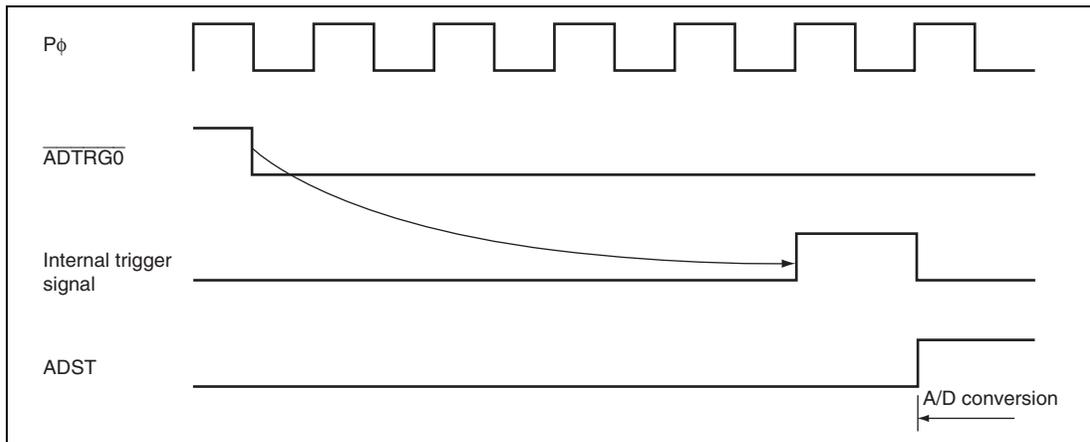
**Figure 19.9 External Trigger Input Timing when Multiple Units Start Simultaneously (TRSG1, TRGS0, and EXTRGS = B'111)**
