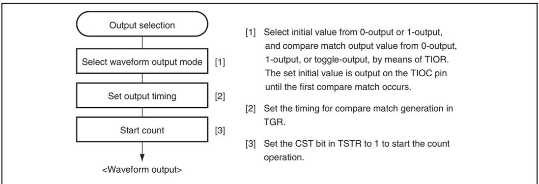
**Figure 13.6 Example of Setting Procedure for Waveform Output by Compare Match**
