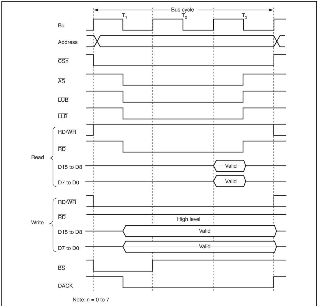
**Figure 9.25 16-Bit 3-State Access Space Bus Timing**
