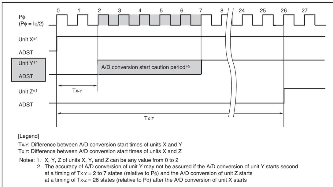
**Figure 19.20 When A/D Conversion Accuracy of Unit Y whose A/D Conversion Starts Second is not Assured: Case 3**
