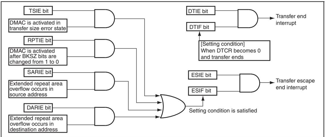
Figure 10.39 Interrupt and Interrupt Sources
