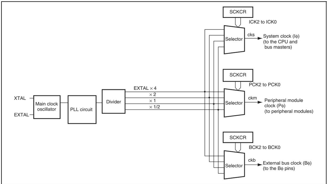
**Figure 24.1 Block Diagram of Clock Pulse Generator**
