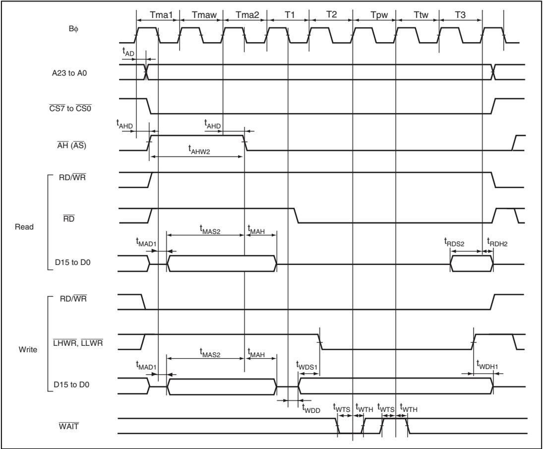
**Figure 27.18 Address/Data Multiplexed Access Timing (Wait Control)**
