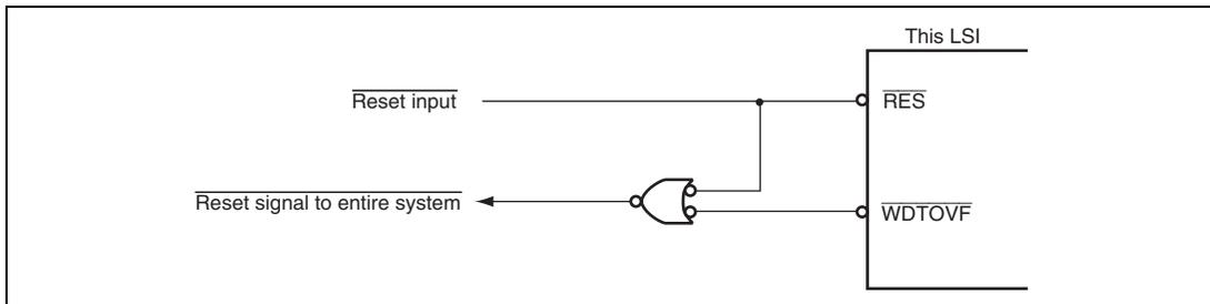
**Figure 16.6** Circuit for System Reset by  $\overline{\text{WDTOVF}}$  Signal (Example)
