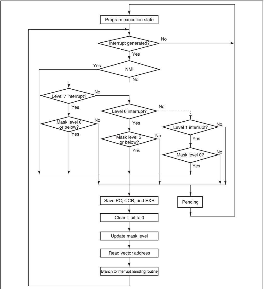
**Figure 7.4 Flowchart of Procedure Up to Interrupt Acceptance
