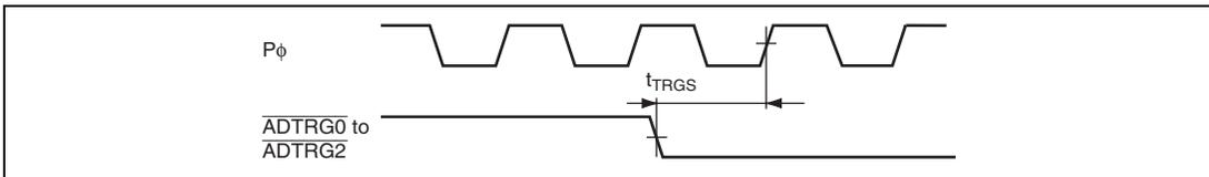
**Figure 27.35 A/D Converter External Trigger Input Timing**
