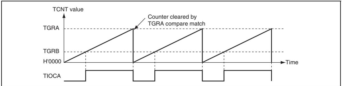
**Figure 13.22 Example of PWM Mode Operation (1)**
