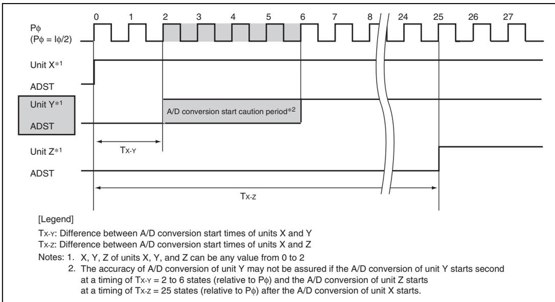
**Figure 19.19 When A/D Conversion Accuracy of Unit Y whose A/D Conversion Starts Second is not Assured: Case 2**
