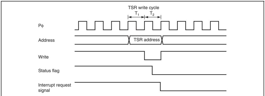
**Figure 13.43 Timing for Status Flag Clearing by CPU**
