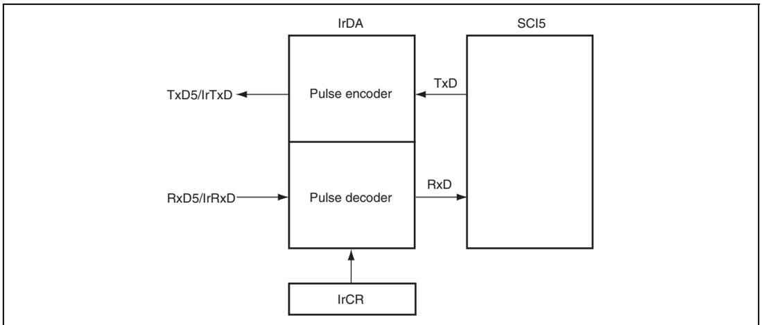
**Figure 17.36 IrDA Block Diagram**
