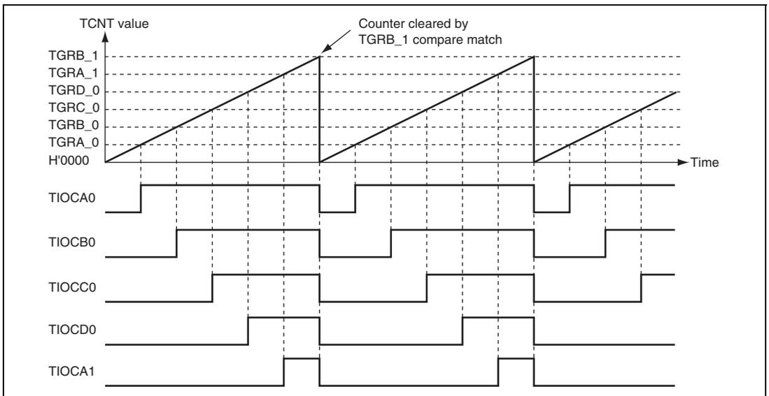
**Figure 13.23 Example of PWM Mode Operation (2)**
