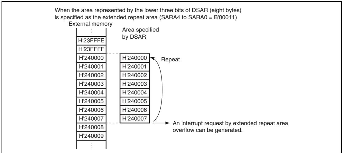
**Figure 10.15 Example of Extended Repeat Area Operation**
