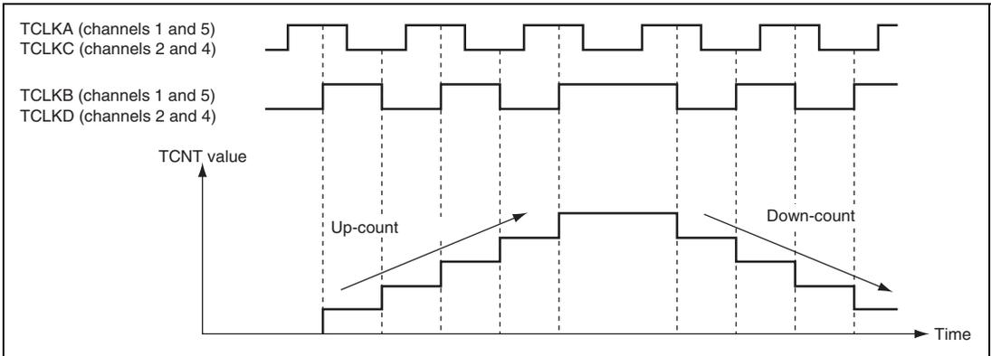
**Figure 13.29 Example of Phase Counting Mode 4 Operation**
