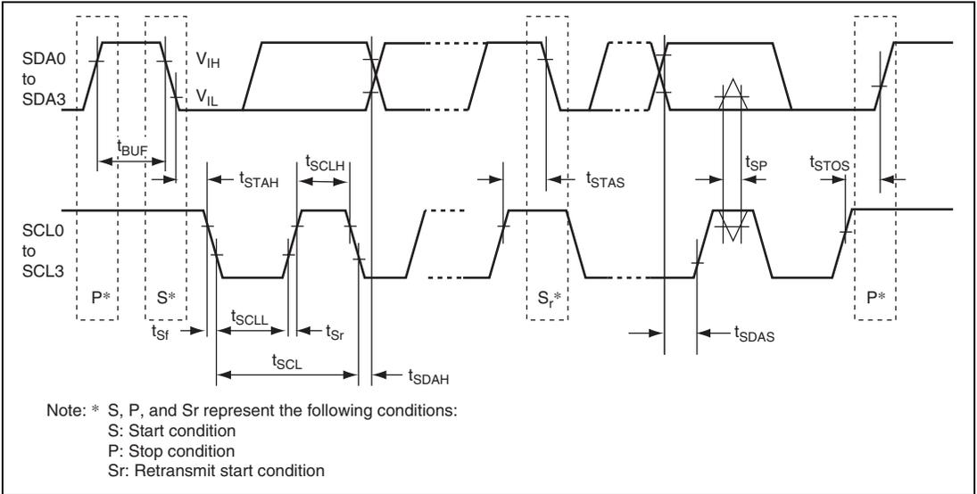
**Figure 27.36 I<sup>2</sup>C Bus Interface 2 Input/Output Timing (Option)**
