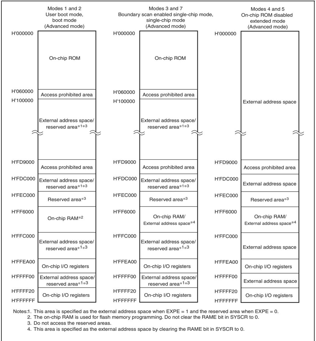
Figure 3.3 Address Map in Each Operating Mode of H8SX/1641 and H8SX/1641L (1)
