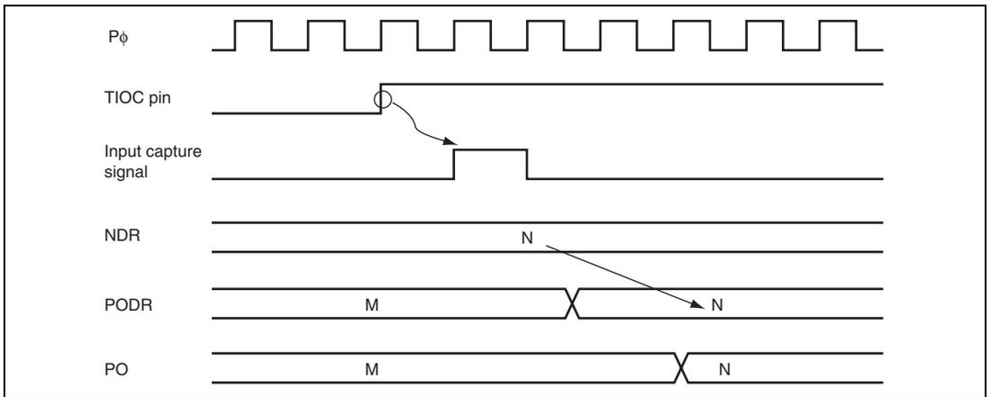
**Figure 14.14 Pulse Output Triggered by Input Capture (Example)**
