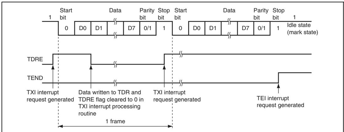
**Figure 17.9 Example of Operation for Transmission in Asynchronous Mode
