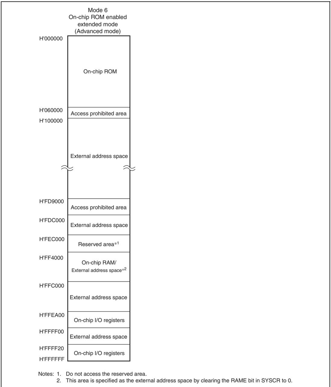
**Figure 3.2 Address Map in Each Operating Mode of H8SX/1643 and H8SX/1643L (2)**
