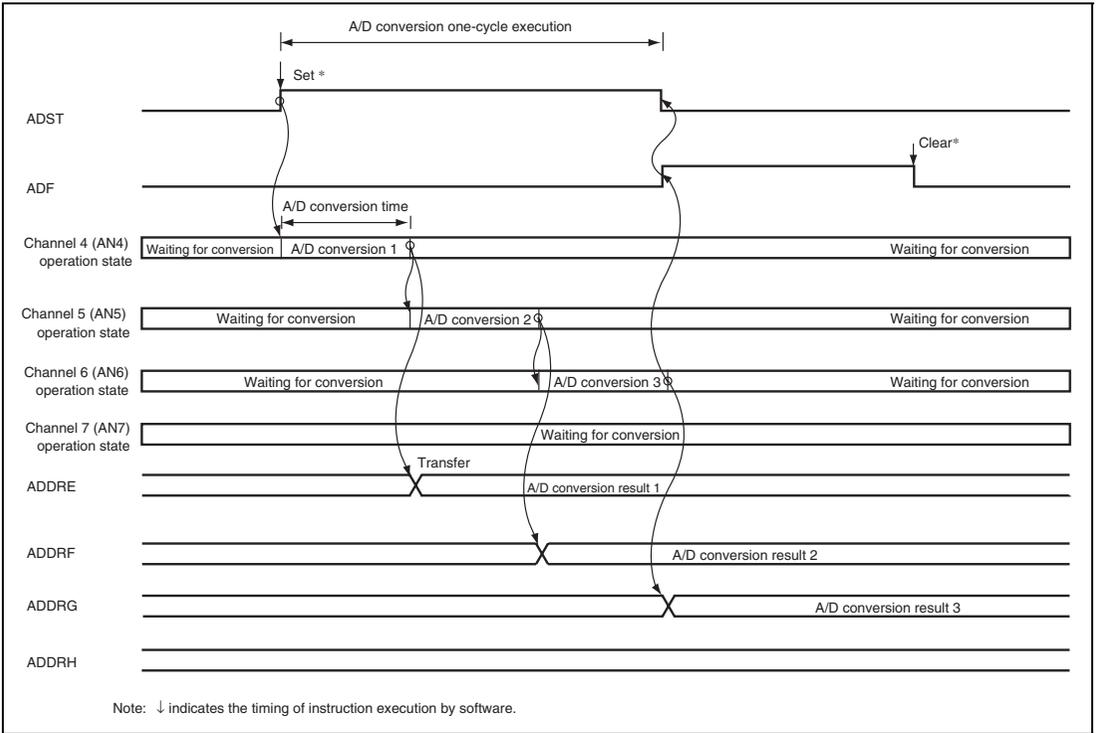
**Figure 19.6 Example of A/D Conversion
