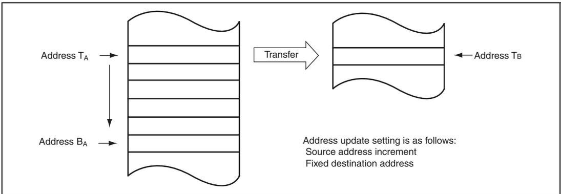
**Figure 10.3 Operations in Dual Address Mode**
