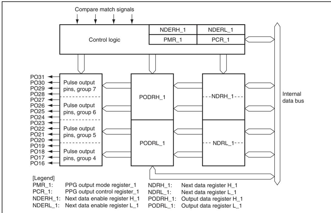
**Figure 14.2 Block Diagram of PPG (Unit 1)**
