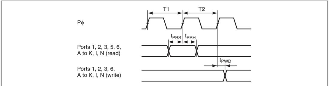
**Figure 27.25 I/O Port Input/Output Timing**
