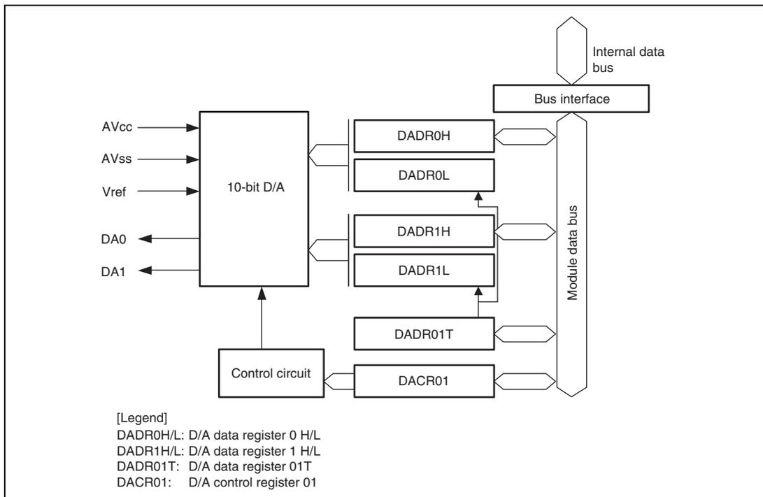
**Figure 20.1 Block Diagram of the 10-Bit D/A Converter**
