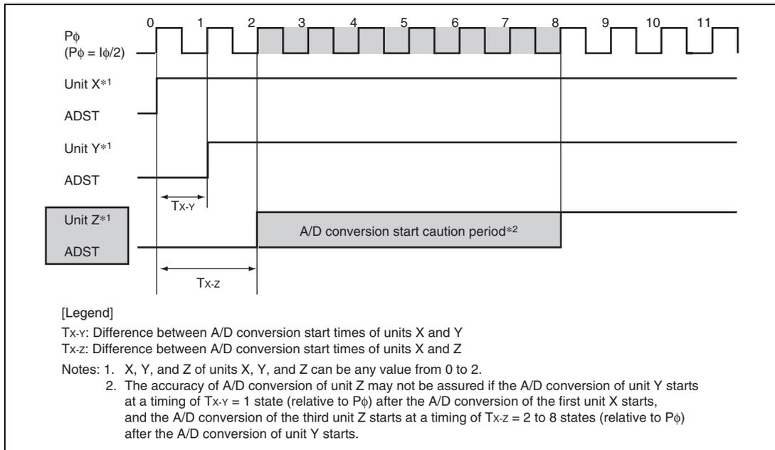
**Figure 19.15 When A/D Conversion Accuracy of Unit Z whose A/D Conversion Starts Third is not Assured: Case 2**
