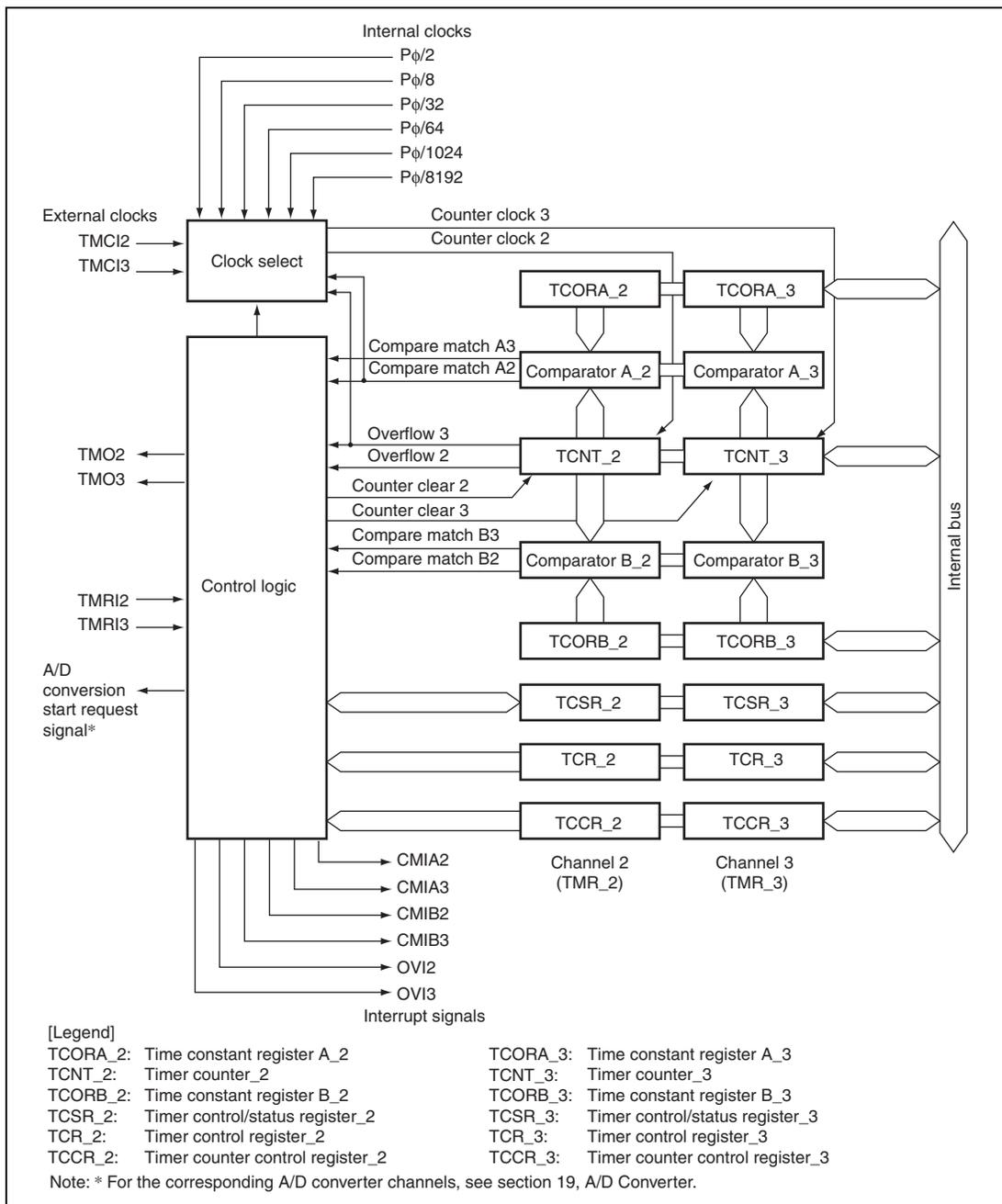
Figure 15.2 Block Diagram of 8-Bit Timer Module (Unit 1)
