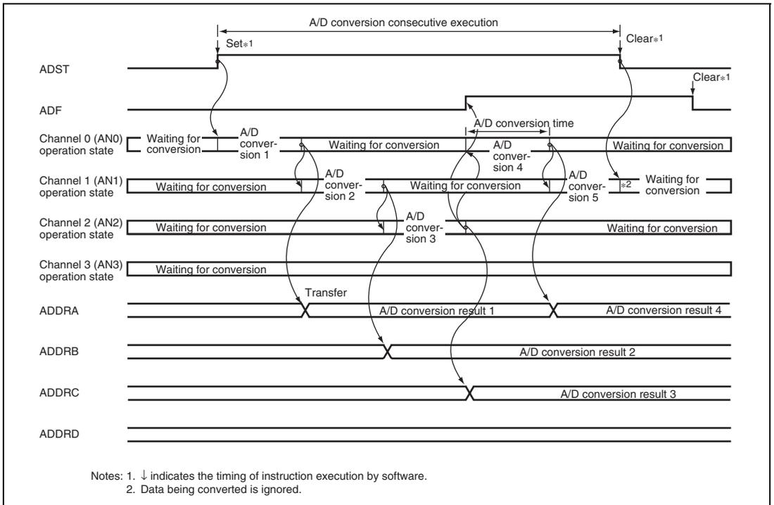
**Figure 19.5 Example of A/D Conversion
