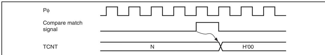
**Figure 15.11 Timing of Counter Clear by Compare Match**
