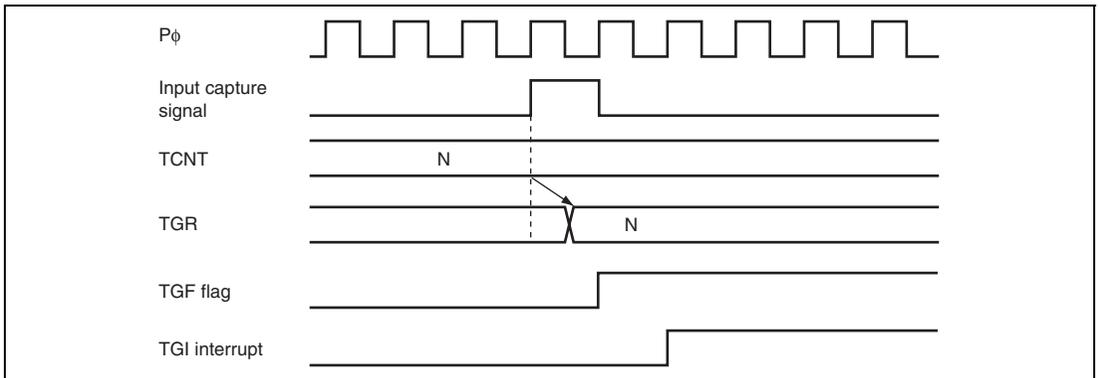
**Figure 13.40 TGI Interrupt Timing (Input Capture)**
