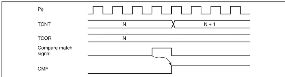
**Figure 15.9 Timing of CMF Setting at Compare Match**
