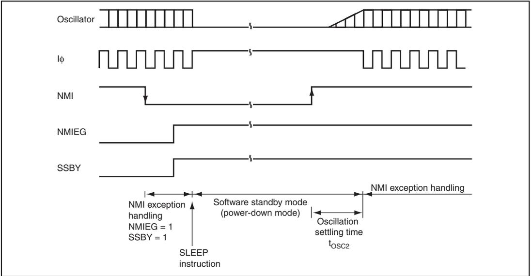
**Figure 27.3 Oscillation Settling Timing after Software Standby Mode**
