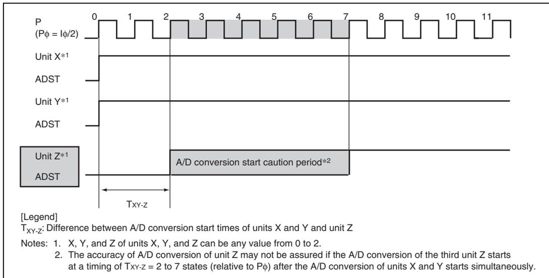
**Figure 19.14 When A/D Conversion Accuracy of Unit Z whose A/D Conversion Starts Third is not Assured: Case 1**
