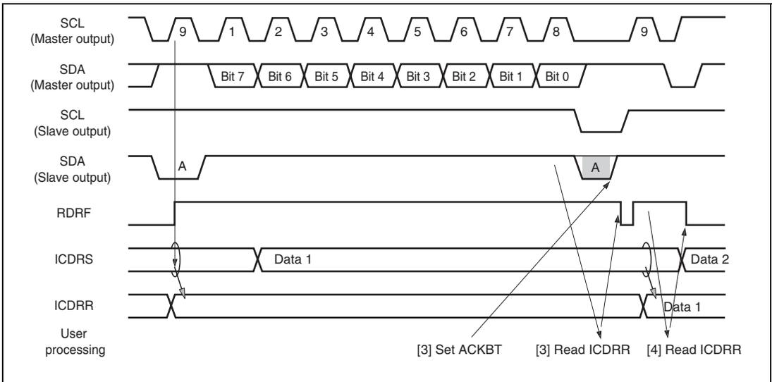
**Figure 18.12 Slave Receive Mode Operation Timing 2**
