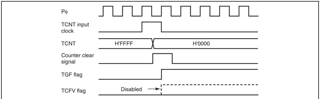
**Figure 13.54 Conflict between Overflow and Counter Clearing**
