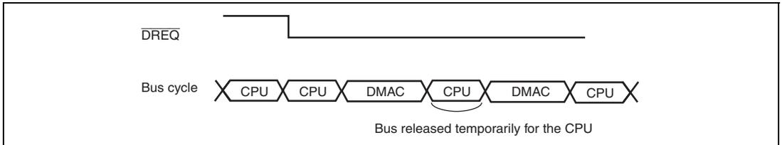
**Figure 10.13 Example of Timing in Cycle Stealing Mode**
