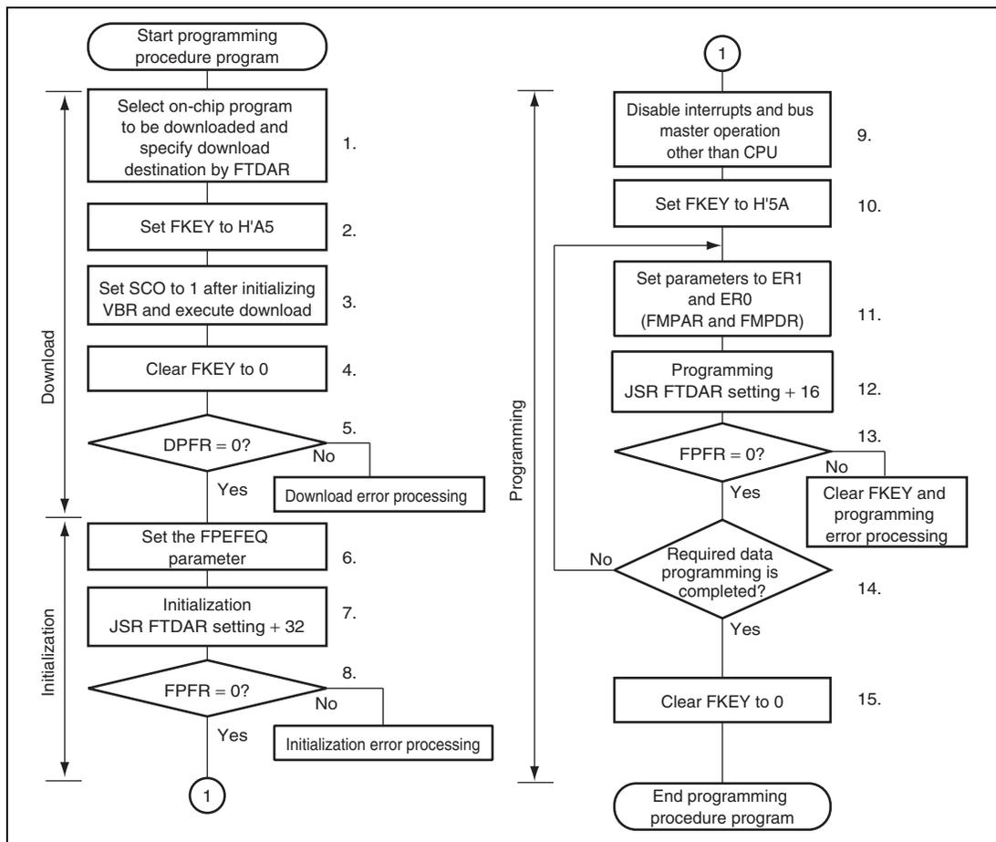
**Figure 22.11 Programming Procedure in User Program Mode**
