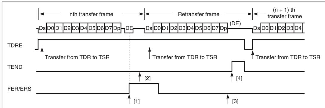
**Figure 17.29 Data Re-Transfer Operation in SCI Transmission Mode**
