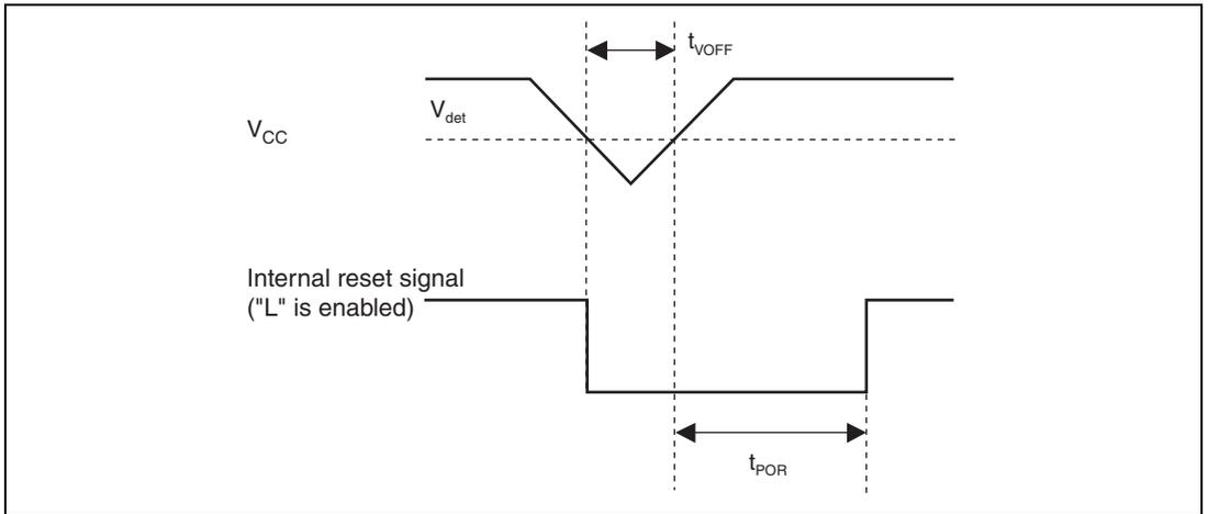
**Figure 27.41 Voltage Detection Circuit Timing**
