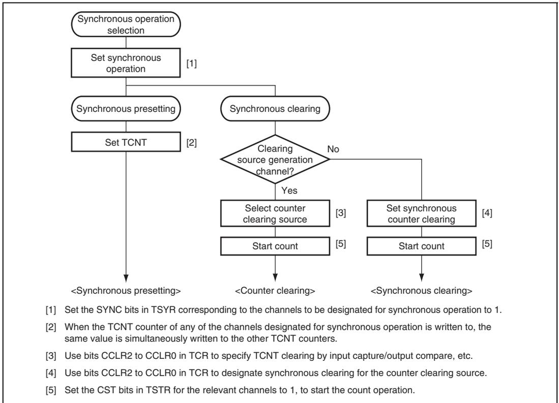
**Figure 13.11 Example of Synchronous Operation Setting Procedure**
