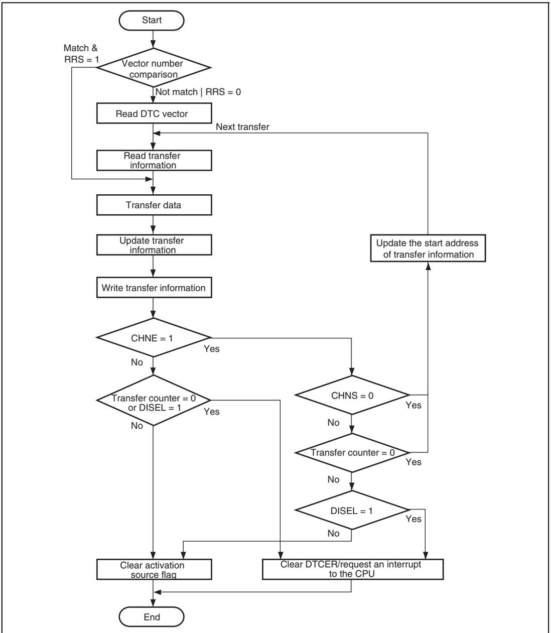
Figure 11.4 Flowchart of DTC Operation
