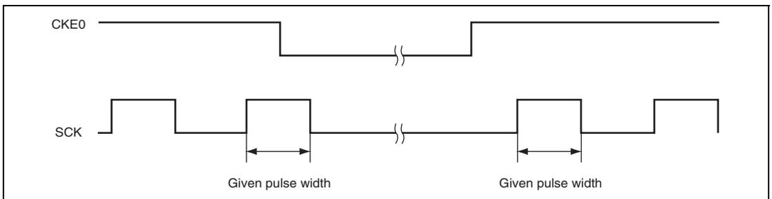
**Figure 17.34 Clock Output Fixing Timing**
