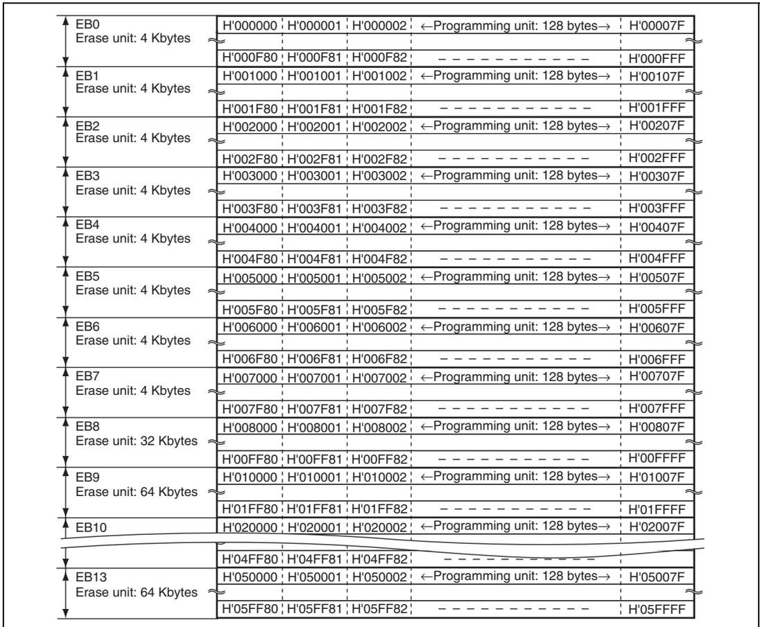
Figure 22.4 (2) User MAT Block Structure of H8SX/1643
