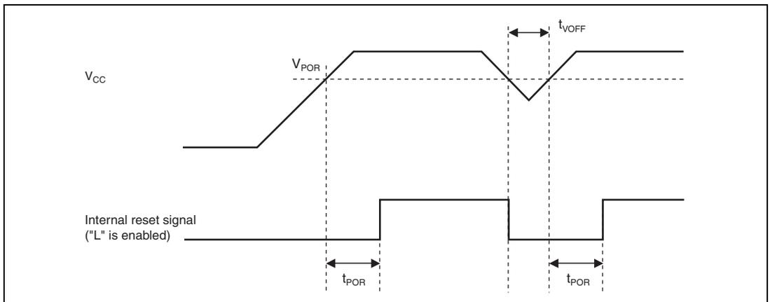
**Figure 27.40 Power-On Reset Timing**
