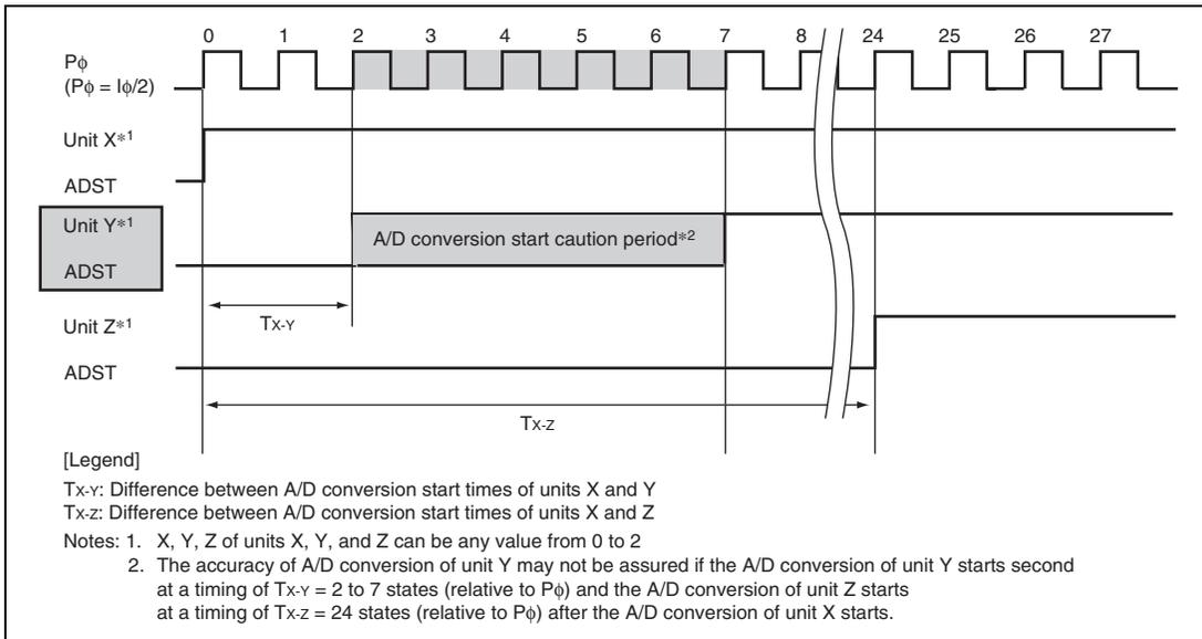
**Figure 19.18 When A/D Conversion Accuracy of Unit Y whose A/D Conversion Starts Second is not Assured: Case 1**
