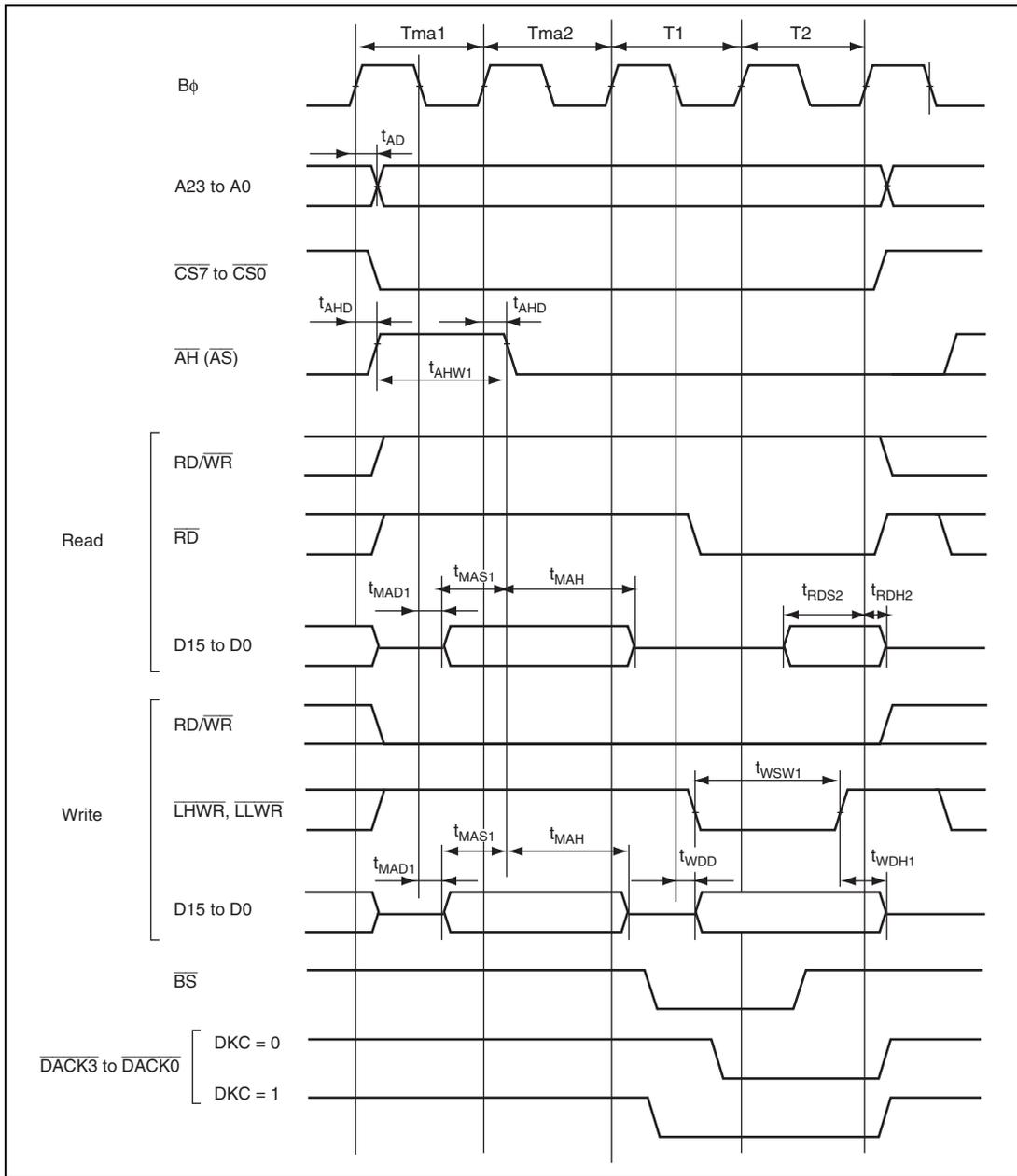
**Figure 27.17 Address/Data Multiplexed Access Timing (No Wait)
