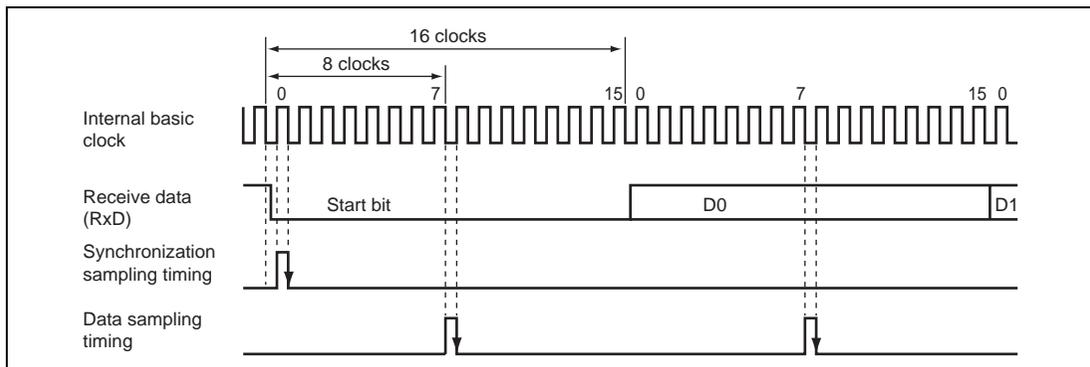
**Figure 17.6 Receive Data Sampling Timing in Asynchronous Mode**
