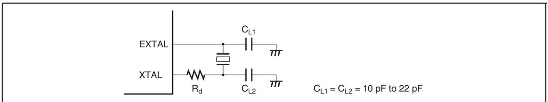
**Figure 24.2 Connection of Crystal Resonator (Example)**
