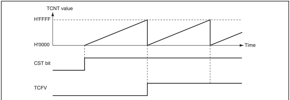
**Figure 13.4 Free-Running Counter Operation**
