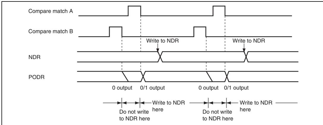
**Figure 14.9 Non-Overlapping Operation and NDR Write Timing**
