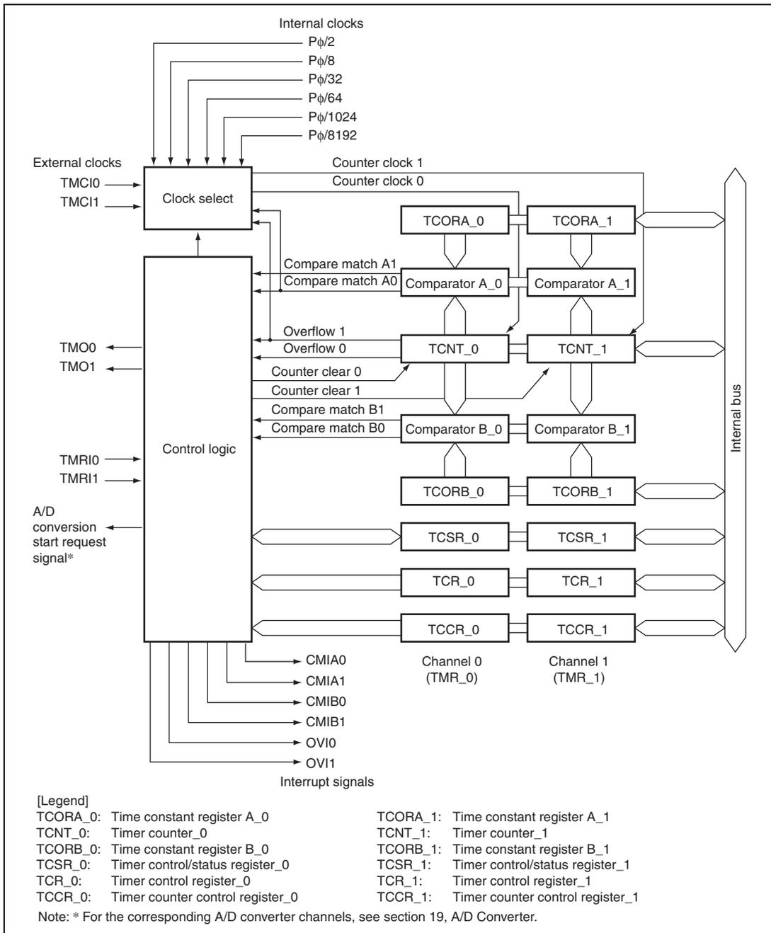
**Figure 15.1 Block Diagram of 8-Bit Timer Module (Unit 0)**
