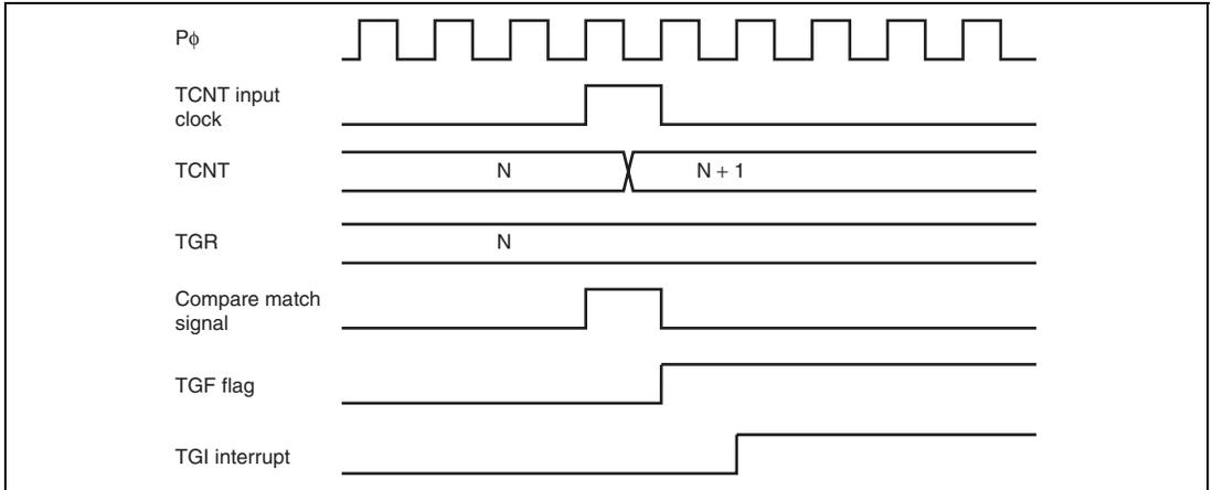
**Figure 13.39 TGI Interrupt Timing (Compare Match)**
