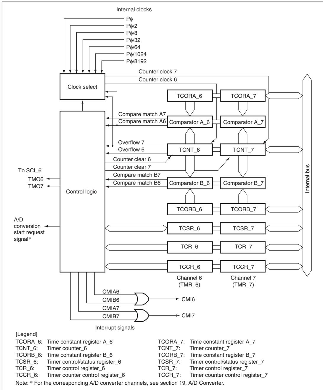
**Figure 15.4 Block Diagram of 8-Bit Timer Module (Unit 3)**
