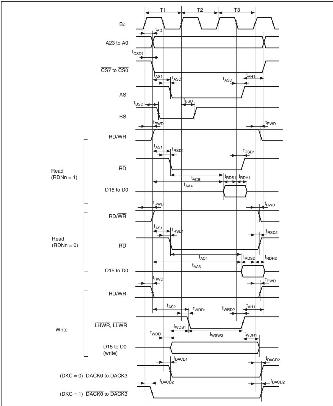
Figure 27.9 Basic Bus Timing: Three-State Access
