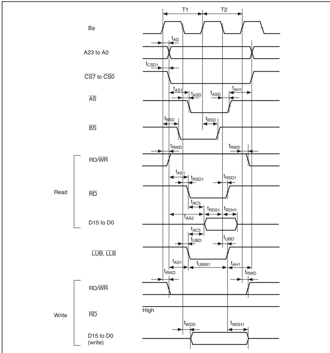
Figure 27.13 Byte Control SRAM: Two-State Read/Write Access
