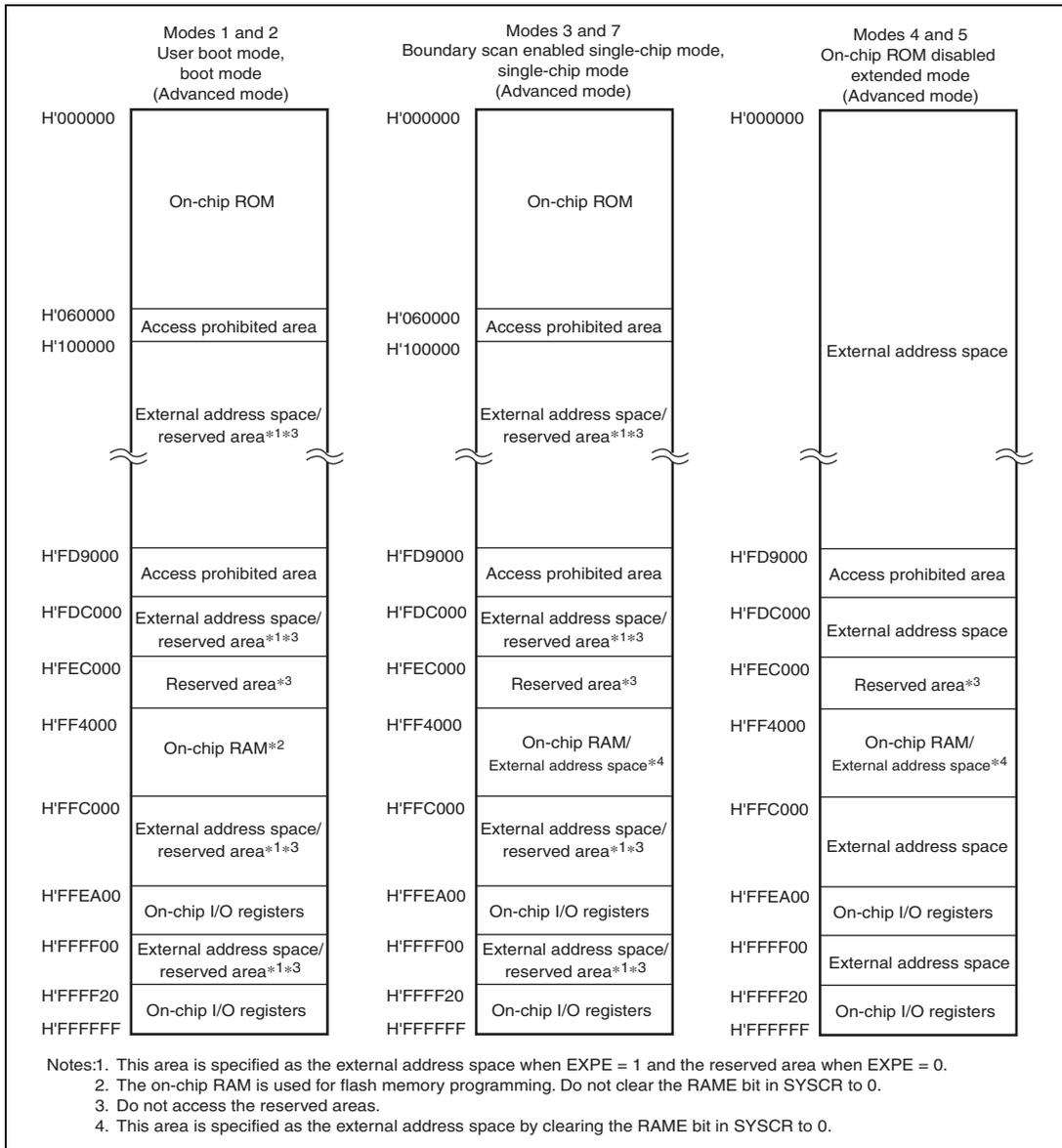
**Figure 3.2 Address Map in Each Operating Mode of H8SX/1643 and H8SX/1643L (1)**
