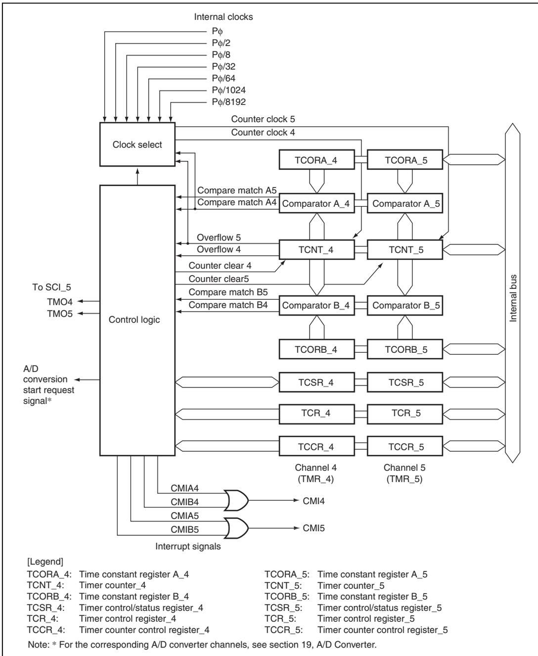
**Figure 15.3 Block Diagram of 8-Bit Timer Module (Unit 2)**
