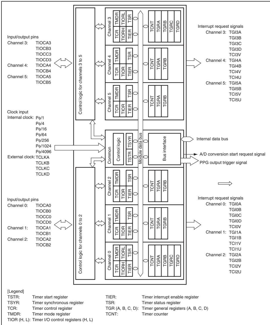
**Figure 13.1 Block Diagram of TPU (Unit 0)**
