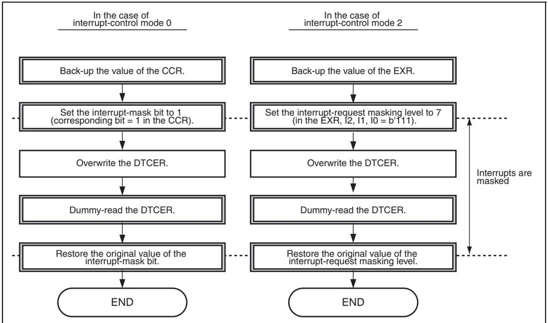
**Figure 11.17 Example of Procedures for Overwriting the DTCER**
