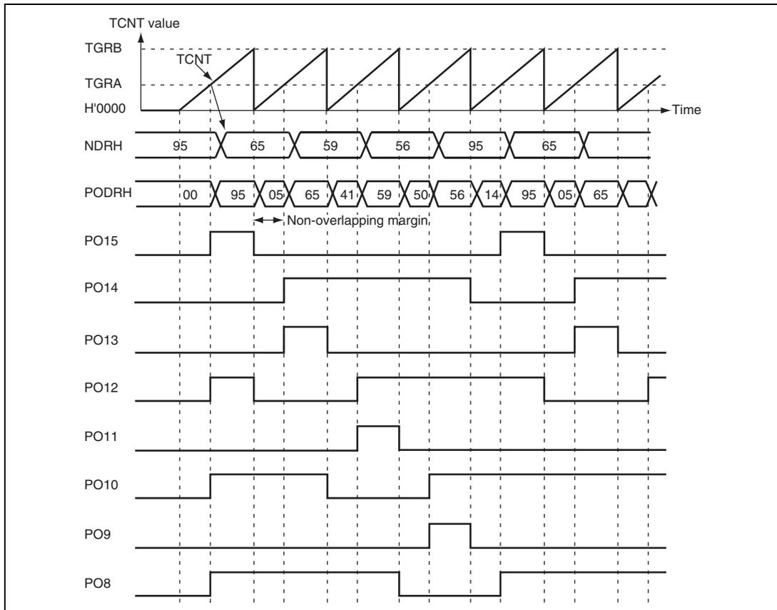
**Figure 14.12 Non-Overlapping Pulse Output Example (4-Phase Complementary)**
