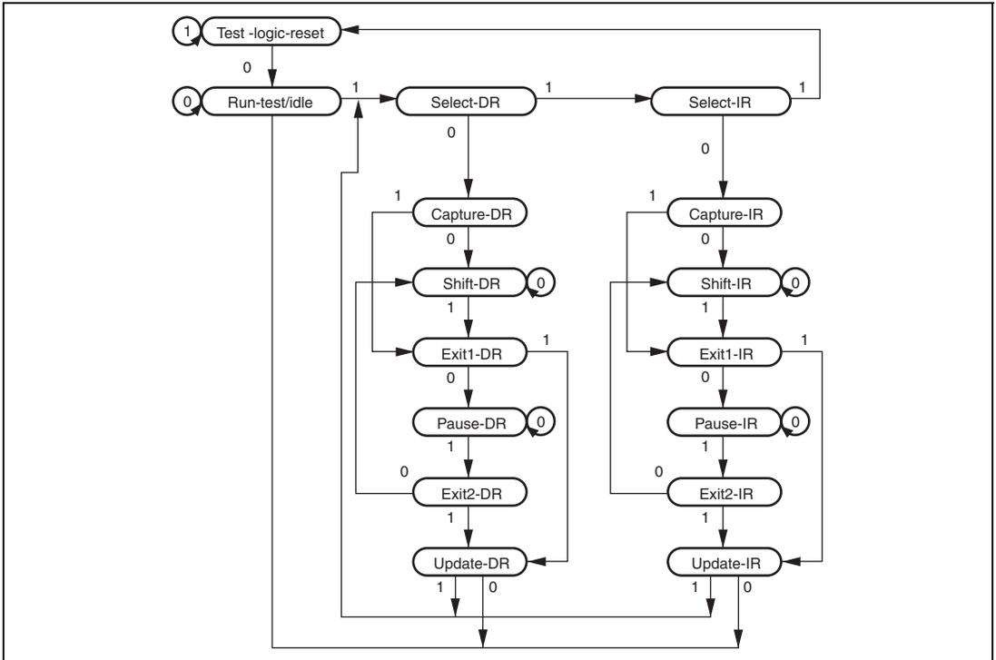
**Figure 23.2 State Transitions of the TAP Controller**
