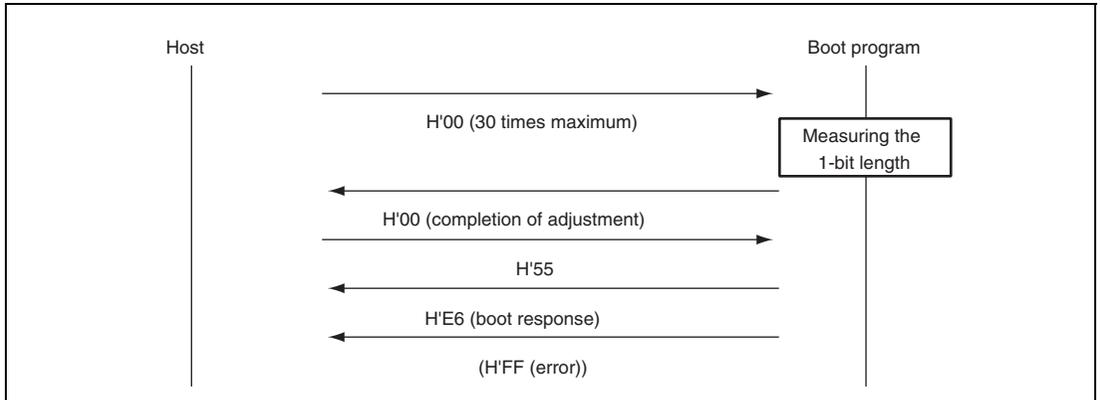
**Figure 22.22 Bit-Rate-Adjustment Sequence**
