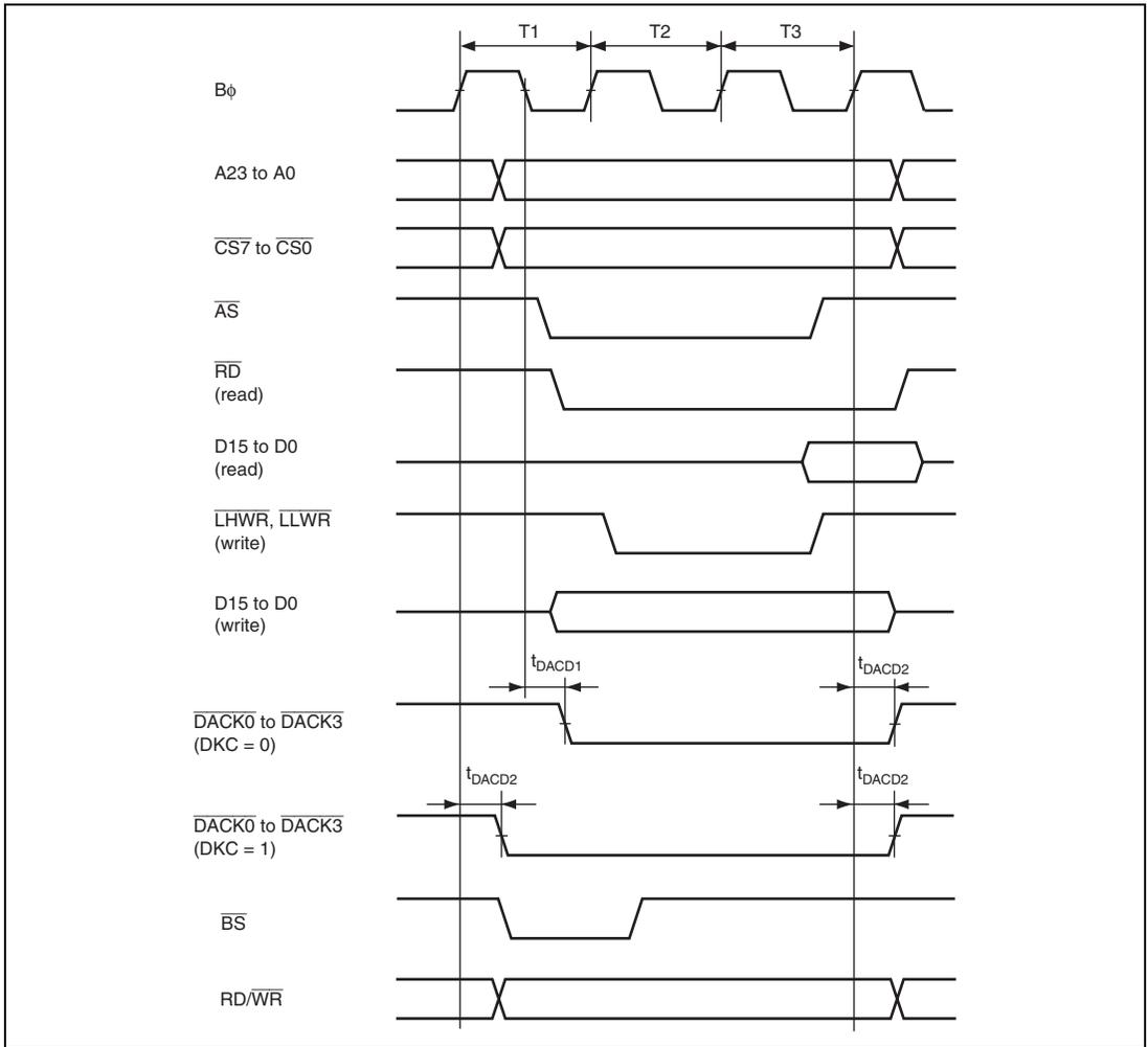
**Figure 27.24 Single Address Transfer Timing for the DMAC (Three-State Access)**
