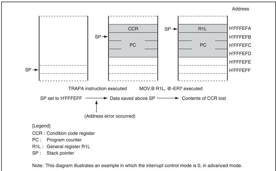
**Figure 6.4 Operation when SP Value is Odd**
