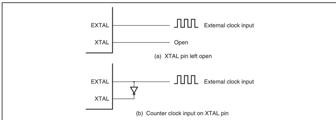
**Figure 24.4 External Clock Input (Examples)**
