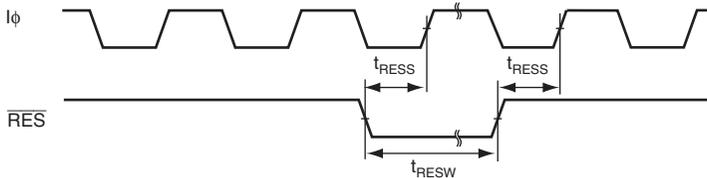
**Figure 27.6 Reset Input Timing**
