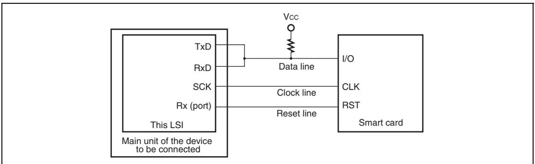
**Figure 17.24 Pin Connection for Smart Card Interface**
