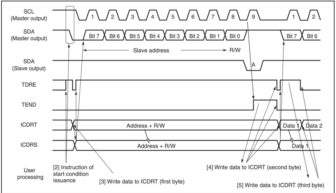
**Figure 18.5 Master Transmit Mode Operation Timing 1**
