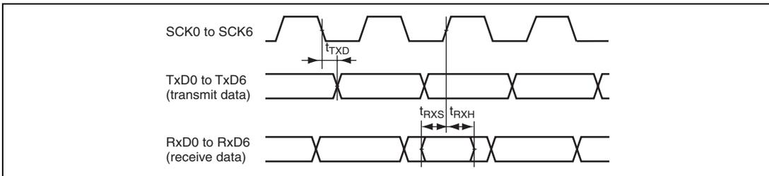
**Figure 27.34 SCI Input/Output Timing: Clocked Synchronous Mode**
