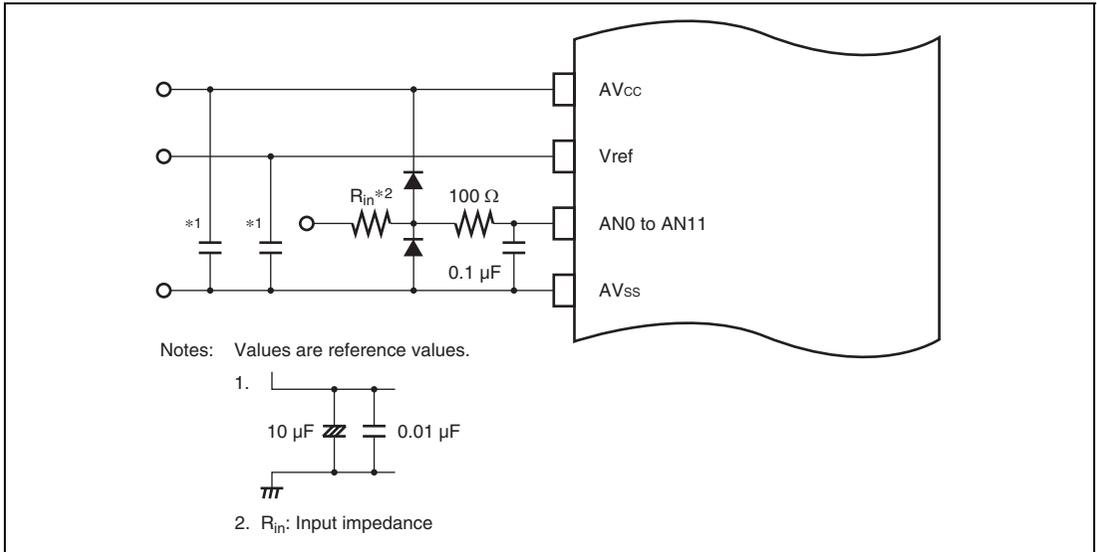
**Figure 19.22 Example of Analog Input Protection Circuit**
