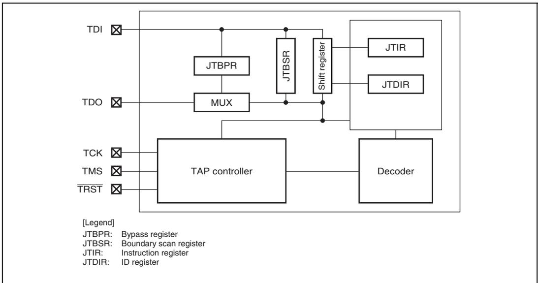
**Figure 23.1 Block Diagram of Boundary Scan Function**
