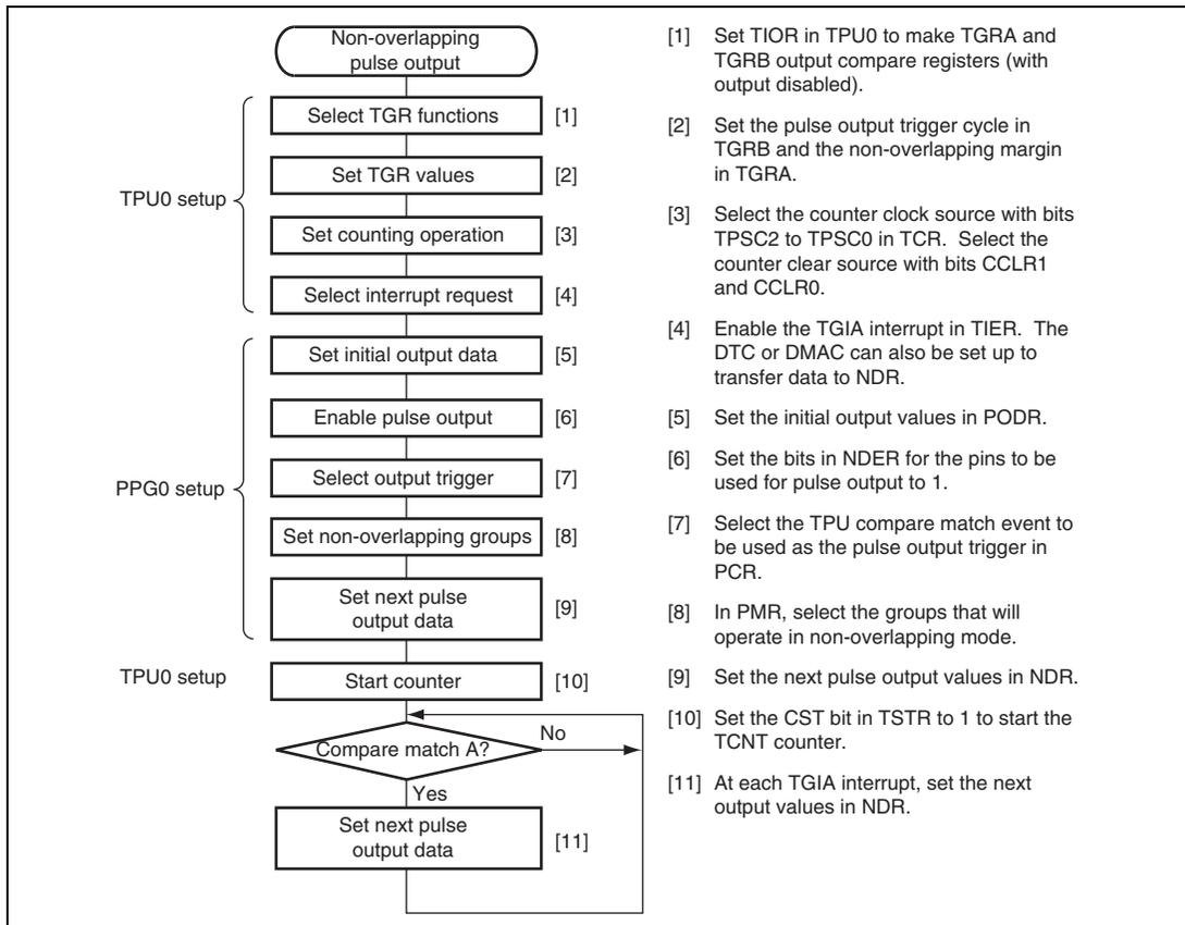
**Figure 14.10 Setup Procedure for Non-Overlapping Pulse Output (PPG0)**
