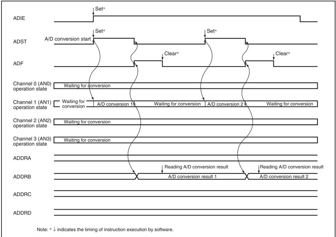
**Figure 19.4 Example of A/D Converter Operation (Single Mode, Channel 1 Selected)**
