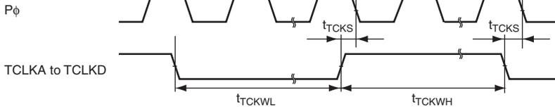
**Figure 27.27 TPU Clock Input Timing**
