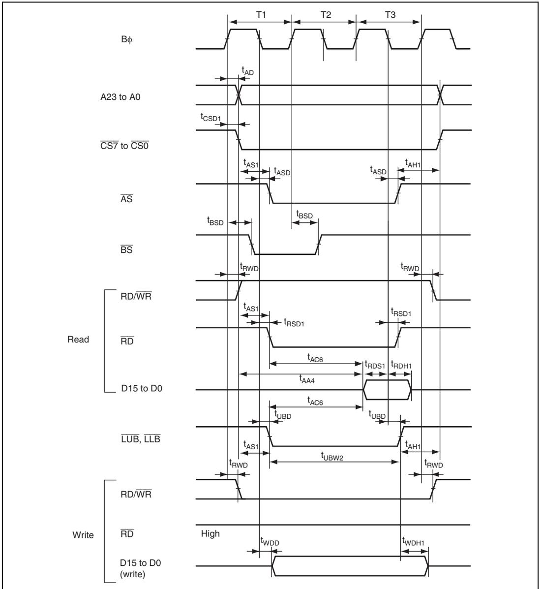
Figure 27.14 Byte Control SRAM: Three-State Read/Write Access
