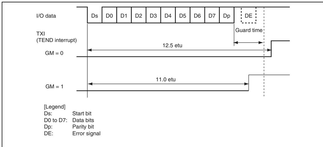
**Figure 17.30 TEND Flag Set Timing during Transmission**
