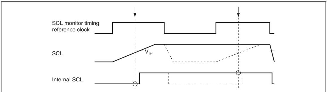
**Figure 18.18 Timing of the Bit Synchronous Circuit**
