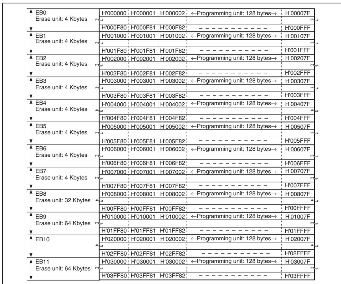
Figure 22.4 (1) User MAT Block Structure of H8SX/1641
