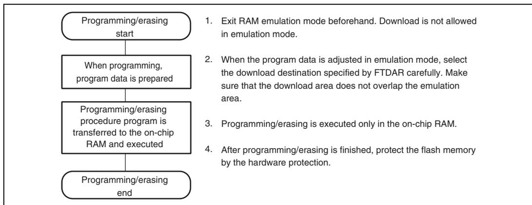
**Figure 22.9 Programming/Erasing Flow**
