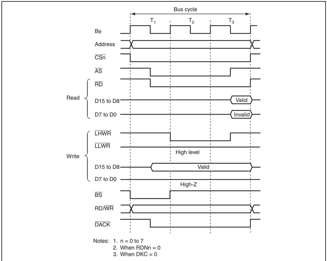
**Figure 9.17 16-Bit 3-State Access Space Bus Timing (Byte Access for Even Address)**
