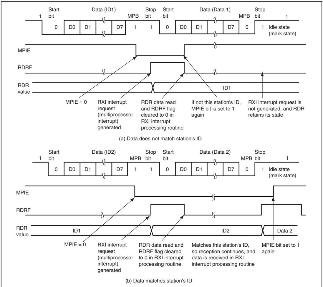
**Figure 17.15 Example of SCI Operation for Reception
