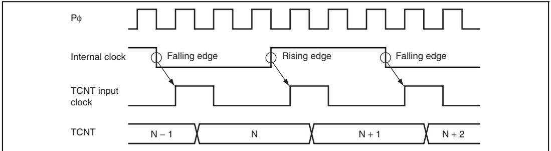
**Figure 13.31 Count Timing in Internal Clock Operation**
