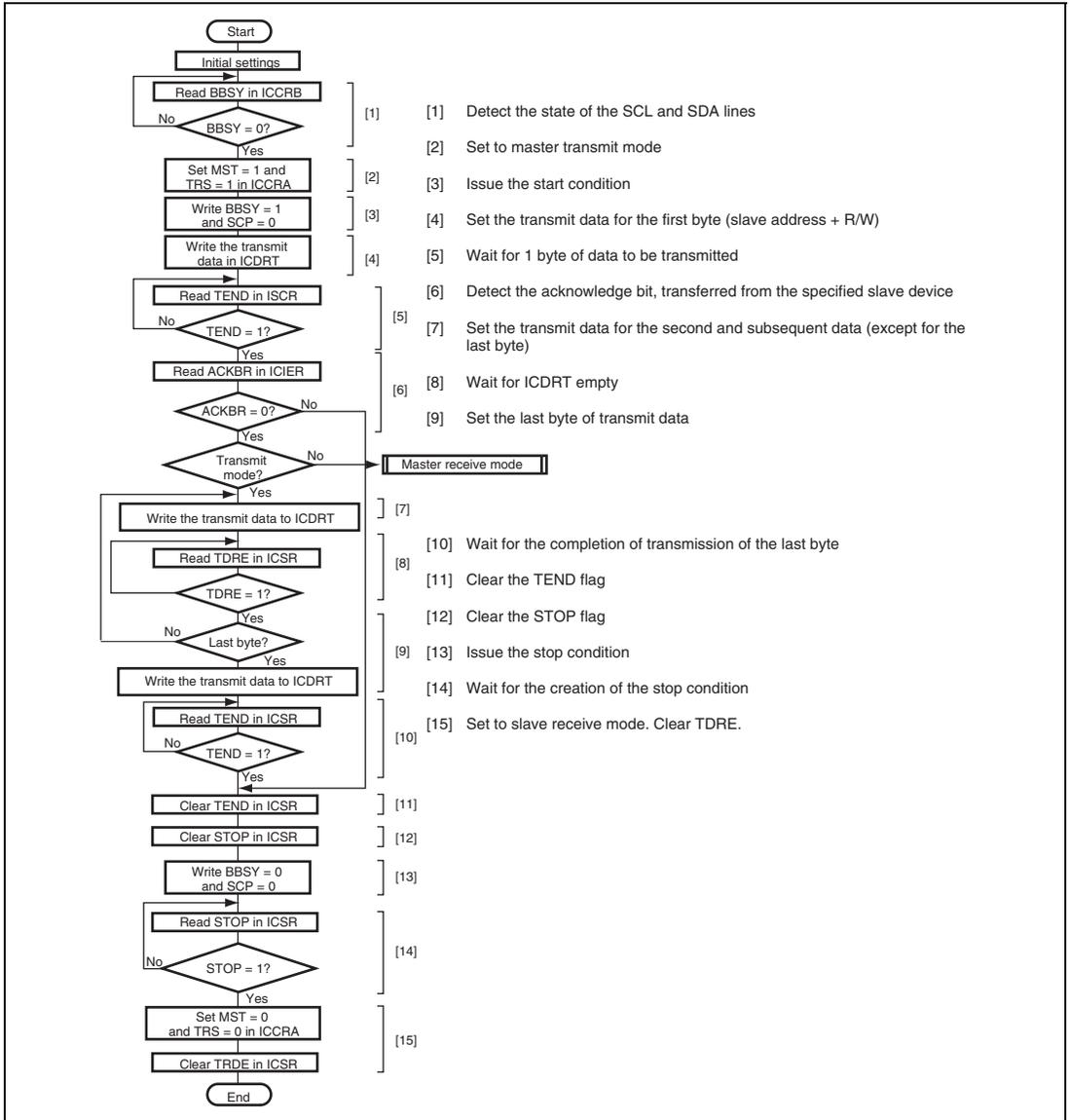
**Figure 18.14 Sample Flowchart of Master Transmit Mode**
