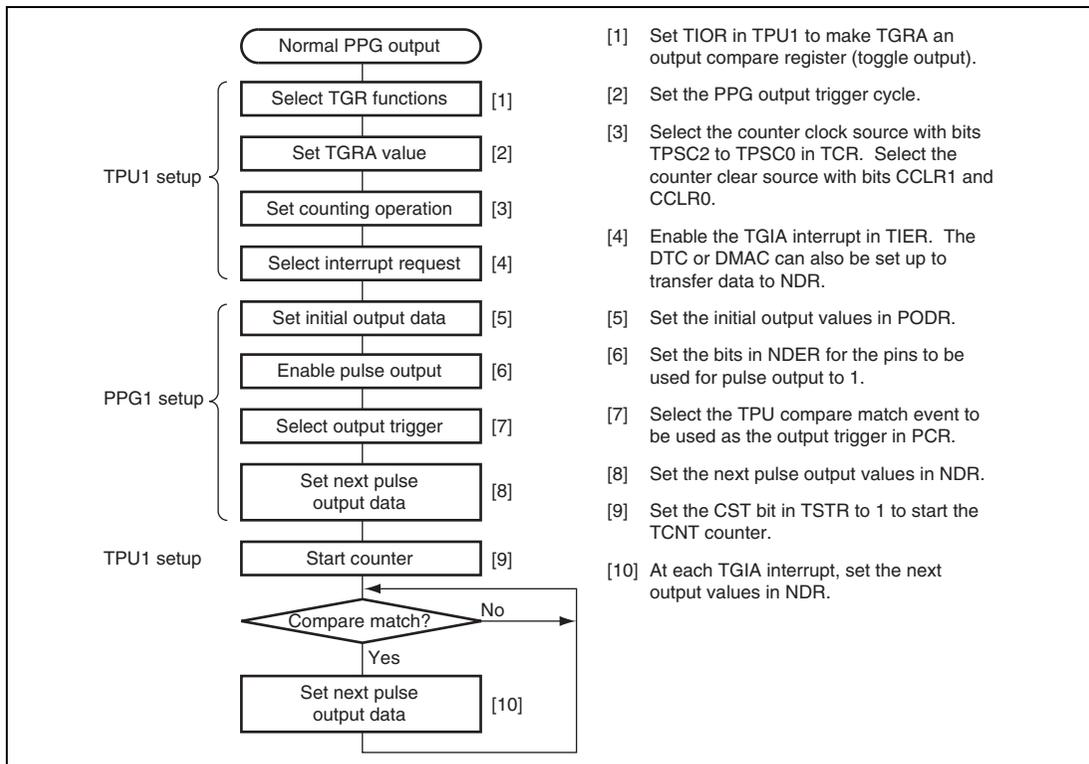
**Figure 14.6 Setup Procedure for Normal Pulse Output (PPG1)**
