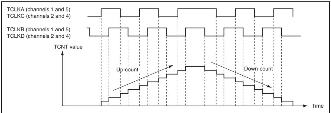
**Figure 13.26 Example of Phase Counting Mode 1 Operation**
