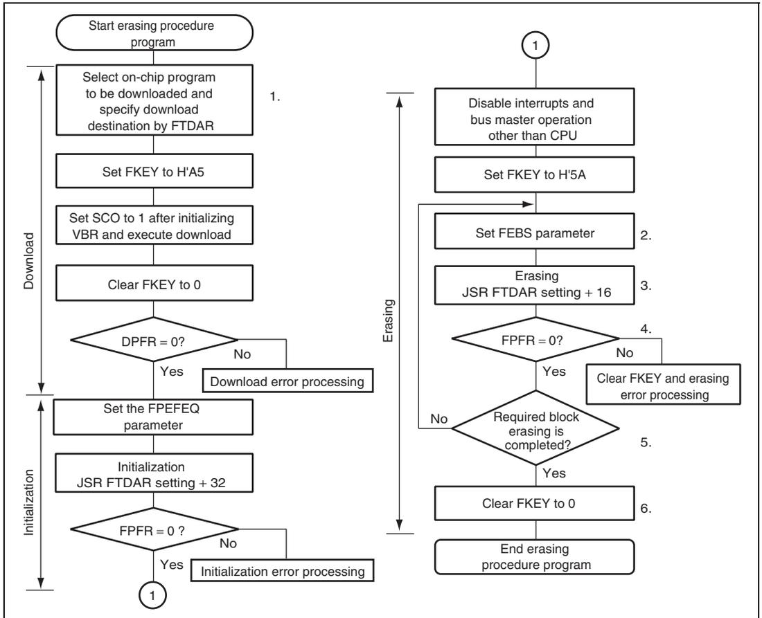
Figure 22.12 Erasing Procedure in User Program Mode
