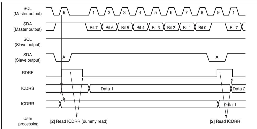
**Figure 18.11 Slave Receive Mode Operation Timing 1**
