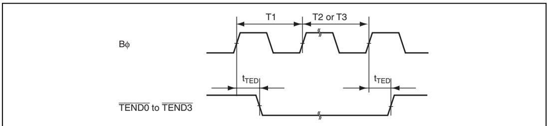
**Figure 27.22 Timing of  $\overline{TEND}$  Output (for the DMAC)**
