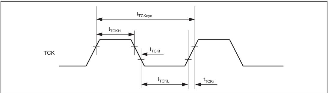
**Figure 27.37 Boundary Scan TCK Timing**
