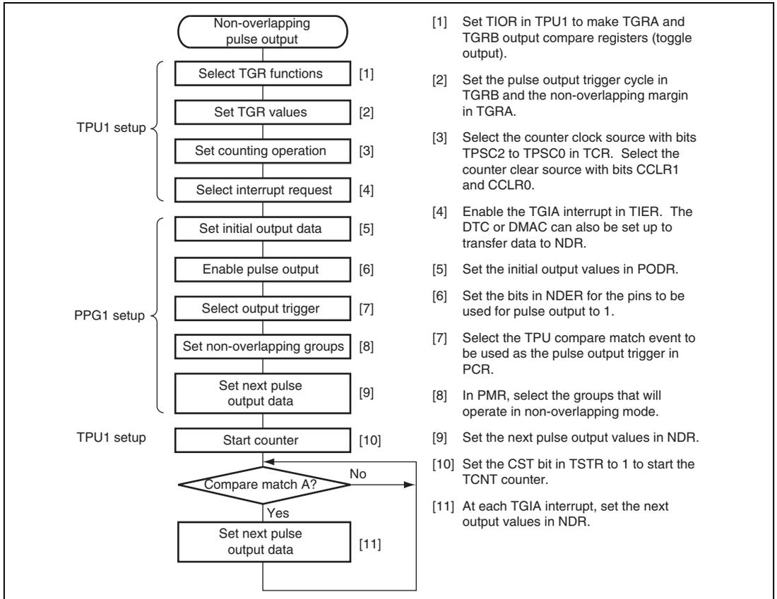
**Figure 14.11 Setup Procedure for Non-Overlapping Pulse Output (PPG1)**
