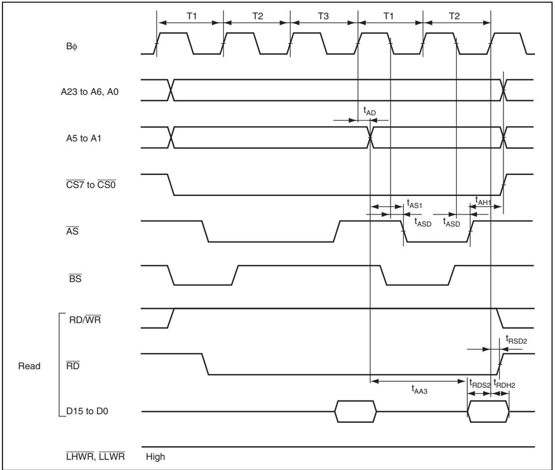
**Figure 27.16 Burst ROM Access Timing: Two-State Burst Access**
