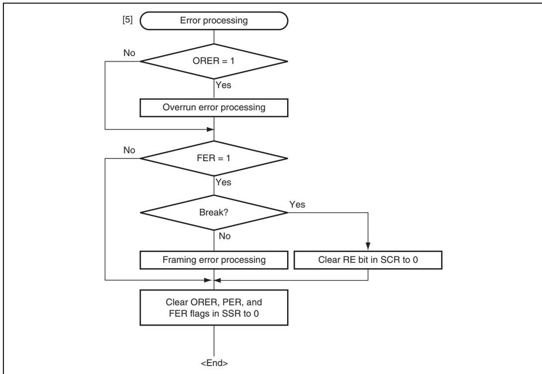
**Figure 17.16 Sample Multiprocessor Serial Reception Flowchart (2)**
