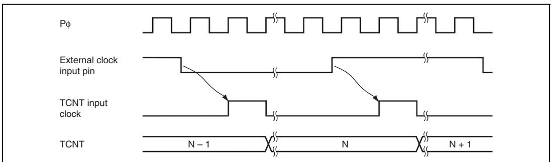
**Figure 15.8** Count Timing for External Clock Input
