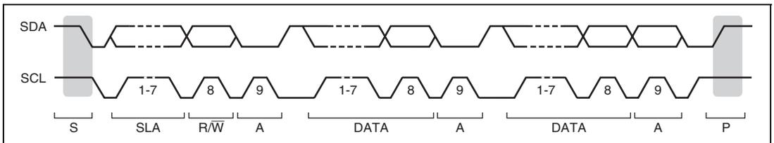
**Figure 18.4 I<sup>2</sup>C Bus Timing**
