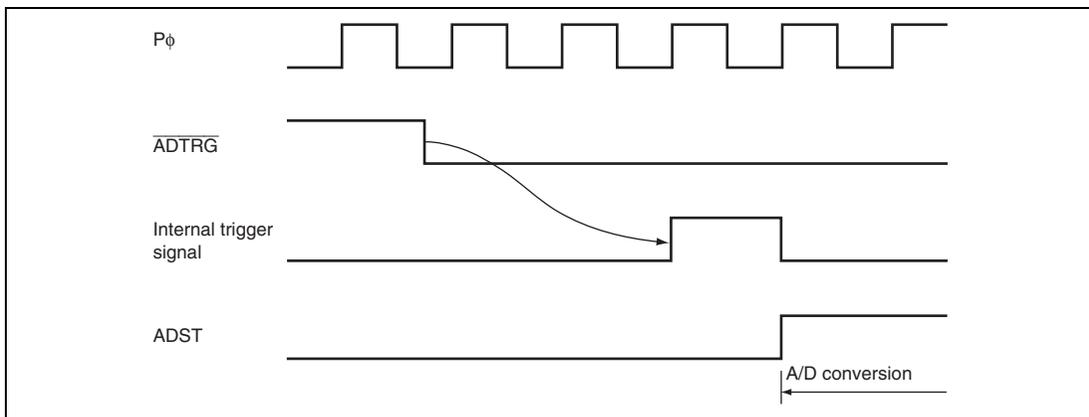
**Figure 19.8 External Trigger Input Timing (TRGS1, TRGS0, and EXTRGS  $\neq$  B'111)**
