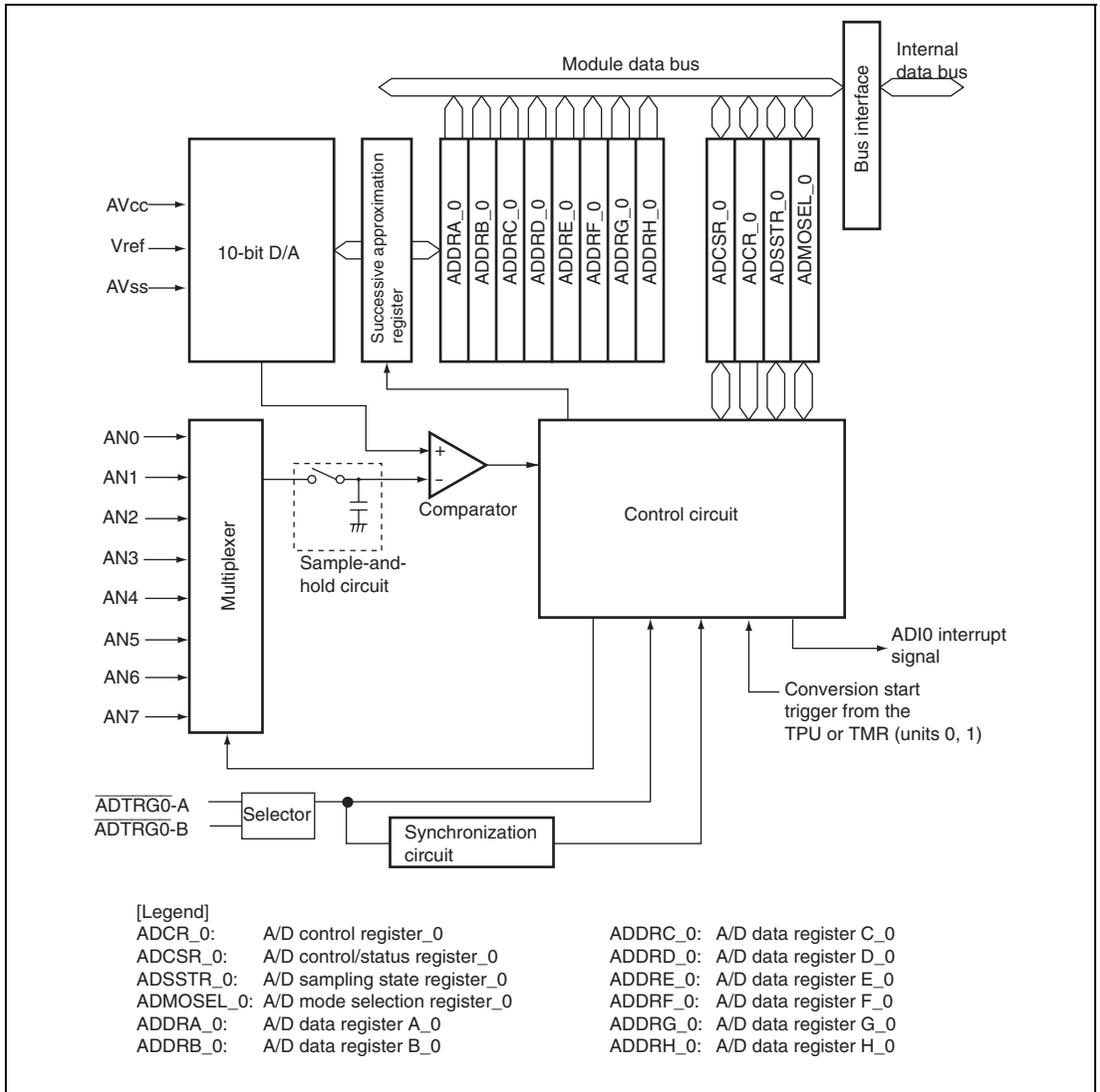
**Figure 19.1 Block Diagram of A/D Converter Unit 0 (AD\_0)**
