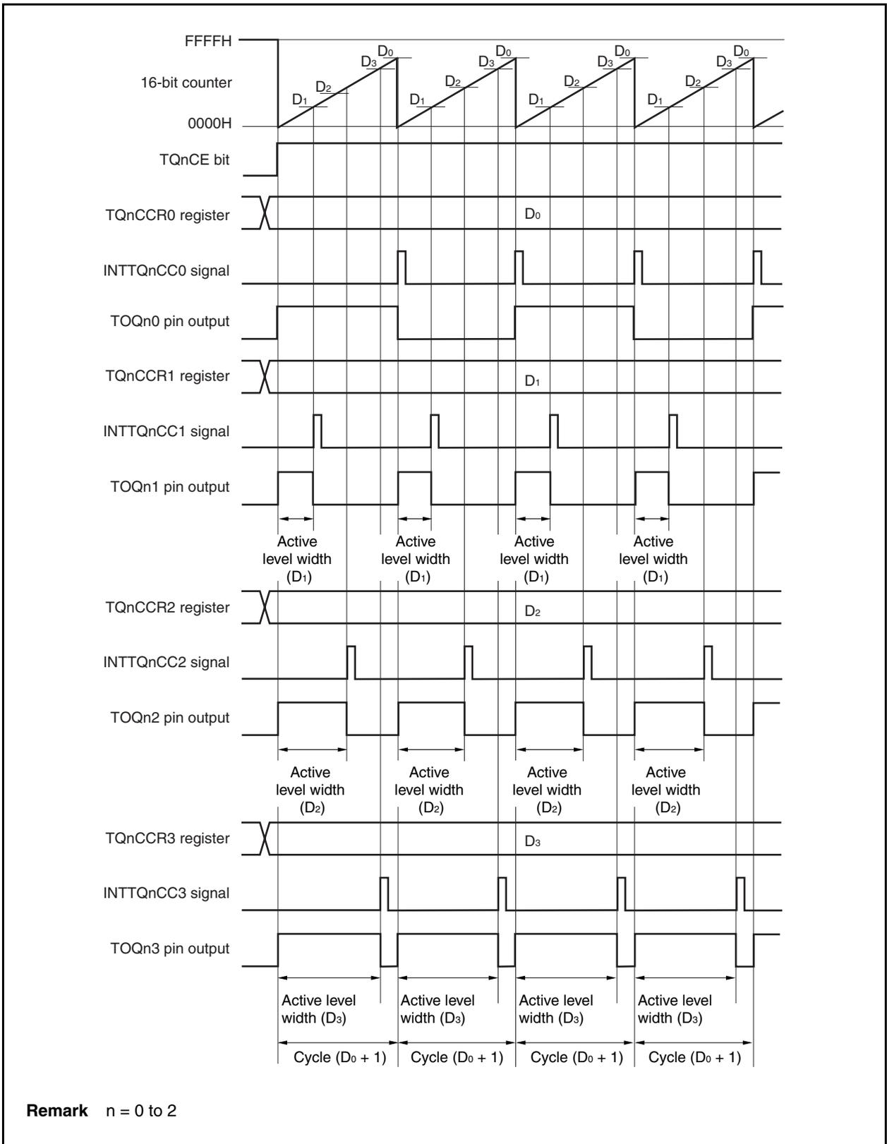
When the TQnCE bit is set to 1, the 16-bit counter is cleared from FFFFH to 0000H, starts counting, and outputs PWM waveform from the TOQnk pin.
