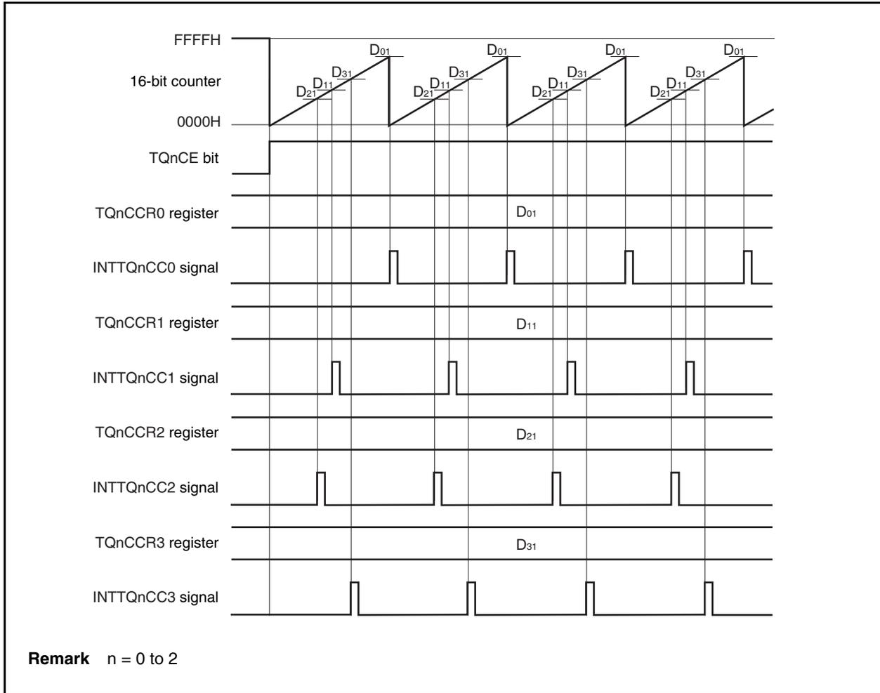
If the set value of the TQnCCRk register is greater than the set value of the TQnCCR0 register, the INTTQnCCk signal is not generated because the count value of the 16-bit counter and the value of the TQnCCRk register do not match.
