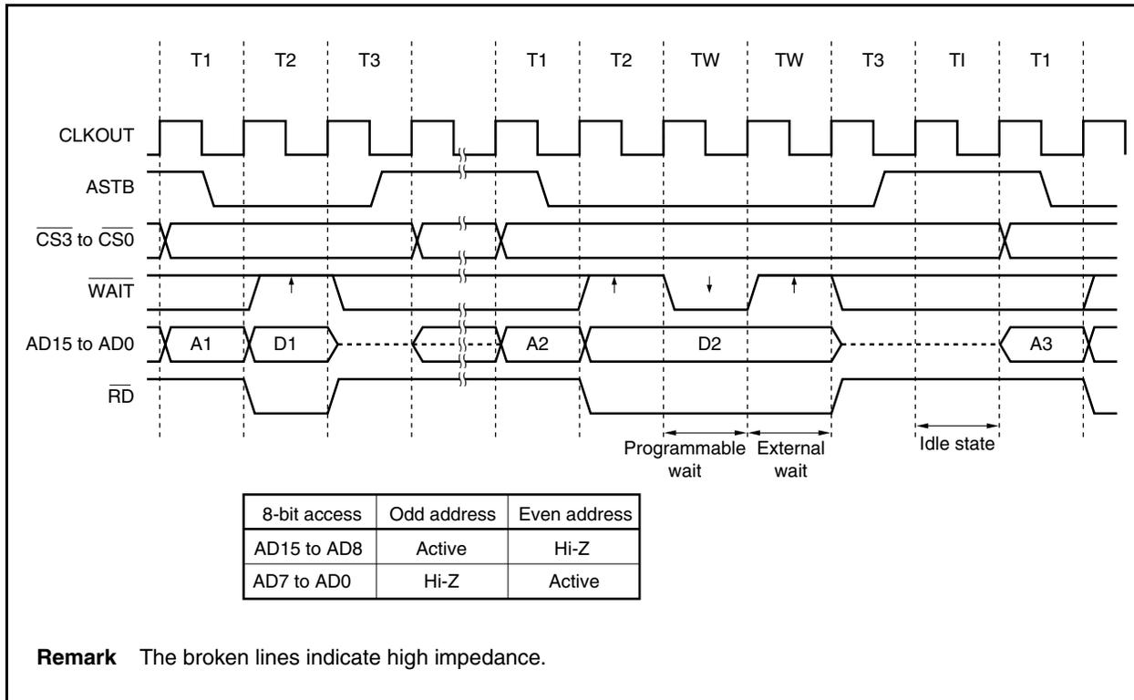
Figure 5-5. Bus Read Timing (Bus Size: 8 Bits)
