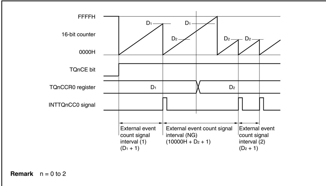
If the value of the TQnCCR0 register is changed from D<sub>1</sub> to D<sub>2</sub> while the count value is greater than D<sub>2</sub> but less than D<sub>1</sub>, the count value is transferred to the CCR0 buffer register as soon as the TQnCCR0 register has been rewritten. Consequently, the value that is compared with the 16-bit counter is D<sub>2</sub>.
