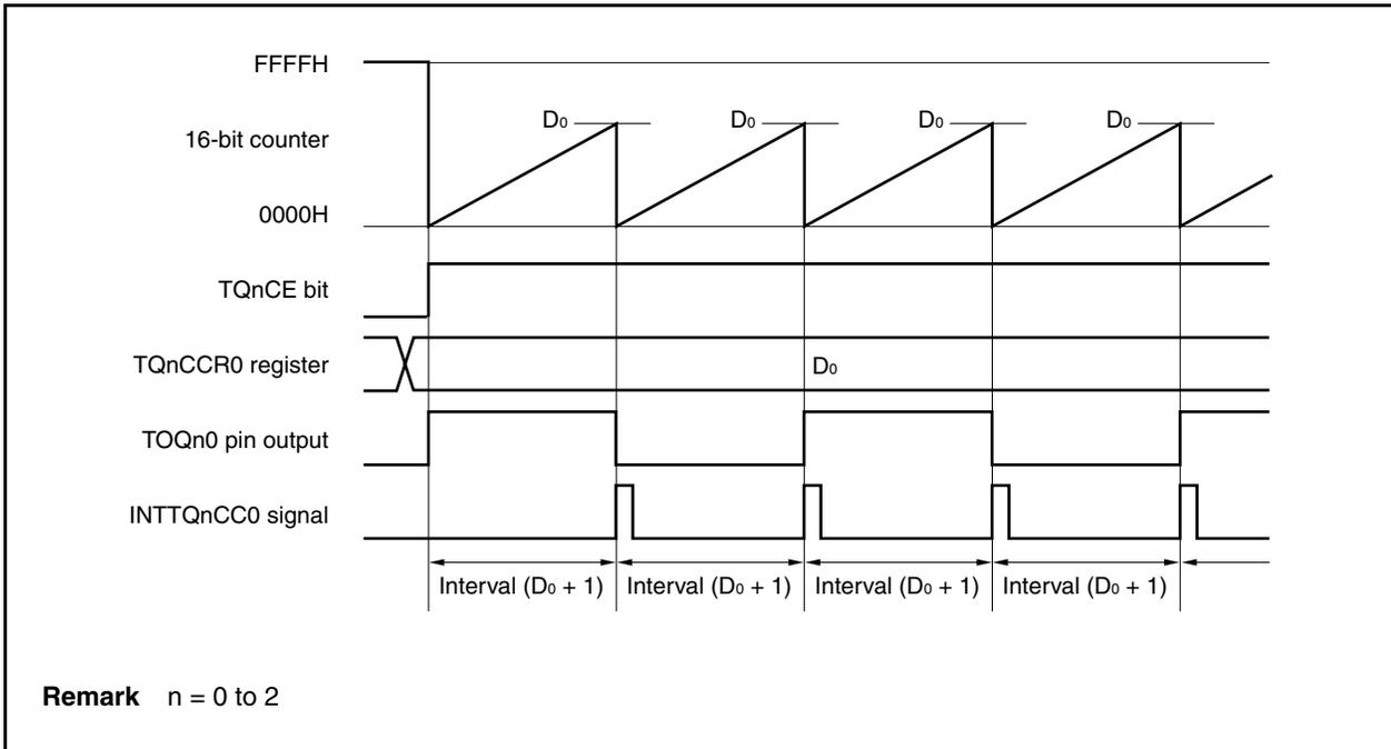
When the TQnCE bit is set to 1, the value of the 16-bit counter is cleared from FFFFH to 0000H in synchronization with the count clock, and the counter starts counting. At this time, the output of the TOQn0 pin is inverted. Additionally, the set value of the TQnCCR0 register is transferred to the CCR0 buffer register.
