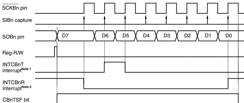
**Notes 1.** The INTCBnT interrupt is set when the data written to the CBnTX register is transferred to the data shift register in the continuous transmission or continuous transmission/reception modes. In the single transmission or single transmission/reception modes, the INTCBnT interrupt request signal is not generated, but the INTCBnR interrupt request signal is generated upon end of communication.
