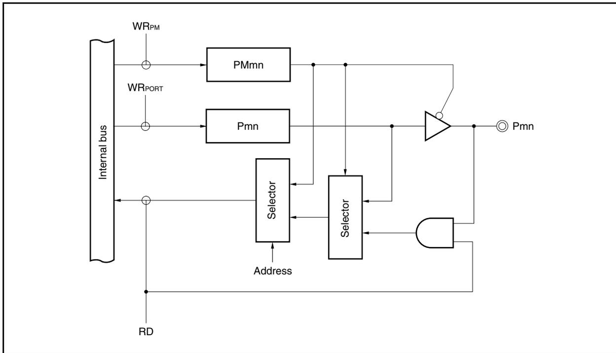
Figure 4-4. Block Diagram of Type C-1
