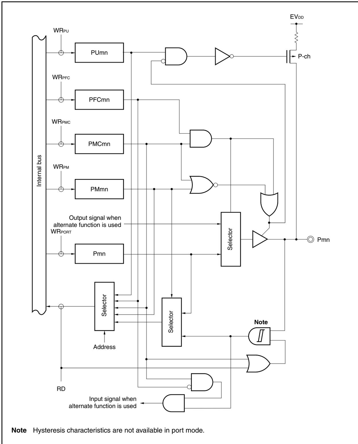
Figure 4-12. Block Diagram of Type G-2
