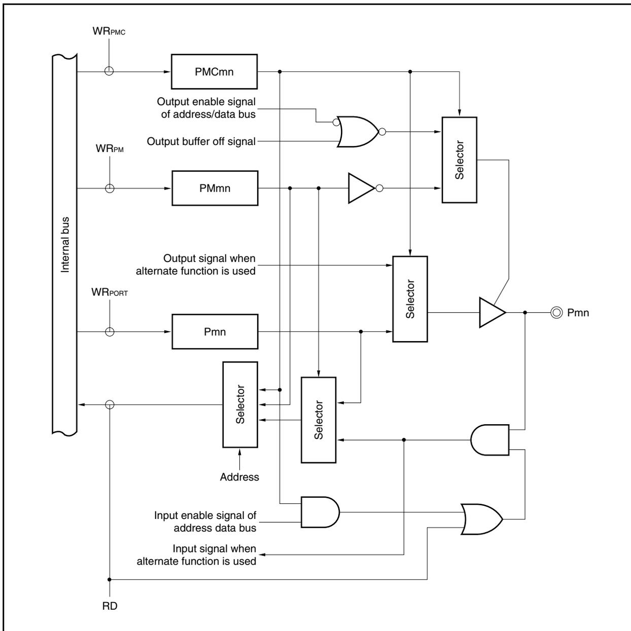
Figure 4-8. Block Diagram of Type E-1
