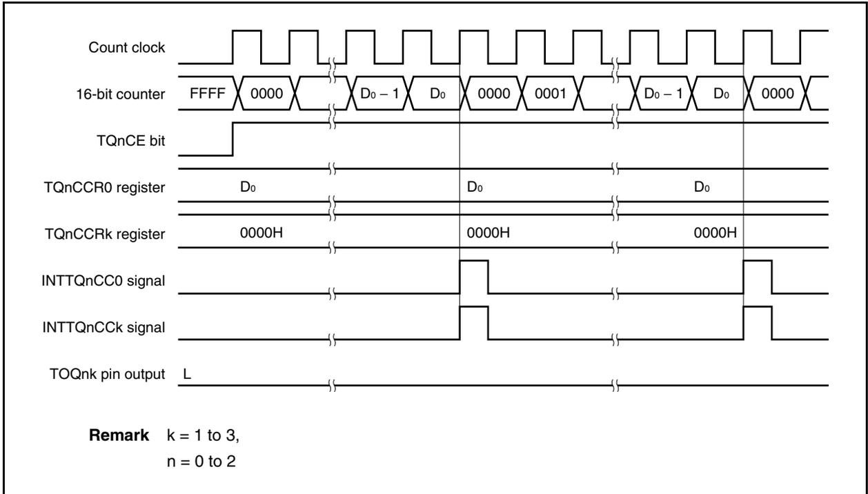
To output a 100% waveform, set a value of (set value of TQnCCR0 register + 1) to the TQnCCRk register. If the set value of the TQnCCR0 register is FFFFH, 100% output cannot be produced.
