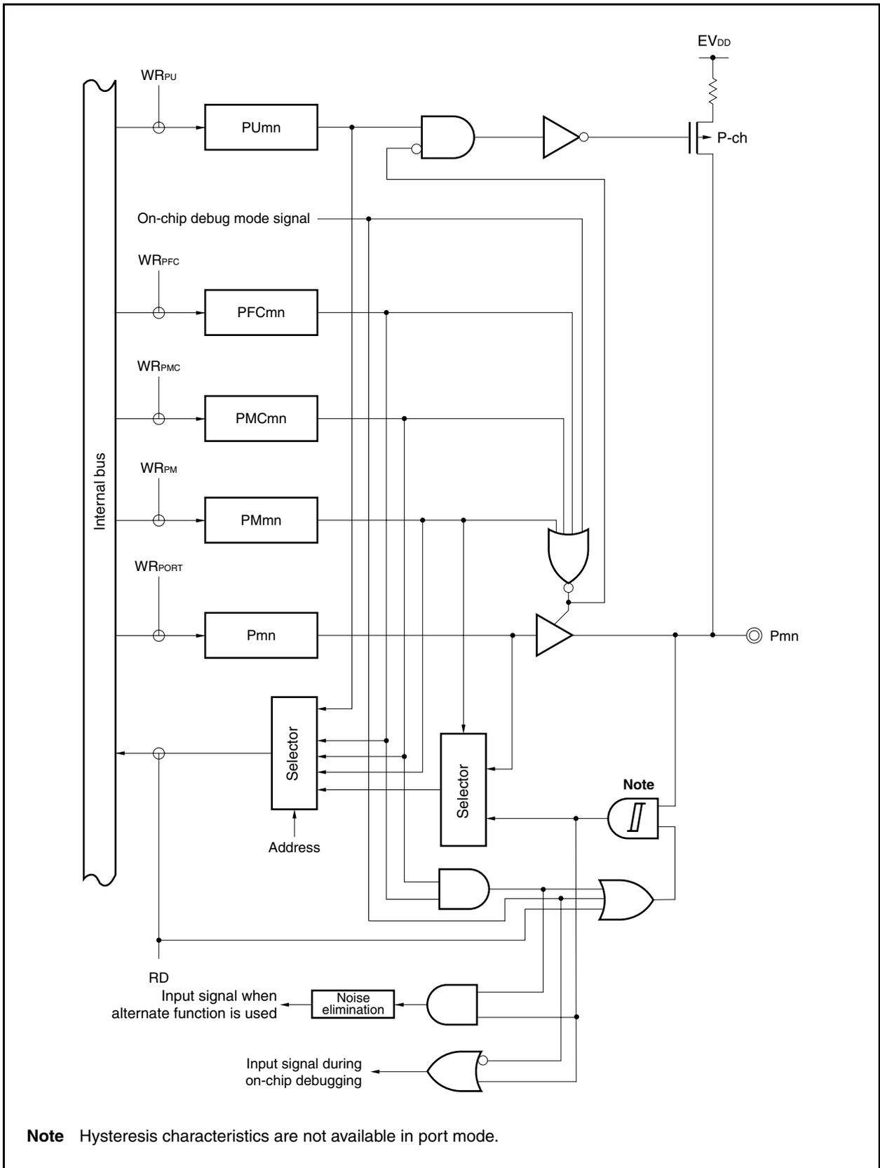
Figure 4-13. Block Diagram of Type G-3
