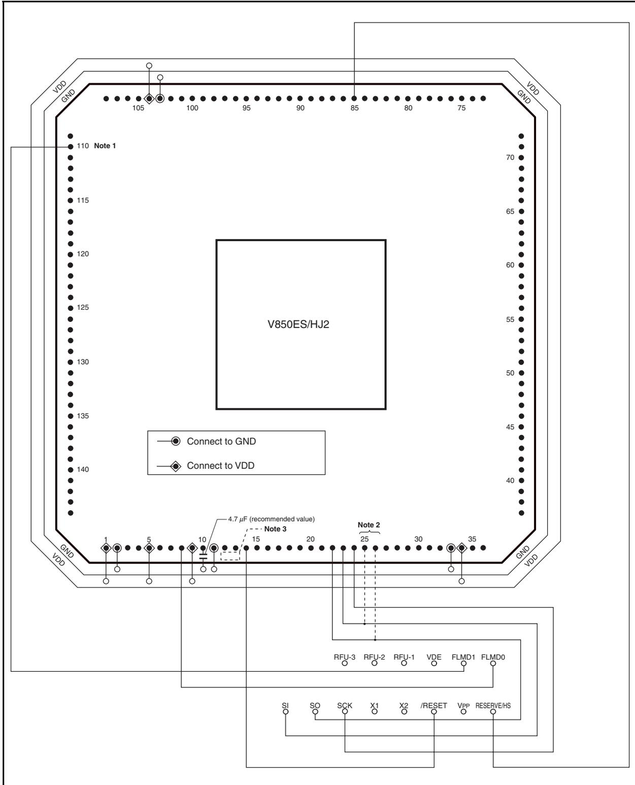
**Figure 24-6. Example of Wiring of V850ES/HJ2 Flash Writing Adapter (FA-144GJ-UEN-A)
