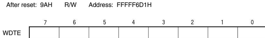
**Cautions** 1. When a value other than “ACH” is written to the WDTE register, an overflow signal is forcibly output.
