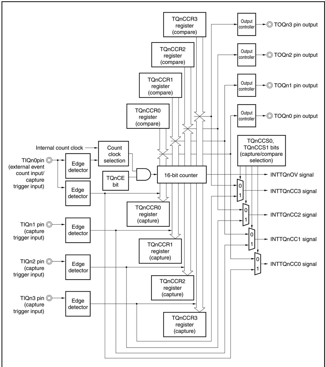
When the TQnCE bit is set to 1, 16-bit timer/event counter Q starts counting, and the output signals of the TOQn0 to TOQn3 pins are inverted. When the count value of the 16-bit counter later matches the set value of the TQnCCRm register, a compare match interrupt request signal (INTTQnCCm) is generated, and the output signal of the TOQnm pin is inverted.
