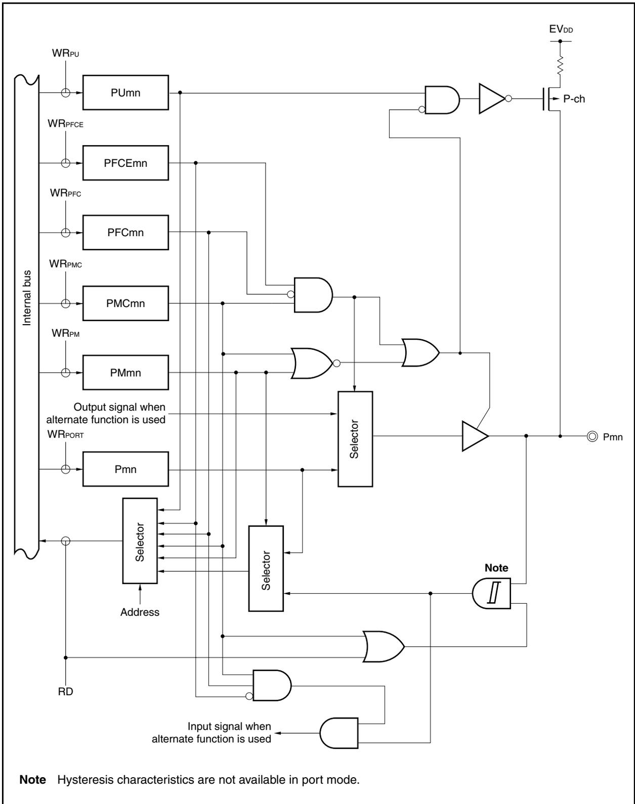
Figure 4-27. Block Diagram of Type U-12
