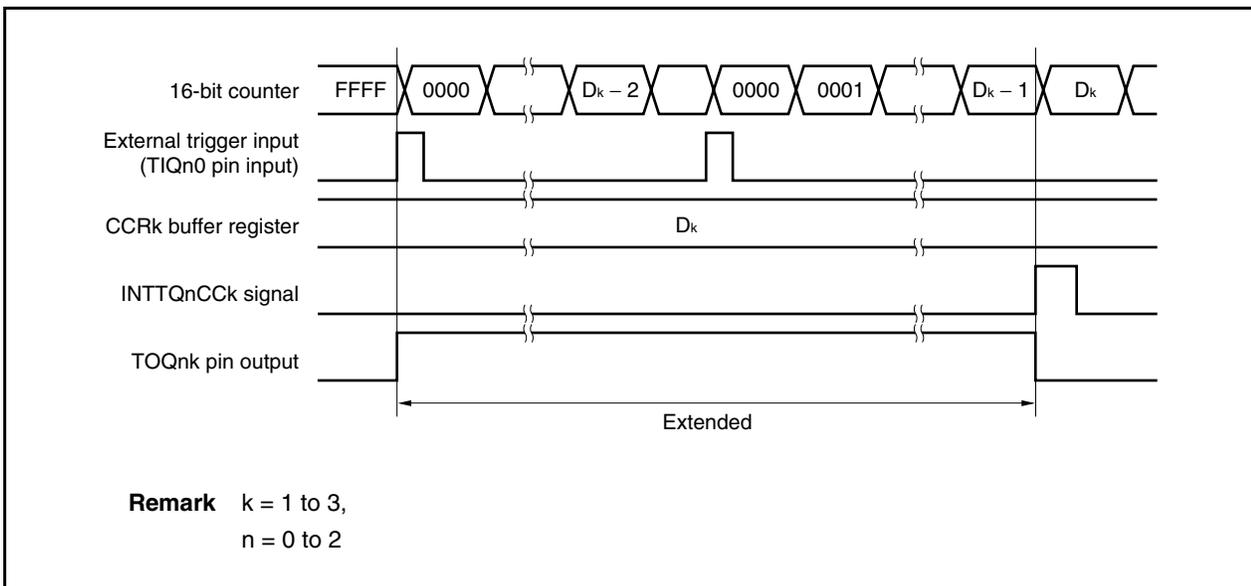
**(d) Conflict between trigger detection and match with CCR0 buffer register**
