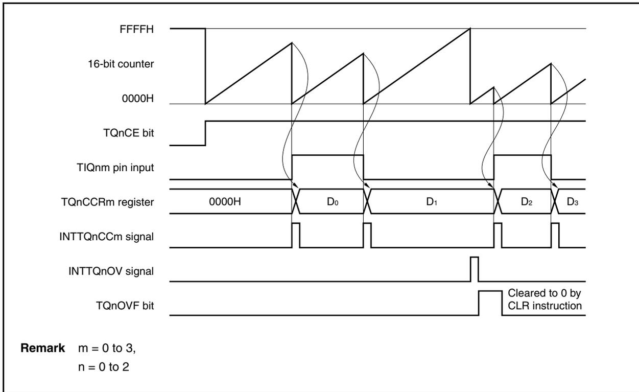
When the TQnCE bit is set to 1, the 16-bit counter starts counting. When the valid edge input to the TIQnm pin is later detected, the count value of the 16-bit counter is stored in the TQnCCRm register, the 16-bit counter is cleared to 0000H, and a capture interrupt request signal (INTTQnCCm) is generated.
