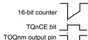
**Cautions** 1. Rewrite the TQnOLm and TQnOEm bits when the TQnCTL0.TQnCE bit = 0. (The same value can be written when the TQnCE bit = 1.) If rewriting was mistakenly performed, clear the TQnCE bit to 0 and then set the bits again.
