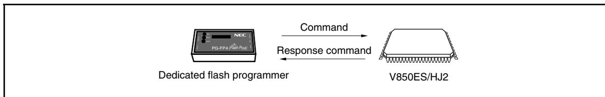
The following shows the commands for flash memory control in the V850ES/HJ2. All of these commands are issued from the dedicated flash programmer, and the V850ES/HJ2 performs the processing corresponding to the commands.
