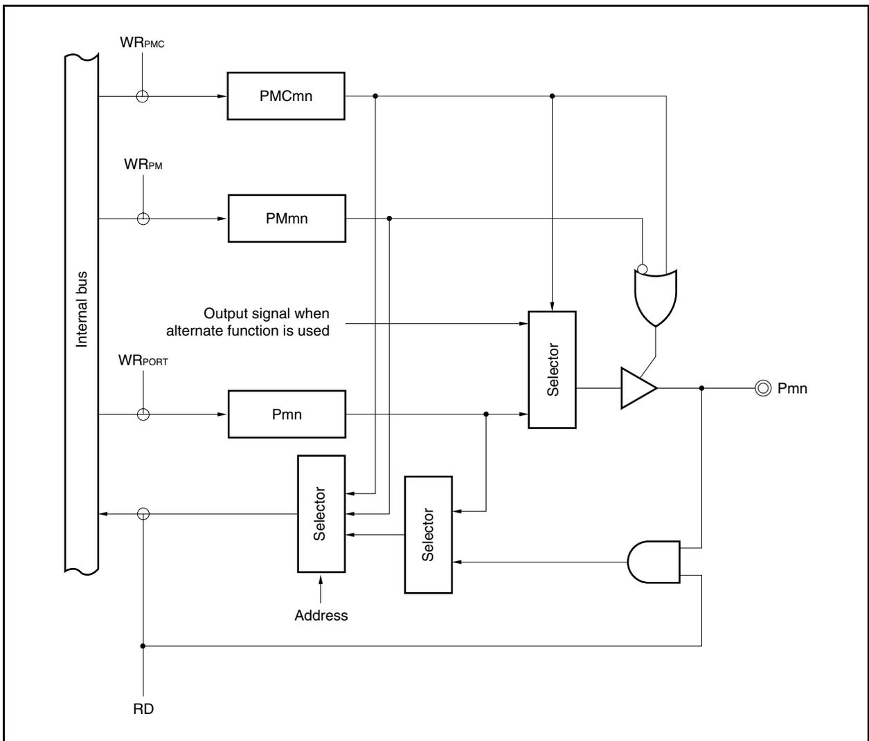
Figure 4-7. Block Diagram of Type D-3
