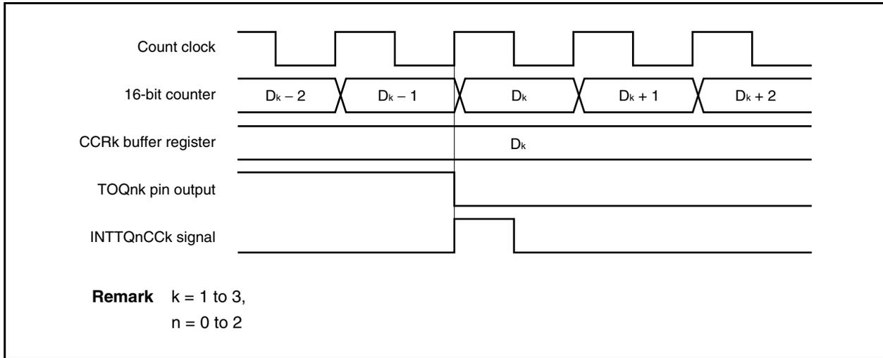
Usually, the INTTQnCCK signal is generated in synchronization with the next counting up after the count value of the 16-bit counter matches the value of the TQnCCRk register.
