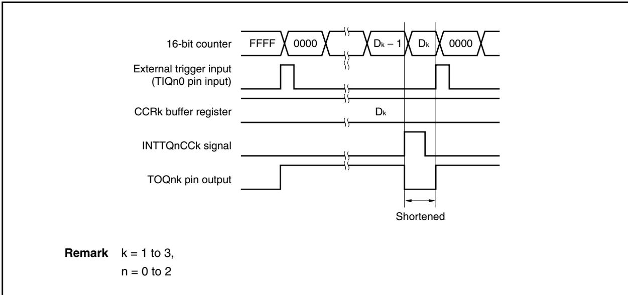
If the trigger is detected immediately before the INTTQnCCK signal is generated, the INTTQnCCK signal is not generated, and the 16-bit counter is cleared to 0000H and continues counting. The output signal of the TOQnk pin remains active. Consequently, the active period of the PWM waveform is extended.
