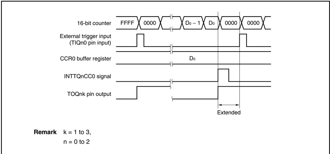
If the trigger is detected immediately before the INTTQnCC0 signal is generated, the INTTQnCC0 signal is not generated. The 16-bit counter is cleared to 0000H, the TOQnk pin is asserted, and the counter continues counting. Consequently, the inactive period of the PWM waveform is shortened.
