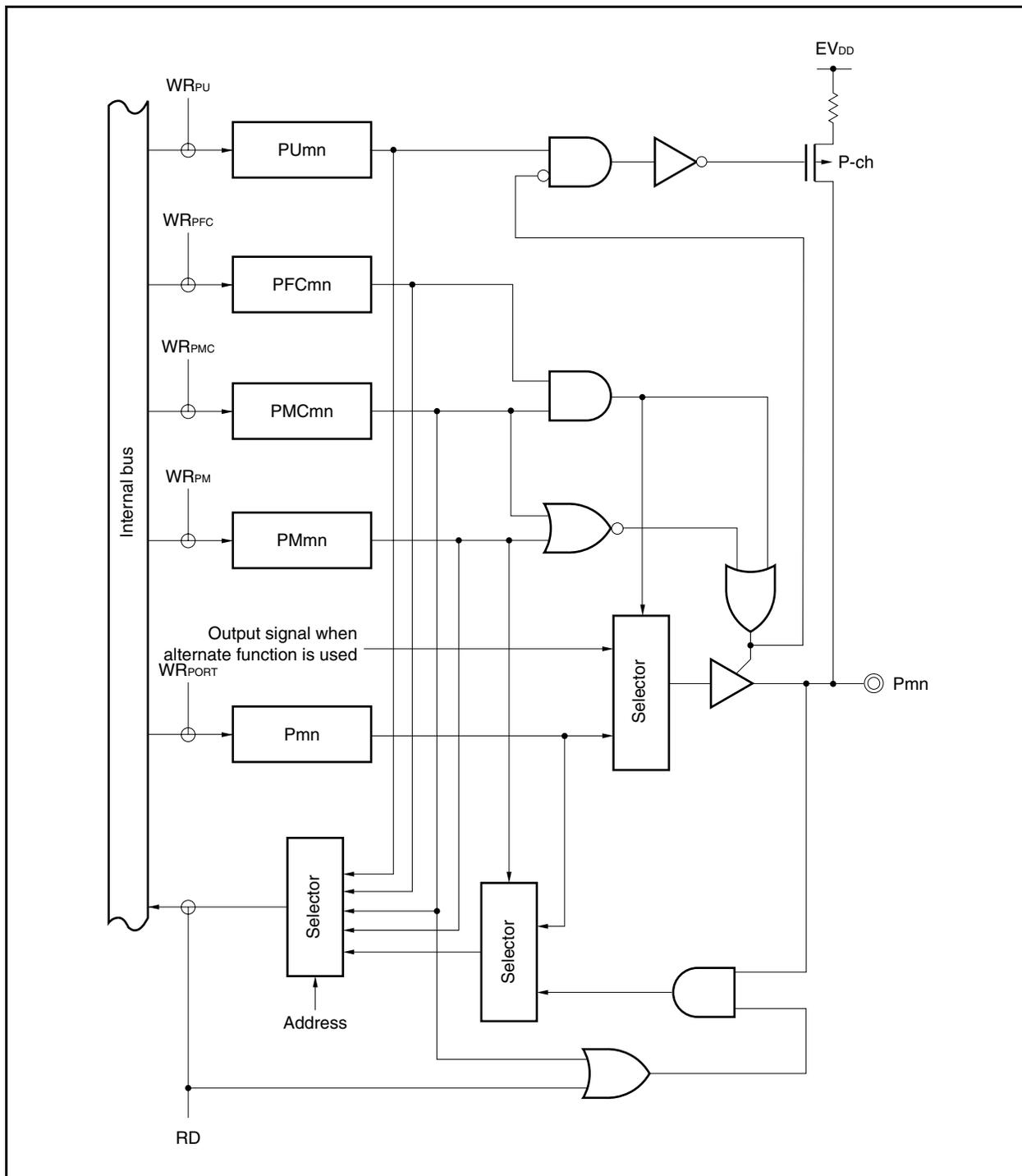
Figure 4-14. Block Diagram of Type G-4
