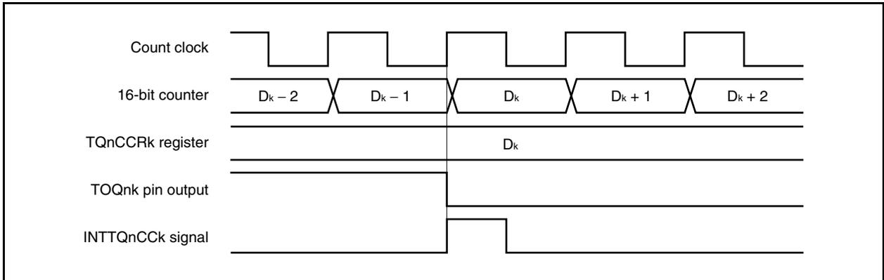
Usually, the INTTQnCCK signal is generated when the 16-bit counter counts up next time after its count value matches the value of the TQnCCRk register.
