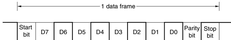
(c) 8-bit data length, MSB first, even parity, 1 stop bit, transfer data: 55H, TXDAn inversion
