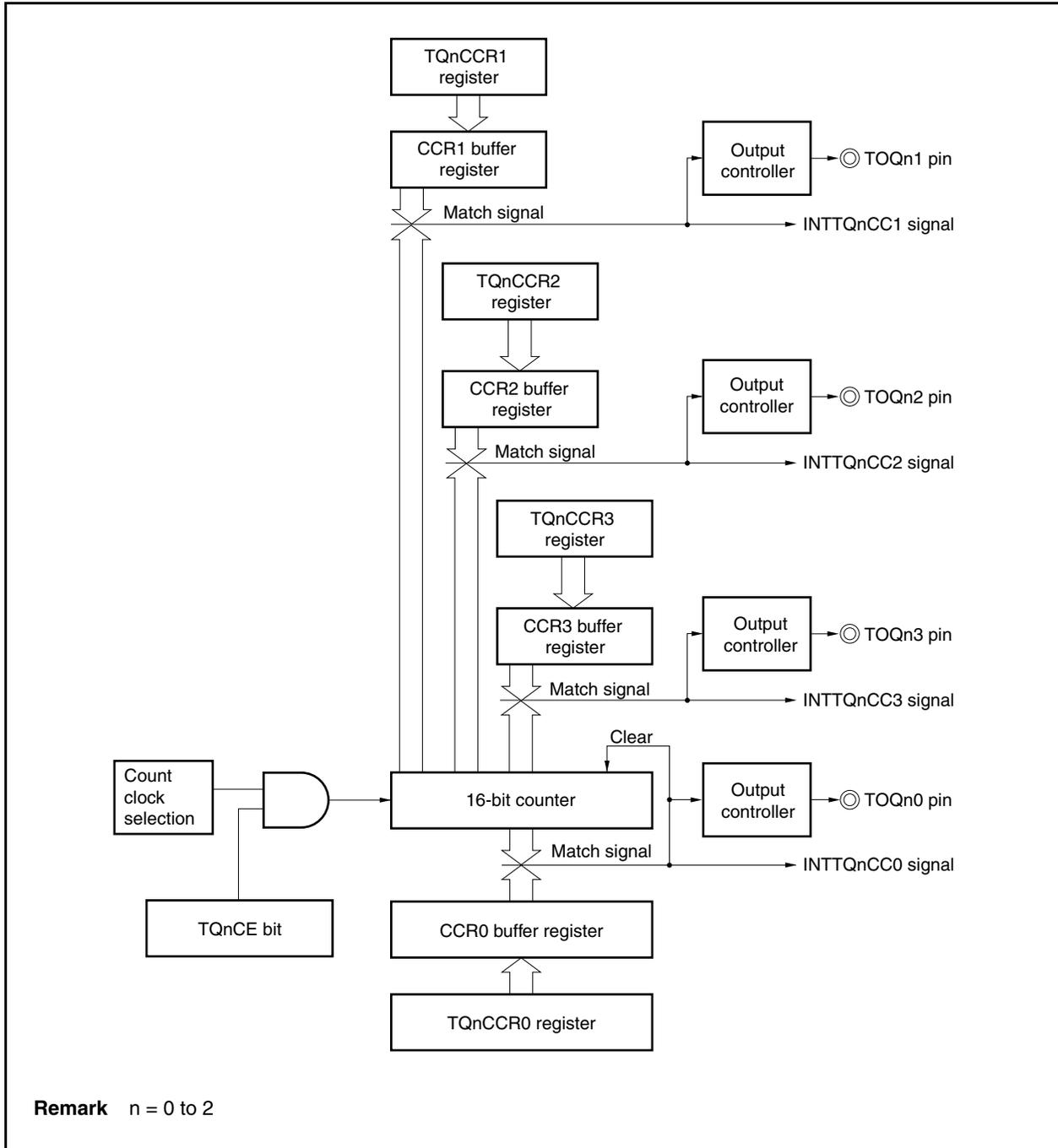
If the set value of the TQnCCRk register is less than the set value of the TQnCCR0 register, the INTTQnCCk signal is generated once per cycle. At the same time, the output of the TOPQnk pin is inverted.
