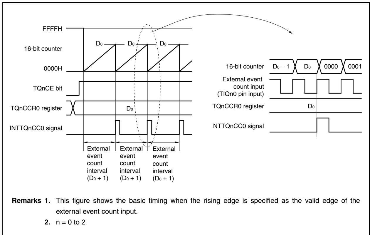
When the TQnCE bit is set to 1, the value of the 16-bit counter is cleared from FFFFH to 0000H. The counter counts each time the valid edge of external event count input is detected. Additionally, the set value of the TQnCCR0 register is transferred to the CCR0 buffer register.
