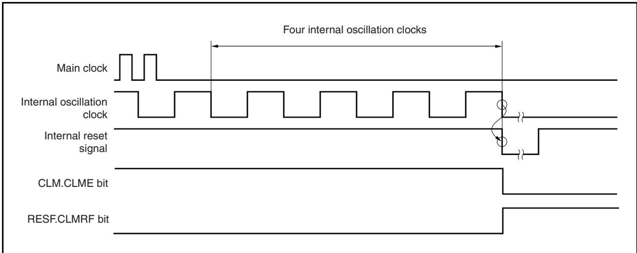
**(2) Clock monitor status after  $\overline{\text{RESET}}$  input**
