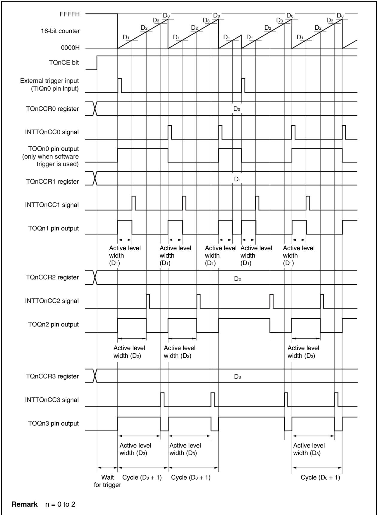
16-bit timer/event counter Q waits for a trigger when the TQnCE bit is set to 1. When the trigger is generated, the 16-bit counter is cleared from FFFFH to 0000H, starts counting at the same time, and outputs a PWM waveform from the TOQnk pin. If the trigger is generated again while the counter is operating, the counter is cleared to 0000H and restarted. (The output of the TOQn0 pin is inverted. The TOQnk pin outputs a high-level regardless of the status (high/low) when a trigger is generated.)
