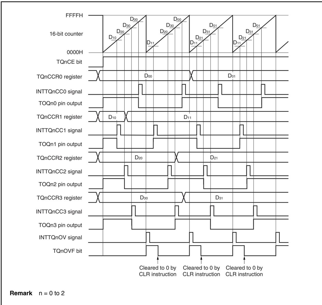
When the TQnCE bit is set to 1, the 16-bit counter starts counting. When the valid edge input to the TIQnm pin is detected, the count value of the 16-bit counter is stored in the TQnCCRm register, and a capture interrupt request signal (INTTQnCCm) is generated.
