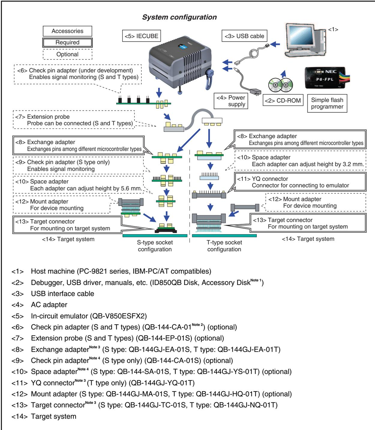
Figure A-2. System Configuration (When Using QB-V850ESFX2) (2/2)
