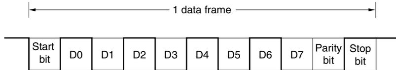
(b) 8-bit data length, MSB first, even parity, 1 stop bit, transfer data: 55H
