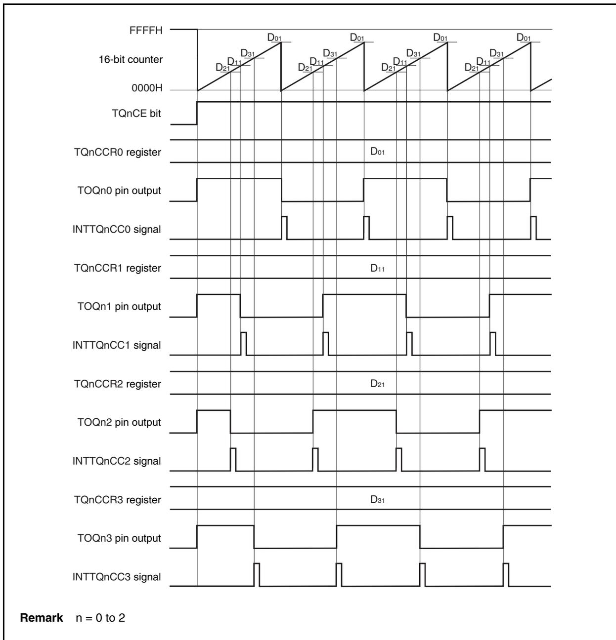
If the set value of the TQnCCRk register is greater than the set value of the TQnCCR0 register, the count value of the 16-bit counter does not match the value of the TQnCCRk register. Consequently, the INTTQnCCk signal is not generated, nor is the output of the TOQnk pin changed.
