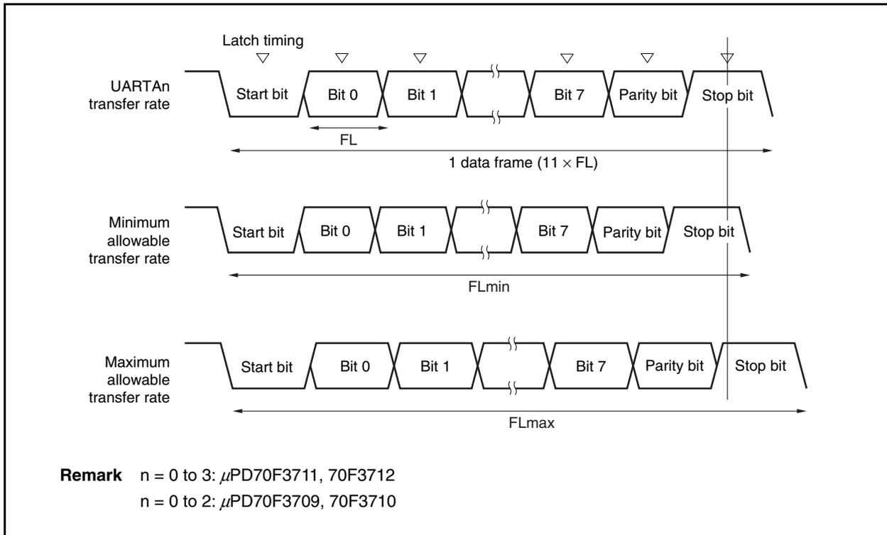
As shown in Figure 13-14, the receive data latch timing is determined by the counter set using the UAnCTL2 register following start bit detection. The transmit data can be normally received if up to the last data (stop bit) can be received in time for this latch timing.
