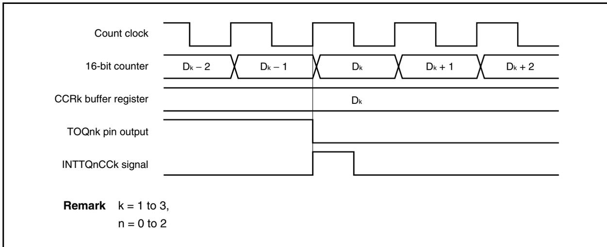
Usually, the INTTQnCCK signal is generated in synchronization with the next count up after the count value of the 16-bit counter matches the value of the CCRk buffer register.
