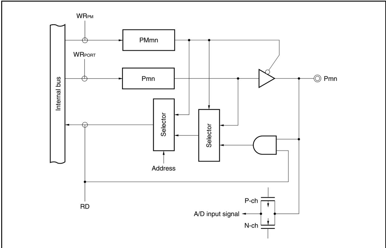
Figure 4-3. Block Diagram of Type B-1
