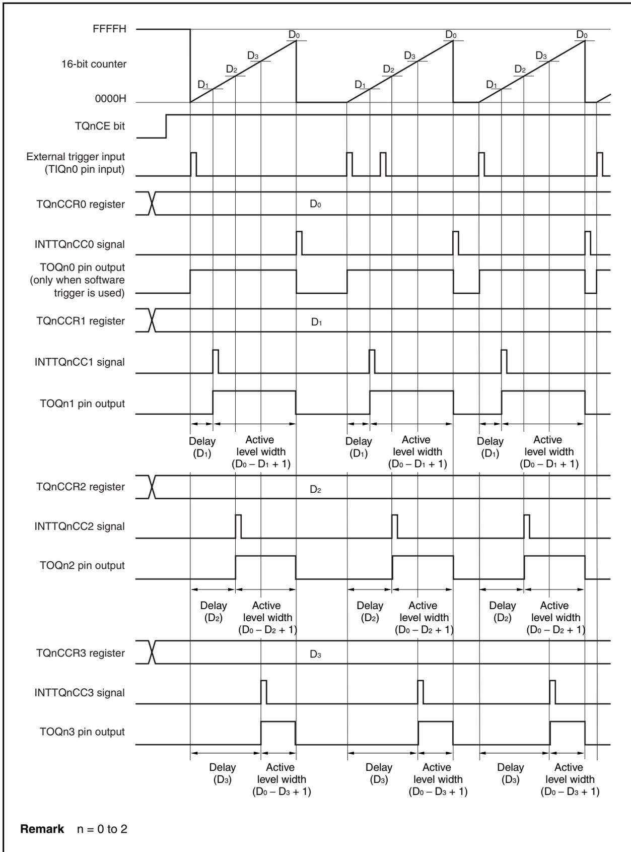
When the TQnCE bit is set to 1, 16-bit timer/event counter Q waits for a trigger. When the trigger is generated, the 16-bit counter is cleared from FFFFH to 0000H, starts counting, and outputs a one-shot pulse from the TOQnk pin. After the one-shot pulse is output, the 16-bit counter is set to FFFFH, stops counting, and waits for a trigger. If a trigger is generated again while the one-shot pulse is being output, it is ignored.
